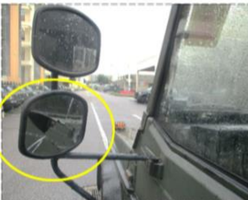
Damage Assessment: Left blind-spot mirror cracked.
