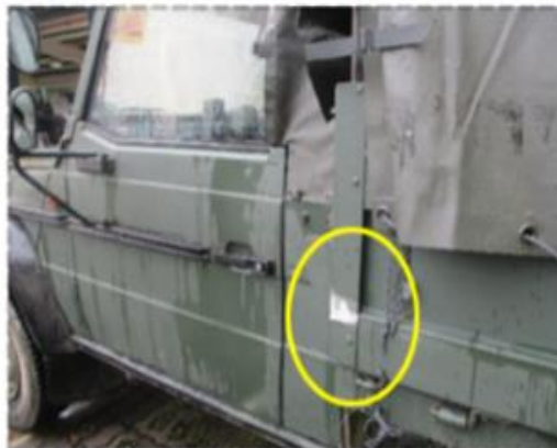
Damage Assessment: Left front of the vehicle sideboard scratched.
