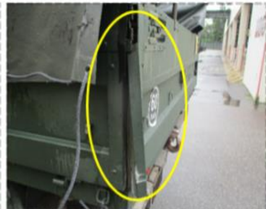
Damage Assessment: Left side of the vehicle tailboard was dented.
