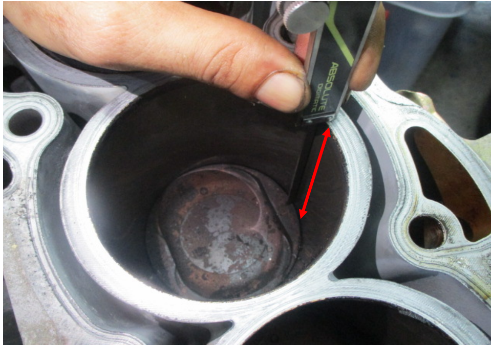
Photo 13 shows measurement of the stroke (arrowed) for cylinder 2 of the Toyota engine that I had inspected. The bore and stroke measurements of the Toyota engine were carried out using a digital Vernier Caliper that was calibrated before the start of the measurements.
