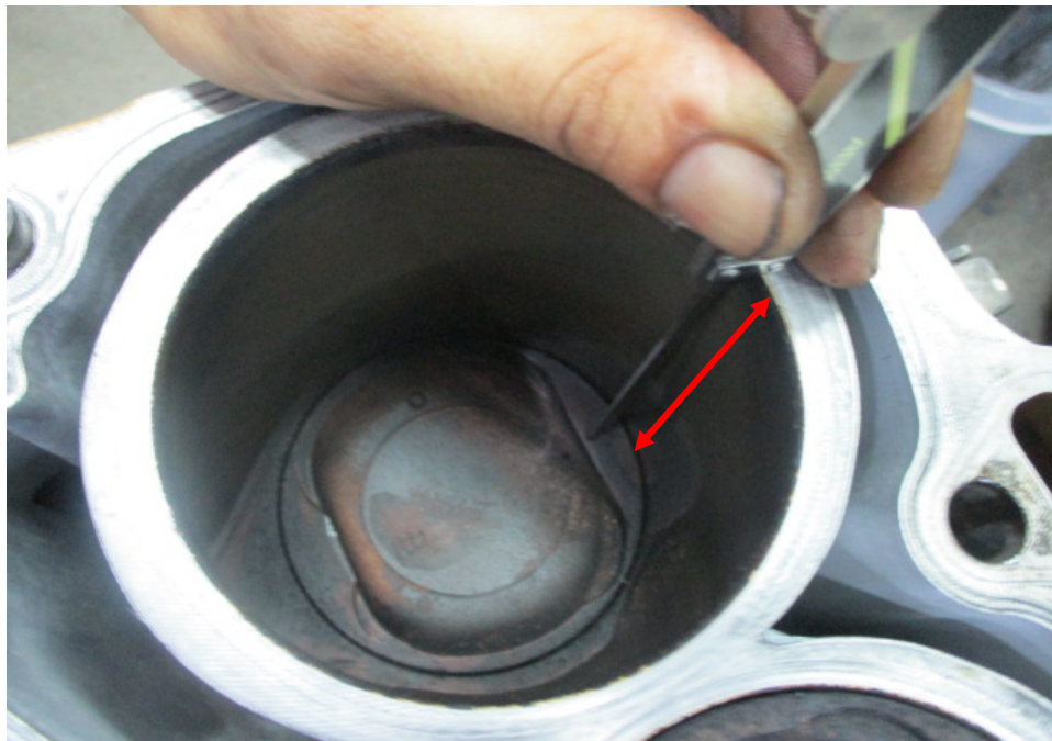
Photo 10 shows measurement of the stroke (arrowed) for cylinder 1 of the Toyota engine that I had inspected. The bore and stroke measurements of the Toyota engine were carried out using a digital Vernier Caliper that was calibrated before the start of measurements.
