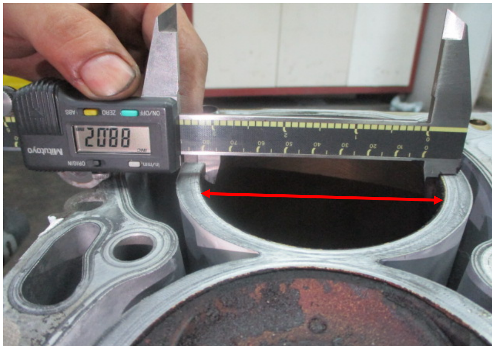
Photo 8 shows measurement being carried out to the bore (arrowed) of cylinder 1 of the Toyota engine, which was recorded to be 88.02mm.
