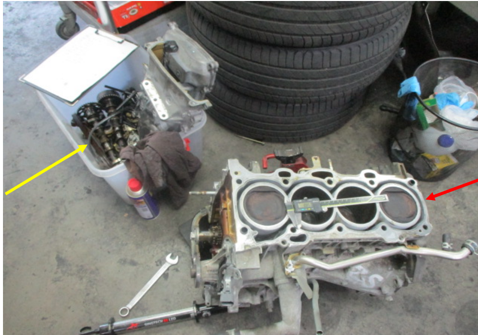
Photo 5 shows the top block (yellow arrow) of the Toyota engine separated from its bottom block (red arrow). This was to enable me to carry out measurements of its cylinders, in particular the bore and stroke measurements of each cylinder, which typically can be used to determine the engine displacement or more commonly referred to as engine cc.
