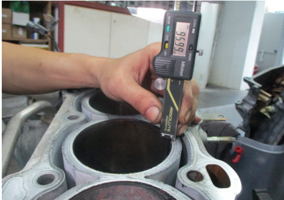
Photo 17 shows the stroke measurement of cylinder 3, which was recorded to be 95.99mm.
