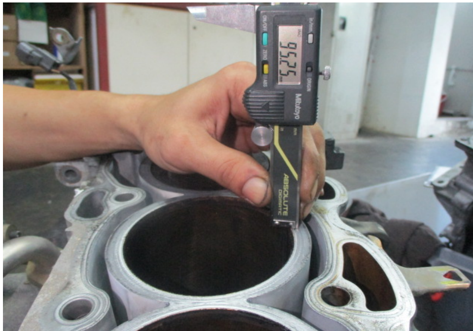
Photo 14 shows the stroke measurement of cylinder 2, which was recorded to be 95.25mm.
