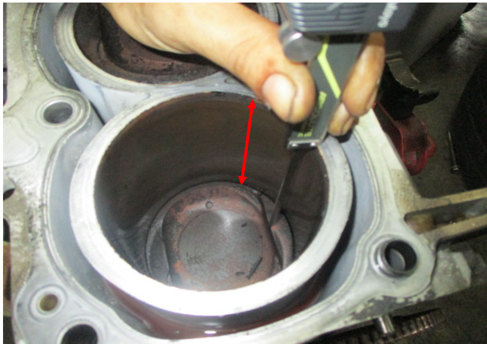
Photo 20 shows measurement being carried out to the stroke (arrowed) of cylinder 4 of the Toyota engine. The bore and stroke measurements of the Toyota engine were carried out using a digital Vernier Caliper that was calibrated prior to the start of measurements.
