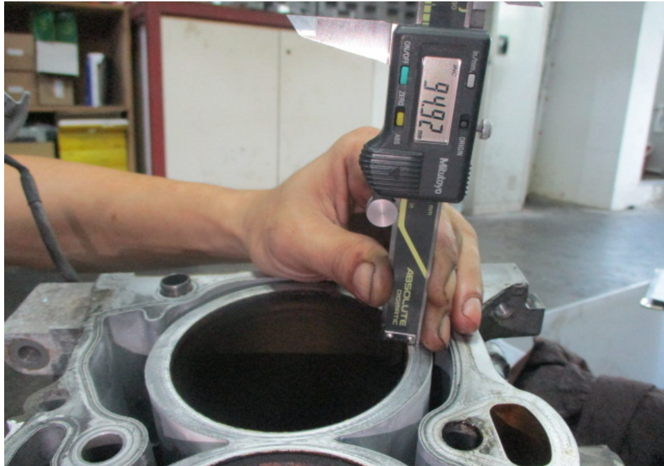
Photo 11 shows the stroke measurement of cylinder 1, which was recorded to be 94.92mm.
