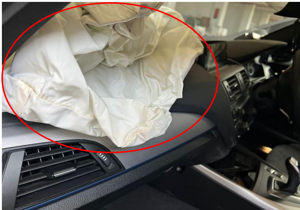
Photo 6 shows the close up view of the interior portion of the Insured Vehicle at the time of our inspection. Its airbag's deployed (circled) as a result of the accident.
