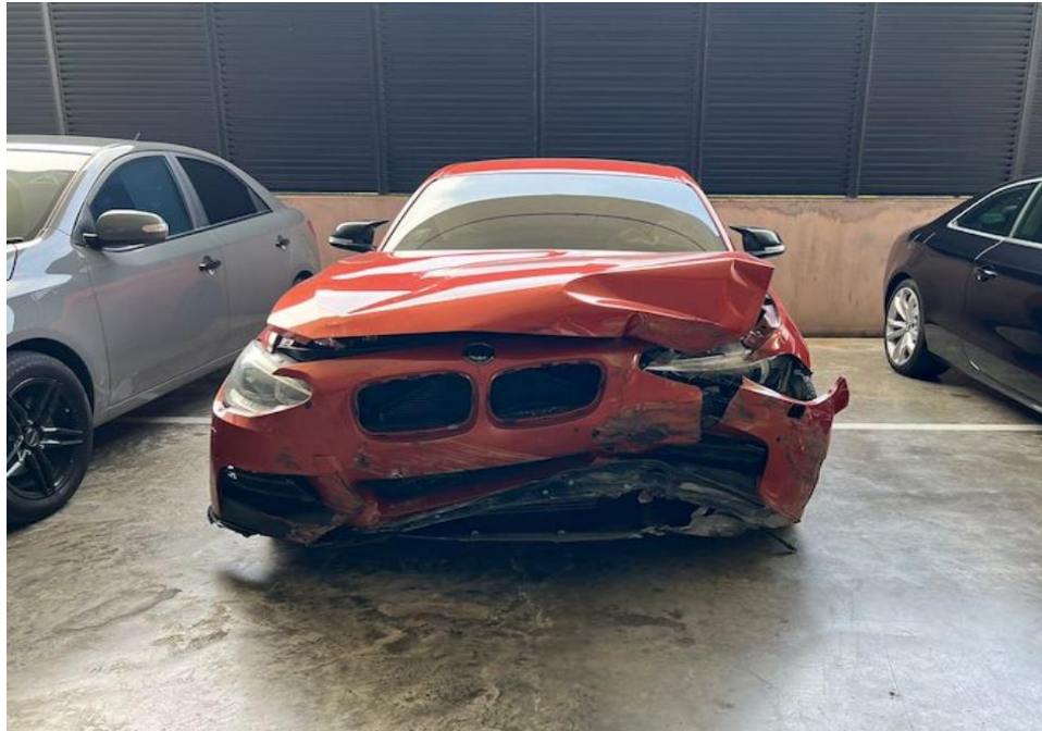
Photo 3 shows the general view of the front portion of the Insured Vehicle at the time of our inspection. Its front bonnet, front left headlamp and front bumper, was amongst the body parts that were damaged as a result of the accident.
