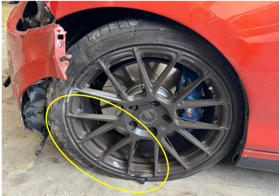
Photo 5 shows the close up view of the front left tyre of the Insured Vehicle at the time of our inspection. Its front left tyre and wheel rim (circled) were damaged as a result of the accident.
