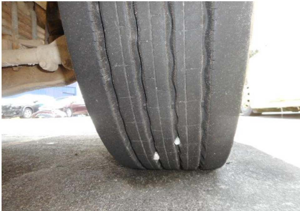
Photo 7 shows the condition of the front right tyre of the Tipper Truck, which was observed to be in serviceable condition with remaining tread depth of approximately 11.7mm. The tyre, which was wrapped around standard steel wheel rim, was also observed to be sufficiently inflated for vehicular operation. There was no tear, cut or burst mark(s) on the outer and the inner sidewalls as well as across the tread of the 6 tyres that were fitted on the Tipper Truck.
