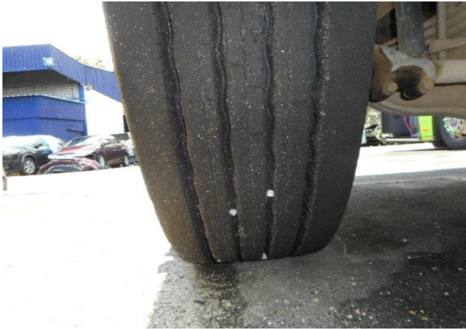
Photo 10 shows the condition of the front left tyres of the Tipper Truck, which were observed to be in serviceable condition with remaining tread depth of approximately 11.3mm. There was also no tear, cut or burst mark(s) on the outer and the inner sidewalls as well as across the tread of the 6 tyres that were fitted on the Tipper Truck.
