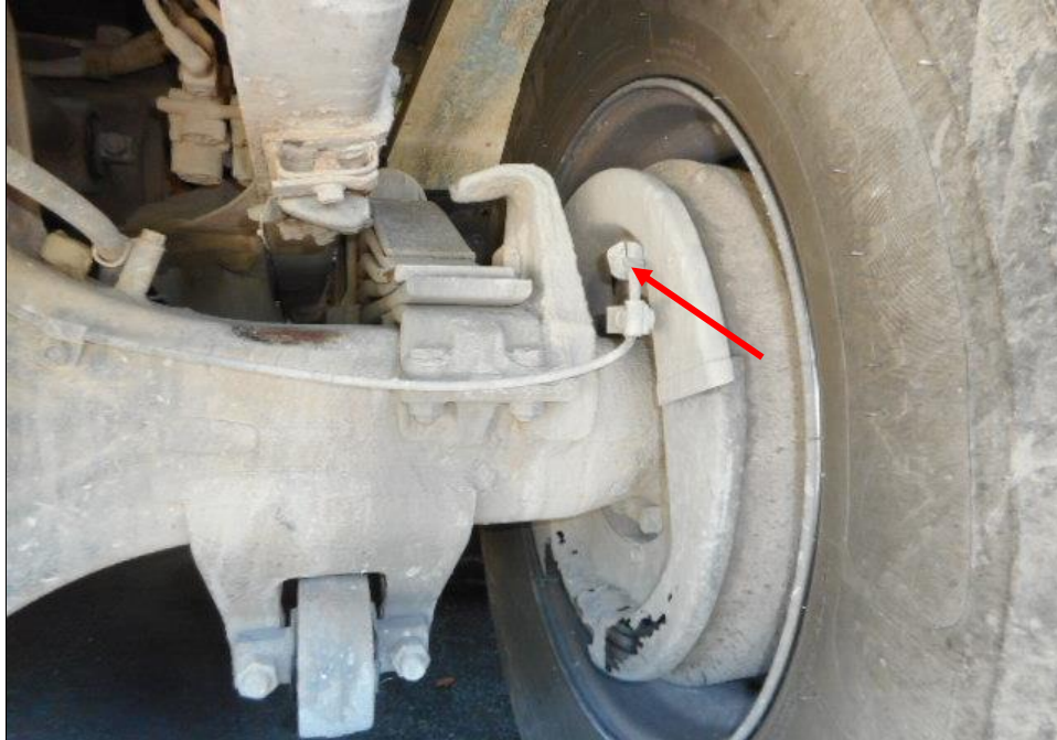
Photo 18 shows the brake pipe (arrowed) at the rear left wheel of the Tipper Truck. I did not observe any leakage of brake fluid at the time of my inspection of the Tipper Truck. My static tests of the Tipper Truck's braking system, along with my visual examination of the various mechanical components in the braking system, had indicated that there was no internal leakage of pressure/vacuum. Hence the braking system of the Tipper Truck was likely to be in serviceable condition at the material time of accident.
