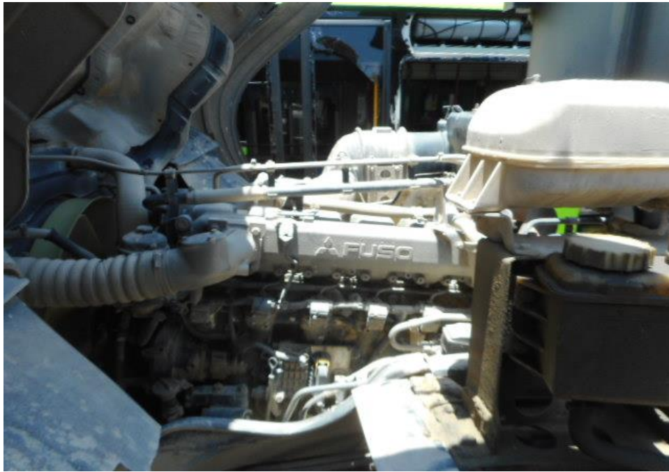
Photo 11 shows a general view of the Tipper Truck's engine compartment, which was accessed by lifting the front cabin of the Tipper Truck. The various parts and components inside the engine compartment were unaffected by the accident. There was also no sign(s) or indication(s) of fresh fluid leakage and/or fluid stain within the engine compartment
