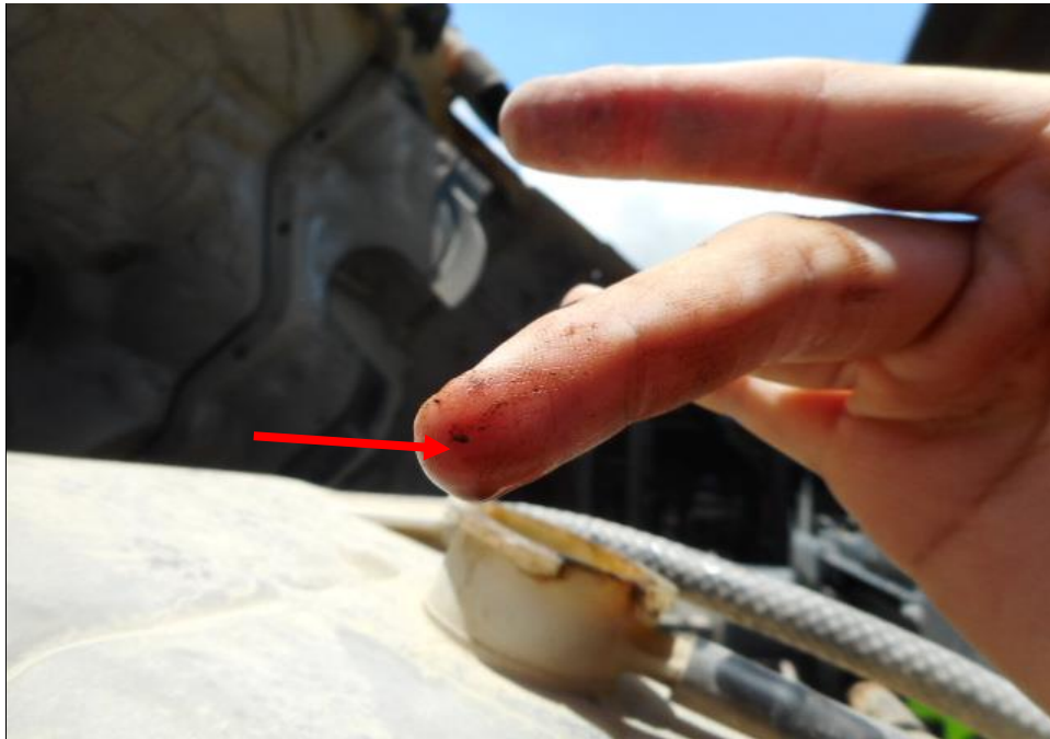
Photo 13 shows the engine coolant reservoir of the Tipper Truck at the time of my inspection. The engine coolant was observed to be of sufficient level (arrowed) and without any visible contamination.
