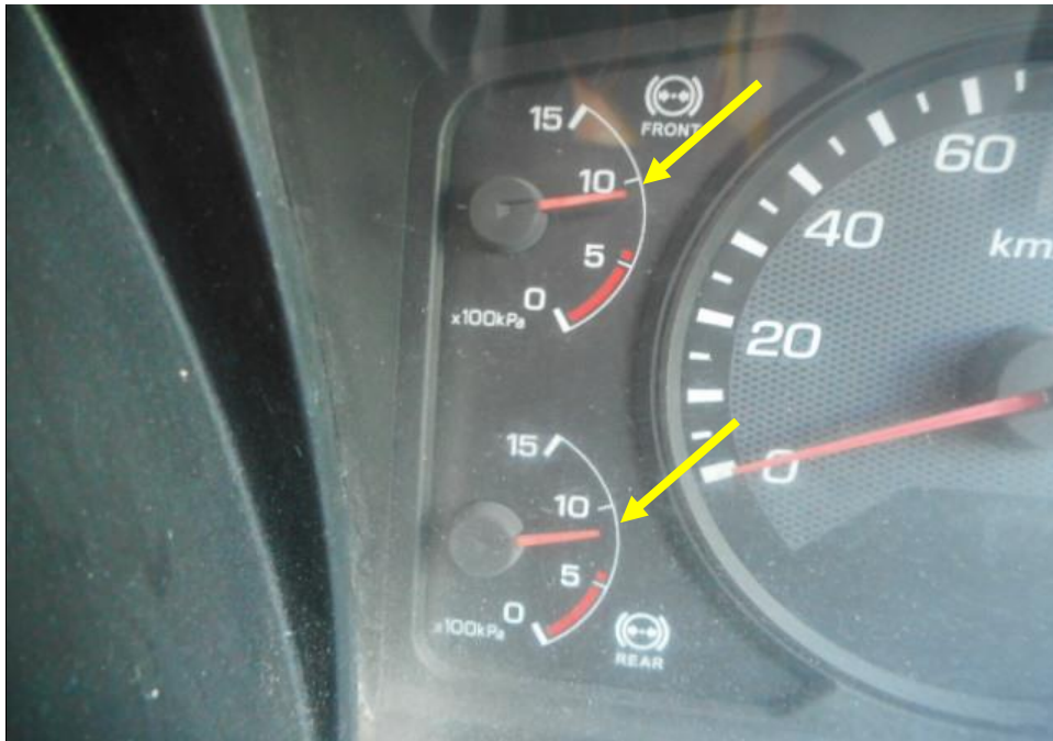
Photo 12 shows the air in the air brake cylinders of the Tipper Truck at the time of my inspection. The air in the cylinder was observed to be of sufficient level & serviceable at the time of the accident.
