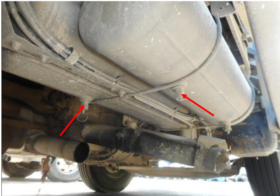
Photo 21 shows the air brake cylinders (arrowed) at the undercarriage of the Tipper Truck. I did not observe any leakage of air brake fluid at the time of my inspection of the Tipper Truck. My static tests of the Tipper Truck's braking system, along with my visual examination of the various mechanical components in the braking system had indicated that there was no internal leakage of pressure/vacuum. Hence the braking system of the Tipper Truck was likely to be in serviceable condition at the material time of accident.
