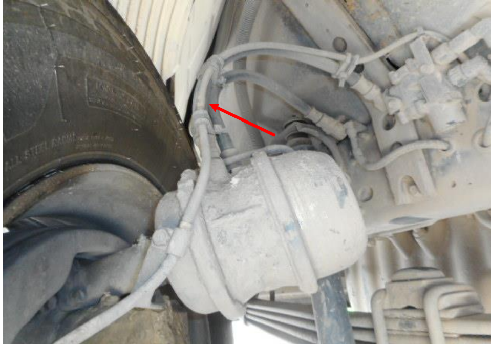
Photo 20 shows the brake pipe (arrowed) at the front left wheel of the Tipper Truck. I did not observe any leakage of brake fluid at the time of my inspection of the Tipper Truck. My static tests of the Tipper Truck's braking system, along with my visual examination of the various mechanical components in the braking system had indicated that there was no internal leakage of pressure/vacuum. Hence the braking system of the Tipper Truck was likely to be in serviceable condition at the material time of accident.
