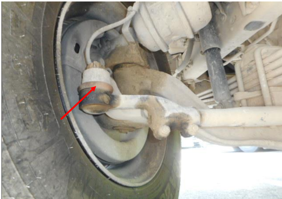
Photo 23 shows the various undercarriage components at the front left wheel of the Tipper Truck, in particular the steering tie rod end (arrowed). The various undercarriage components of the Tipper Truck were all found to be intact without any visible damage. There was also no sign of fluid stain(s) observed on the various undercarriage components.
