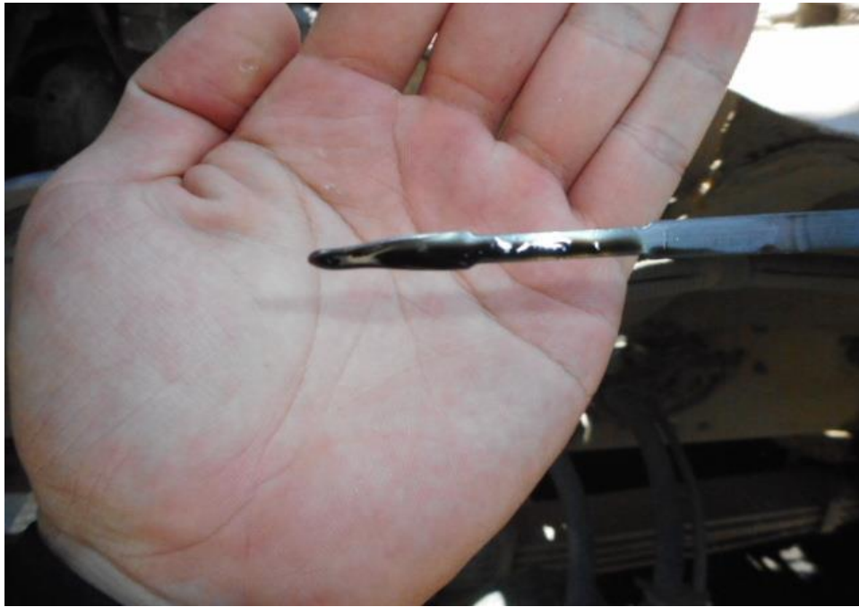
Photo 15 shows the engine oil dip stick of the Tipper Truck at the time of my inspection. The engine oil was observed to be of insufficient level at the time of our inspection.
