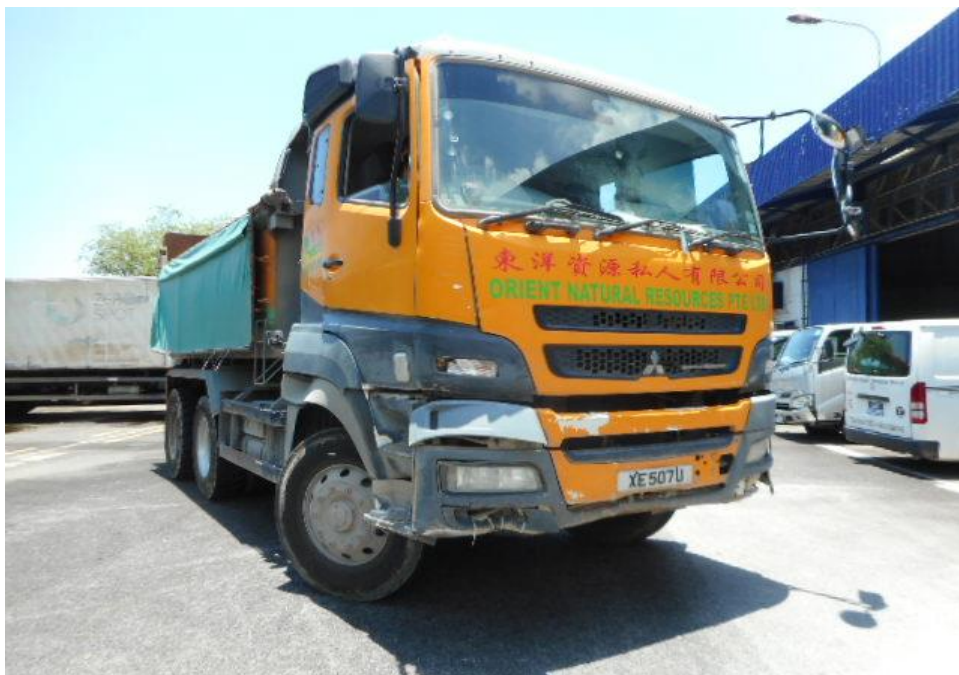
Photo 25 shows the front right wheel of the Tipper Truck turned to its full left. During my steering system test, I did not experience any abnormal free play and/or resistance when I had turned the steering wheel towards full left and full right. This would suggest that the steering system of the Tipper Truck was likely to be in serviceable condition at the material time of accident.
