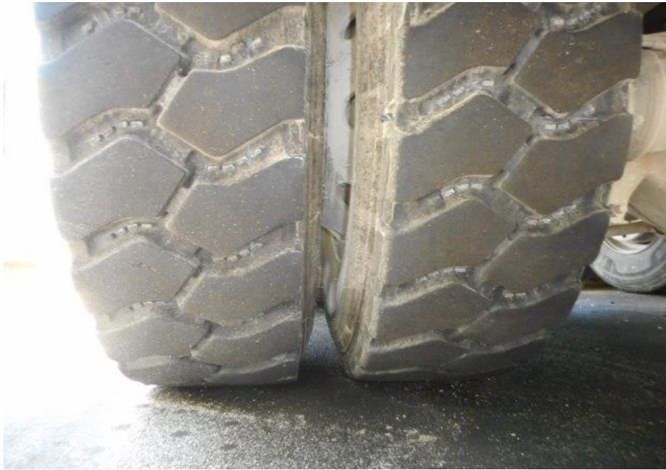
Photo 8 shows the condition of the rear right tyre of the Tipper Truck, which was observed to be in serviceable condition with remaining tread depth of approximately 14.1mm. The tyre, which was wrapped around standard steel wheel rim, was also observed to be sufficiently inflated for vehicular operation.
