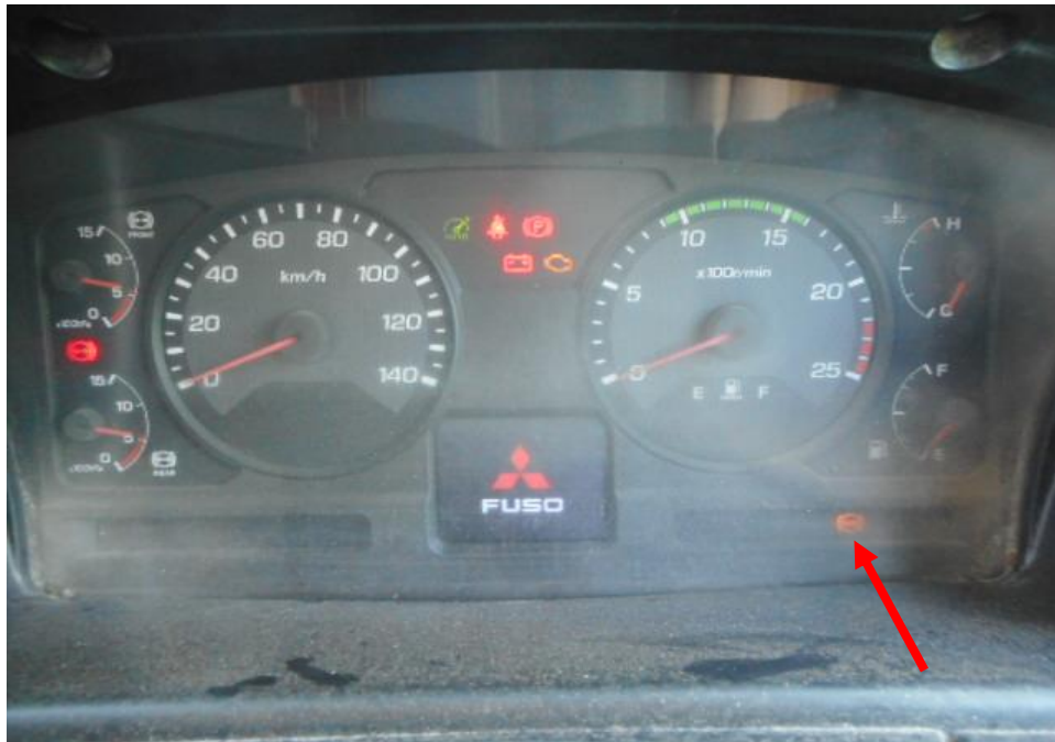
Photo 26 shows the warning light for Anti-Lock Brake System (ABS) (arrowed) appearing on the instrument panel of the Tipper Truck during the self-test of its various electronic operating systems when its engine was cranked.
