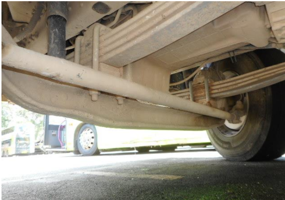
Photo 16 shows the undercarriage of the Tipper Truck, at the area where the engine housing located. I did not find any sign(s) or indication(s) of fluid leak, however old fluid stain(s) was observed on the underside of the Tipper Truck.
