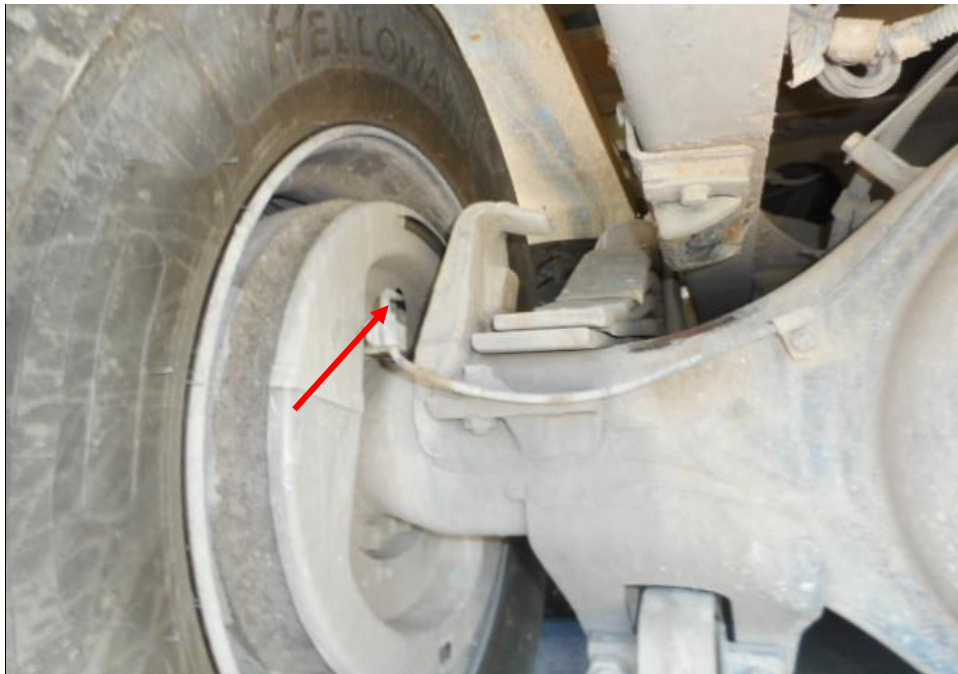
Photo 17 shows the brake pipe (arrowed) at the rear right wheel of the Tipper Truck. I did not observe any leakage of brake fluid at the time of my inspection of the Tipper Truck. My static tests of the Tipper Truck's braking system, along with my visual examination of the various mechanical components in the braking system, had indicated that there was no internal leakage of pressure/vacuum. Hence the braking system of the Tipper Truck was likely to be in serviceable condition at the material time of accident.
