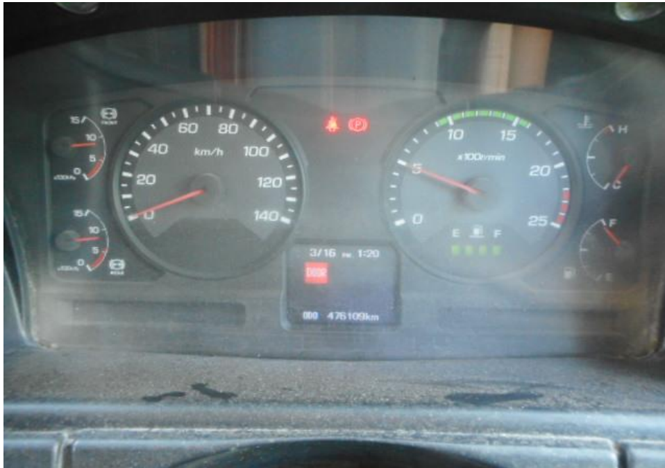
Photo 27 shows no warning lights illuminated on the instrument panel of the Tipper Truck after the engine was cranked. This would suggest that there was no abnormality to the electronic operating system of the Tipper Truck, like the ABS, and etc.
