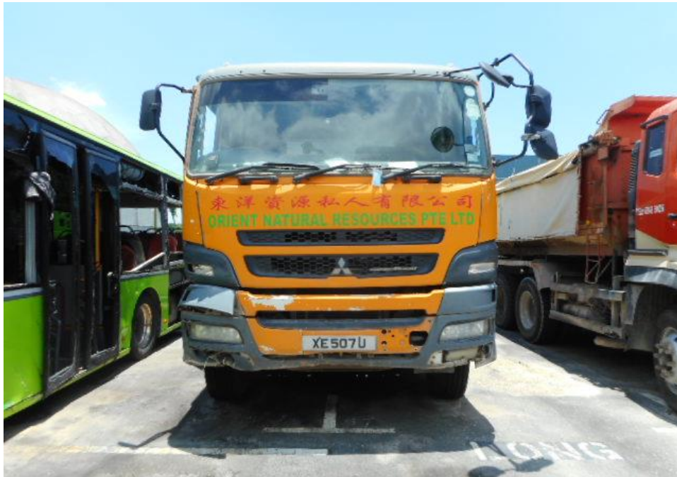
Photo 2 shows a general view of the front body of the Tipper Truck at the time of my inspection. The front portion of the Tipper Truck was observed to sustained damage at the time of inspection. Its front bumper and front right headlamp was amongst the body parts that were damaged as a result of the accident.
