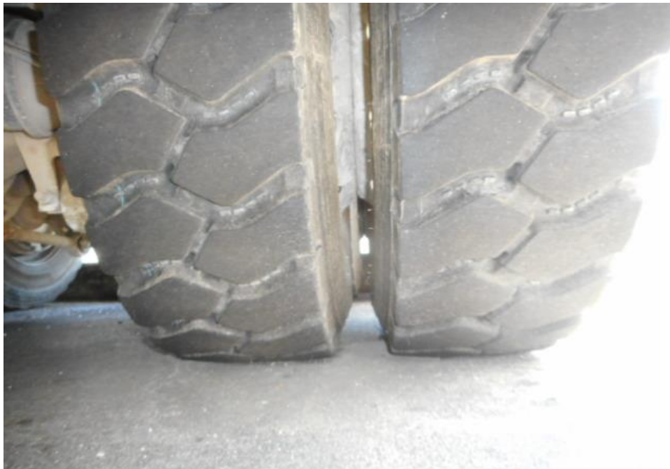
Photo 9 shows the condition of the rear left tyres of the Tipper Truck, which was observed to be in serviceable condition with remaining tread depth of approximately 14.4mm. The tyres, which were wrapped around standard steel wheel rim, were also observed to be sufficiently inflated for vehicular operation. There was also no damage found on all 6 steel wheel rims of the Tipper Truck.
