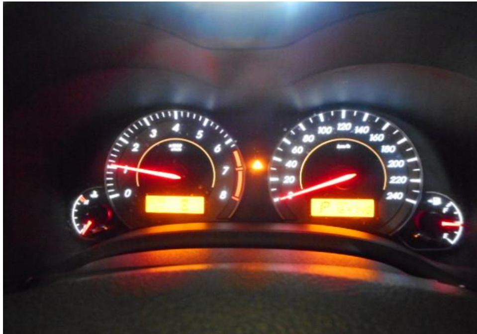
Photo 25 shows no warning lights illuminated on the instrument panel of the Motor Car after the engine was cranked. This would suggest that there was no abnormality to the electronic operating system of the Motor Car, like the ABS and SRS etc.
