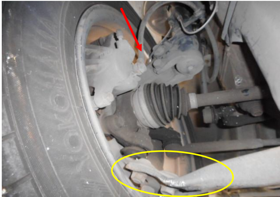
Photo 19 shows the brake hose/pipe (arrowed) at the front right wheel of the Motor Car. I did not observe any leakage of brake fluid at the time of my inspection of the Motor Car. Static tests of the Motor Car's braking system had indicated that there was no internal leakage of pressure/vacuum. I observed that the front right lower arm (circled) was damaged and bent as a result of the accident.
