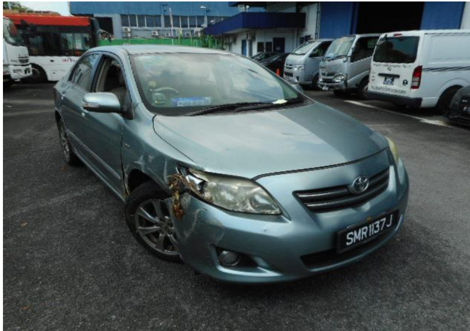
Photo 21 shows the front right wheel of the Motor Car turned to its full left. During my steering system test, I experience abnormal resistance when I had turned the steering wheel towards the left and right due to the damaged front right lower arm as a result of the accident. However, the Motor Car was still able to be driven.
