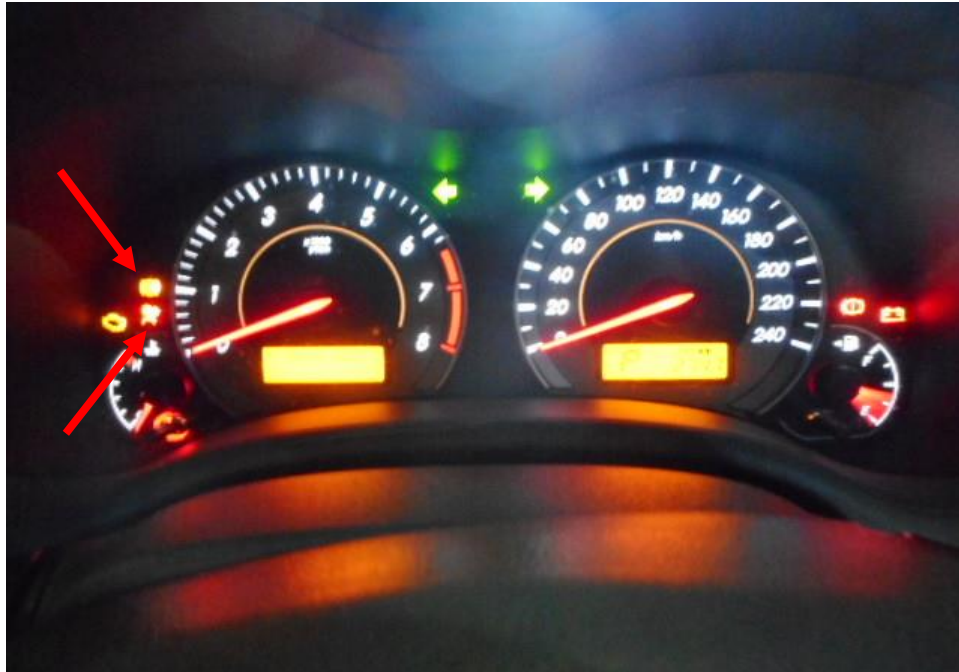
Photo 24 shows the warning light for Anti-Lock Brake System (ABS) and Supplemental Restraint System (SRS) (arrowed) appearing on the instrument panel of the Motor Car during the self-test of its various electronic operating systems when its engine was cranked.
