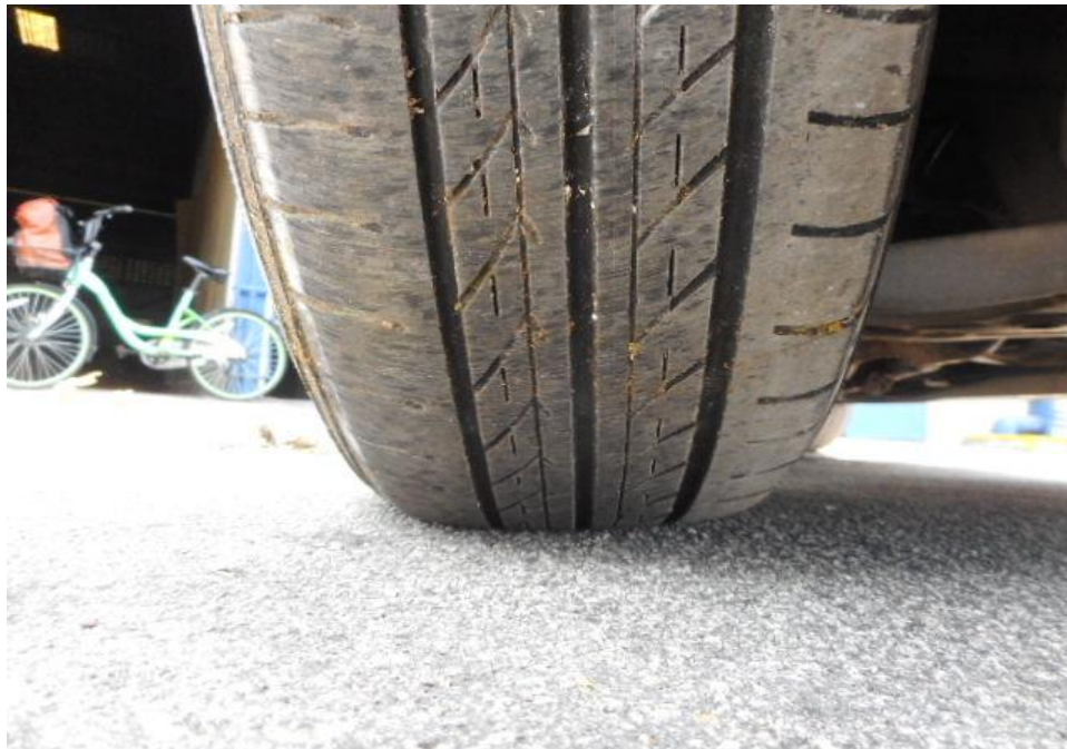
Photo 8 shows the condition of the front right tyre of the Motor Car, which was observed to be in serviceable condition with remaining tread depth of approximately 3.4mm. The tyre was sufficiently inflated for vehicular operation with no tear, cut or burst mark(s) on the outer and the inner sidewalls as well as across the tread. The 4 tyres of the Motor Car were wrapped around standard steel wheel rims without any damage.
