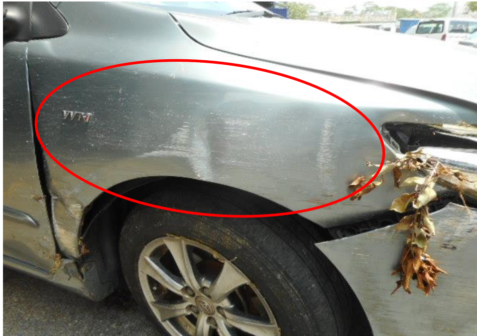
Photo 4 shows a close up view of the Motor Car's front body at the time of my inspection. The front portion of the Motor Car was observed to have sustained damage. Its front right fender (circled) was the body parts that were damaged as a result of the accident.
