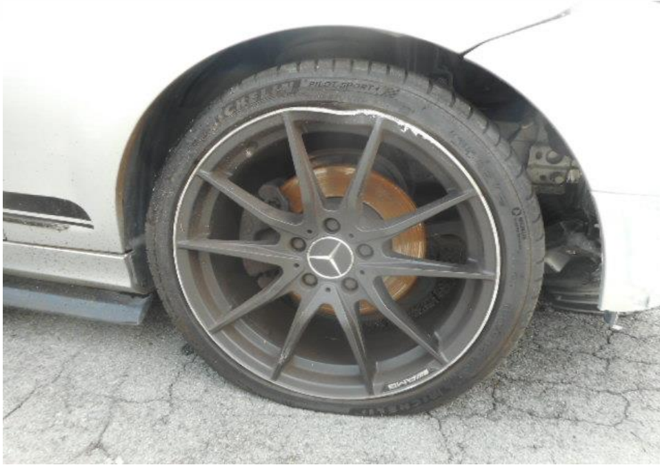
Photo 8 shows the condition of the front right tyre of the Motor Car, which was observed to be in serviceable condition with remaining tread depth of approximately 4.9mm. The tyre was sufficiently inflated for vehicular operation with no tear, cut or burst mark(s) on the outer and the inner sidewalls as well as across the tread. However, the wheel rim was observed to be damaged as a result of the accident.
