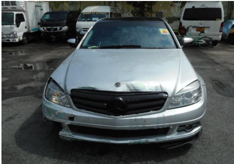
Photo 3 shows a general view of the Motor Car's front body at the time of my inspection. The Motor Car was observed to have sustained damage at its front portion. Its front bonnet, front bumper as well as its front grille were amongst the body parts that were damaged as a result of the accident.
