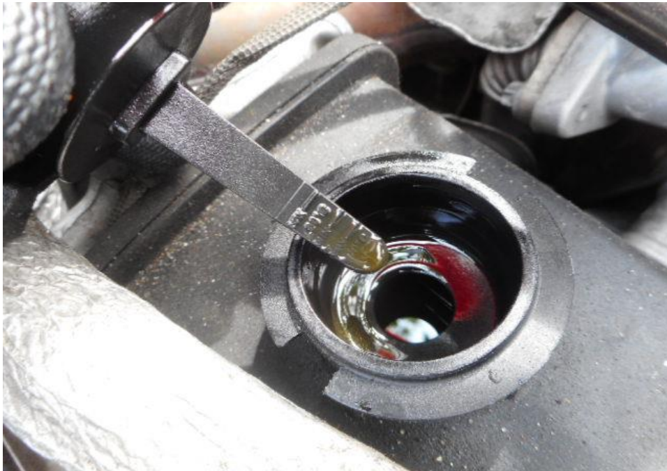
Photo 17 shows the power steering fluid dipstick of the Motor Car at the time of my inspection. The steering fluid was observed to be of sufficient level and without any visible contamination.
