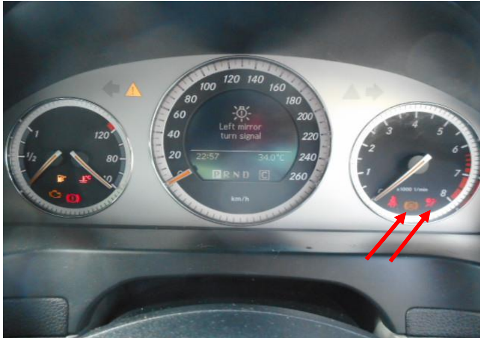
Photo 27 shows the warning light for Anti-Lock Brake System (ABS), and Supplemental Restraint System (SRS) (arrowed) appearing on the instrument panel of the Motor Car during the self-test of its various electronic operating systems when its engine was cranked.
