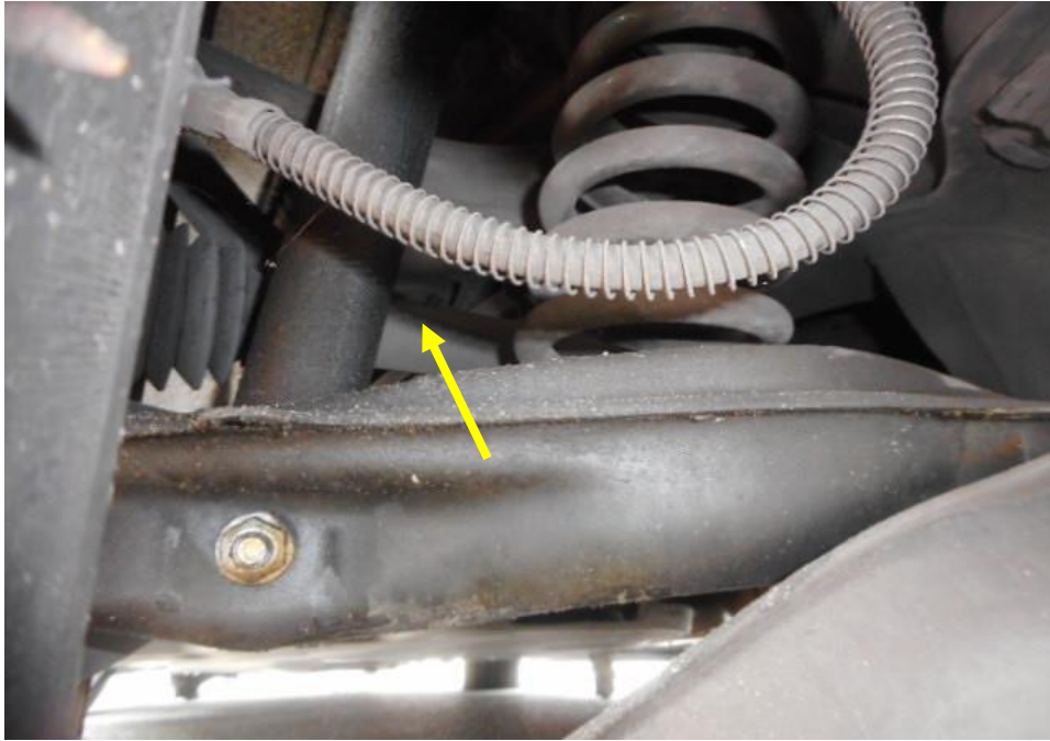
Photo 26 shows the various undercarriage components at the rear left wheel of the Motor Car, in particular the drive shaft (arrowed). The components were all found to be intact, suggesting that the steering system of the Motor Car was likely to be in serviceable condition at the material time of accident. There was also no sign of fluid stain observed on the various undercarriage components at the front right wheel of the Motor Car.
