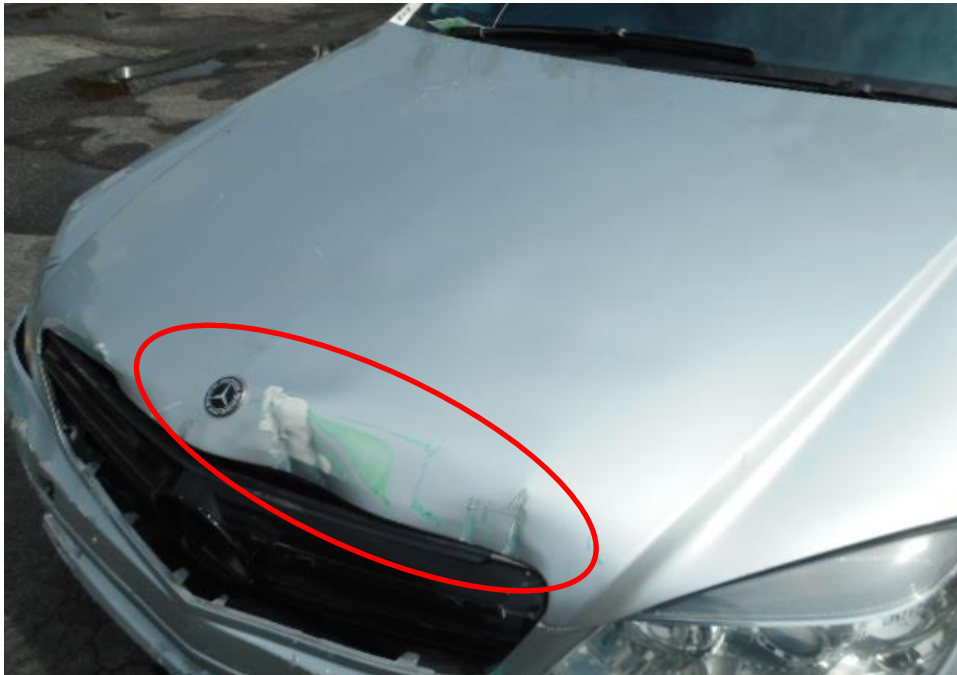
Photo 4 shows a close up view of the Motor Car's front body at the time of my inspection. The front portion of the Motor Car was observed to have sustained damage. Its front bonnet (circled) was the body parts that were damaged as a result of the accident.
