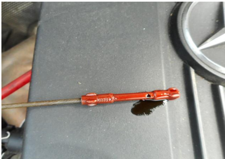
Photo 16 shows the engine oil dipstick of the Motor Car at the time of my inspection. The engine oil was observed to be of sufficient level and without any visible contamination.
