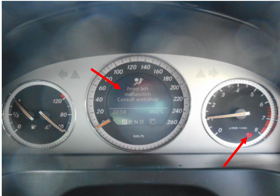
Photo 28 shows only the Supplemental Restraint System (SRS) remained illuminated up, the fault was a pre-existing fault. There was no other warning lights illuminated on the instrument panel of the Motor Car after the engine was cranked. This would suggest that there was no abnormality to the electronic operating system of the Motor Car, like the ABS and etc.
