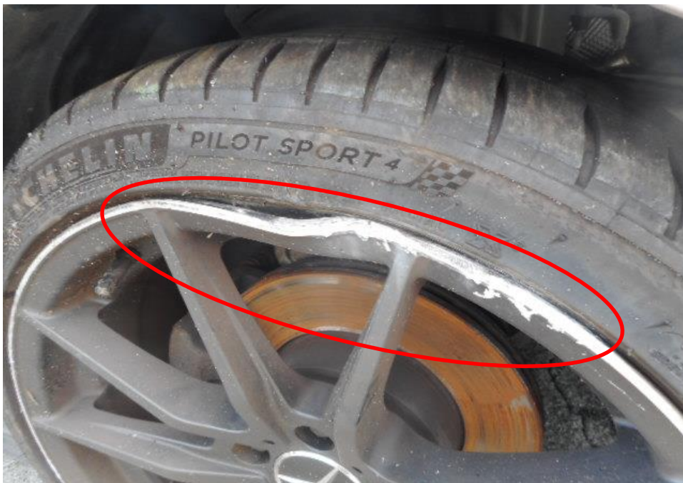
Photo 9 shows the close up condition of the front right tyre wheel rim (circled) of the Motor Car which was observed to be damaged as a result of the accident.
