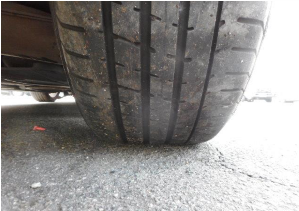
Photo 10 shows the condition of the rear right tyre of the Motor Car, which was observed to be in serviceable condition with remaining tread depth of approximately 4.4mm. The tyre was also observed to be sufficiently inflated for vehicular operation with no tear, cut or burst mark(s).
