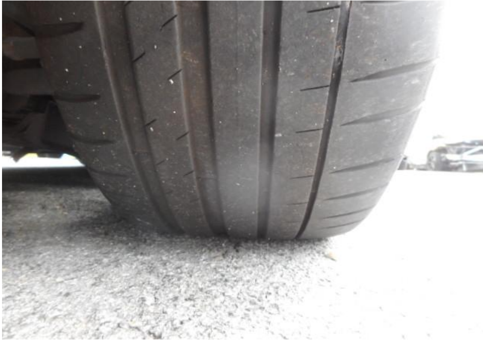
Photo 12 shows the condition of the front left tyre of the Motor Car, which was observed to be in serviceable condition with remaining tread depth of approximately 4.7mm. There was also no tear, cut or burst mark(s) on the outer and the inner sidewalls as well as across the tread of the Motor Car's 4 tyres.
