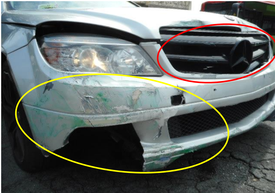
Photo 5 shows a close up view of the Motor Car's front body at the time of my inspection. The front portion of the Motor Car was observed to have sustained damage. Its front bumper (yellow circle) and front grille (red circle) was the body parts that were damaged as a result of the accident.
