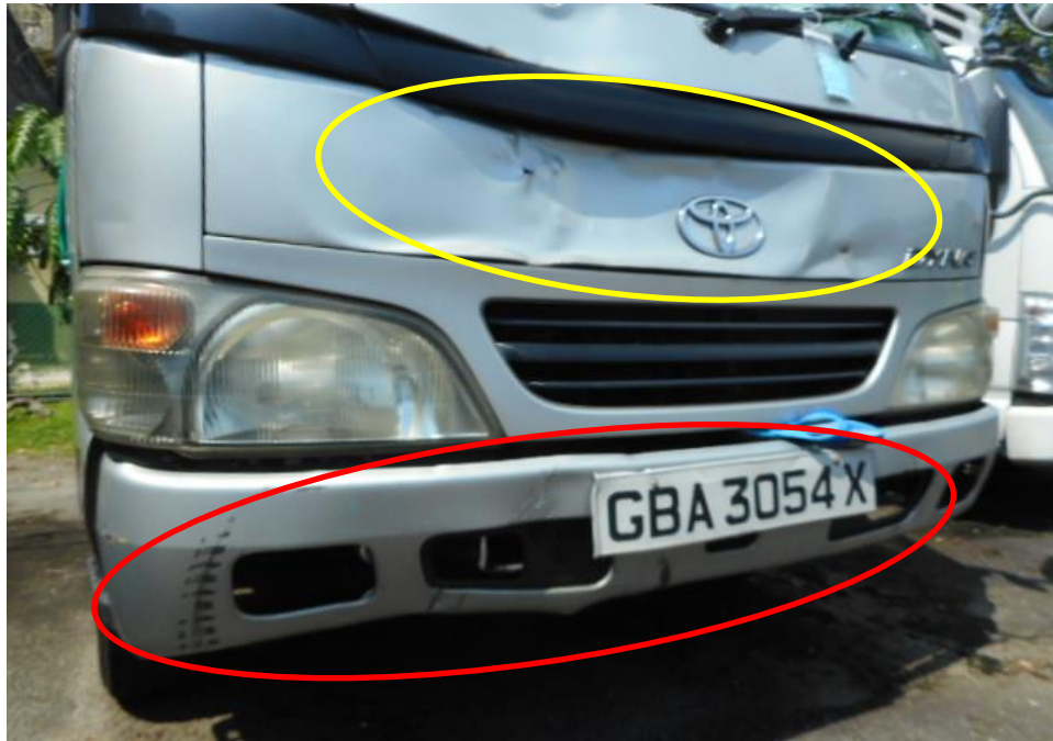
Photo 4 shows a close up view of the Motor Lorry's front portion at the time of my inspection. Its front bumper (red circle) and front body panel (yellow circle) was damage at the time of my inspection as a result of the accident.
