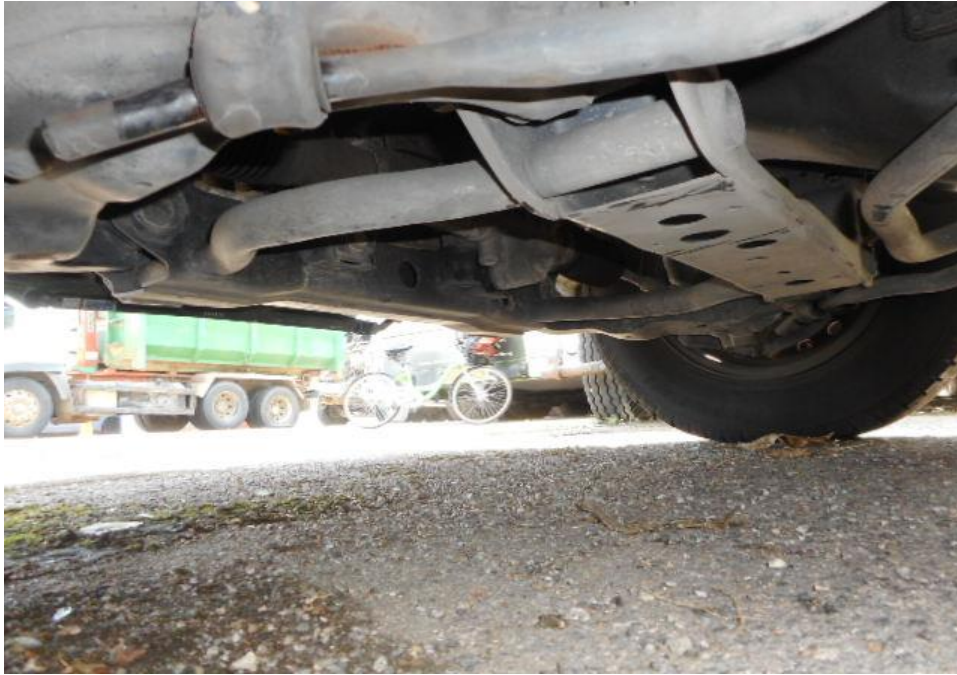
Photo 17 shows the undercarriage of the Motor Lorry, at the area where the engine housing and transmission housing are located. I did not find any sign(s) or indication(s) of fluid leak and/or fluid stain(s) on the underside of the Motor Lorry.
