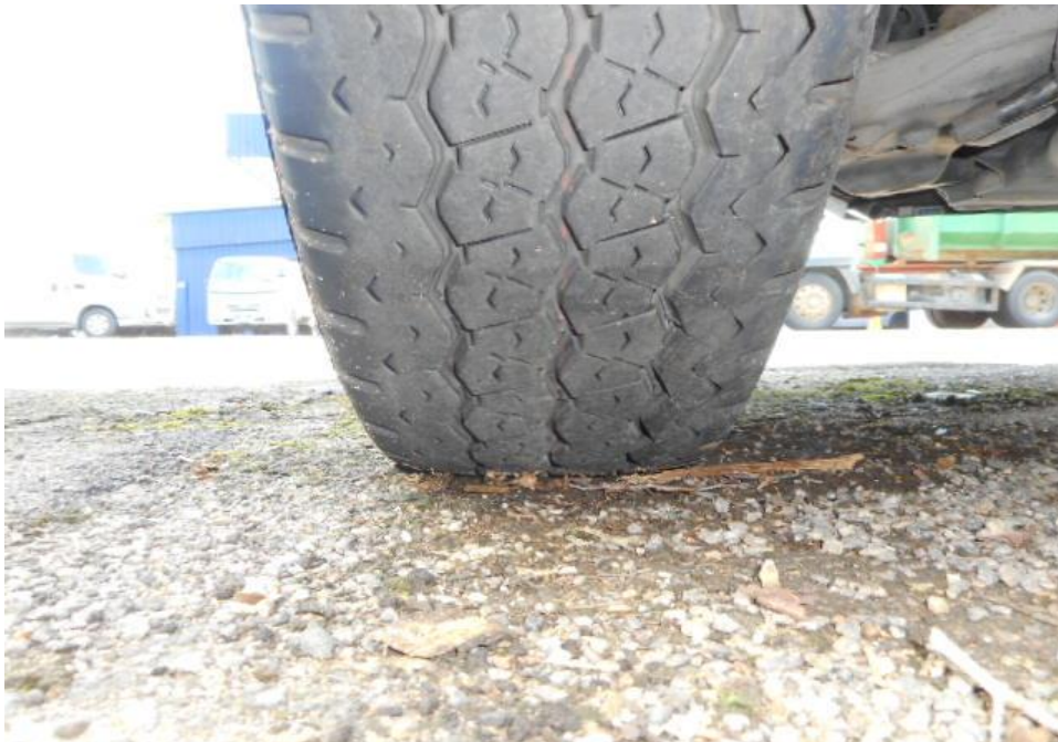
Photo 11 shows the condition of the rear right tyres of the Motor Lorry, which were observed to be in serviceable condition with remaining, tread depth of approximately 4.9mm. There was also no tear, cut or burst mark(s) on the outer and the inner sidewalls as well as across the tread of the 6 tyres that were fitted on the Motor Lorry.
