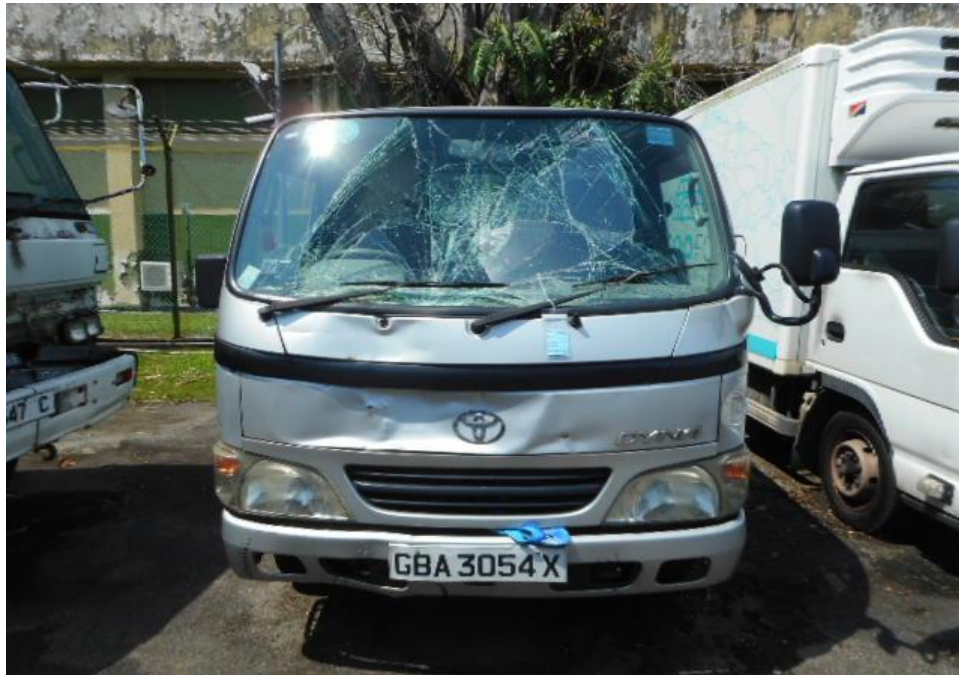
Photo 2 shows a general view of the Motor Lorry's frontal portion at the time of my inspection. It appeared to have sustained damage at its front portion. Its front windscreen, front body panel as well as its front bumper were damaged at the time of my inspection as a result of the accident.
