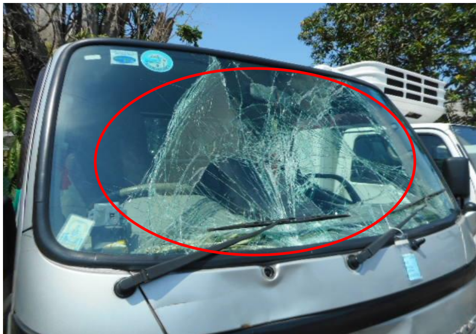
Photo 3 shows a close up view of the Motor Lorry's front portion at the time of my inspection. Its front windscreen (circled) was damaged at the time of my inspection as a result of the accident.
