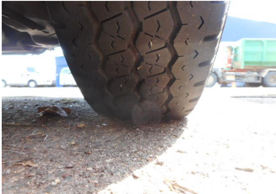
Photo 8 shows the condition of the front right tyre of the Motor Lorry, which was observed to be in serviceable condition with remaining tread depth of approximately 5.5mm. The tyre, which was wrapped around standard steel wheel rim, was also observed to be sufficiently inflated for vehicular operation. There was no tear, cut or burst mark(s) on the outer and the inner sidewalls as well as across the tread of the 6 tyres that were fitted on the Motor Lorry.
