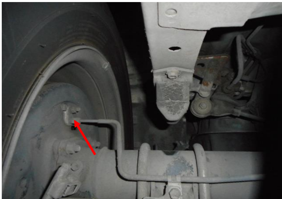
Photo 26 shows the various undercarriage components at the rear left wheel of the Motor Van, in particular the brake hose and drum brake (arrowed). The various undercarriage components of the Motor Van were all found to be intact without any visible damage. There was also no sign of fluid stain(s) observed on the various undercarriage components.
