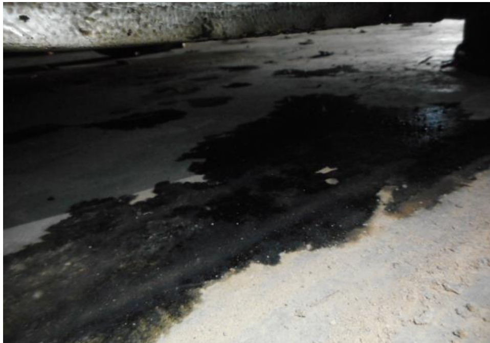
Photo 21 shows the undercarriage of the Motor Van, at the area where the engine housing and transmission housing are located. I have found engine oil leakage and fluid stain(s) on the underside of the Motor Van as a result of the accident.
