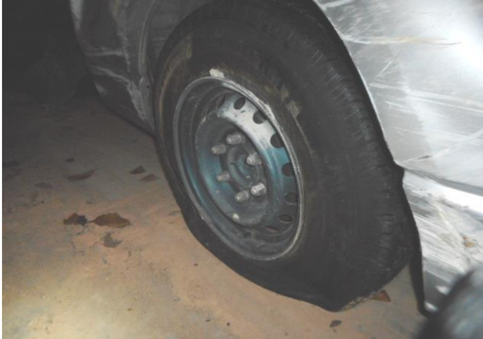
Photo 13 shows the condition of the rear right tyres of the Motor Van, which was observed to be in unserviceable condition with remaining tread depth of approximately 5.5mm. The steel wheel rim, was observed damage (circled) and the tyre was deflated as a result of the accident.
