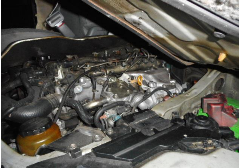
Photo 16 shows a general view of the Motor Van's engine compartment, which was accessed by lifting the front cabin of the Motor Van. The various parts and components inside the engine compartment were unaffected by the accident. There was also no sign(s) or indication(s) of fresh fluid leakage and/or fluid stain within the engine compartment
