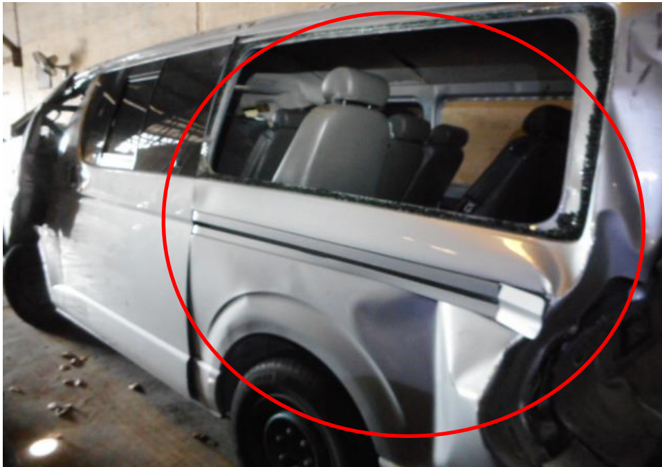
Photo 7 shows a general view of the Motor Van's left body at the time of my inspection. The left portion of the Motor Van was observed to have been affected by the accident. Its body panels (circled) was damaged as a result of the accident.
