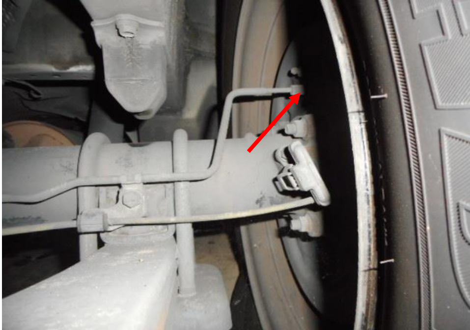
Photo 27 shows the various undercarriage components at the rear right wheel of the Motor Van, in particular the brake hose and drum brake (arrowed). The various undercarriage components of the Motor Van were all found to be intact without any visible damage. There was also no sign of fluid stain(s) observed on the various undercarriage components.
