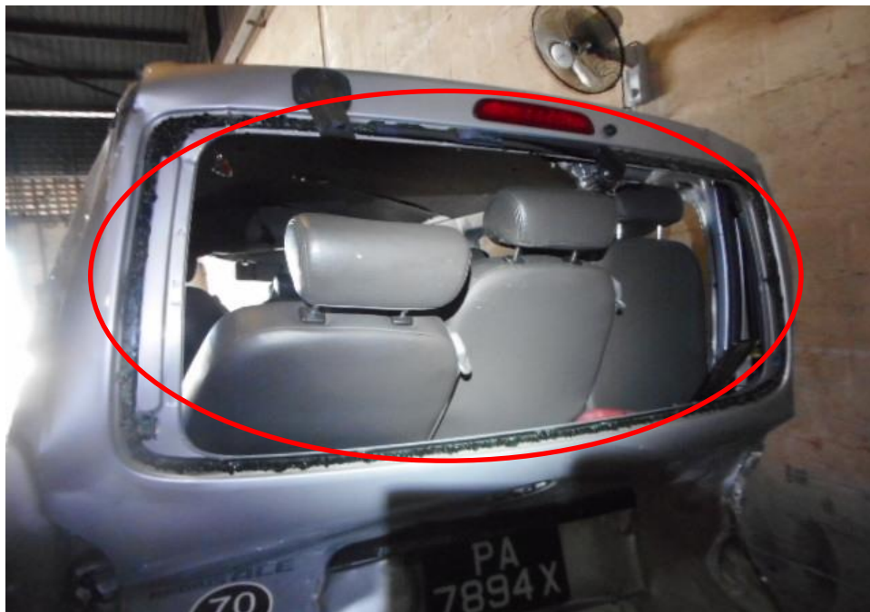
Photo 10 shows the general view of the Motor Van's rear body at the time of my inspection. The rear portion of the Motor Van was observed to have been affected by the accident. Its windscreen (circled) was damaged as a result of the accident.
