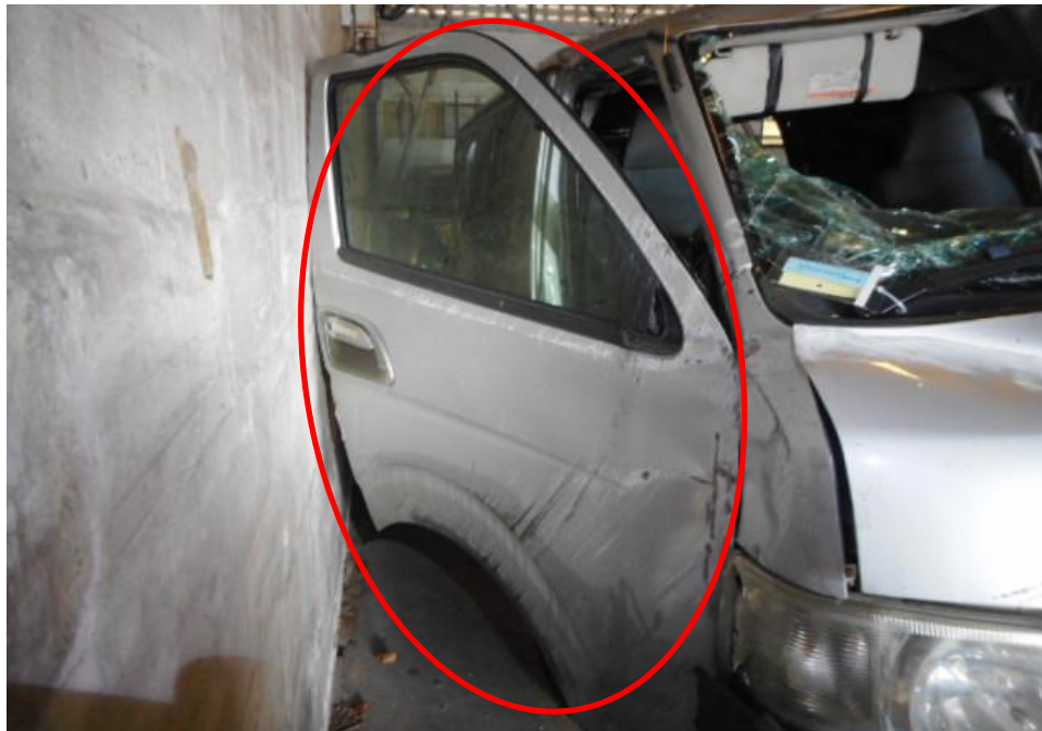
Photo 4 shows the close up view of the right door of the Motor Van at the time of our inspection. The Motor Van was observed to have sustained damages to its right door (circled) as a result of the accident.
