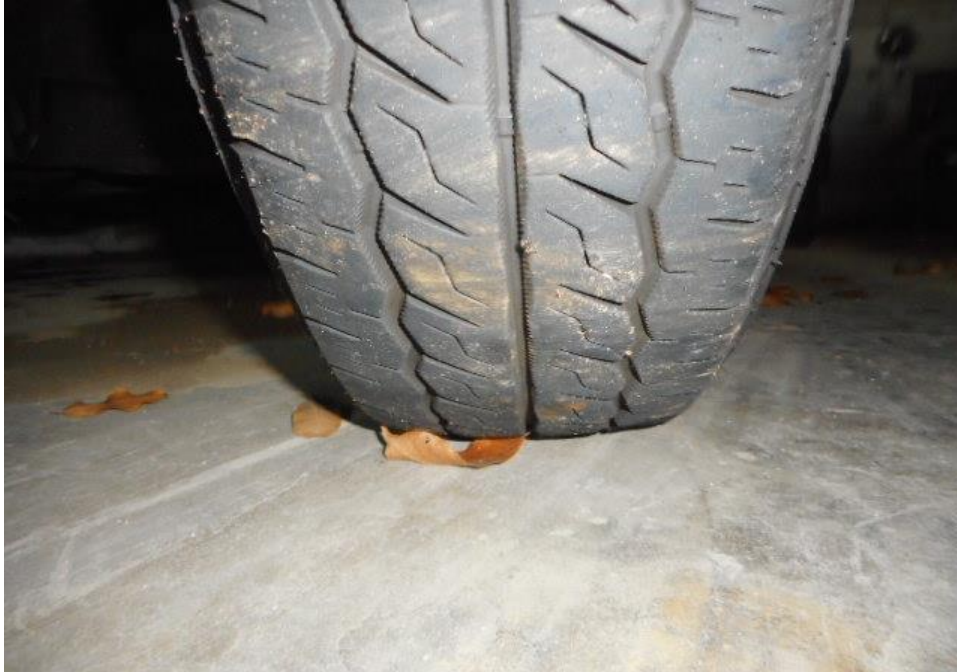
Photo 15 shows the condition of the front left tyre of the Motor Van, which were observed to be in serviceable condition with remaining, tread depth of approximately 6.4mm. See above.
