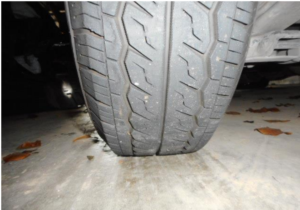
Photo 14 shows the condition of the rear left tyres of the Motor Van, which were observed to be in serviceable condition with remaining, tread depth of approximately 5.2mm. See above.
