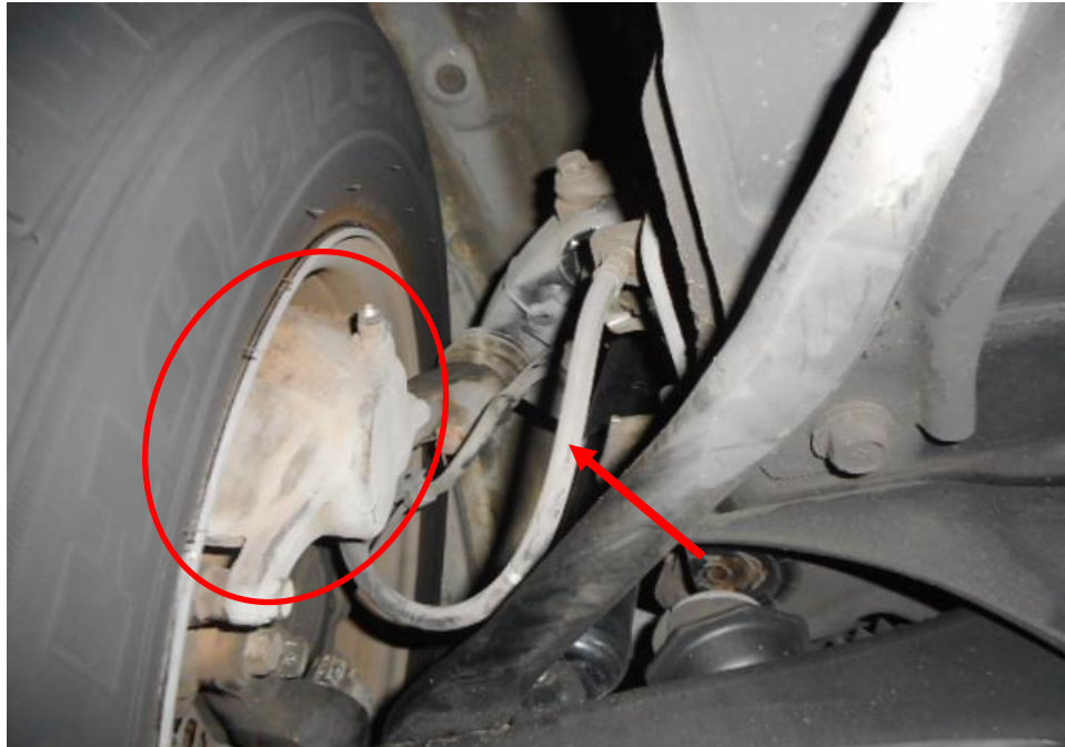
Photo 25 shows the various undercarriage components at the front left wheel of the Motor Van, in particular the brake hose (arrowed) and callipers (circled). The various undercarriage components of the Motor Van were all found to be intact without any visible damage. There was also no sign of fluid stain(s) observed on the various undercarriage components.
