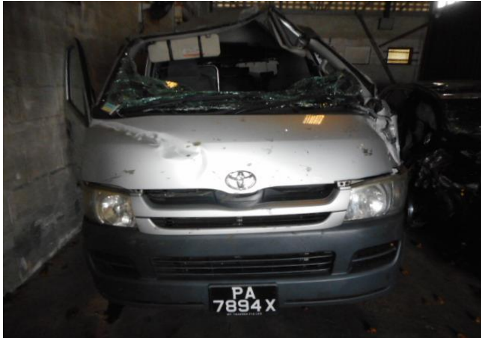
Photo 1 shows a general view of the front portion of the Motor Van at the time of our inspection. The Motor Van was observed sustained damage all around, front windscreen, front cabin, front body panel, front left and right door. Its left and right body panel as well as its rear door and rear windscreen was damaged as a result of the accident.
