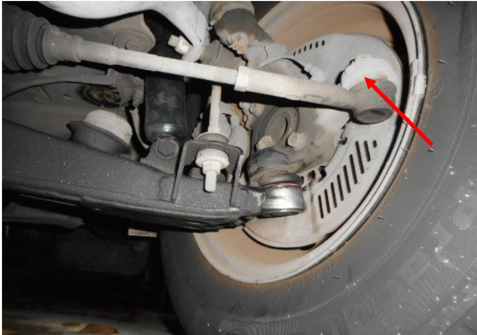
Photo 23 shows the various undercarriage components at the front left wheel of the Motor Van, in particular the steering tie rod end and ball joints (arrowed) were observed to be intact. There was also no sign of fluid stain observed on the various undercarriage components at the front right wheel of the Motor Van.
