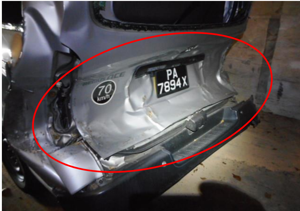
Photo 11 shows the general view of the Motor Van's rear body at the time of my inspection. The rear portion of the Motor Van was observed to have been affected by the accident. Its rear door (circled) was damaged as a result of the accident.
