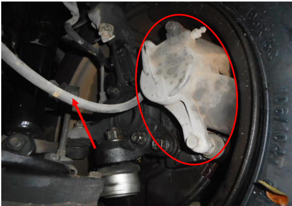
Photo 24 shows the various undercarriage components at the front right wheel of the Motor Van, in particular the brake hose (arrowed) and callipers (circled). The various undercarriage components of the Motor Van were all found to be intact without any visible damage. There was also no sign of fluid stain(s) observed on the various undercarriage components.
