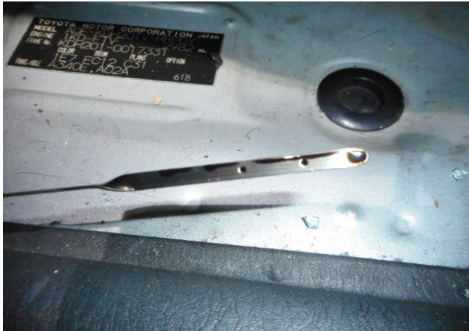
Photo 20 shows the engine oil dip stick of the Motor Van at the time of my inspection. The engine oil was observed to be of insufficient level due to a leakage as a result of the accident.
