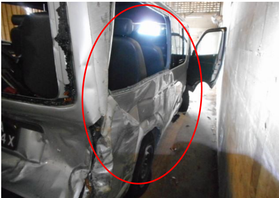
Photo 8 shows a general view of the Motor Van's right body at the time of my inspection. The right portion of the Motor Van was observed to have been affected by the accident. Its body panels (circled) was damaged as a result of the accident.
