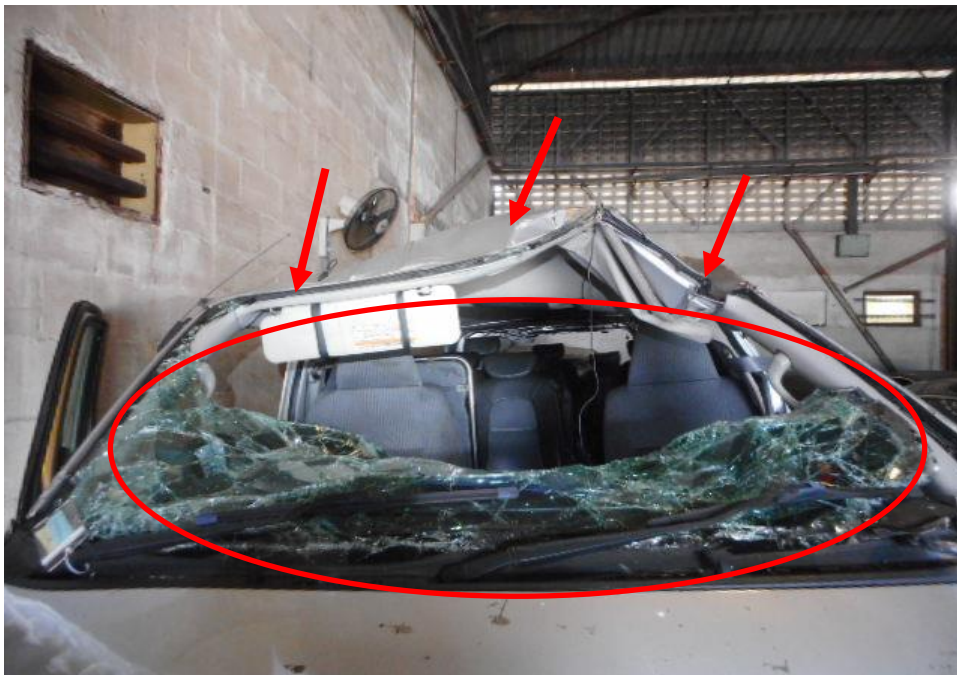
Photo 2 shows the close up view of the front portion of the Motor Van at the time of our inspection. The Motor Van was observed to have sustained major damages to its front windscreen (circled) and its front cabin (arrowed) that was crushed due to the accident's impact.
