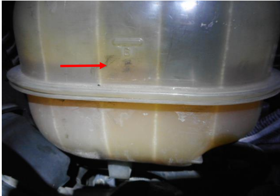
Photo 18 shows the engine coolant of the Motor Van at the time of my inspection. The engine coolant was observed to be of sufficient level and without any visible contamination.
