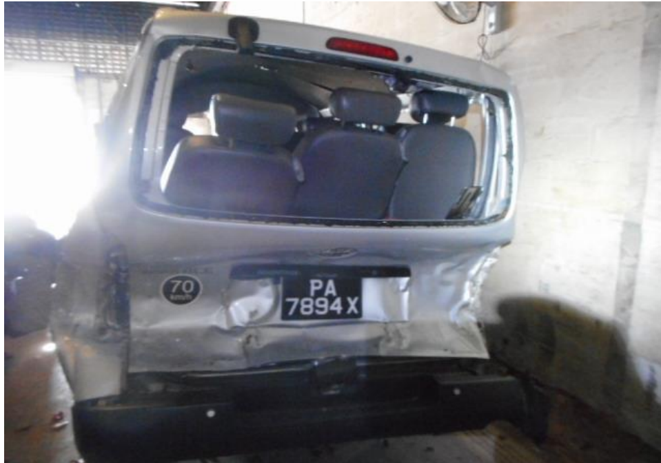
Photo 9 shows the general view of the Motor Van's rear body at the time of my inspection. The rear portion of the Motor Van was observed to have been affected by the accident. Its rear door and windscreen (circled) was damaged as a result of the accident.
