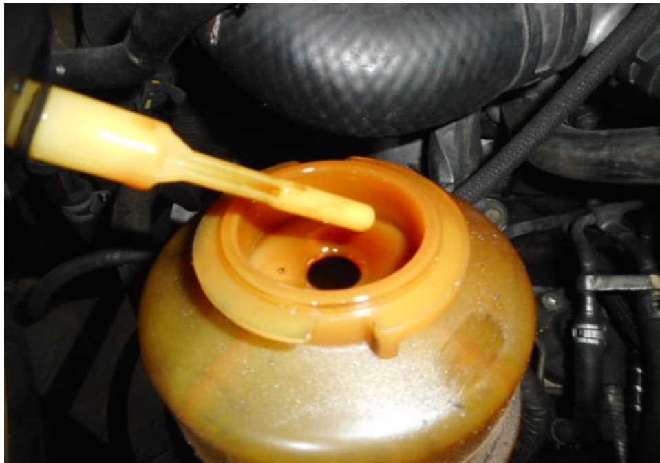
Photo 19 shows the power steering fluid dip stick of the Motor Van at the time of my inspection. The steering fluid was observed to be of sufficient level and without any visible contamination.
