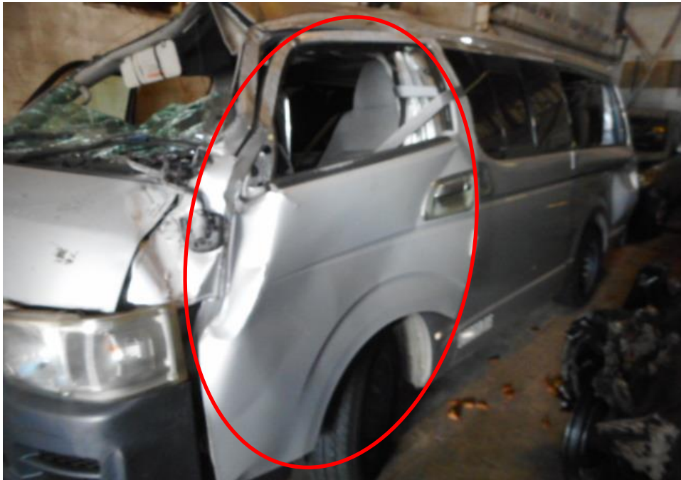
Photo 5 shows the close up view of the left door of the Motor Van at the time of our inspection. The Motor Van was observed to have sustained damages to its left door (circled) as a result of the accident.
