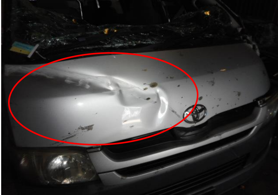
Photo 3 shows the close up view of the front portion of the Motor Van at the time of our inspection. The Motor Van was observed to have sustained major damages to its front body panel (circled) that was damaged as a result of the accident's impact.
