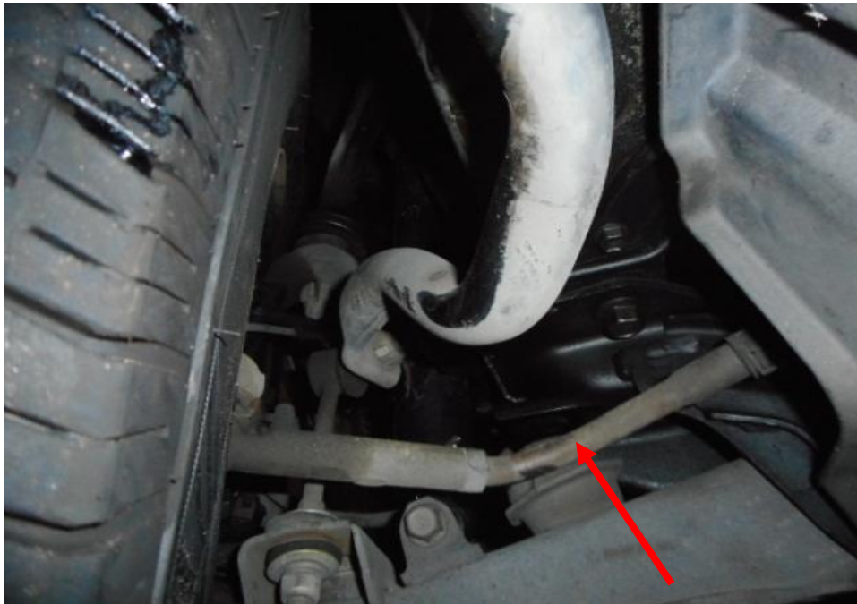
Photo 22 shows the various undercarriage components at the front right wheel of the Motor Van, in particular the steering tie rod (arrowed) were found to be bent as a result of the accident.
