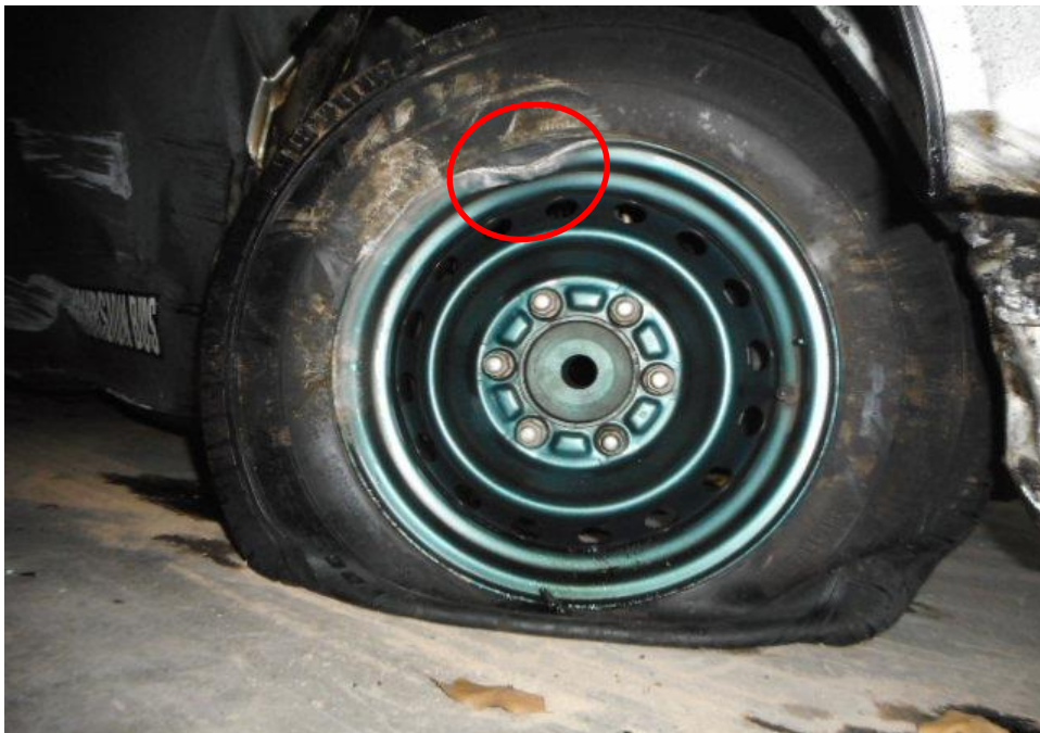
Photo 12 shows the condition of the front right tyre of the Motor Van, which was observed to be in unserviceable condition with remaining tread depth of approximately 5.4mm. The steel wheel rim, was observed damage (circled) and the tyre was deflated as a result of the accident.
