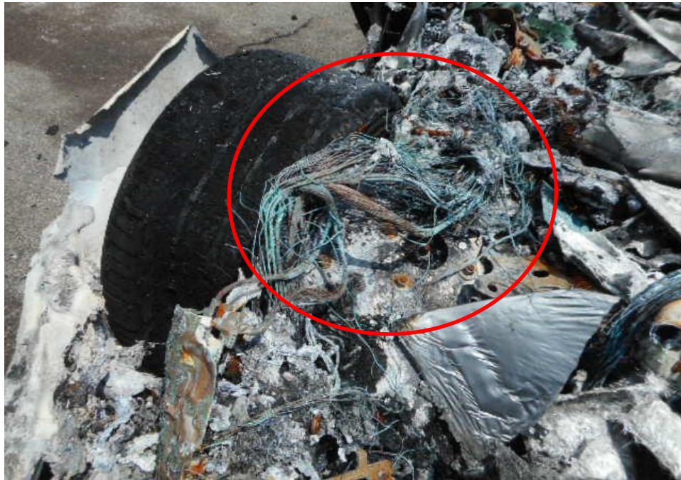
Photo 9 shows a general view of the original wiring harness in the rear left interior compartment. The original wiring harness (circled) was observed with greenish residue on the surface. The presence of greenish residue indicates internal heating of copper wires, a sign of an electrical short circuit occurring. The greenish residue is normally left behind from oxidation as a result of chemical reaction involving the copper wires.
