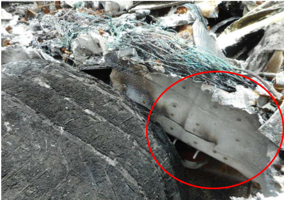
Photo 8 shows the exterior of the rear left portion of the Motor Car at the time of our inspection. The high heat intensity burn marks (whitish burn marks) and rust that had development found on the exterior surface (circled) indicates that the fire had originated from the rear left portion of the Motor Car.
