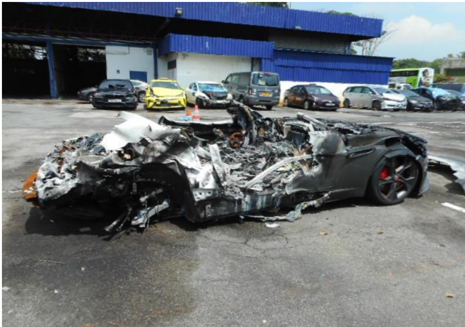
Photo 4 shows the general view of the right portion of the Motor Car at the time of our inspection. The Motor Car was observed to have sustained physical damage at its right portion. Its right body panel and right rear fender portion was observed to have been damaged as a result of the road traffic accident. The fire had also affect the right of the Motor car.
