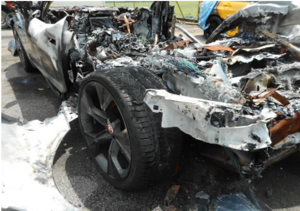
Photo 7 shows the exterior of the rear left portion of the Motor Car at the time of our inspection. The high heat intensity burn marks (whitish burn marks) and rust that had development found on the exterior surface indicates that the fire had originated from the rear left portion of the Motor Car.
