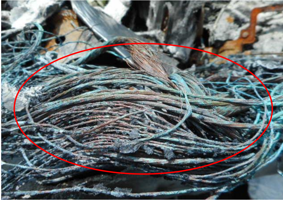
Photo 11 shows a close up view of the original wiring harness in the rear left interior compartment. The original wiring harness (circled) was observed with greenish residue on the surface. The presence of greenish residue indicates internal heating of copper wires, a sign of an electrical short circuit occurring. The greenish residue is normally left behind from oxidation as a result of chemical reaction involving the copper wires.
