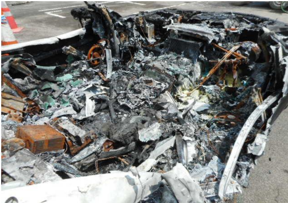
Photo 6 shows the general view of the interior compartment of the Motor Car at the time of our inspection. Its interior compartment was completely burnt as a result of the fire.
