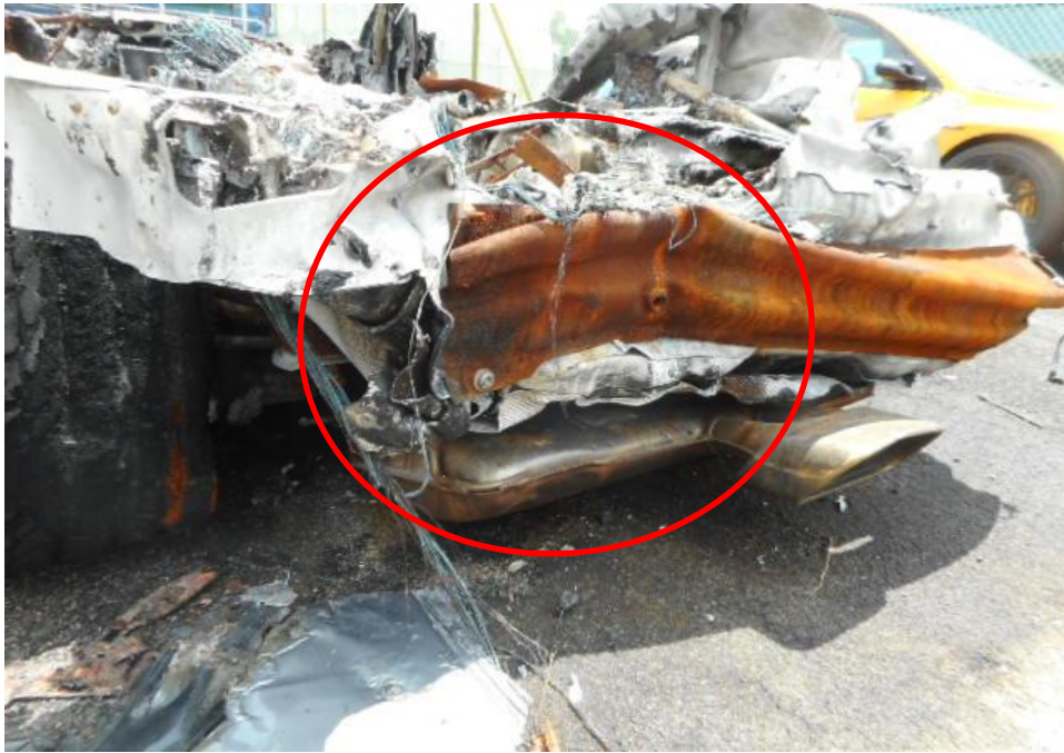
Photo 3 shows the close up view of the rear portion of the Motor Car at the time of our inspection. The Motor Car was observed to have sustained physical damage at its rear portion. Its rear left bumper portion (circled) was observed to have been damaged as a result of the road traffic accident. The fire had also affect the rear of the Motor car.
