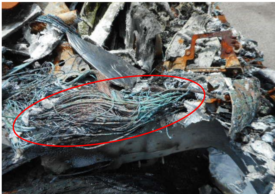
Photo 10 shows a close up view of the original wiring harness in rear left interior compartment. The original wiring harness (circled) was observed with greenish residue on the surface. The presence of greenish residue indicates internal heating of copper wires, a sign of an electrical short circuit occurring. The greenish residue is normally left behind from oxidation as a result of chemical reaction involving the copper wires.
