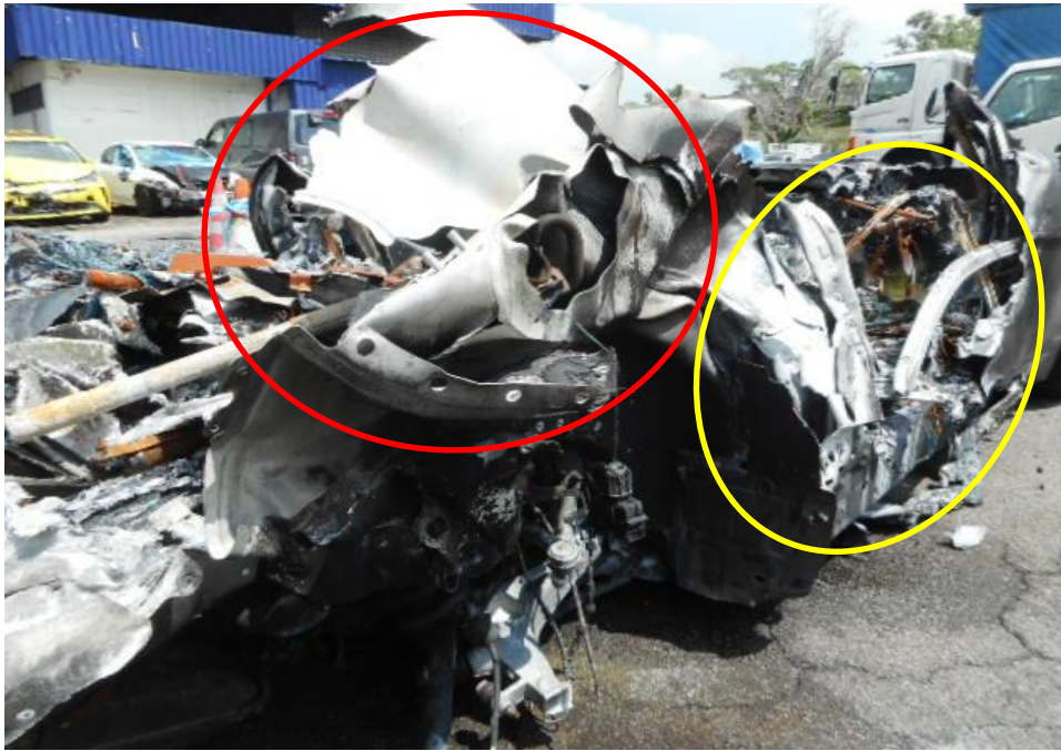
Photo 5 shows the close up view of the rear portion of the Motor Car at the time of our inspection. The Motor Car was observed to have sustained physical damage at its right portion. Its right body panel (yellow circle) and right rear fender (red circle) portion was observed to have been damaged as a result of the road traffic accident. The fire had also affect the right of the Motor car.
