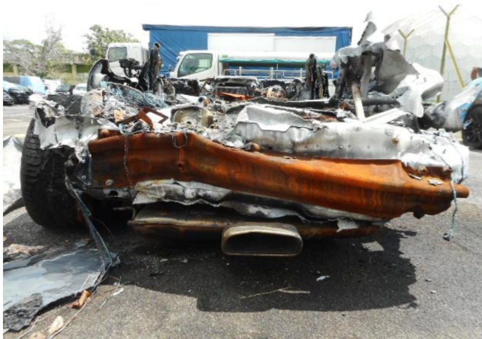
Photo 2 shows the general view of the rear portion of the Motor Car at the time of our inspection. The Motor Car was observed to have sustained physical damage at its rear portion. Its rear left bumper portion was observed to have been damaged as a result of the road traffic accident. The fire had also affect the rear of the Motor car.
