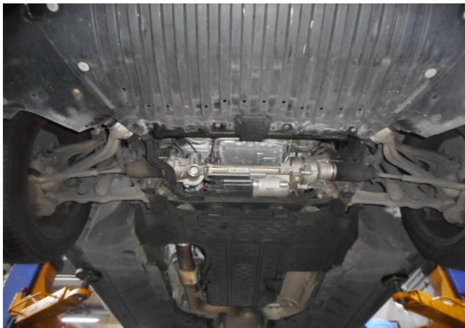
Photo 5 shows the general view of the engine underside portion of the Insured Vehicle at the time of our inspection. The engine underside compartment is observed to be unaffected and by any signs of accident.
