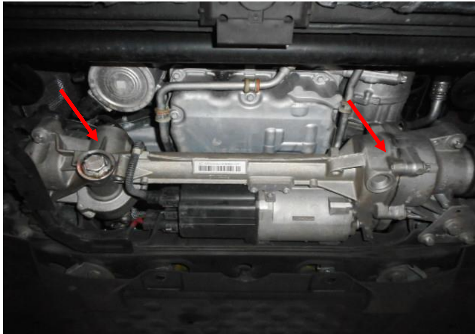
Photo 6 shows the close up view of the power steering portion of the Insured Vehicle at the time of our inspection. The Electronic Power Steering unit and its steering rack and pinion component is observed to be unaffected and by any signs of accident.
