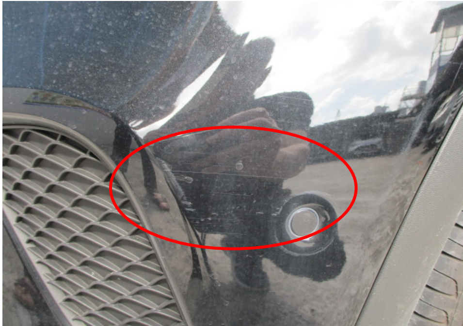
Photo 7 shows the relatively faint grazed marks (circled) that I had observed on the lower left corner area of the Insured Vehicle's front bumper.
