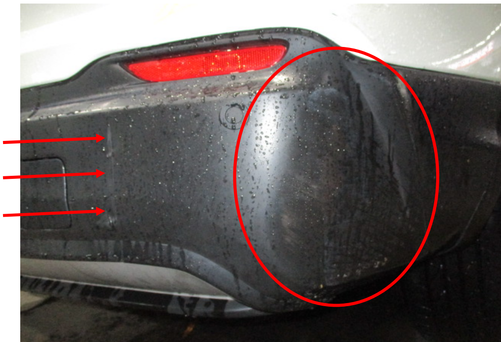
Photo 3 shows a close up view of the dent/distortion (circled) that was seen on the lower right corner area of the Third Party Vehicle's rear bumper at the time of physical inspection by LKK Auto Consultants Pte Ltd. The vertical indentation at the area below the rear bumper right reflector is also highlighted by the rear arrows. Both these damages arose from direct contact with an object(s).
