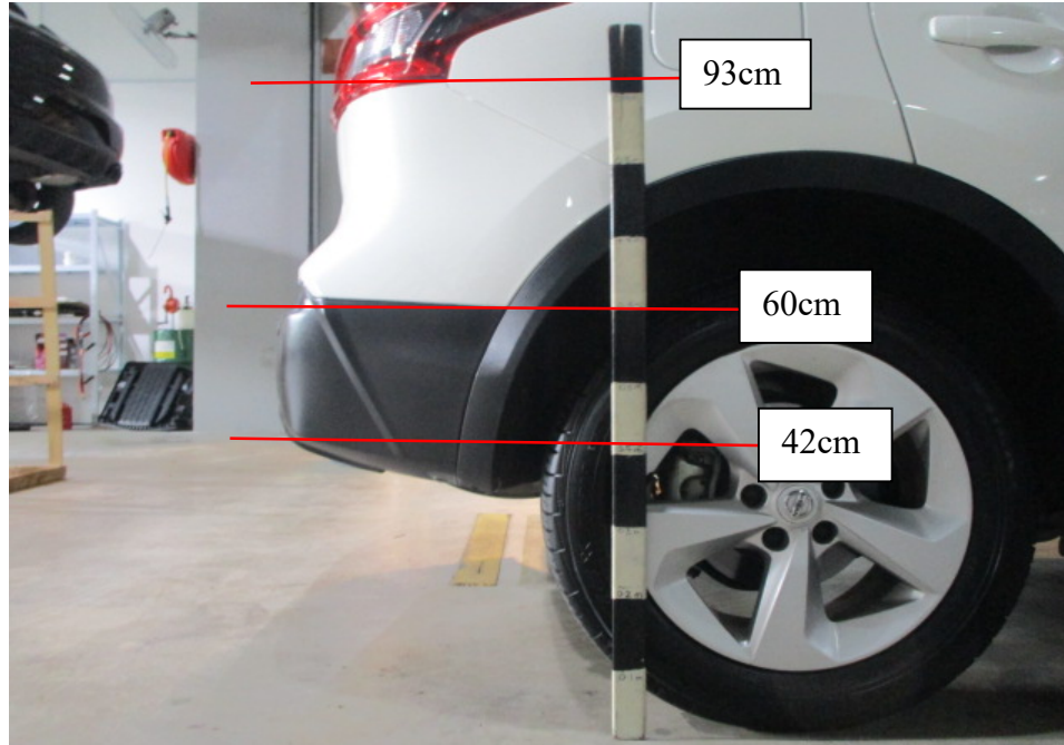
Photo 15 shows height measurement being carried out at the rear right, side profile of a similar make and model vehicle as the Third Party Vehicle. The height of the dent/distortion at the lower right corner area of the Third Party Vehicle's rear bumper (refer to photograph 3 above) was measured to be 42cm to 60cm above ground level. The crack at the rear right taillamp (refer to photograph 4 above) of the Third Party Vehicle was 93cm above ground level.
