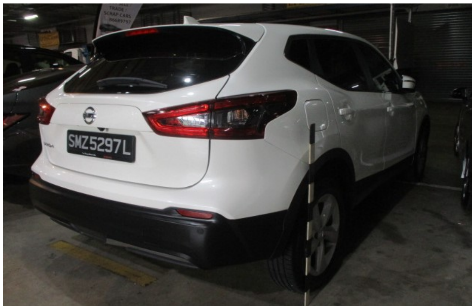
Photo 14 shows height measurement being carried out at the rear right, side profile of a similar make and model vehicle as the Third Party Vehicle.
