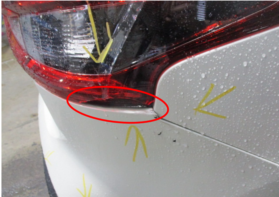
Photo 4 shows a close up view of the crack (circled) that was seen on the Third Party Vehicle's rear right taillamp at the time of physical inspection by LKK Auto Consultants Pte Ltd. The crack was observed to be at the area where the rear bumper aligns with the rear right fender. This damage arose from direct contact with an object(s).
