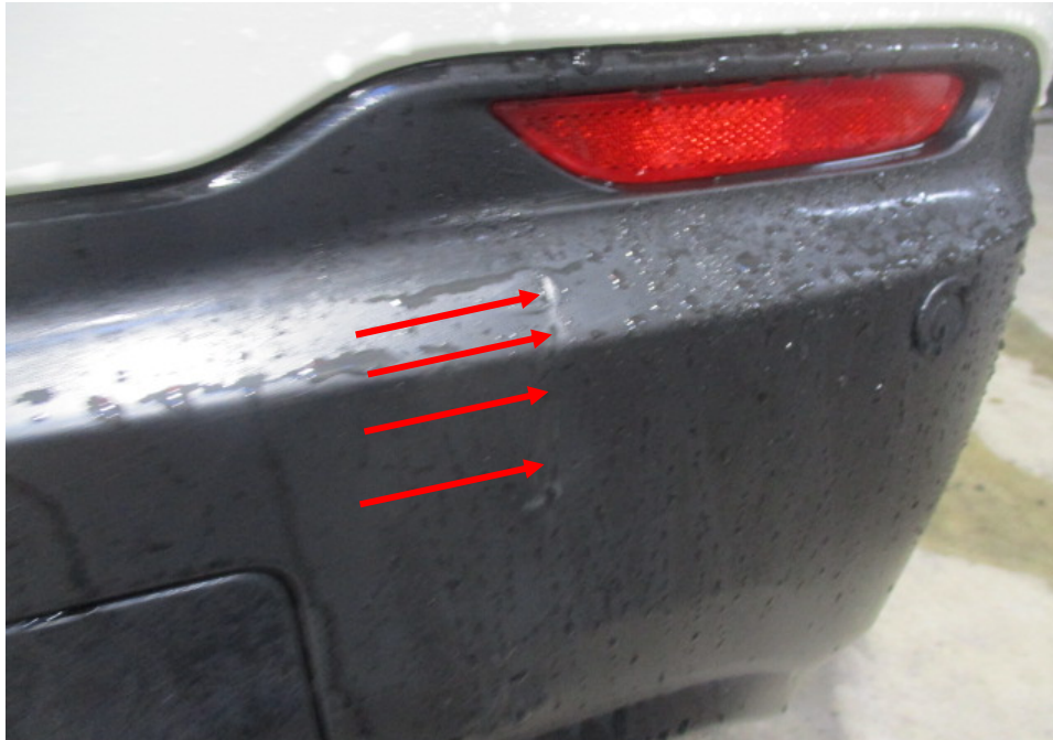
Photo 2 shows a close up view of the vertical indentation (arrowed) that was seen on the rear bumper of the Third Party Vehicle at the time of physical inspection by LKK Auto Consultants Pte Ltd. This was at the area below the rear bumper right reflector. This damage arose from direct contact with an object(s).
