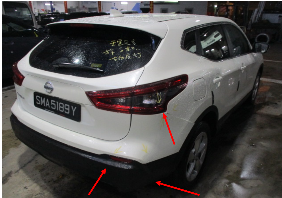
Photo 1 shows the rear right portion of the Third Party Vehicle at the time of physical inspection by LKK Auto Consultants Pte Ltd. The Third Party Vehicle was observed to have sustained damage that was confined to its rear right portion. Direct contact damage was seen at 3 areas at the rear right portion. The rear bumper was distorted with a vertical indentation below the rear bumper right reflector; the lower right corner of the rear bumper was dented/distorted; the rear right taillamp was cracked at the area where the rear bumper aligns with the rear right fender. The aforesaid damage areas are highlighted by the red arrows with close up shown in the below photographs.
