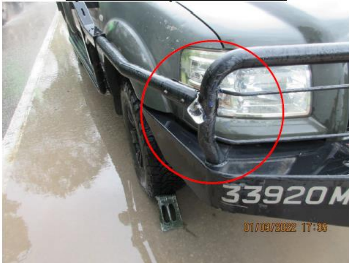
Figure C-5: Dent at front protection bar of MID 33920
