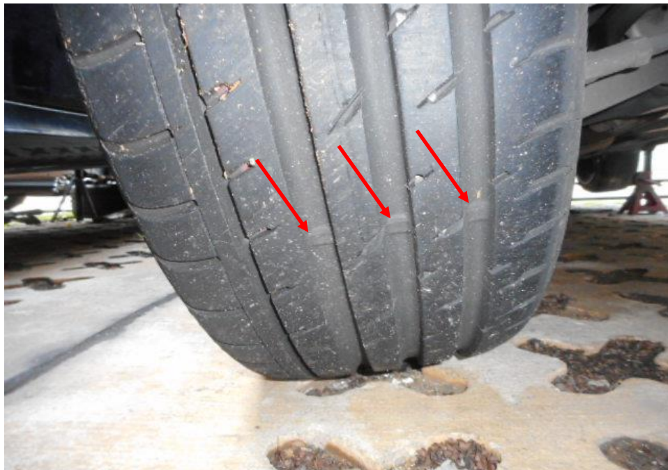
Photo 5 shows the front right tyre of the of the Insured Vehicle, which was observed to be in serviceable condition with remaining tread depth of approximately 7mm. The pattern of the tread was generally still visible. The tyre wear indicators (arrowed), normally built into the groove of the tread pattern, and were also observed to be not flushed with the tread pattern.
