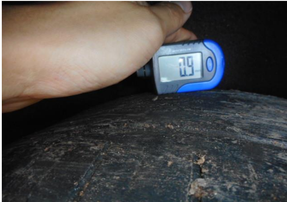
Photo 16 shows measurements being conducted on the inner to outer side of the tread on the rear left tyre of the Insured vehicle. The remaining tread depth was measured to be approximately 0.9mm.
