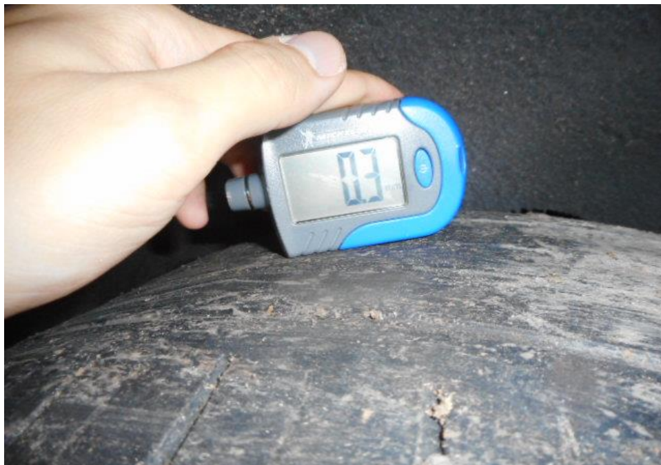
Photo 17 shows measurements being conducted on the inner to outer side of the tread on the rear left tyre of the Insured vehicle. The remaining tread depth was measured to be approximately 0.3mm.
