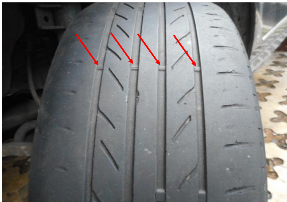
Photo 7 shows the condition of the front left tyre of the Insured vehicle, which was observed to be in serviceable condition with remaining tread depth of approximately 2.4mm. The pattern of the tread was generally still visible. The tyre wear indicators (arrowed), normally built into the groove of the tread pattern, and were also observed to be not flushed with the tread pattern.
