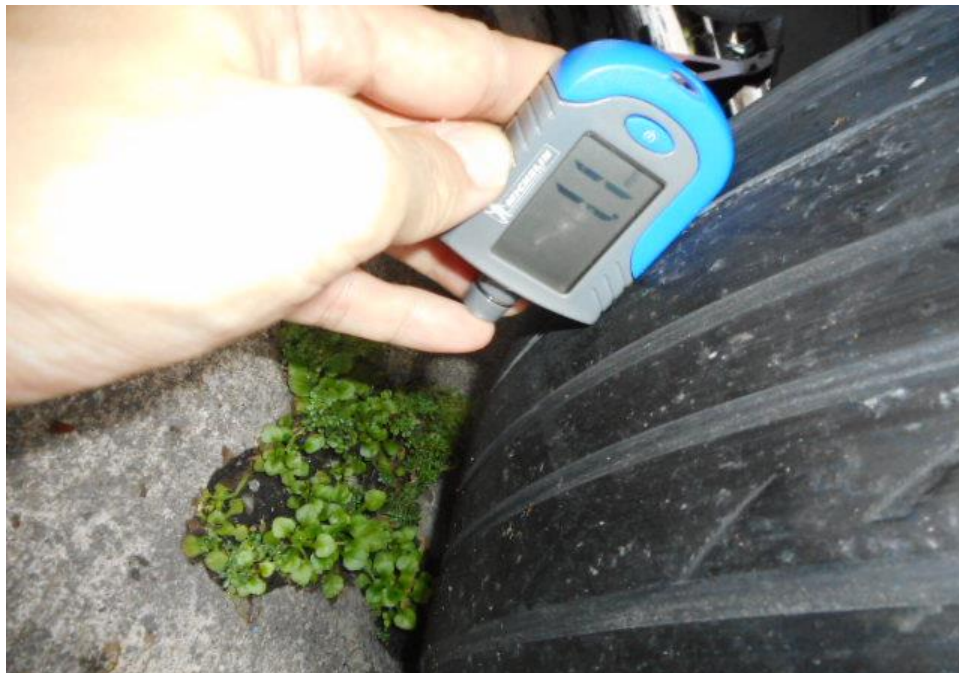
Photo 11 shows measurements being conducted on the inner to outer side of the tread on the rear right tyre of the Insured vehicle. The remaining tread depth was measured to be approximately 1.1mm.
