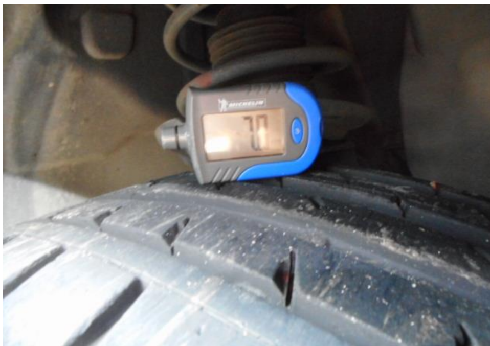
Photo 6 shows measurements being conducted on the remaining tread depth of the front right tyre of the Insured vehicle. The remaining tread depth was measured to be approximately 7mm.
