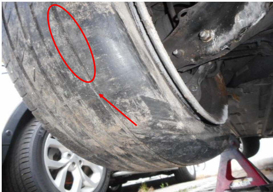
Photo 15 shows the rear left tyre of the Insured vehicle at the time of our inspection. The rubber at the inner side of the tread (circled) was partially worn. The pattern at some areas on the inner side of the tread was vaguely visible due to worn rubber and flushed with the tyre wear indicator (arrowed) however the reinforcing belts that are found within the tyre were not exposed at the time of our inspection.
