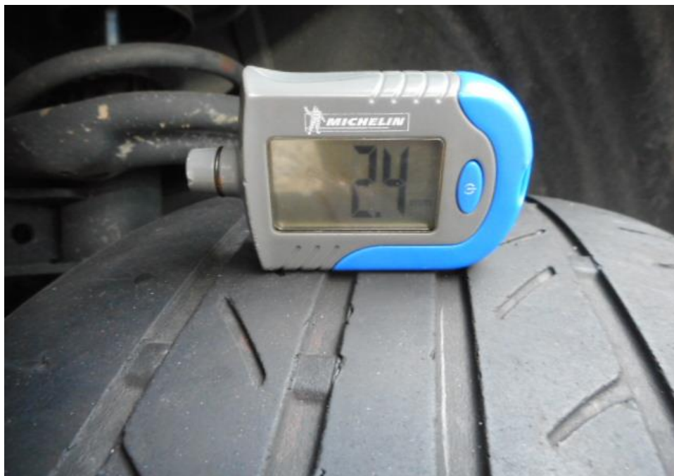
Photo 8 shows measurements being conducted on the remaining tread depth of the front left tyre of the Insured vehicle. The remaining tread depth was measured to be approximately 2.4mm.
