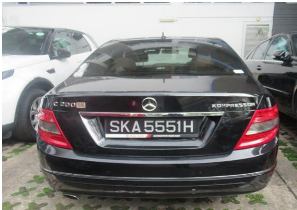
Photo 3 shows the general view of the rear portion of the Insured vehicle at the time of my inspection its rear portion was observed to be affected by the accident. Its rear bumper was damaged as a result of the accident.
