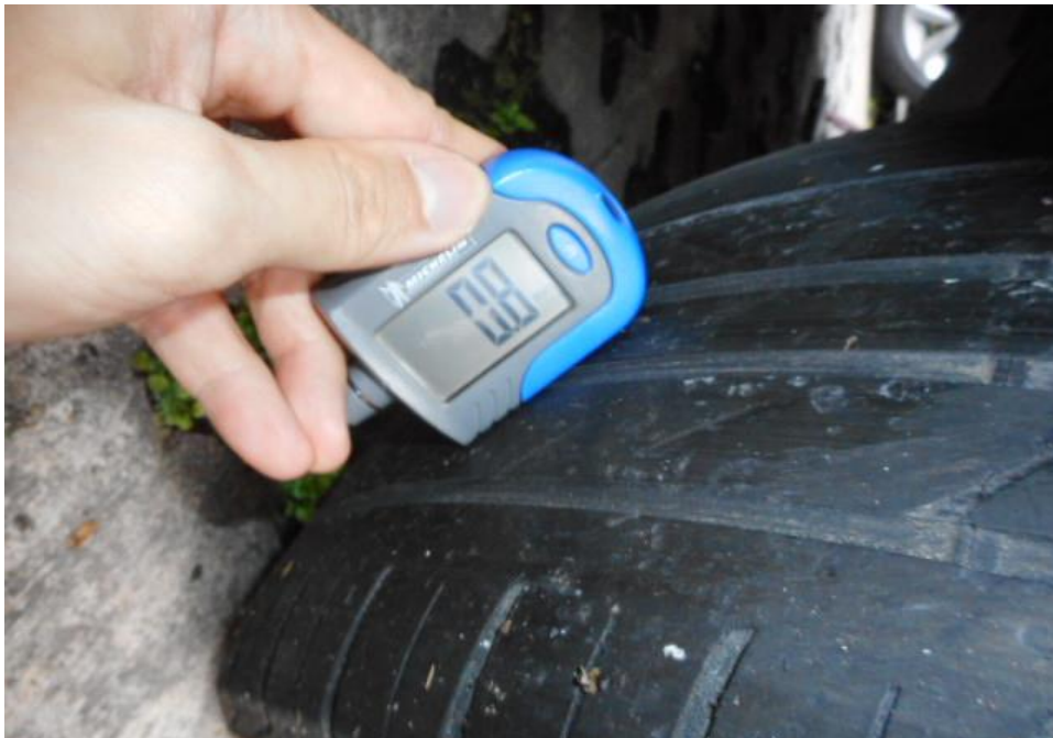
Photo 13 shows measurements being conducted on the outer side of the tread on the rear right tyre of the Insured vehicle. The remaining tread depth was measured to be approximately 0.8mm.
