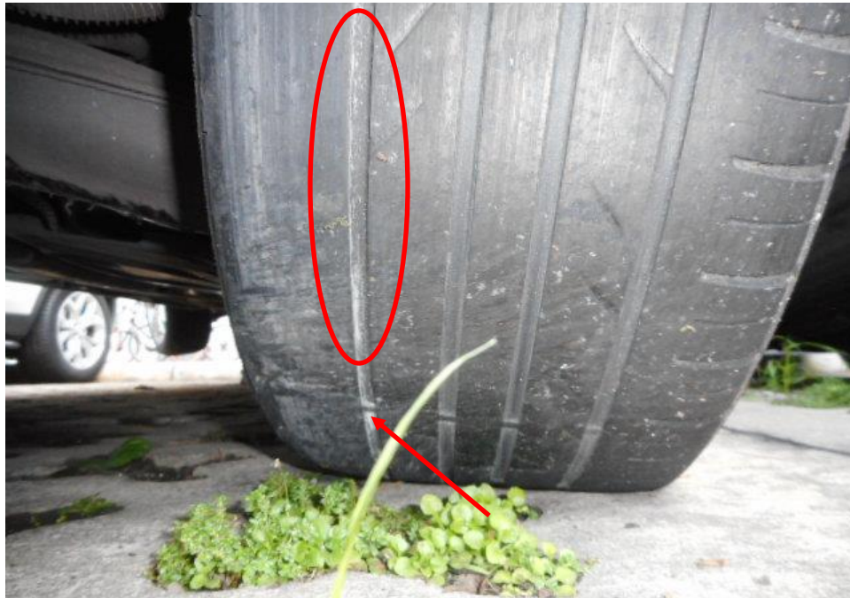
Photo 9 shows the rear right tyre of the Insured vehicle at the time of our inspection. The rubber at the inner side of the tread (circled) was partially worn. The pattern at some areas on the inner side of the tread was vaguely visible due to worn rubber and flushed with the tyre wear indicator (arrowed) however the reinforcing belts that are found within the tyre were not exposed at the time of our inspection.
