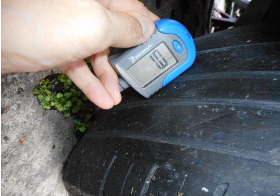
Photo 12 shows measurements being conducted on the outer side of the tread on the rear right tyre of the Insured vehicle. The remaining tread depth was measured to be approximately 1mm.
