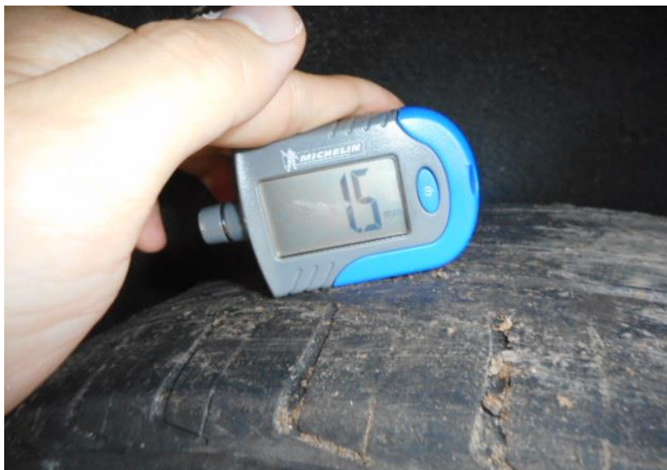
Photo 19 shows measurements being conducted on the inner to outer side of the tread on the rear left tyre of the Insured vehicle. The remaining tread depth was measured to be approximately 1.5mm.
