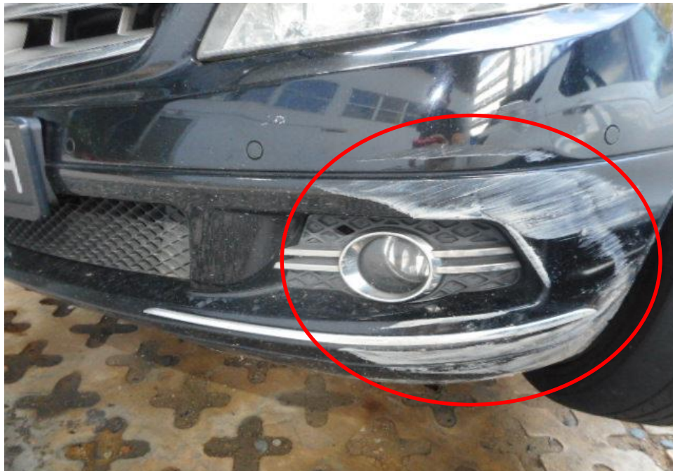
Photo 2 shows the close up view of the front portion of the Insured vehicle at the time of my inspection its front portion was observed to be affected by the accident. Its front bumper (circled) was damaged as a result of the accident.
