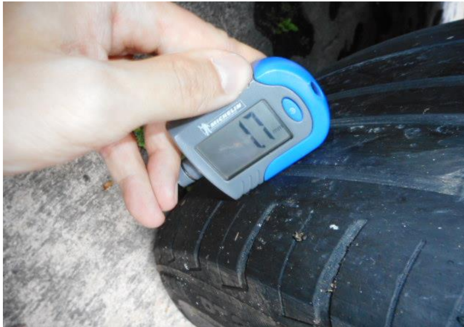
Photo 14 shows measurements being conducted on the outer side of the tread on the rear right tyre of the Insured vehicle. The remaining tread depth was measured to be approximately 1.7mm.
