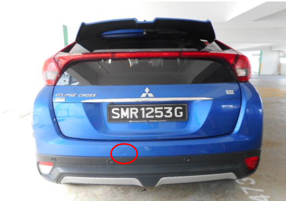
Photo 1 shows the general view of the rear portion of Third Party at the time of inspection. The rear bumper had been damaged. It was also noted that there were paint scratch marks (circled) on the rear bumper of Third Party.
