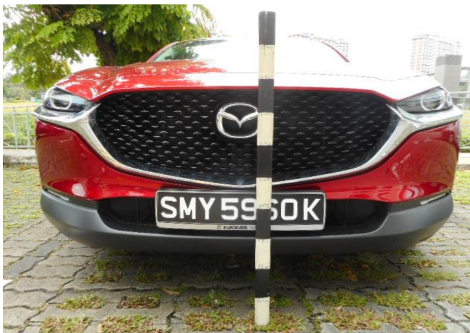
Photo 8 shows a general view of the height measurement being conducted on the front portion of Insured. The front right chrome and body panels was measured to be between 65cm above ground level.
