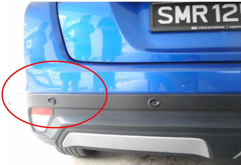
Photo 4 shows a close up view of the rear portion of the Third Party. We note that there was neither dislodgement nor misalignment of the rear bumper at the rear portion (circled) of Third Party.
