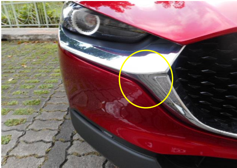
Photo 6 shows a close up view of the front portion of the Insured. We observed that there were no scratches or paint transfer marks on its front chrome and body panel portion of the Insured and that there was neither dislodgement nor misalignment of the front bumper at the front right portion (circled) of Insured.
