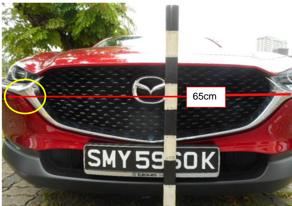
Photo 10 shows the close up view of the height measurement being conducted on the front portion of Insured. The front right chrome and body panels (circled) was measured to be between 65cm above ground level.
