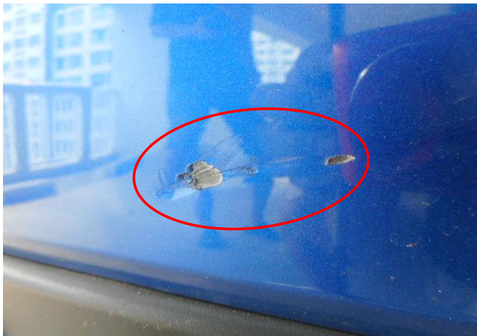
Photo 2 shows a close up view of the rear portion of the Third Party. We noted that there were paint scratch and dent marks the rear bumper with horizontal indentation from the right to the left which had resulted in the accumulation of blue paint of Third Party vehicle color on the rear bumper (circled).
