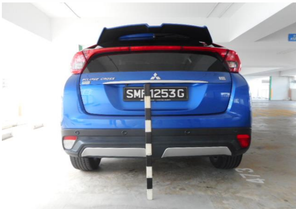
Photo 7 shows the general view of the height measurement being conducted on the rear portion of Third Party. The height above ground level of where the damages were found to the rear bumper of the Third Party was at 64cm to 65cm.
