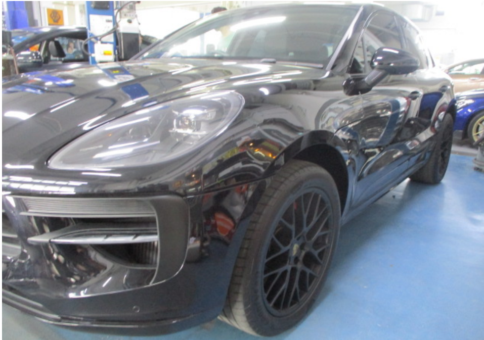
Photo 6 shows a closer view of the Motor Car's front bonnet, front left headlamp, front left wheel rim, front bumper left grille and front left day light. The body parts at the frontal portion of the Motor Car were visually examined and it was observed that the repair/restoration works carried out to the damaged area of the Motor Car (refer to photograph 1 above) were reasonably adequate and in order.
