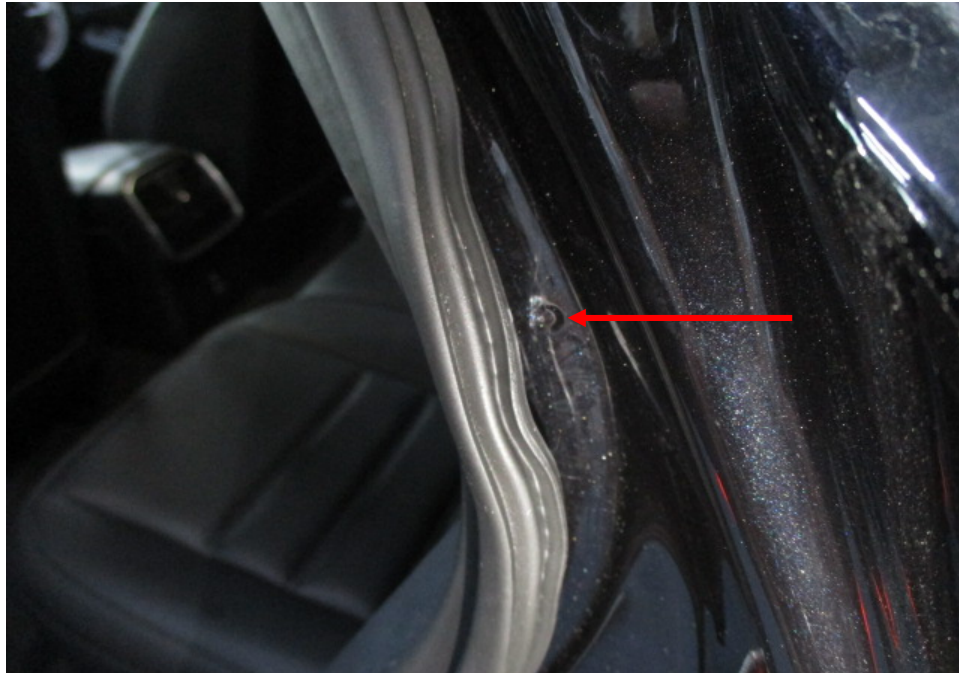
Photo 30 shows the left side “C” pillar of the Motor Car. I did not find any weld marks other than original spot weld marks (arrowed) on the left side “C” pillar of the Motor Car which, indicates that there was no re-welding works carried out. In general, I had found all the non-detachable body panels of the Motor Car to be originally fitted at the time of my inspection.
