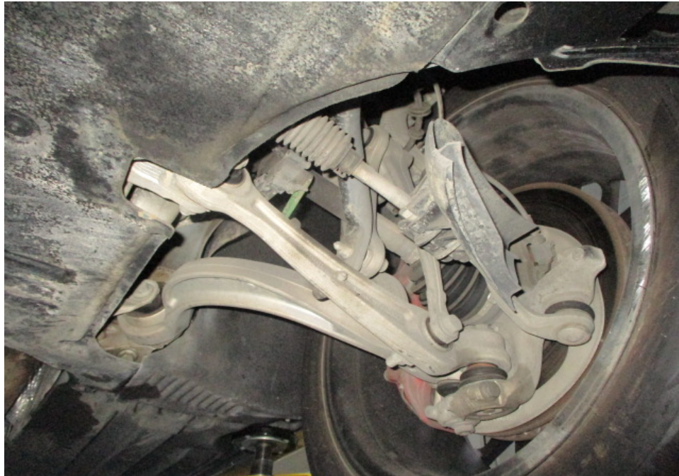
Photo 22 shows a general view of the control arms and linkages at the front left wheel of the Motor Car. I did not observe any fluid leak and/or fluid stain on the underside of the Motor Car. All of the Motor Car's undercarriage components were observed to be intact and secured in an appropriate manner.
