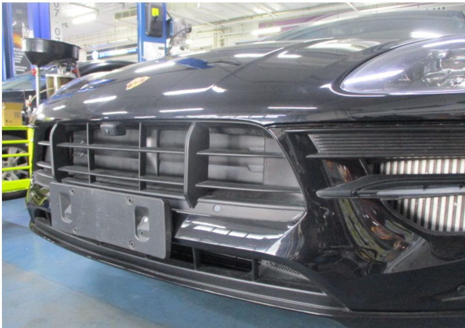
Photo 7 shows a closer view of the Motor Car's front bumper, front bumper centre lower grille, radiator grille, and front number plate garnish. The body parts at the frontal portion of the Motor Car were visually examined and it was observed that the repair/restoration works carried out to the damaged area of the Motor Car (refer to photograph 1 above) were reasonably adequate and in order.
