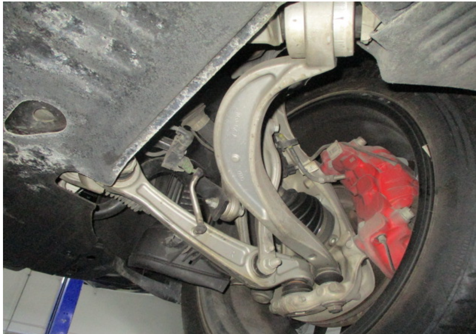
Photo 23 shows the various undercarriage components at the front right wheel of the Motor Car. The mechanical components, control arms and linkages were all found to be intact and secured in an appropriate manner. I also did not observe any fluid leak and/or fluid stain on the underside of the Motor Car.
