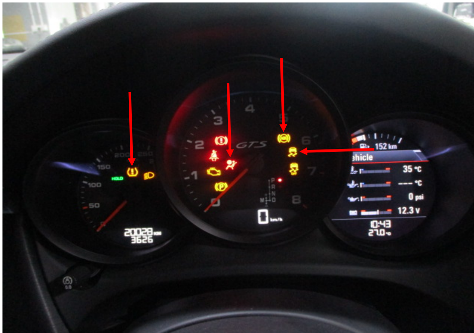
Photo 17 shows the warning lights for the various electronic safety features appearing on the instrument panel of the Motor Car during its self-test when the engine is cranked, in particular the ABS, SRS, TPM and TCS lights (arrowed).
