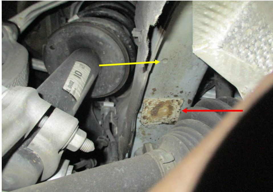
Photo 28 shows the chassis/structural body at the underside front left of the Motor Car. I did not find any weld marks other than original spot weld marks (yellow arrow) on the chassis/structural body of the Motor Car. The original factory sealant (red arrow) at the joints along the chassis/structural body was untouched, indicating no work was done on the chassis/structural body of the Motor Car and that the chassis/structural body was originally fitted.
