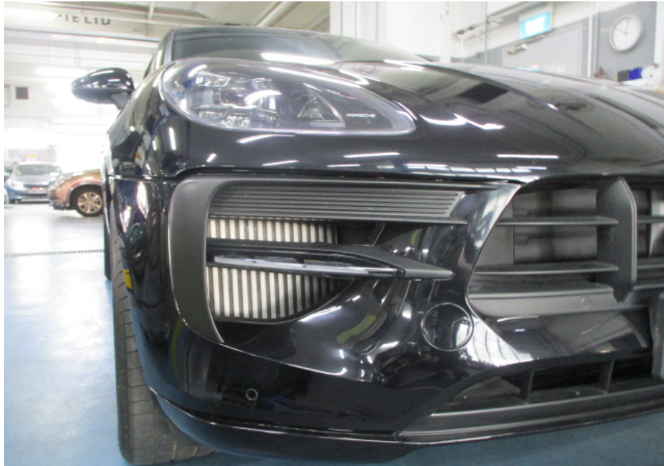
Photo 10 shows a closer view of the Motor Car's front bumper, front bumper front bumper right grille, front right day light and front right headlamp. The body parts at the frontal portion of the Motor Car were visually examined and it was observed that the repair/restoration works carried out to the damaged area of the Motor Car (refer to photograph 1 above) were reasonably adequate and in order.
