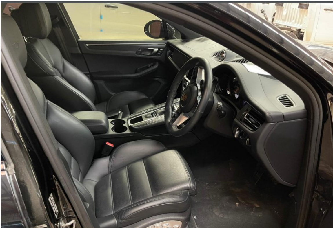
Photo 4 shows the interior compartment of the Motor Car (photograph provided to me). The various parts and components within the interior compartment were all intact and unaffected. The airbag(s) was not deployed as seen from the photographs that were provided to me.
