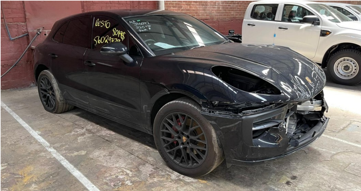
Photo 1 shows the front right body of the Motor Car (photograph provided to me). The Motor Car was observed to have sustained damage at its frontal portion. The front bumper, front bumper centre lower grille, front bumper reinforcement, radiator grille, front bonnet, front bonnet locks, front number plate garnish, front sensor, front support panel, front support panel top garnish, aircon condenser and radiator were amongst the body parts that were observed to have been damaged. The front right headlamp was also observed to be damaged/dislodge/missing.
