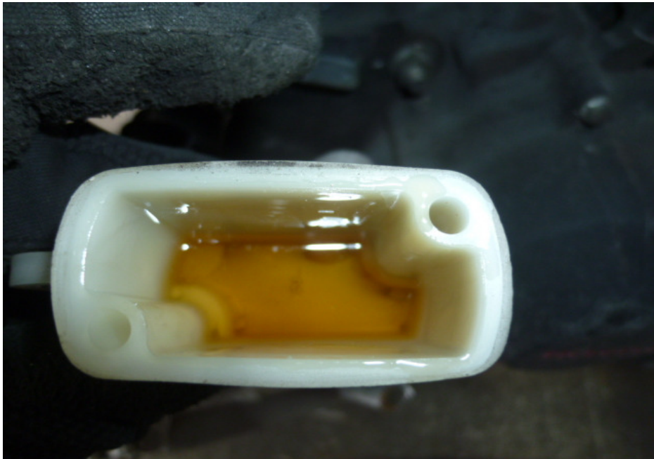
Photo 22 shows the brake fluid reservoir for the rear brake of the Motorcycle. The brake fluid was observed to be of sufficient level for operational purposes and without contamination.
