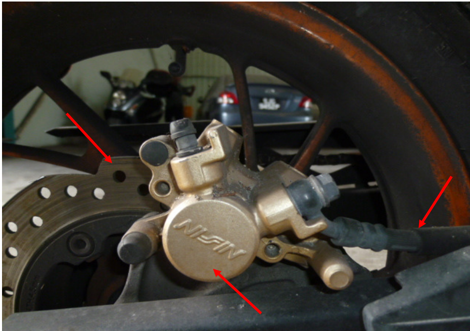
Photo 27 shows a close up view of the rear brake caliper, rear brake disc and rear brake hose (arrowed) of the Motorcycle, which are all part of the components in the hydraulic rear brake system of the Motorcycle. Our visual checks of these various components had revealed all to be intact with no visible damage. No leakage of brake fluid was also observed.
