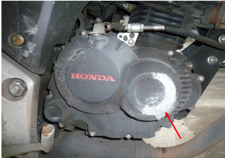
Photo 18 shows the right side of the engine of the Motorcycle at the time of our inspection. The various right engine components had sustained damage of grazing nature as a result of the accident (arrowed) however the engine components were still intact. There was also no fluid leak and/or fluid stain found around the right engine area of the Motorcycle.
