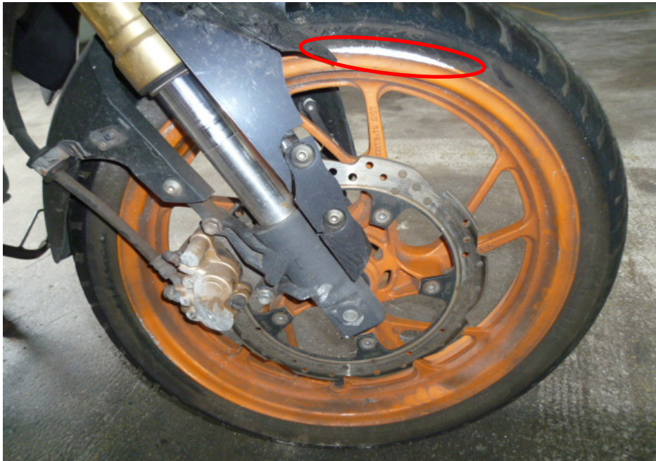
Photo 15 shows the front wheel rim of the Motorcycle at the time of our inspection. Some relatively minor marks of grazing nature were observed on the edges of the front wheel rim (circled), at the right side of the Motorcycle.
