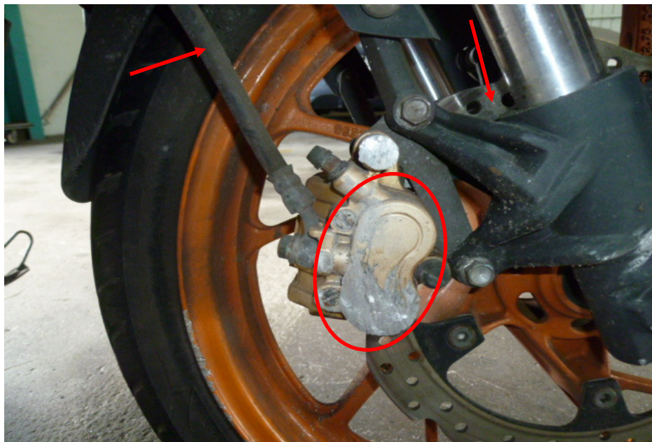
Photo 24 shows a close up view of the front brake disc and front brake hose (arrowed) of the Motorcycle, which are all part of the components in the hydraulic front brake system of the Motorcycle. Our visual checks of these various components had revealed all to be intact with no visible damage. No leakage of brake fluid was also observed. However the front brake caliper had sustained damages of grazing nature as a result of the accident (circled).
