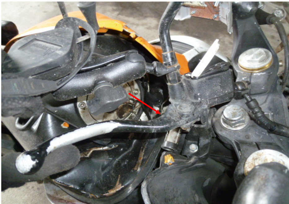
Photo 26 shows the front brake reservoir. We were unable to depress the front brake lever as the front brake clamp had broken off as a result of the accident (arrowed). Hence static as well as operational brake tests could not be conducted on the Motorcycle's front braking system. We were unable to determine if there was any leakage of pressure/vacuum in the front braking system.
