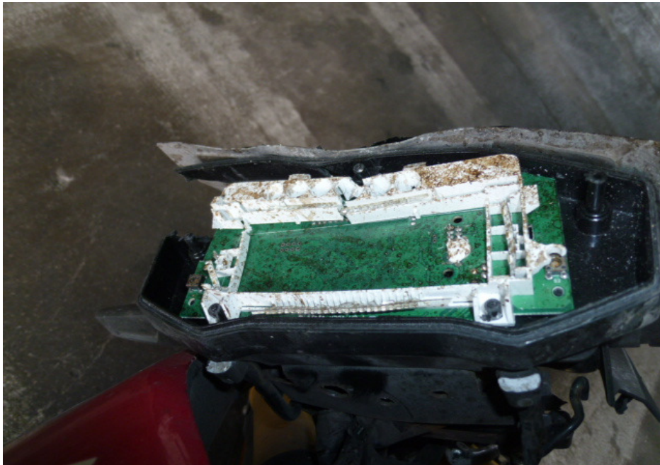
Photo 1 shows the damages sustained to the speedometer gauge of the Motorcycle as a result of the accident. Hence the mileage could not be recorded at the time of our inspection.
