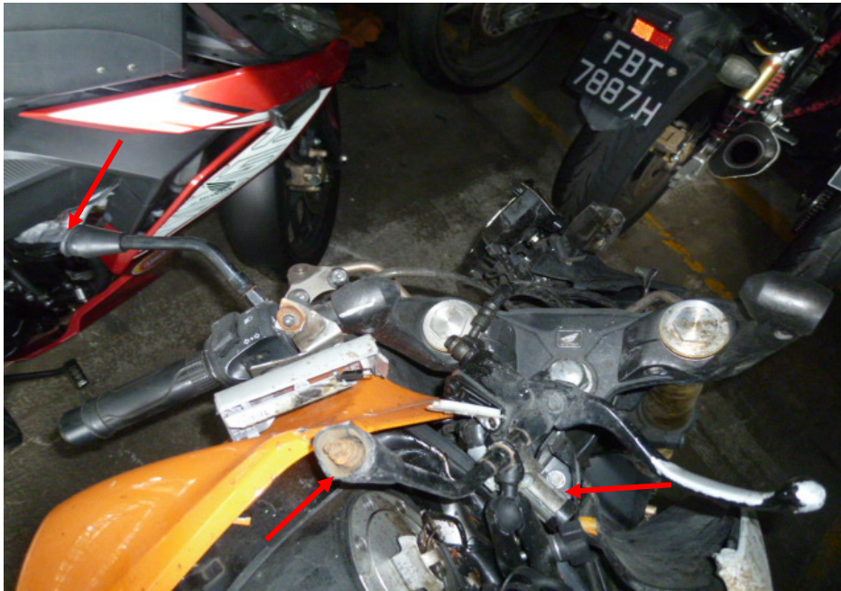
Photo 9 shows a closer view of the handlebars, side mirrors, front brake lever and side mirrors (arrowed) which were amongst the body parts of the Motorcycle that had sustained damage as a result of the accident.
