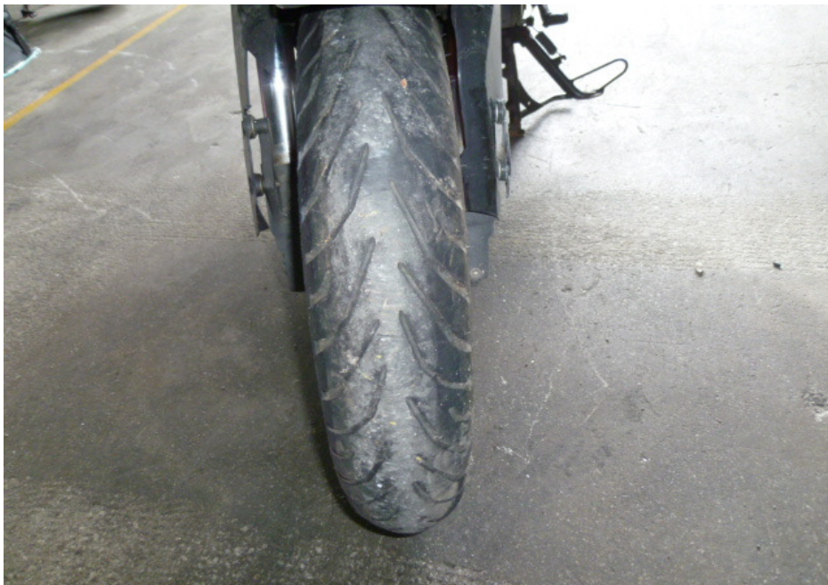
Photo 14 shows the condition of the Motorcycle's front tyre. The front tyre was observed to be in serviceable condition with remaining tread depth of approximately 3mm. There was no tear, burst mark(s) and/or punctured hole(s) on the sidewalls as well as across the tread of the front tyre.
