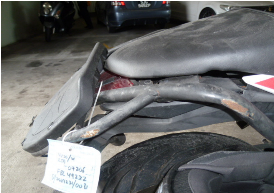
Photo 13 shows a closer view of the deformed top box rack of the Motorcycle as a result of the accident.
