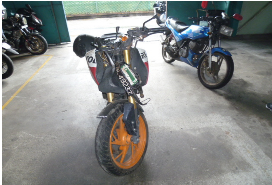
Photo 23 shows the front wheel of the Motorcycle turned towards its full right. Turning the Motorcycle's handle bar towards the left and right did not produce any abnormal free play and/or resistance. This would indicate that the steering system of the Motorcycle was in serviceable condition at the time of our inspection.
