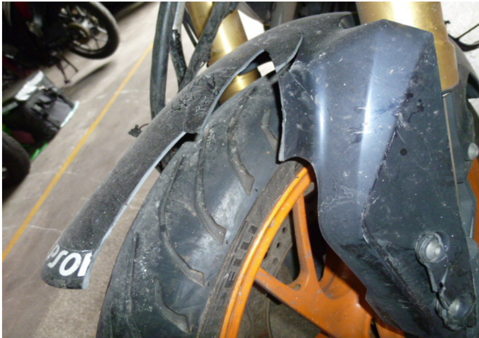
Photo 7 shows a close up view of the cracked front mudguard of the Motorcycle as a result of the accident.
