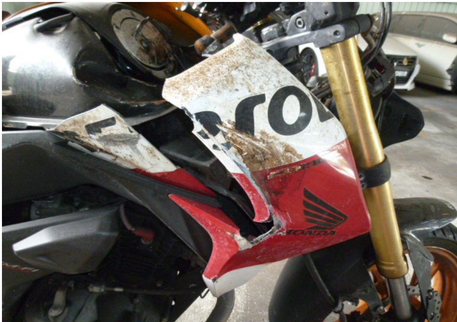
Photo 12 shows a closer view of the cracked right cowling of the Motorcycle as a result of the accident.
