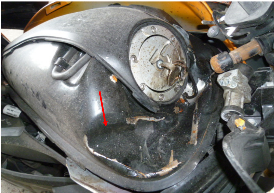
Photo 8 shows a closer view of the dented petrol tank of the Motorcycle as a result of the accident (arrowed).
