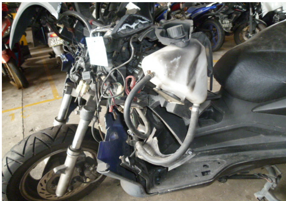
Photo 11 shows the missing left side cowling of the Motorcycle as a result of the accident.
