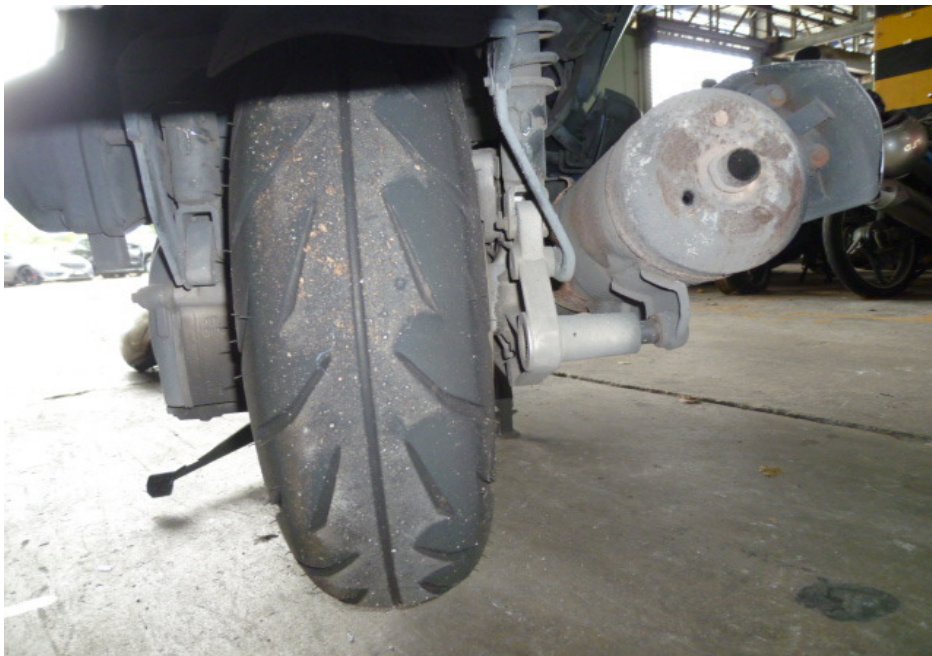
Photo 20 shows the condition of the Motorcycle's rear tyre. The rear tyre was observed to be in serviceable condition with remaining tread depth of approximately 5mm. The tyre was also observed to be sufficiently inflated for vehicular operation. We did not observe any tear, burst mark(s) and/or punctured hole(s) on the sidewalls as well as across the tread of the rear tyre.
