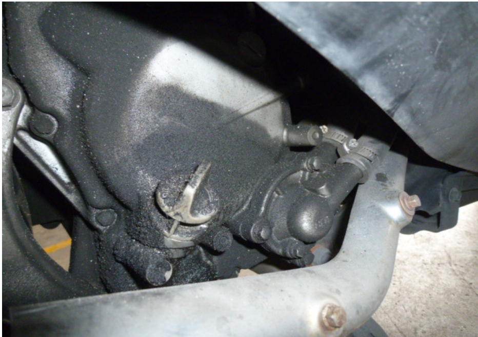
Photo 22 shows the right side of the engine of the Motorcycle at the time of our inspection. The various engine related parts and components were found to be intact with no visible damage. There was also no sign(s) or indication(s) of fluid leak observed around the right engine area of the Motorcycle.
