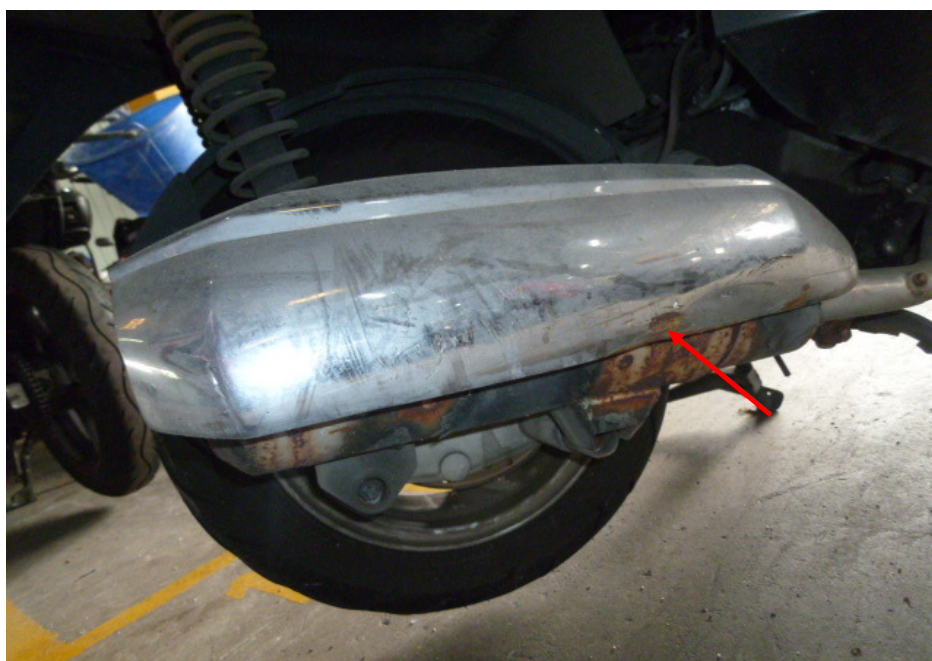
Photo 18 shows a close-up view of the deformed exhaust muffler heat shield of the Motorcycle as a result of the accident (arrowed).
