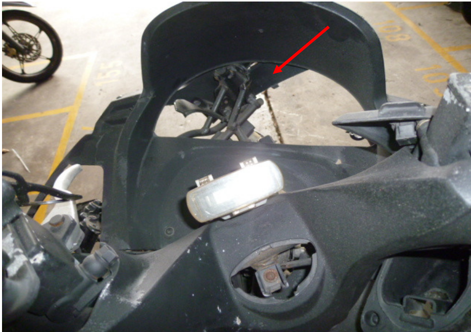
Photo 1 shows the mileage of the Motorcycle which could not be recorded at the time of our inspection due to a missing speedometer gauge (arrowed).
