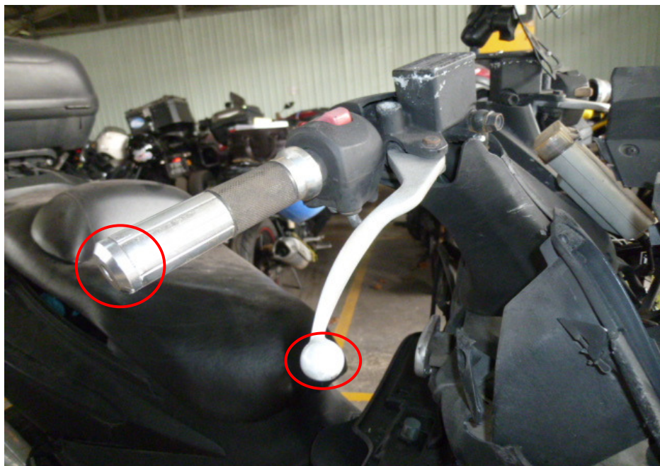
Photo 8 shows a closer view of the right handlebar end and front brake lever of the Motorcycle which were observed to be damaged due to the accident (circled).
