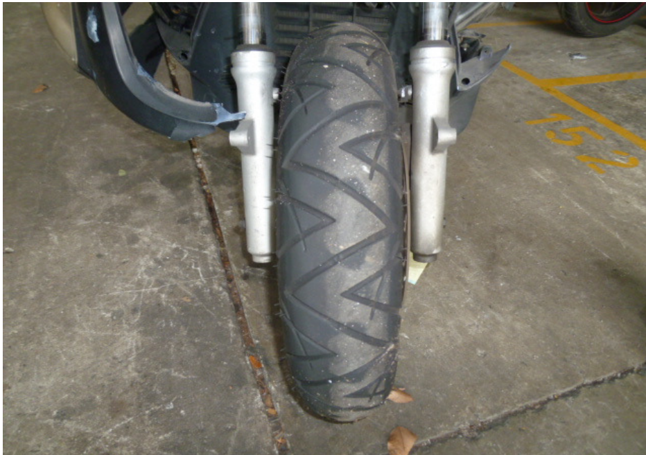
Photo 19 shows the condition of the Motorcycle's front tyre. The front tyre was observed to be in serviceable condition with remaining tread depth of approximately 6mm. There was no tear, burst mark(s) and/or punctured hole(s) on the sidewalls as well as across the tread of the front tyre.
