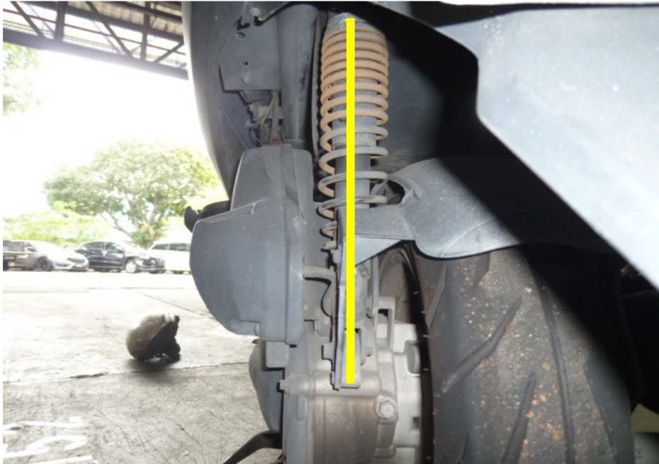
Photo 24 shows the left shock absorber of the Motorcycle which was found to be intact without any misalignment.
