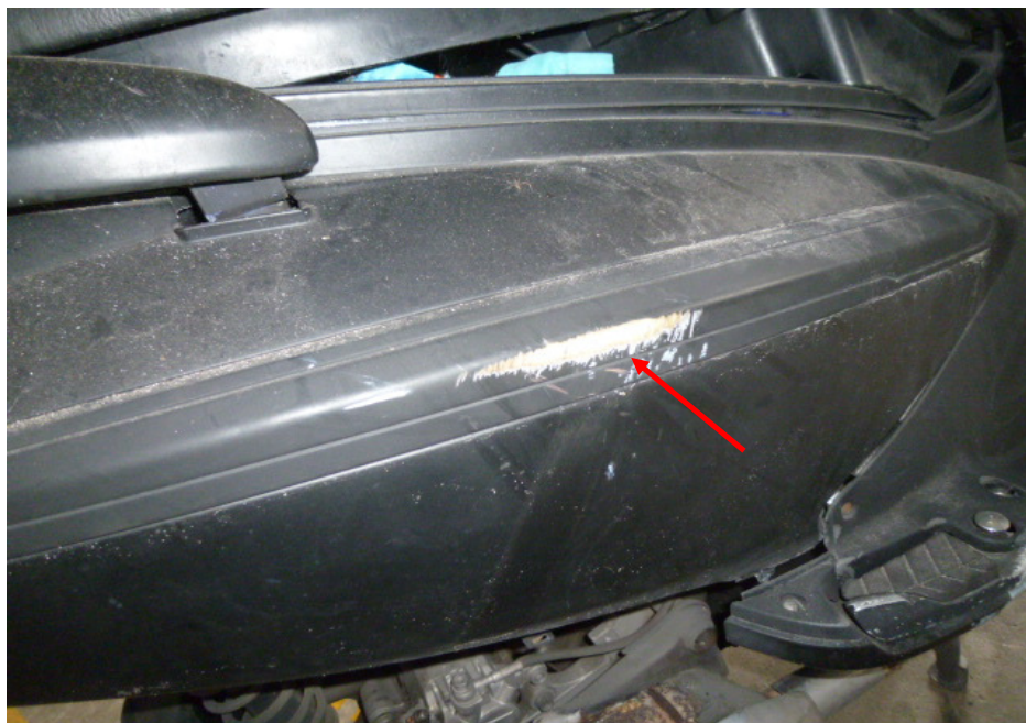
Photo 15 shows a close-up view of the grazed right rear side cover of the Motorcycle as a result of the accident (arrowed).
