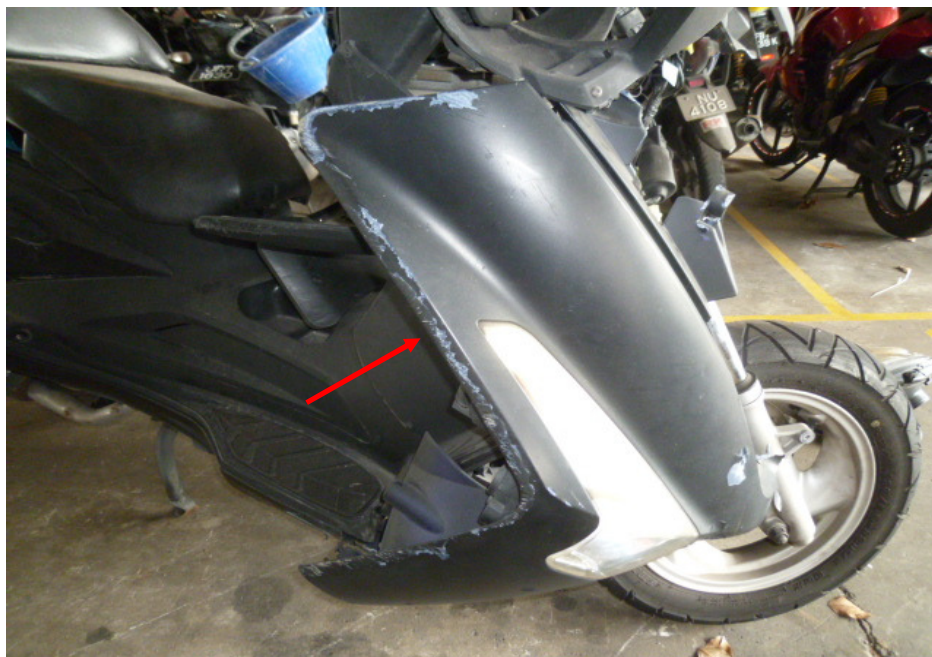
Photo 9 shows a general view of the grazed right cowling of the Motorcycle as a result of the accident (arrowed).
