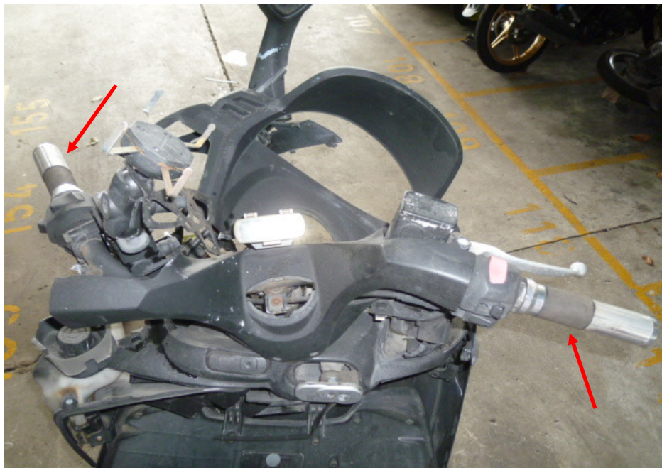
Photo 26 shows the handlebar of the Motorcycle. The handlebar was observed to be bent (arrowed) as a result of the accident. We were hence not able to conduct any tests on the steering system of the Motorcycle.
