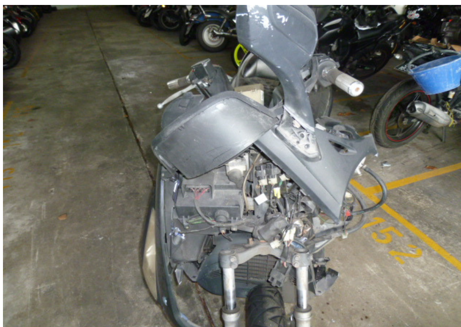
Photo 6 shows a closer view of the missing head cowl of the Motorcycle as a result of the accident.
