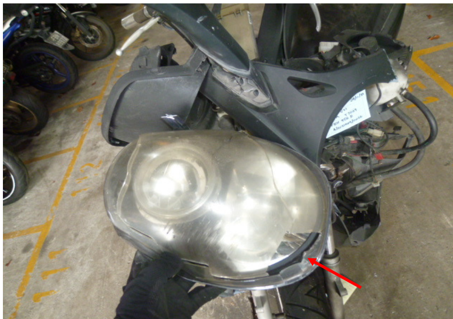
Photo 5 shows a closer view of the cracked headlight of the Motorcycle at the time of our inspection (arrowed).
