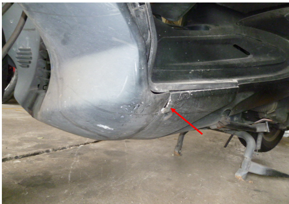
Photo 12 shows a close-up view of the cracked left bottom cowling of the Motorcycle as a result of the accident (arrowed).
