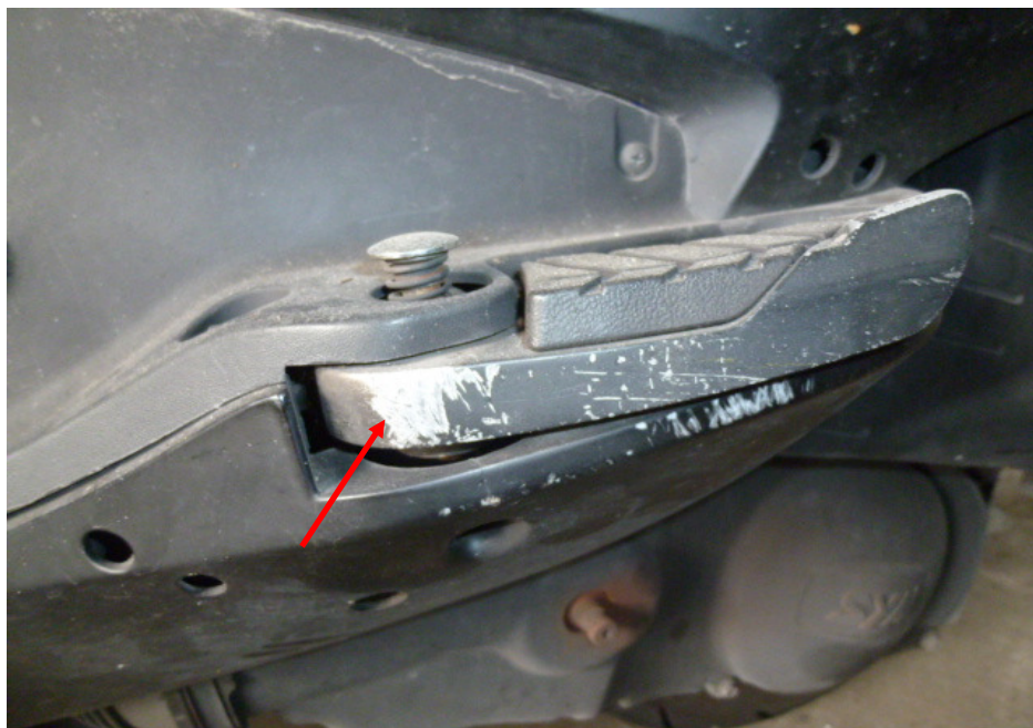
Photo 13 shows a close-up view of the grazed left pillion foot peg of the Motorcycle as a result of the accident (arrowed).
