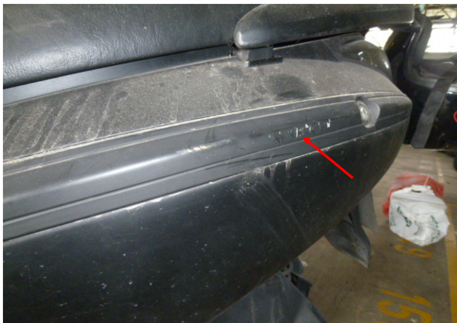
Photo 16 shows a close-up view of the grazed left rear side cover of the Motorcycle as a result of the accident (arrowed).
