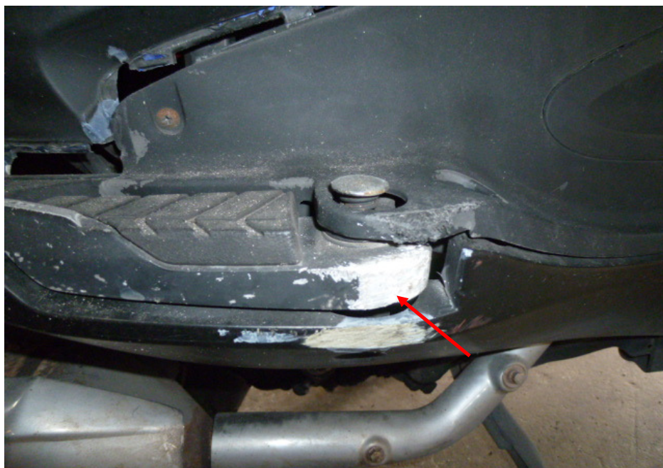
Photo 14 shows a close-up view of the grazed right pillion foot peg of the Motorcycle as a result of the accident (arrowed).
