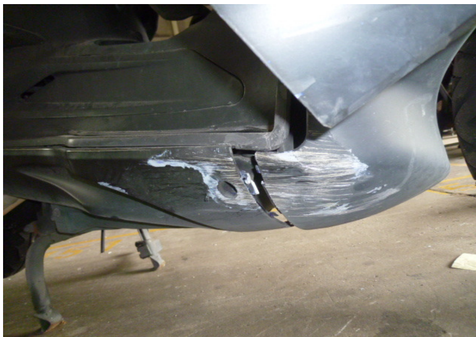
Photo 10 shows a close-up view of the cracked right bottom cowling of the Motorcycle as a result of the accident.
