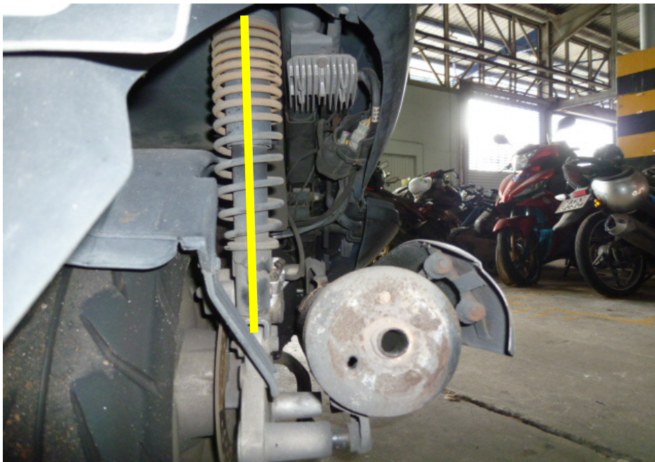
Photo 25 shows the right shock absorber of the Motorcycle which was found to be intact without any misalignment.
