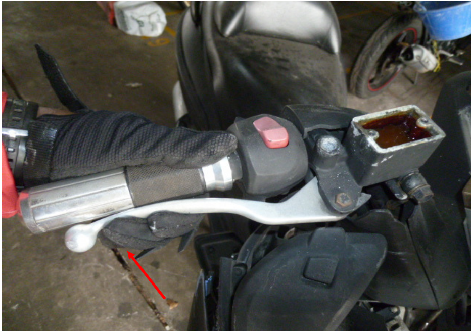
Photo 29 shows the front brake lever being depressed. There was no resistance felt (spongy like feel) upon pressing the front brake lever (arrowed). This would indicate that there may be a leakage of pressure/vacuum in the front brake system.
