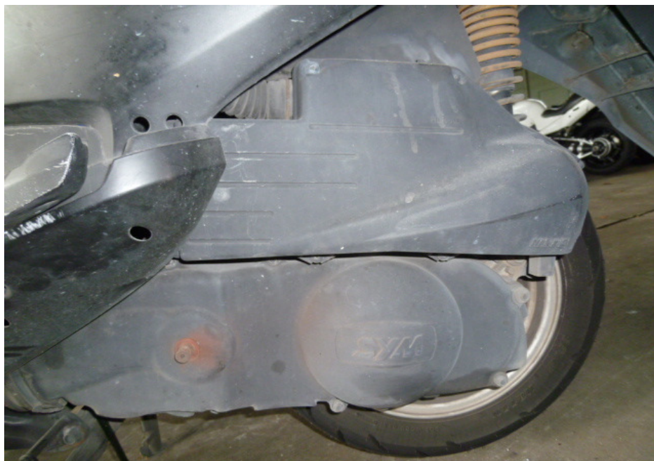
Photo 23 shows the drive train cover of the Motorcycle which was found to be intact without any misalignment.
