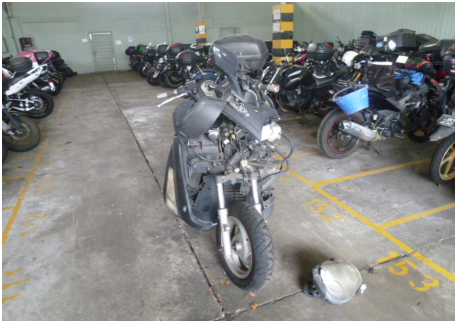
Photo 4 shows a general view of the frontal portion of the Motorcycle at the time of our inspection. The Motorcycle was observed to have sustained damages all around. The body parts that were found to have been damaged include its handlebar, head cowlings, headlight, side cowlings, front brake lever, right handlebar end, radiator, bottom cowlings, pillion foot pegs, rear side covers, top box and exhaust muffler heat shield, amongst others as a result of the accident.
