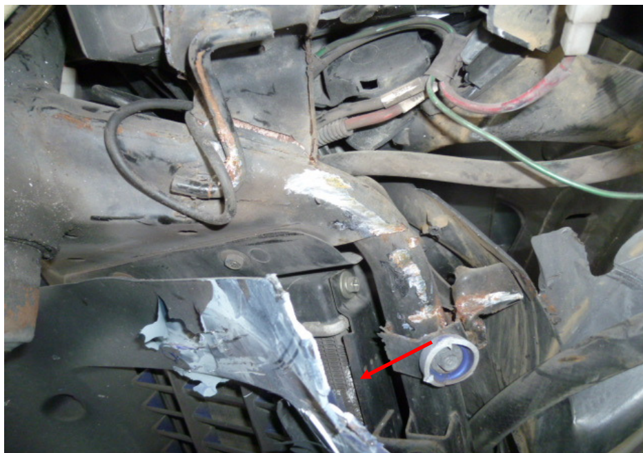
Photo 7 shows a closer view of the deformed radiator which was amongst the body parts at the front body of the Motorcycle that had sustained damage as a result of the accident (arrowed).
