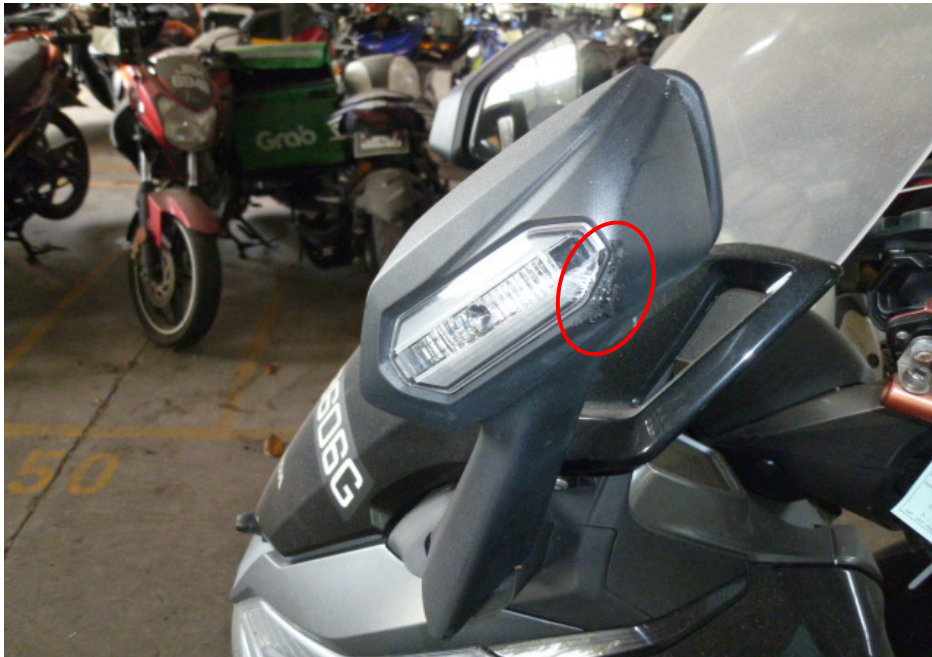
Photo 5 shows a closer view of the grazed left side mirror of the Motorcycle at the time of our inspection (circled).
