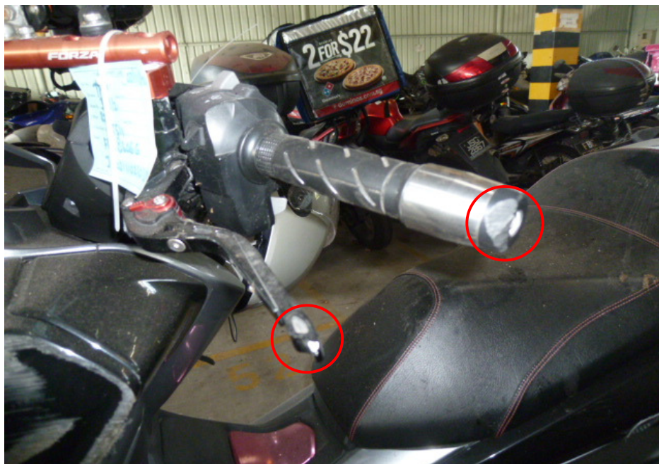
Photo 7 shows a closer view of the left handlebar end and rear brake lever of the Motorcycle which was observed to be damaged due to the accident (circled).
