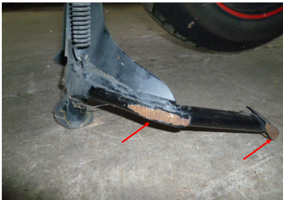
Photo 12 shows a closer view of the grazed main stand of the Motorcycle as a result of the accident (arrowed).
