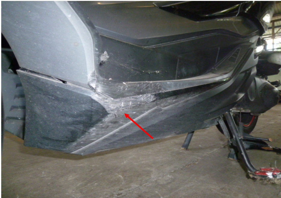
Photo 9 shows a closer view of the grazed left bottom cowling of the Motorcycle as a result of the accident (arrowed).
