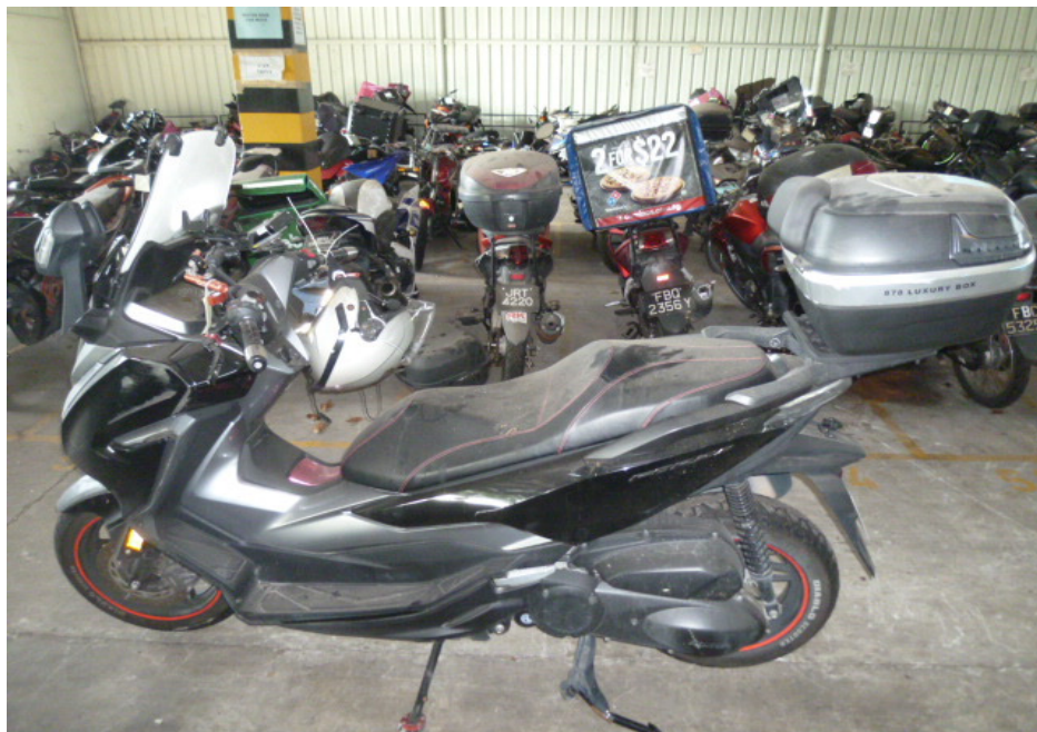
Photo 4 shows a general view of the left body of the Motorcycle at the time of our inspection. The Motorcycle was observed to have sustained damages at its frontal portion and left body. The body parts that were found to have been damaged include its front mudguard, left side mirror, left handlebar end, rear brake lever, left cowling, left bottom cowling, side stand, main stand, left rear side cover and top box, amongst others as a result of the accident
