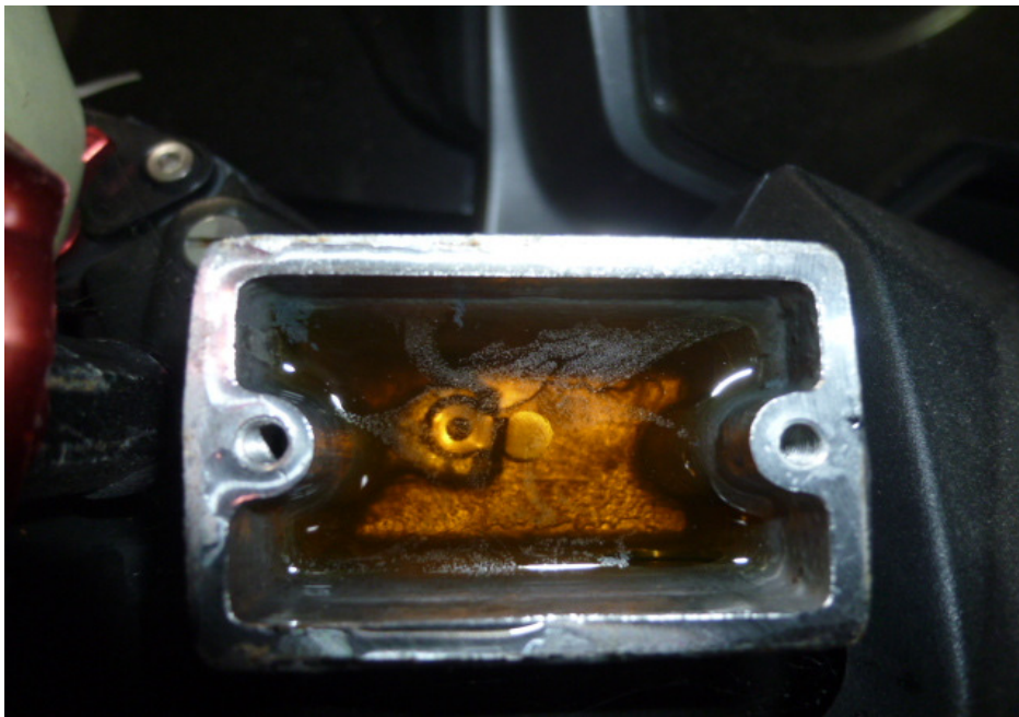
Photo 26 shows the brake fluid reservoir for the rear brake of the Motorcycle. The brake fluid was observed to be of sufficient level for operational purposes and without any contamination.
