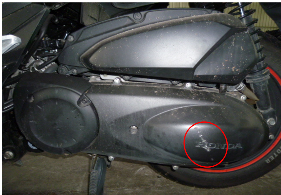
Photo 17 shows the drive train of the Motorcycle which was found to be intact without any misalignment. However the drive train cover had sustained damages of grazing nature as a result of the accident (circled). Upon examination of the Motorcycle's engine area, we had observed that the various engine related parts and components were intact with no visible damage. There was also no sign(s) or indication(s) of fluid leak observed around the engine area of the Motorcycle.
