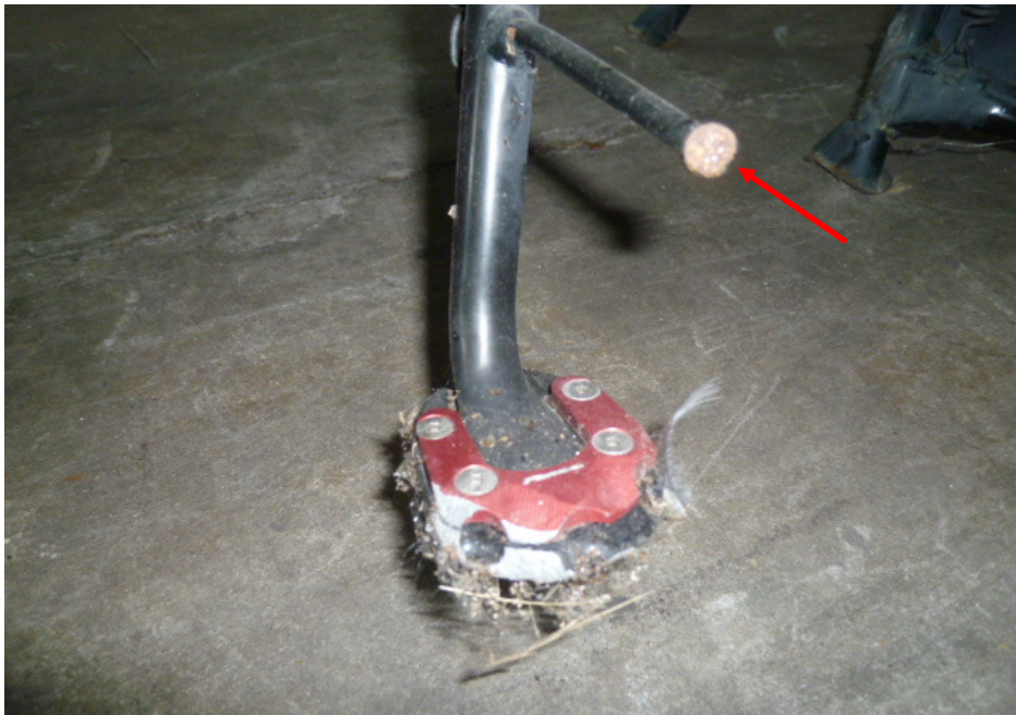
Photo 10 shows a closer view of the grazed side stand of the Motorcycle at the time of our inspection (arrowed).
