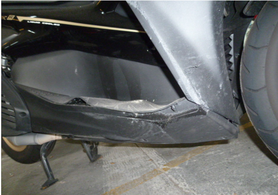
Photo 7 shows a closer view of the right bottom cowling of the Motorcycle which was observed to be damaged due to the accident.
