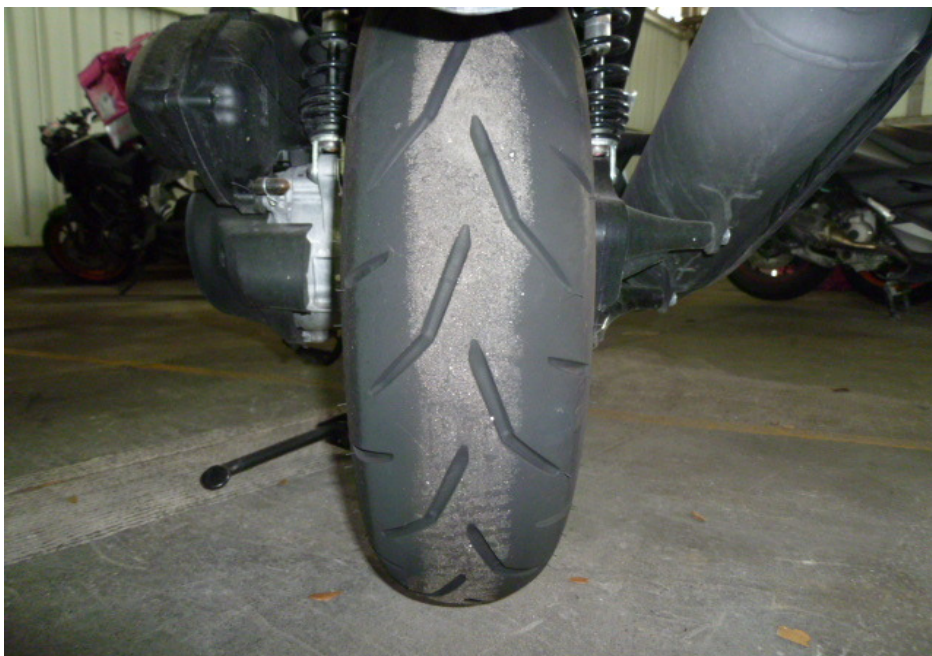
Photo 14 shows the condition of the Motorcycle's rear tyre. The rear tyre was observed to be in serviceable condition with remaining tread depth of approximately 8mm. The tyre was also observed to be sufficiently inflated for vehicular operation. We did not observe any tear, burst mark(s) and/or punctured hole(s) on the sidewalls as well as across the tread of the rear tyre.
