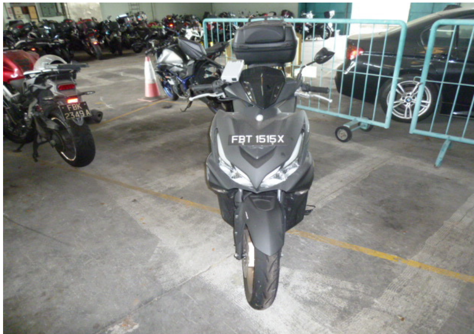
Photo 1 shows a general view of the frontal portion of the Motorcycle at the time of our inspection. The Motorcycle was observed to have sustained damages at its frontal portion and right body. The mileage of the Motorcycle could not be recorded at the time of our inspection due to the flat battery of the key fob.
