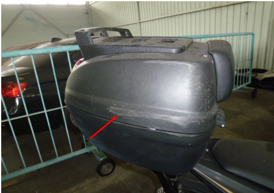
Photo 12 shows a closer view of the grazed top box (arrowed) of the Motorcycle as a result of the accident.
