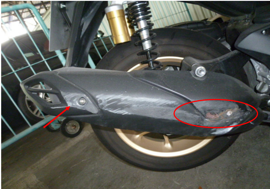
Photo 11 shows a closer view of the grazed exhaust muffer heat shield (arrowed) and dented exhaust muffer (arrowed) of the Motorcycle as a result of the accident.
