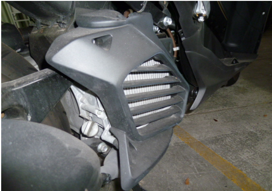
Photo 16 shows the radiator of the Motorcycle at the time of our inspection. The radiator was found to be intact with no visible damage. There was also no sign(s) or indication(s) of fluid leak observed around the radiator of the Motorcycle.
