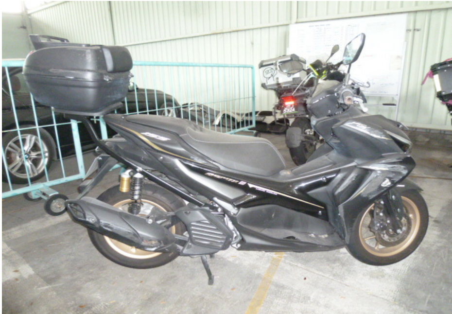
Photo 3 shows a general view of the right body of the Motorcycle at the time of our inspection. The Motorcycle was observed to have sustained damages at its frontal portion and right body. The body parts that were found to have been damaged include its front mudguard, right cowling, right side mirror, front brake lever, right handlebar end, right bottom cowling, right pillion foot peg, right rear side cover, top box rack, exhaust muffler heat shield, exhaust muffler and rear number plate, amongst others as a result of the accident.
