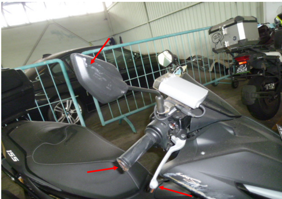
Photo 4 shows a closer view of the front brake lever, right side mirror and right handlebar end of the Motorcycle which were observed to be damaged due to the accident (arrowed).
