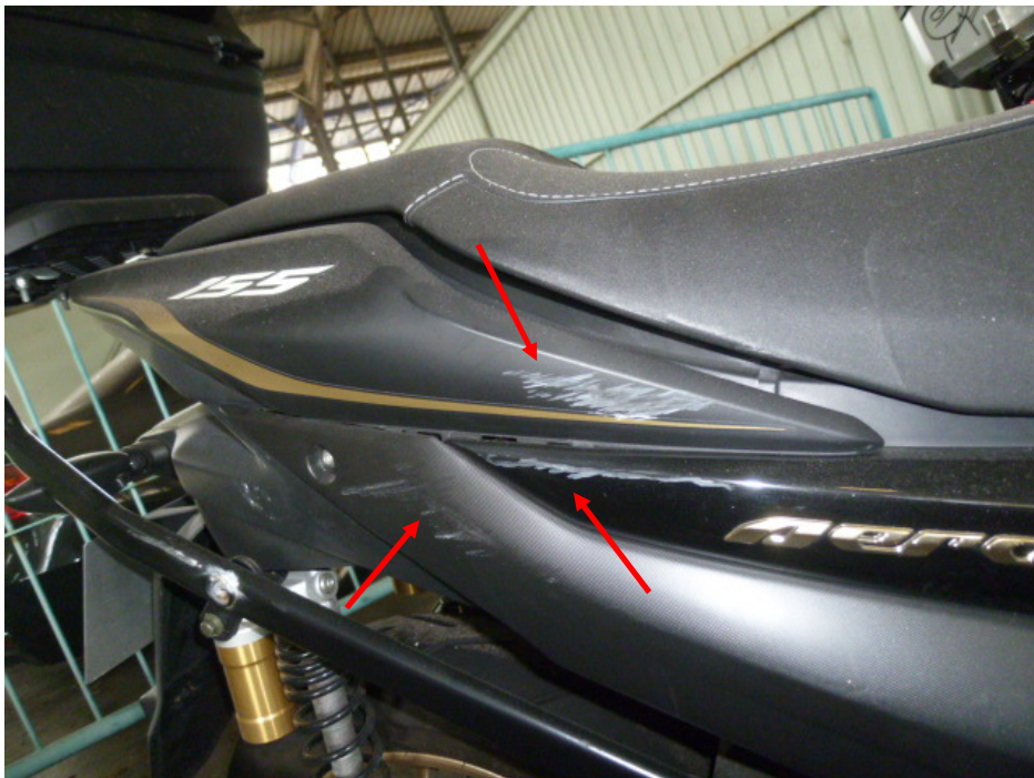
Photo 10 show a closer view of the right rear side cover of the Motorcycle which was observed to be damaged due to the accident (arrowed).
