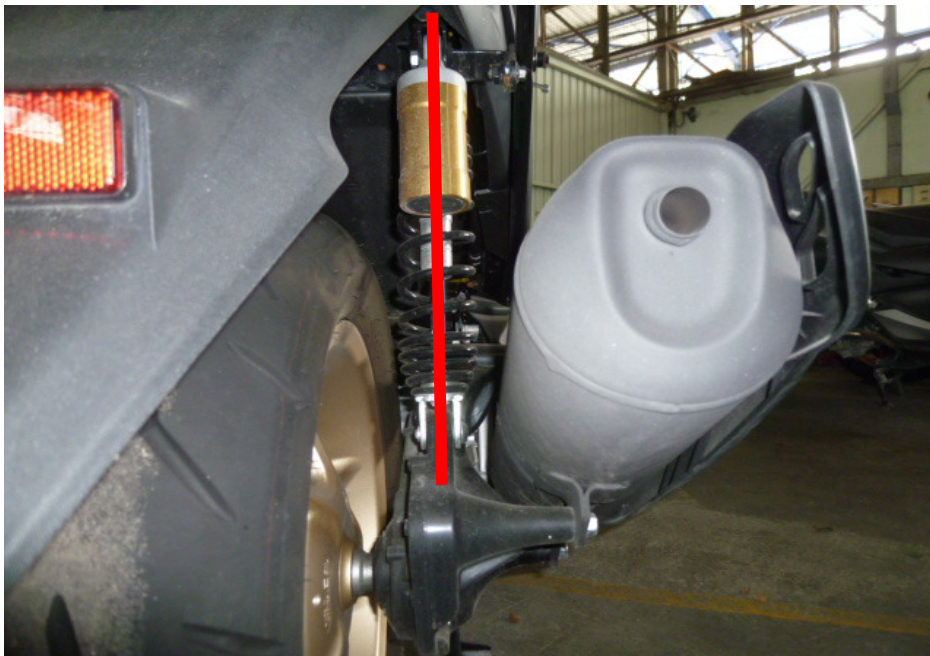
Photo 19 shows the right shock absorber of the Motorcycle which was found to be intact without any misalignment.
