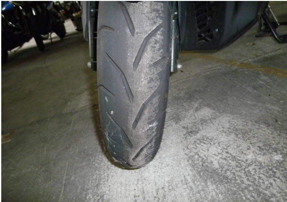
Photo 13 shows the condition of the Motorcycle's front tyre. The front tyre was observed to be in serviceable condition with remaining tread depth of approximately 6mm. There was no tear, burst mark(s) and/or punctured hole(s) on the sidewalls as well as across the tread of the front tyre.
