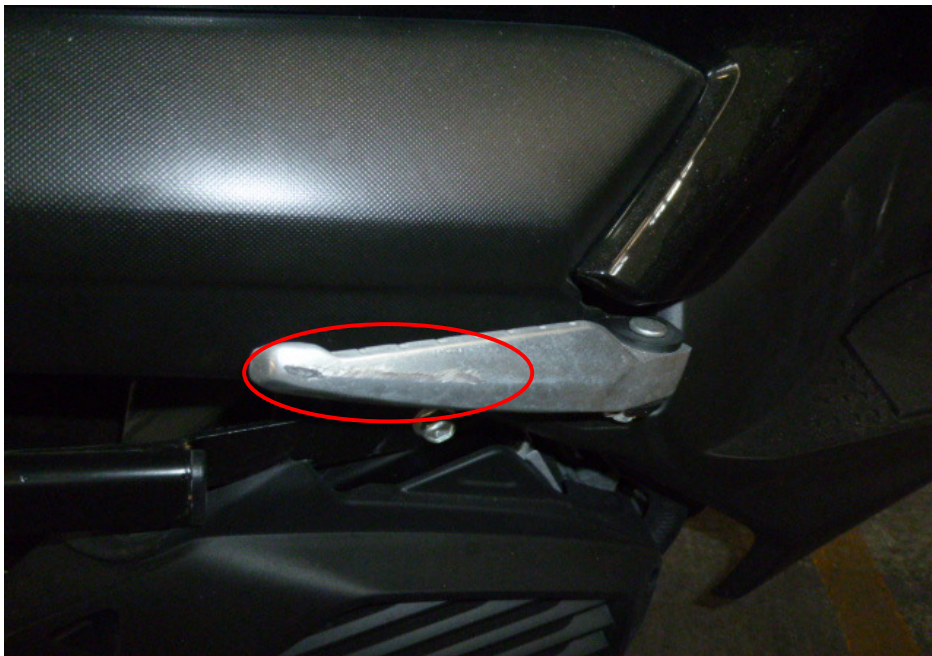
Photo 8 shows a closer view of the grazed right pillion foot peg (circled) of the Motorcycle at the time of our inspection.
