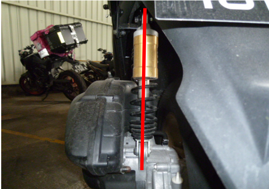
Photo 18 shows the left shock absorber of the Motorcycle which was found to be intact without any misalignment.
