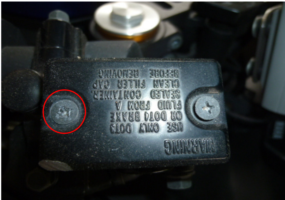
Photo 25 shows the brake fluid reservoir cover for the front brake of the Motorcycle. We were unable to examine whether the front brake fluid was without contamination due to the worn out screw (circled).
