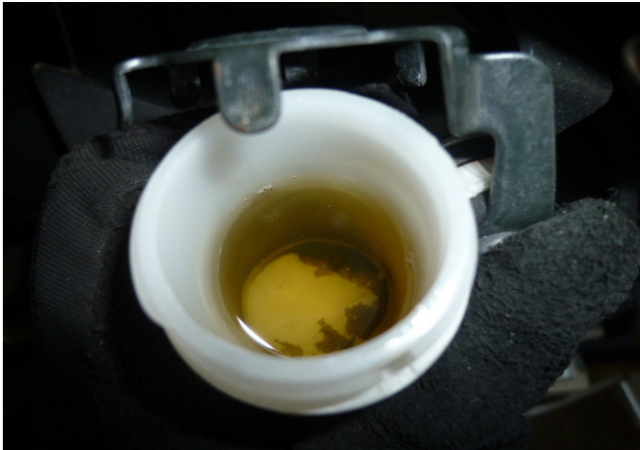
Photo 29 shows a close up view of the brake fluid reservoir for the rear brake of the Motorcycle. The rear brake fluid was observed to be of sufficient level for operational purposes and without contamination.
