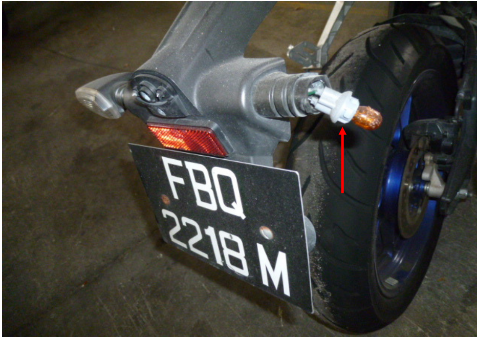
Photo 12 shows a closer view of the broken right rear signal lamp (arrowed) of the Motorcycle as a result of the accident.
