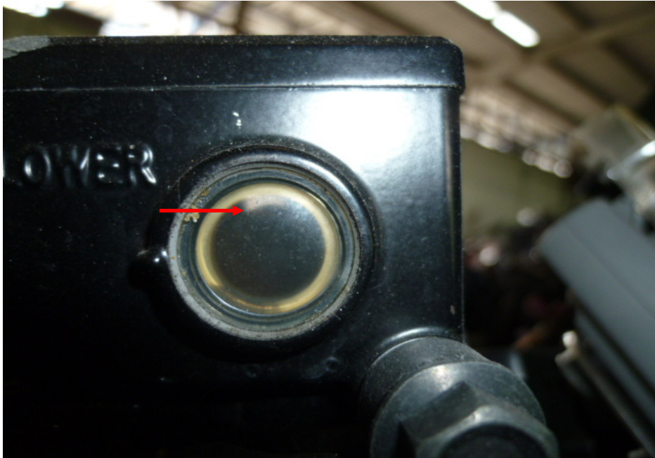
Photo 26 shows a close up view of the brake fluid reservoir for the front brake of the Motorcycle. The brake fluid was observed to be of sufficient level for operational purposes (arrowed).
