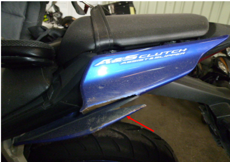
Photo 11 shows a closer view of the cracked left rear side cover of the Motorcycle as a result of the accident (arrowed).
