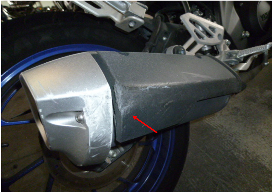
Photo 14 shows the grazed exhaust muffler heat shield of the Motorcycle as a result of the accident (arrowed).
