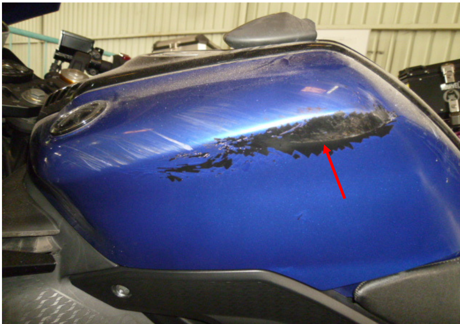
Photo 9 shows a closer view of the dented petrol tank of the Motorcycle as a result of the accident (arrowed).
