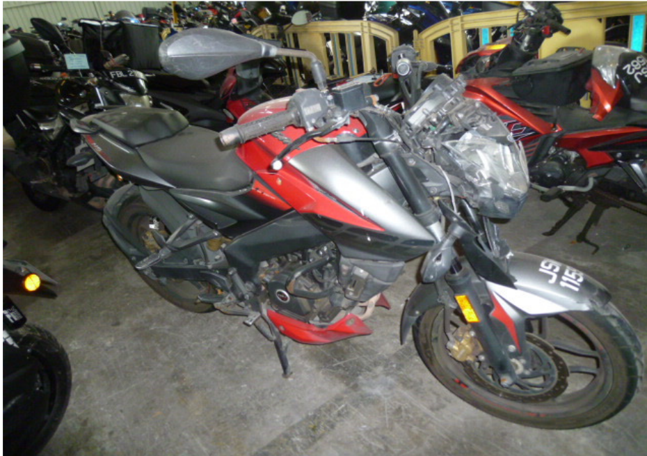
Photo 4 shows a general view of the right body of the Motorcycle at the time of our inspection. The Motorcycle was observed to have sustained damages all around. The body parts that were found to have been damaged include its head cowl, headlight assembly, front mudguard, left cowl, right side mirror, front brake lever, right engine crashbar, rear brake pedal, right front footrest, rear side covers, rear number plate and rear reflector, amongst others.
