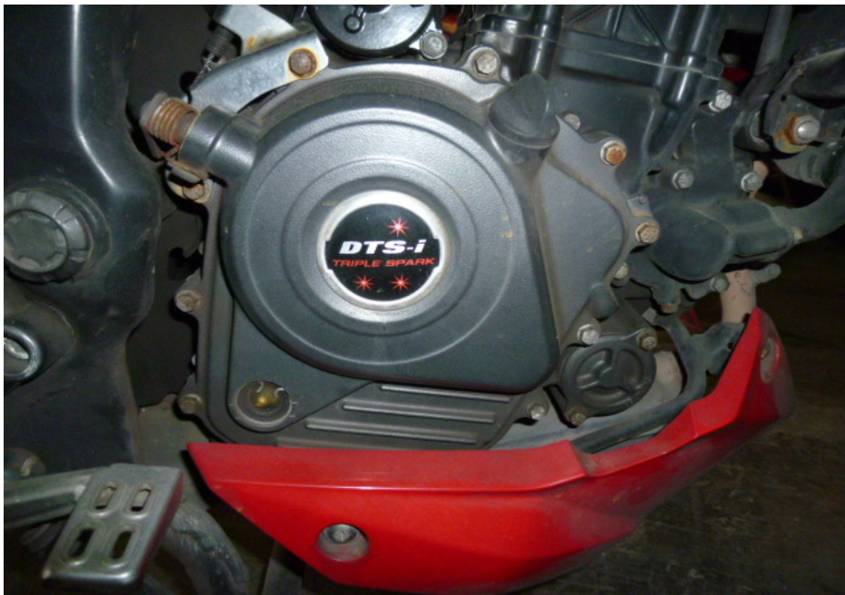
Photo 18 shows the right side of the engine of the Motorcycle at the time of our inspection. The various engine related parts and components were found to be intact with no visible damage. There was also no sign(s) or indication(s) of fluid leak observed around the right engine area of the Motorcycle.
