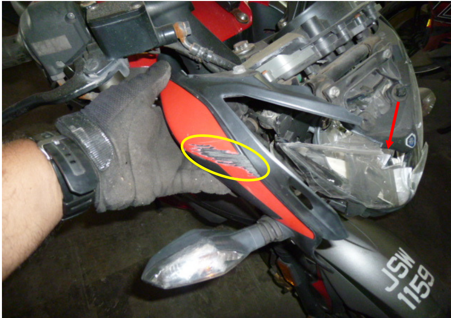
Photo 6 shows the grazed head cowling (circled) and cracked headlight assembly (arrowed), which were amongst the body parts of the Motorcycle that had sustained damage as a result of the accident.
