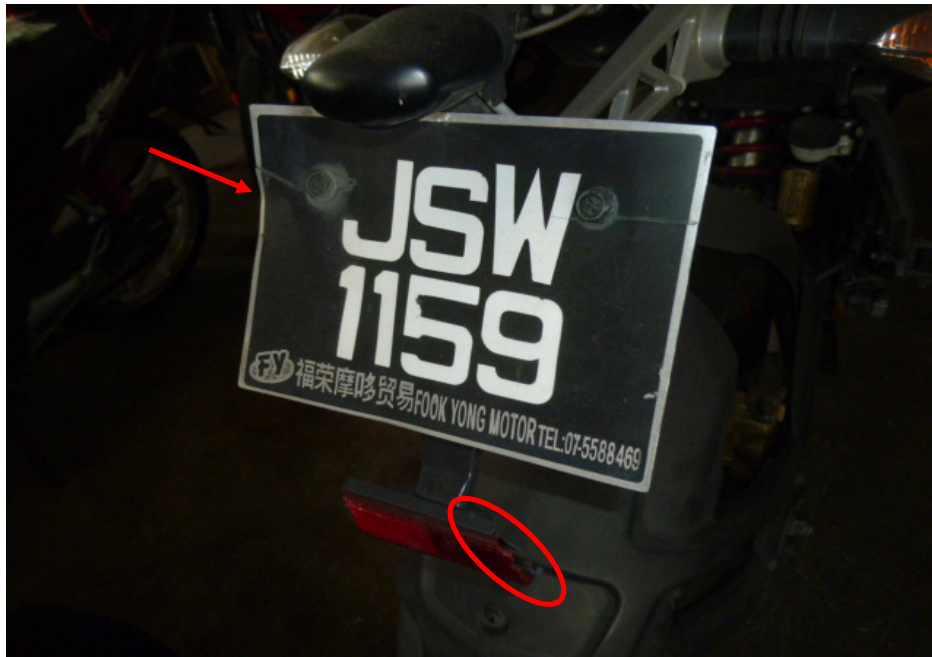
Photo 12 shows a closer view of the broken rear reflector (circled) and dented rear number plate (arrowed) of the Motorcycle as a result of the accident.
