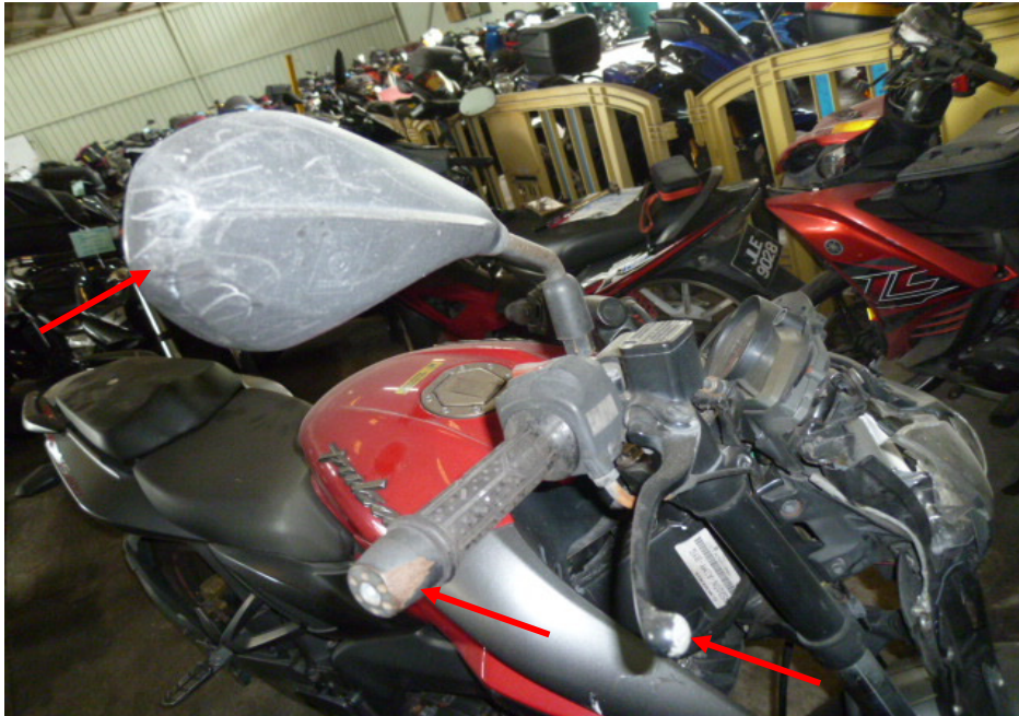
Photo 8 shows the right handlebar end, front brake lever and right side mirror (arrowed), which were amongst the body parts of the Motorcycle that had sustained damage as a result of the accident.
