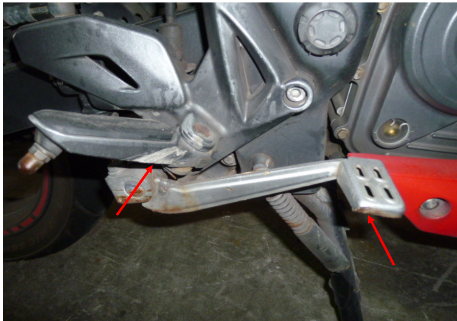
Photo 13 shows the rear brake pedal and right front footrest of the Motorcycle that had sustained damage as a result of the accident (arrowed).
