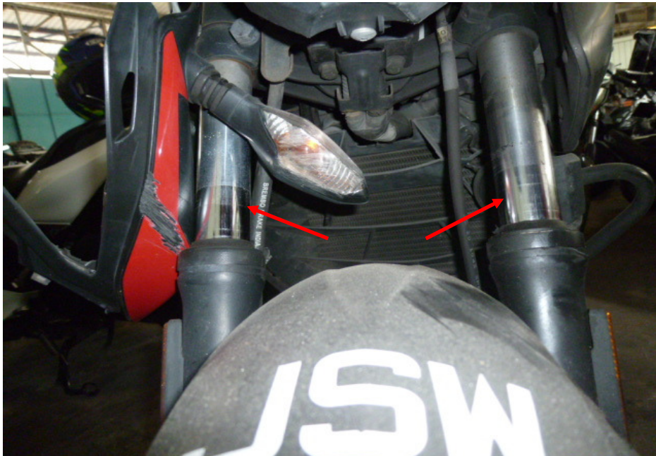
Photo 21 shows the front forks (arrowed) of the Motorcycle. The front forks and fork bracket of the Motorcycle were both found to be intact and undamaged. Turning the Motorcycle's handle bar towards the left and right did not produce any abnormal free play. The steering system of the Motorcycle was in serviceable condition at the time of our inspection.
