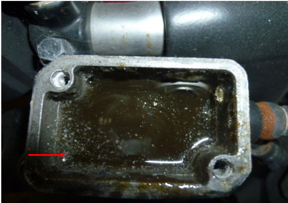
Photo 25 shows a close up view of the brake fluid reservoir for the front brake of the Motorcycle. The front brake fluid was observed to be of sufficient level for operational purposes. However it was found to be contaminated (arrowed).
