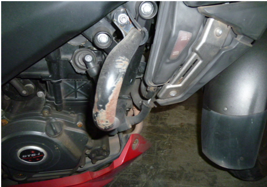
Photo 7 shows a closer view of the grazed right engine crashbar of the Motorcycle as a result of the accident.
