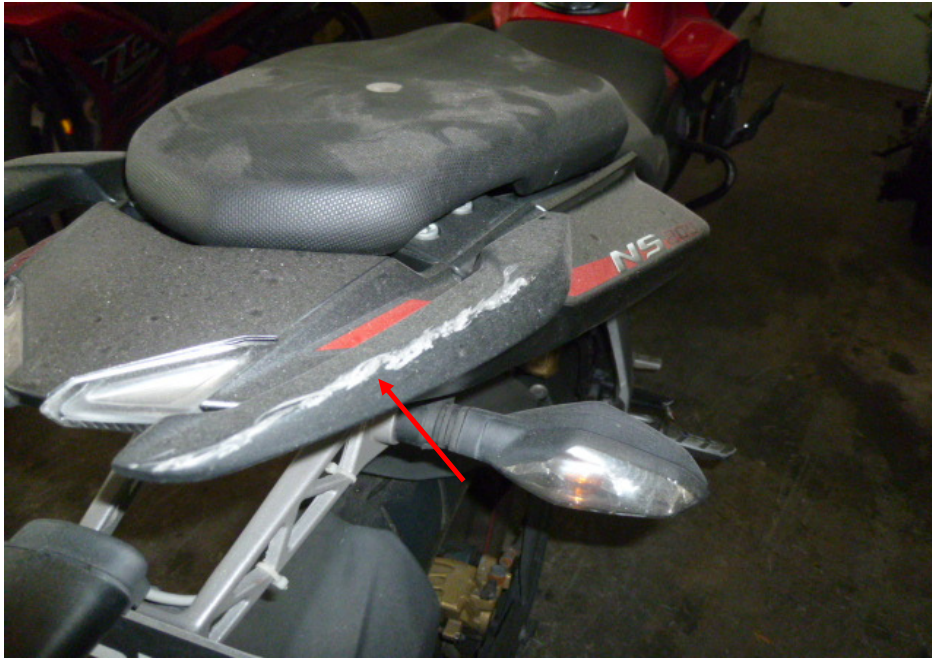
Photo 14 shows the grazed right rear side cover of the Motorcycle as a result of the accident (arrowed).
