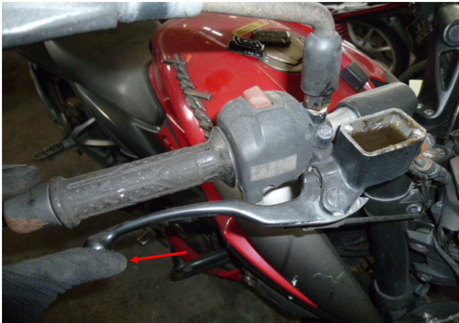
Photo 26 shows the front brake lever being depressed. There was some resistance felt (spongy like feel) upon pressing the front brake lever (arrowed). This would indicate that there is no leakage of pressure/vacuum in the front brake system.
