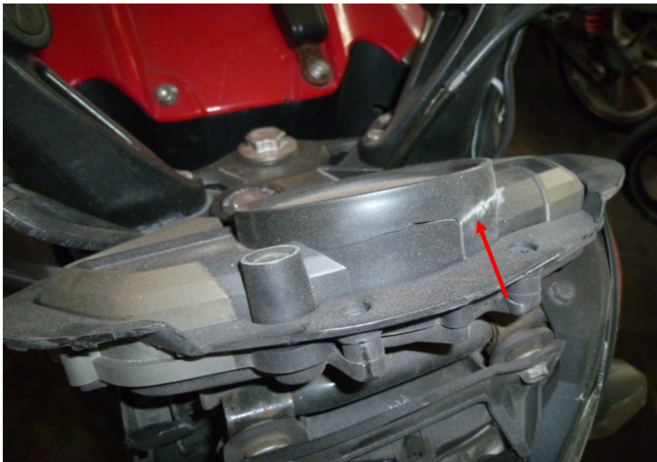
Photo 9 shows a closer view of the grazed speedometer gauge of the Motorcycle as a result of the accident (arrowed).
