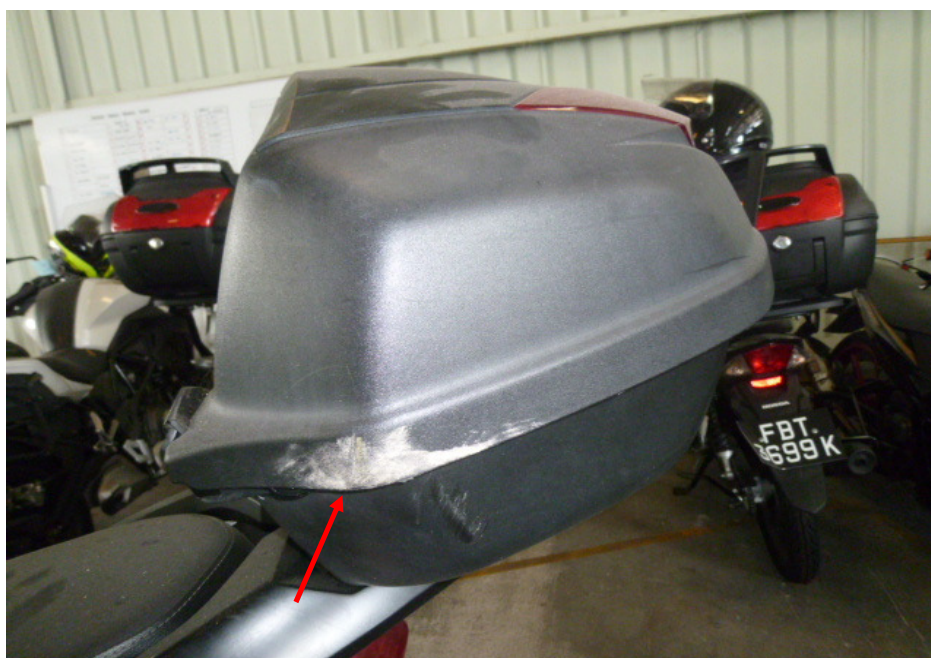
Photo 13 shows a closer view of the grazed top box of the Motorcycle as a result of the accident (arrowed).
