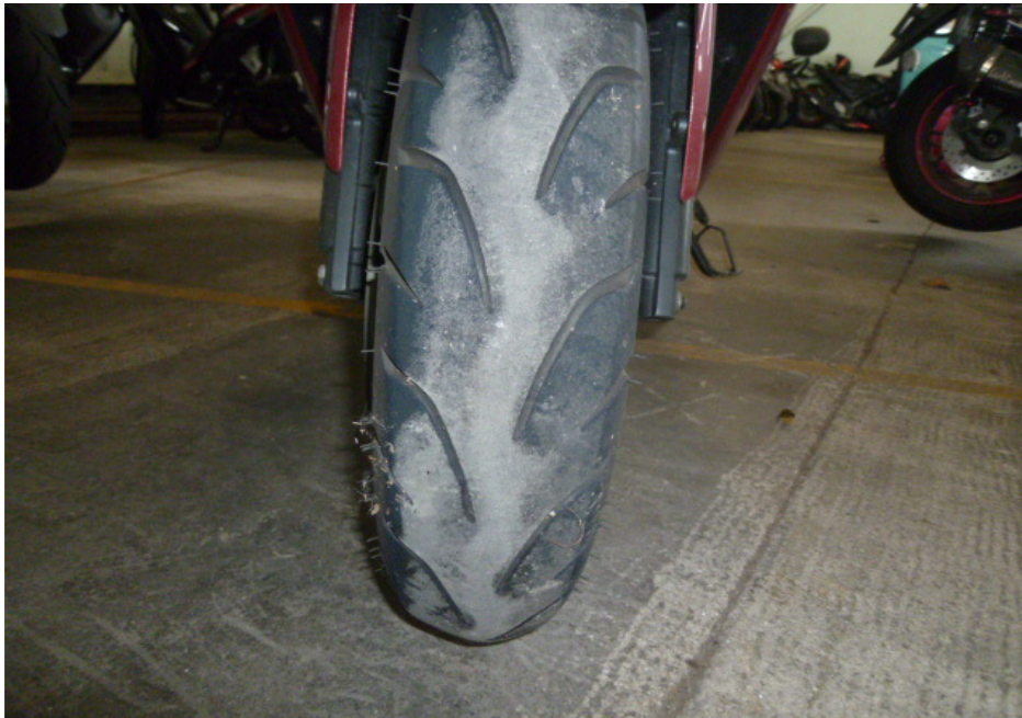
Photo 14 shows the condition of the Motorcycle's front tyre. The front tyre was observed to be in serviceable condition with remaining tread depth of approximately 4mm. There was no tear, burst mark(s) and/or punctured hole(s) on the sidewalls as well as across the tread of the front tyre.
