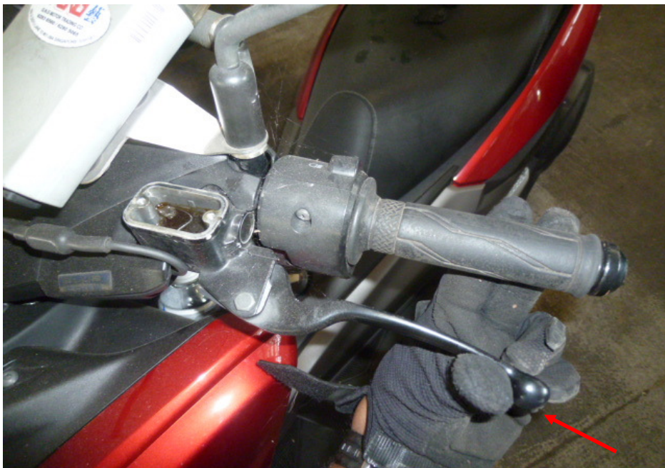
Photo 28 shows the rear brake lever being depressed. There was some resistance felt (spongy like feel) upon pressing the rear brake lever (arrowed). This would indicate that there is no leakage of pressure/vacuum in the rear brake system.
