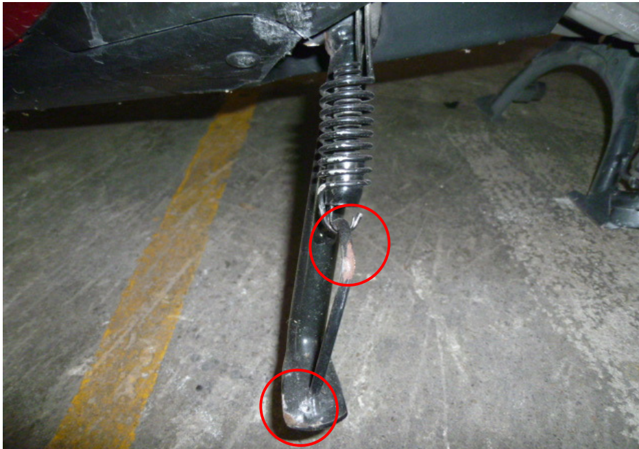
Photo 9 shows the grazed side stand (circled) of the Motorcycle as a result of the accident.
