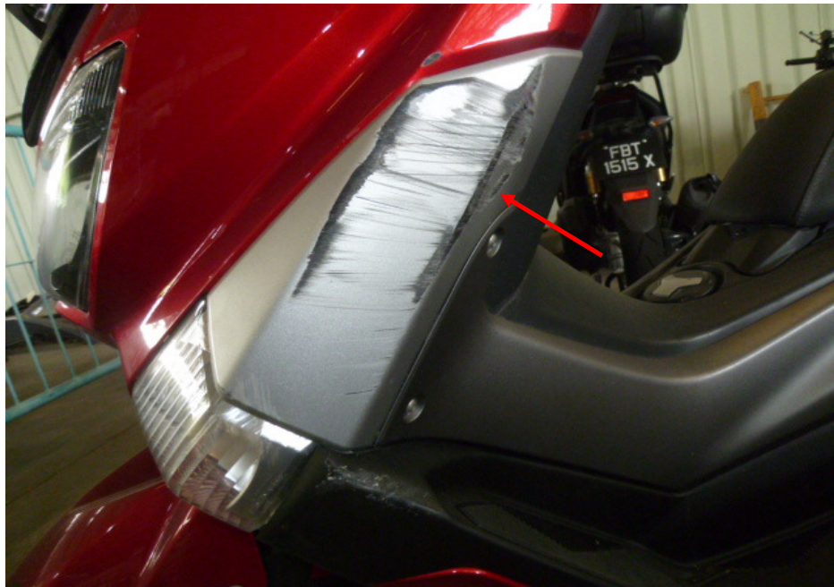
Photo 8 shows a close-up view of the grazed left cowling of the Motorcycle at the time of our inspection (arrowed).
