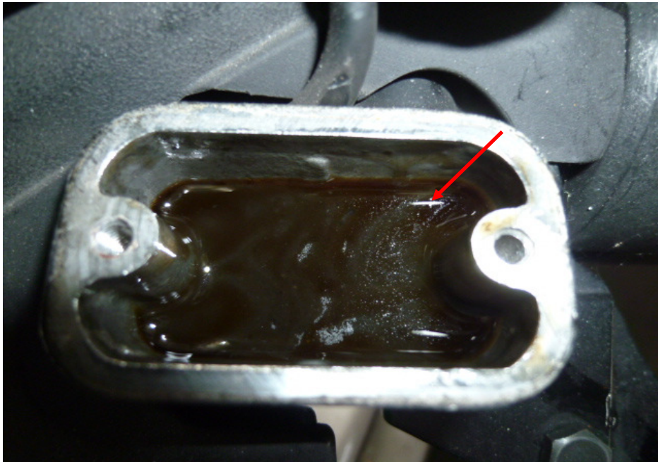
Photo 27 shows the brake fluid reservoir for the rear brake of the Motorcycle. The brake fluid was observed to be of sufficient level for operational purposes. However it was found to be contaminated (arrowed).
