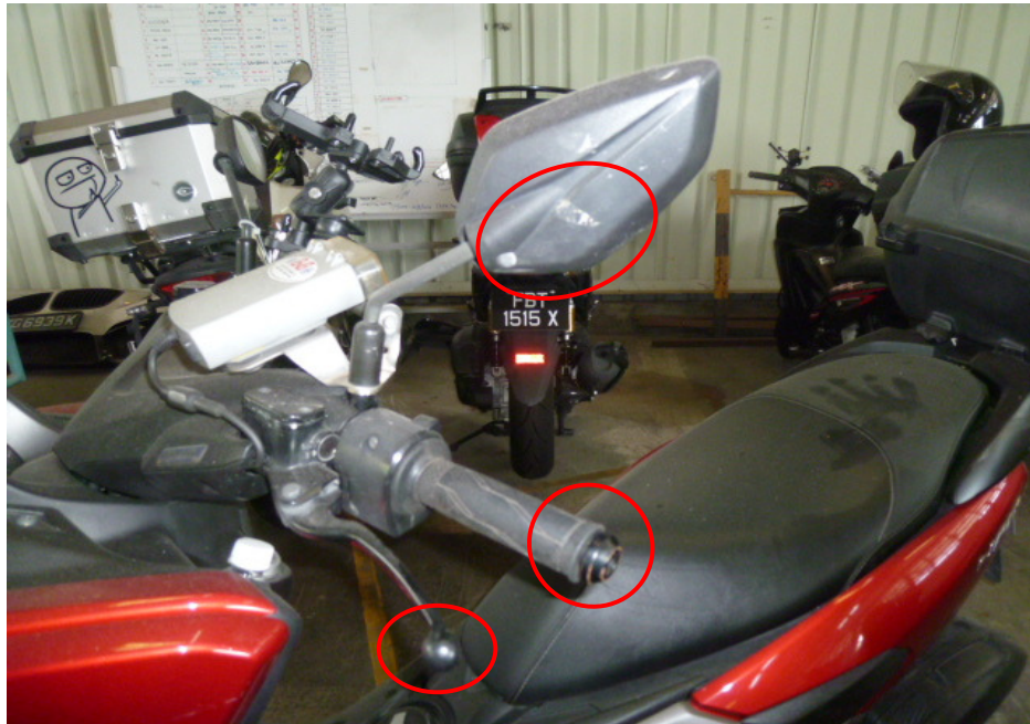
Photo 7 shows a closer view of the left side mirror, left handlebar end and rear brake lever of the Motorcycle which were observed to be damaged due to the accident (circled).
