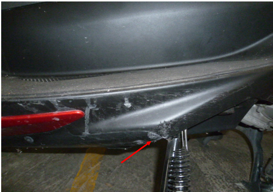
Photo 10 shows a closer view of the grazed left bottom cowling of the Motorcycle as a result of the accident (arrowed).
