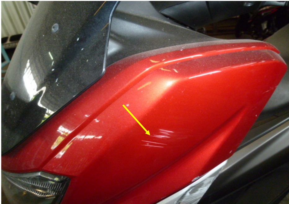
Photo 5 shows a closer view of the grazed front cowling of the Motorcycle at the time of our inspection (arrowed).
