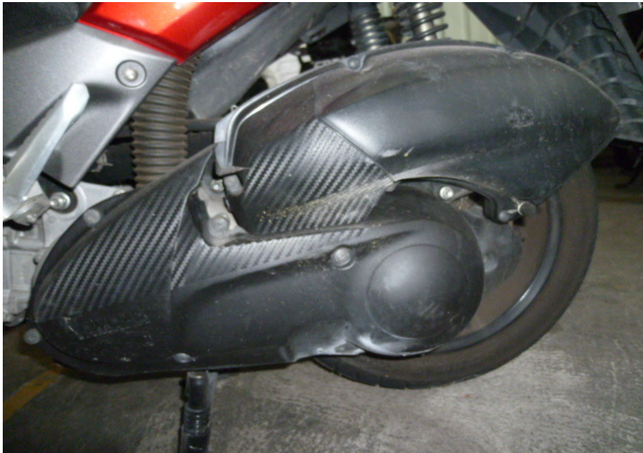
Photo 18 shows the drive train cover of the Motorcycle which was found to be intact without any misalignment. Upon examination of the Motorcycle's engine area, we had observed that the various engine related parts and components were intact with no visible damage. There was also no sign(s) or indication(s) of fluid leak observed around the engine area of the Motorcycle.
