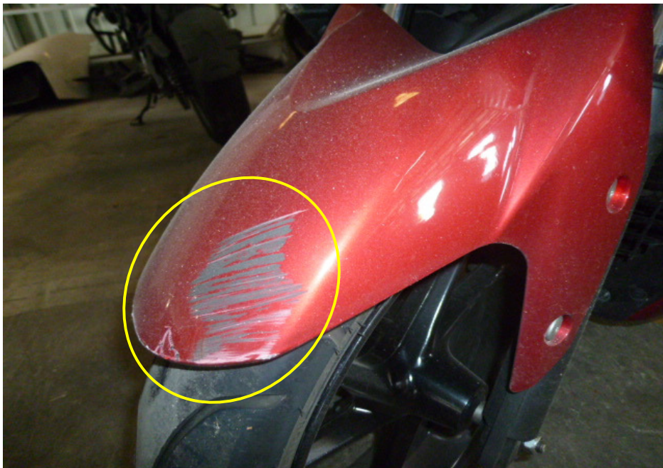
Photo 6 shows a closer view of the front mudguard which was amongst the body parts at the front body of the Motorcycle that had sustained damage as a result of the accident (circled).
