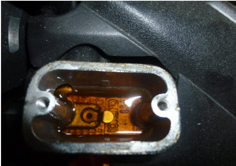
Photo 25 shows the brake fluid reservoir for the front brake of the Motorcycle. The brake fluid was observed to be of sufficient level for operational purposes and without any contamination.
