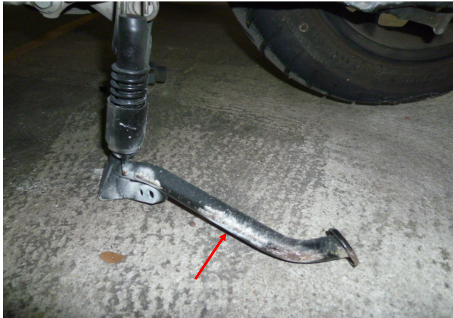
Photo 11 shows a closer view of the grazed main stand (arrowed) of the Motorcycle as a result of the accident.
