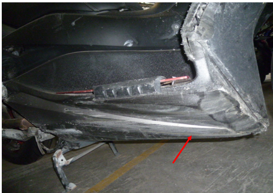
Photo 12 shows a close-up view of the grazed right lower side cowling of the Motorcycle as a result of the accident.
