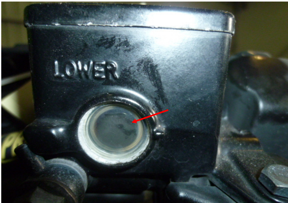
Photo 29 shows the brake fluid reservoir for the rear brake of the Motorcycle. The brake fluid was observed to be of sufficient level for operational purposes and without contamination (arrowed).
