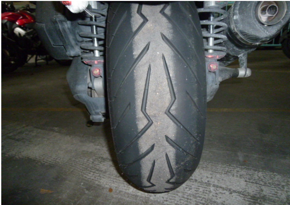
Photo 17 shows the condition of the Motorcycle's rear tyre. The rear tyre was observed to be in serviceable condition with remaining tread depth of approximately 8mm. The tyre was also observed to be sufficiently inflated for vehicular operation. We did not observe any tear, burst mark(s) and/or punctured hole(s) on the sidewalls as well as across the tread of the rear tyre.
