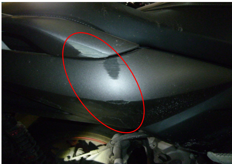
Photo 14 shows a closer view of the grazed right rear side cover (circled) of the Motorcycle as a result of the accident.
