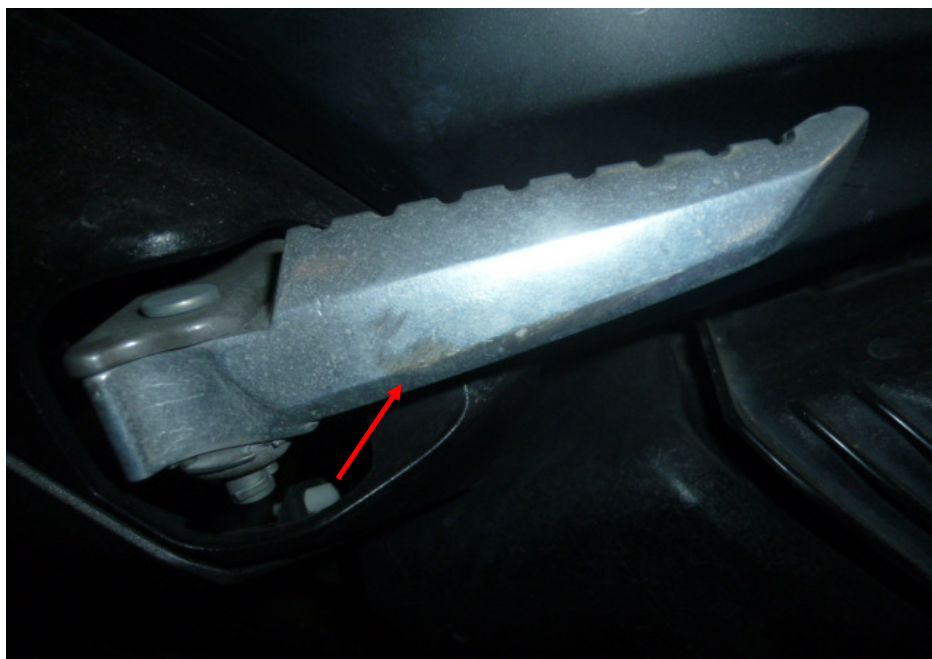
Photo 8 shows a closer view of the grazed left pillion footpeg (arrowed) of the Motorcycle as a result of the accident.
