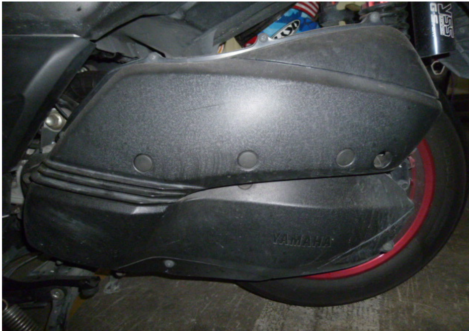
Photo 20 shows the drive train cover of the Motorcycle which was found to be intact without any misalignment.
