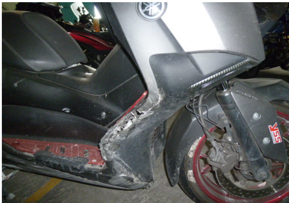
Photo 11 shows the damaged right side cowling of the Motorcycle as a result of the accident.
