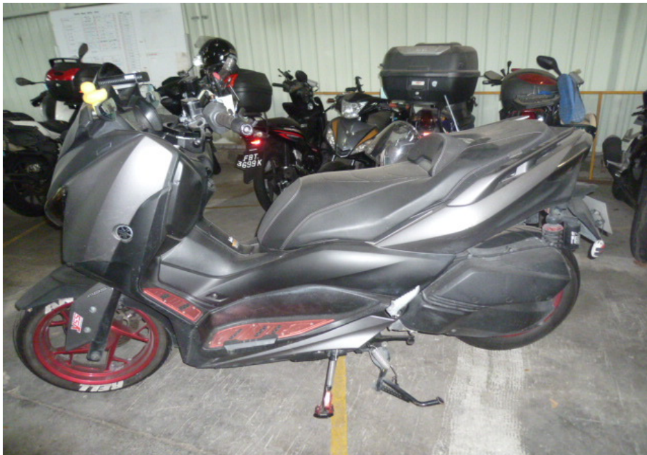
Photo 4 shows a general view of the left body of the Motorcycle at the time of our inspection. The Motorcycle was observed to have sustained damages all around. The body parts that were found to have been damaged include its front brake lever, right handlebar end, side cowlings, side lower cowlings, pillion footpegs, side stand, rear side covers and exhaust muffler, amongst others as a result of the accident.
