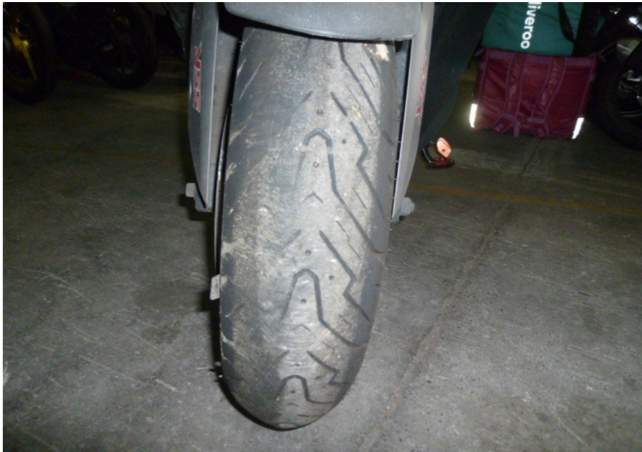
Photo 16 shows the condition of the Motorcycle's front tyre. The front tyre was observed to be in serviceable condition with remaining tread depth of approximately 2mm. There was no tear, burst mark(s) and/or punctured hole(s) on the sidewalls as well as across the tread of the front tyre.
