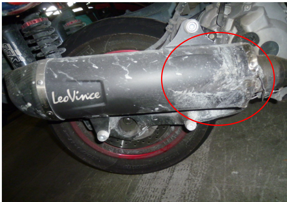
Photo 15 shows a closer view of the deformed exhaust muffler of the Motorcycle as a result of the accident (circled).
