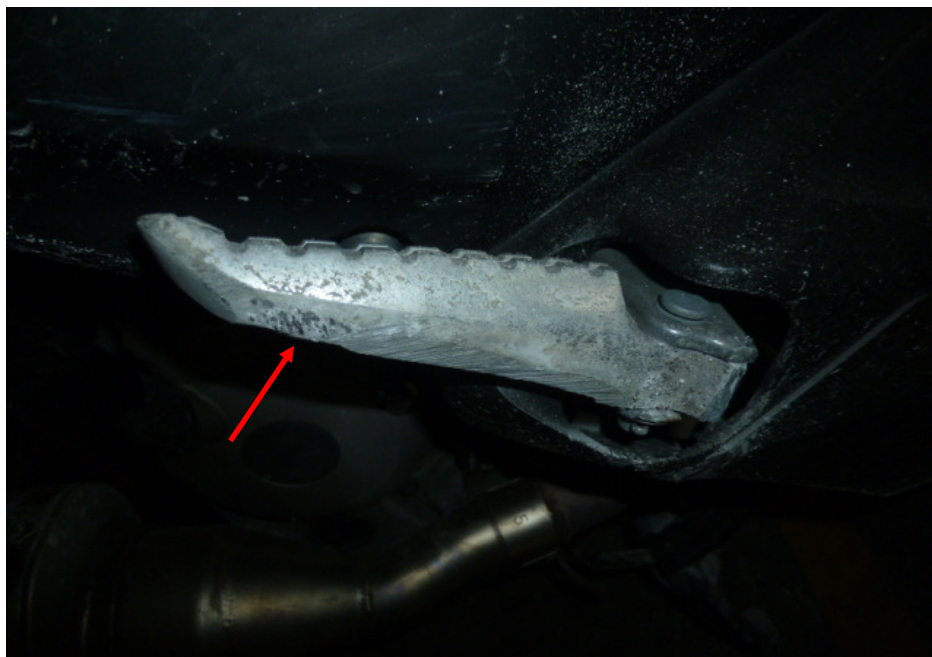
Photo 13 shows a closer view of the grazed right pillion footpeg (arrowed) of the Motorcycle as a result of the accident.
