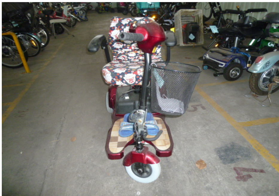
Photo 16 shows the front wheel of the PMA turned towards its full left. Turning the PMA's steering handlebar towards the left did not produce any abnormal free play and/or resistance. This would indicate that the steering system of the PMA was in serviceable condition at the time of our inspection.
