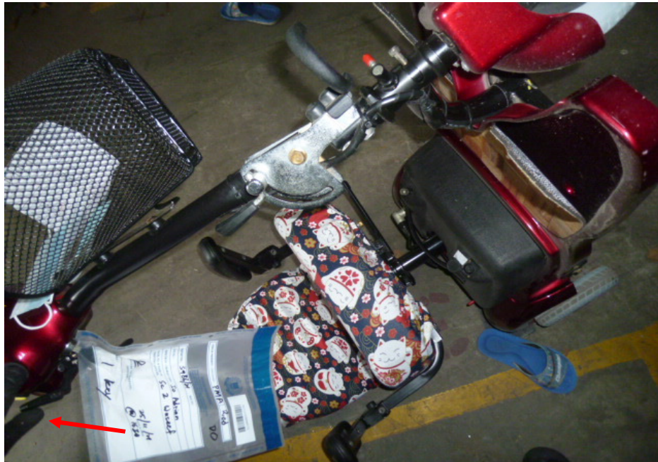
Photo 19 shows a static brake test conducted on the PMA's forward braking system. The test was conducted by lifting the rear wheels above ground. The PMA was switched on and the forward control lever (right hand lever) was pushed to rotate the rear wheels in a forward motion. The forward control lever was then released in order to stop the spinning rear tyres. The result was satisfactory. It stopped after the forward control lever returned to the centre (neutral drive) position.
