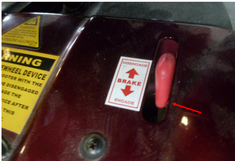
Photo 21 shows the red handled lever was able to be pulled downwards (arrowed) to engage the electric/mechanical disc park brake for the operational test.
