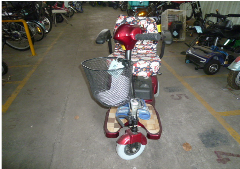
Photo 15 shows the front wheel of the PMA turned towards its full right. Turning the PMA's steering handlebar towards the right did not produce any abnormal free play and/or resistance. This would indicate that the steering system of the PMA was in serviceable condition at the time of our inspection.
