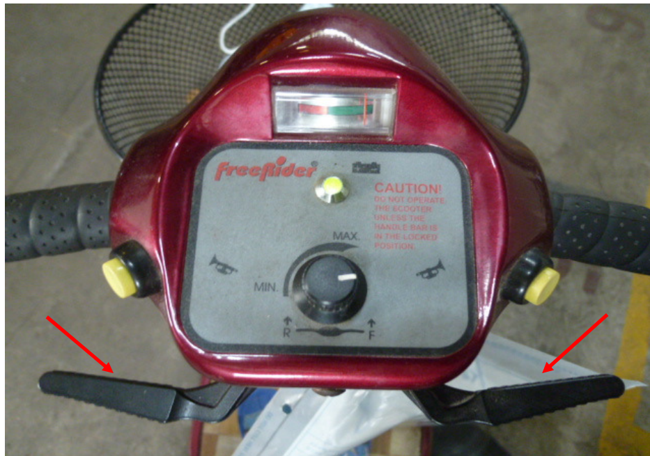
Photo 17 shows a close up view of the forward control lever and reverse control lever of the PMA (arrowed), which are all part of the components in the regenerative braking system of the PMA. Our visual checks of these various components had revealed all to be intact with no visible damage.
