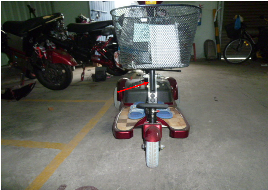
Photo 14 shows the steering handlebar (arrowed) of the PMA. The steering handlebar of the PMA was found to be intact and undamaged. Turning the PMA's steering handlebar towards the left and right did not produce any abnormal free play. The steering system of the PMA was in serviceable condition at the time of our inspection.
