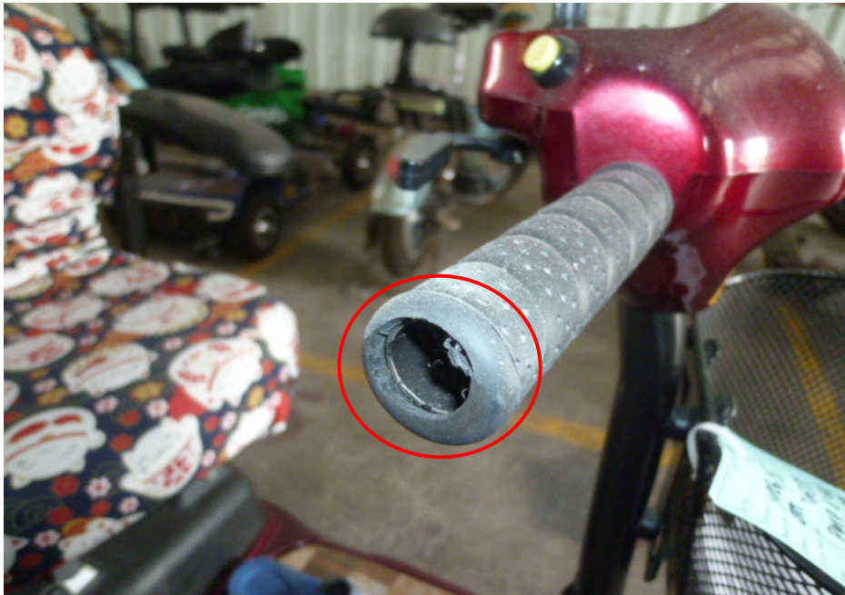
Photo 7 shows a closer view of the right handlebar grip (circled) of the PMA which were observed to be damaged due to the accident
