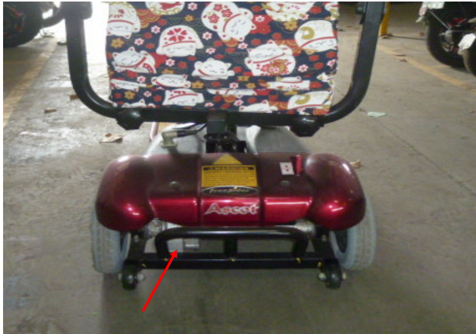
Photo 12 shows the general view of the electric drive motor (arrowed) of the PMA which was observed to be intact with no misalignment or damages. It was also observed to be in operational condition.
