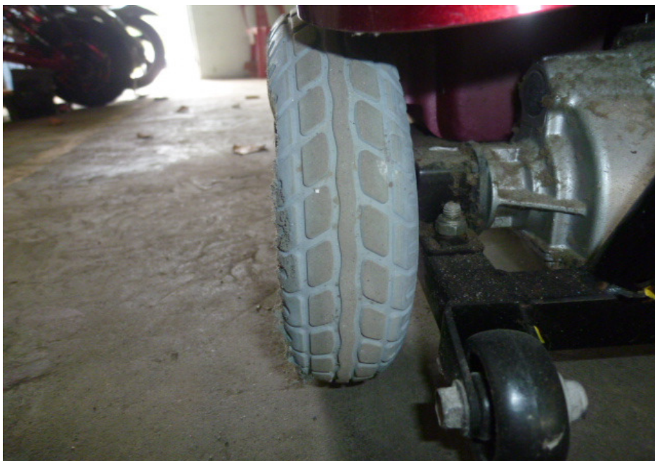
Photo 10 shows the condition of the PMA's left rear tyre. The left rear tyre was observed to have remaining tread depth of approximately 3mm. The left rear tyre was also observed to be sufficiently inflated for vehicular operation. However we found the left sidewall of the left rear tyre to be grazed.
