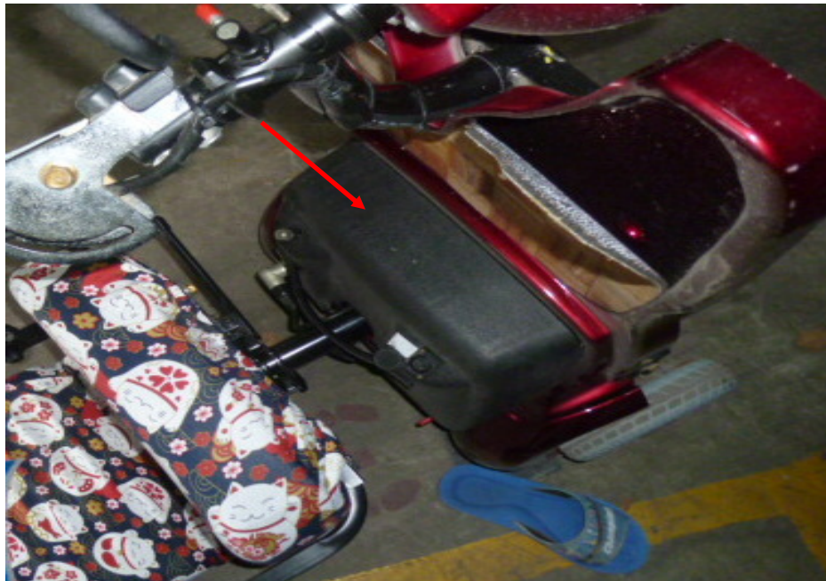
Photo 13 shows the wireless battery pack of the PMA (arrowed) which was found to be intact without any misalignment.
