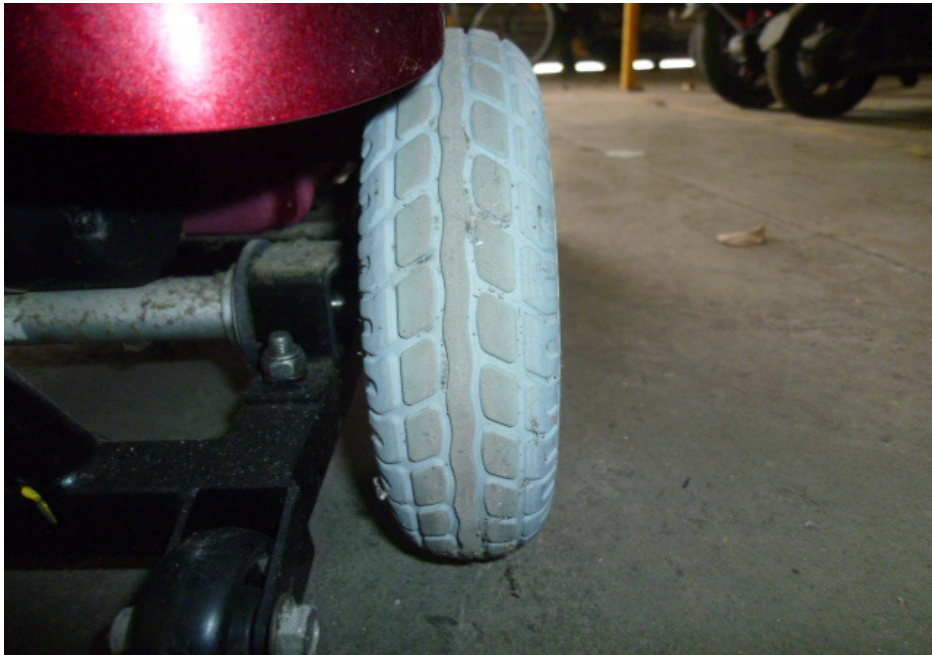
Photo 9 shows the condition of the PMA's right rear tyre. The right rear tyre was observed to be in serviceable condition with remaining tread depth of approximately 3mm. There was no tear, burst mark(s) and/or punctured hole(s) on the sidewalls as well as across the tread of the right rear tyre.
