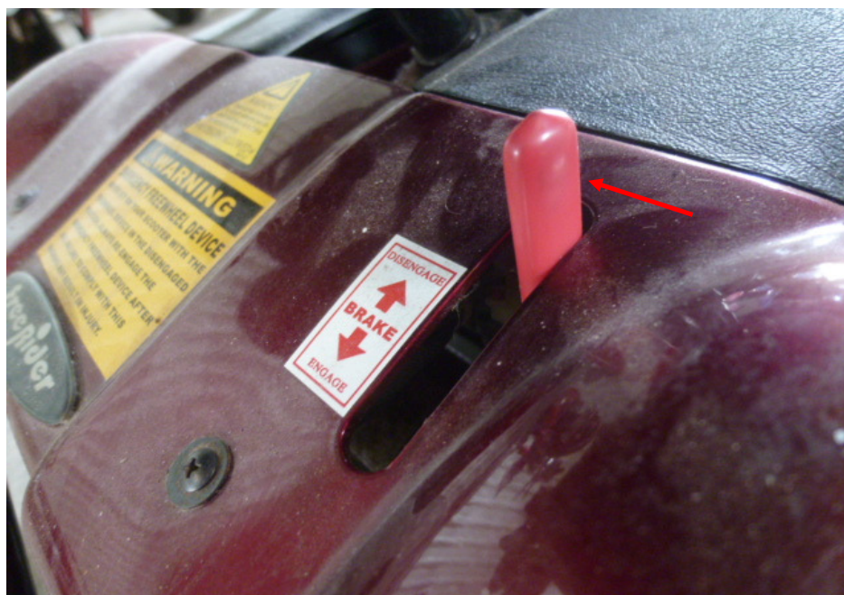
Photo 18 shows a close up view of the electric/mechanical disc park brake lever (arrowed) of the PMA. Our visual check of this component had revealed it to be intact with no visible damage.
