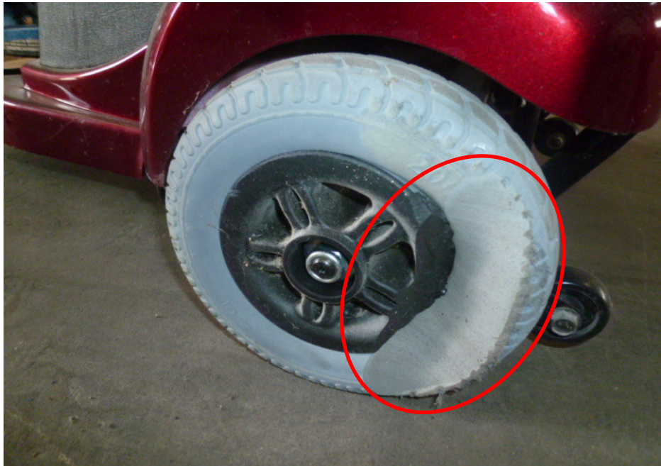
Photo 11 shows the left rear wheel rim and tyre of the PMA at the time of our inspection. Marks of grazing nature were observed on the left rear wheel rim and left sidewall of the left rear tyre of the PMA (circled).
