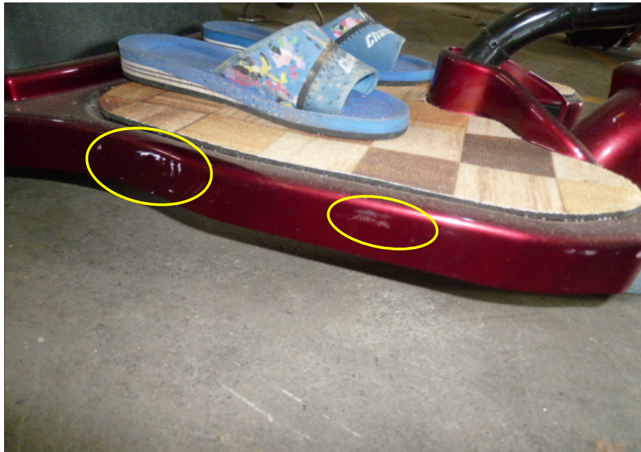
Photo 5 shows a closer view of the right bottom cowling (circled) of the PMA which was observed to be damaged due to the accident.
