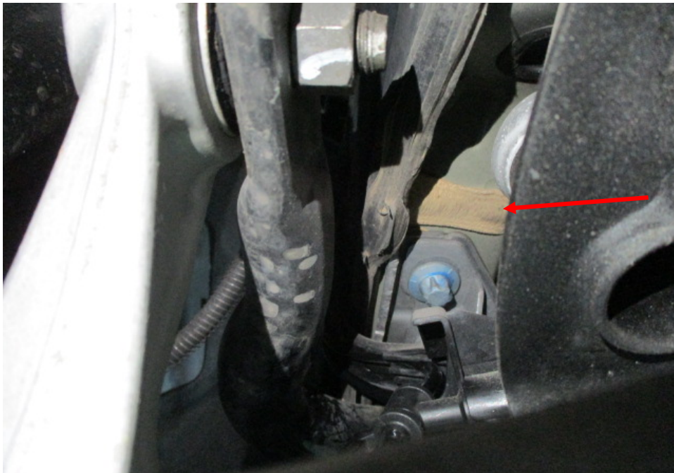
Photo 28 shows the chassis/structural body at the underside front left of the Motor Car. The original factory sealant (arrowed) at the joints along the chassis/structural body was observed to be untouched. In general, I had found no work was carried out on the chassis/structural body of the Motor Car. The chassis/structural body of the Motor Car was originally fitted.
