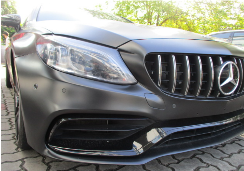
Photo 11 shows a closer view of the Motor Car's front bumper, front bumper right lower grille, front right headlamp, front emblem and radiator grille at the time of my inspection. The body parts at the frontal portion of the Motor Car were visually examined and it was observed that the repair/restoration works carried out to the damaged area of the Motor Car (refer to photograph 4 above) were reasonably adequate and in order.
