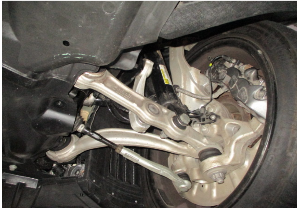
Photo 20 shows the various undercarriage components at the front right wheel of the Motor Car. The mechanical components, control arms and linkages were all found to be intact and secured in an appropriate manner. I also did not observe any fluid leak and/or fluid stain on the underside of the Motor Car.
