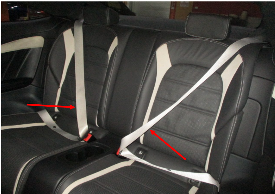
Photo 13 shows the seats of the Motor Car. All the seats of the Motor Car were secured via seat rails to the floorboard. They were also fitted with a retractable seat belt reel and a pre-tensioner. The seat belts (arrowed) were tested and were able to be fastened into the respective pre-tensions that were fitted on the side of each individual seat.
