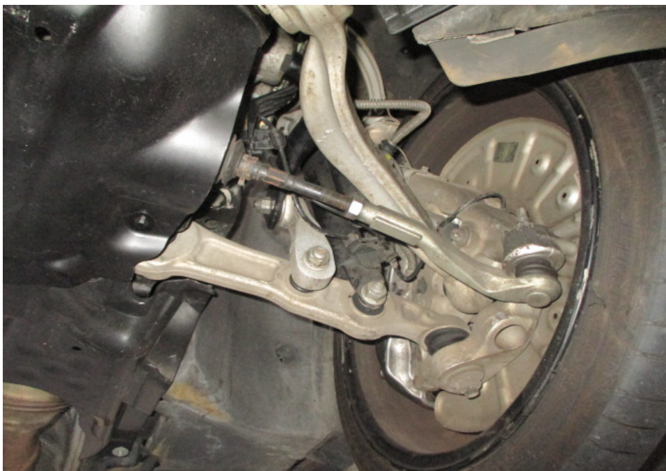
Photo 19 shows the various undercarriage components at the front left wheel of the Motor Car. The mechanical components, control arms and linkages were all found to be intact and secured in an appropriate manner.
