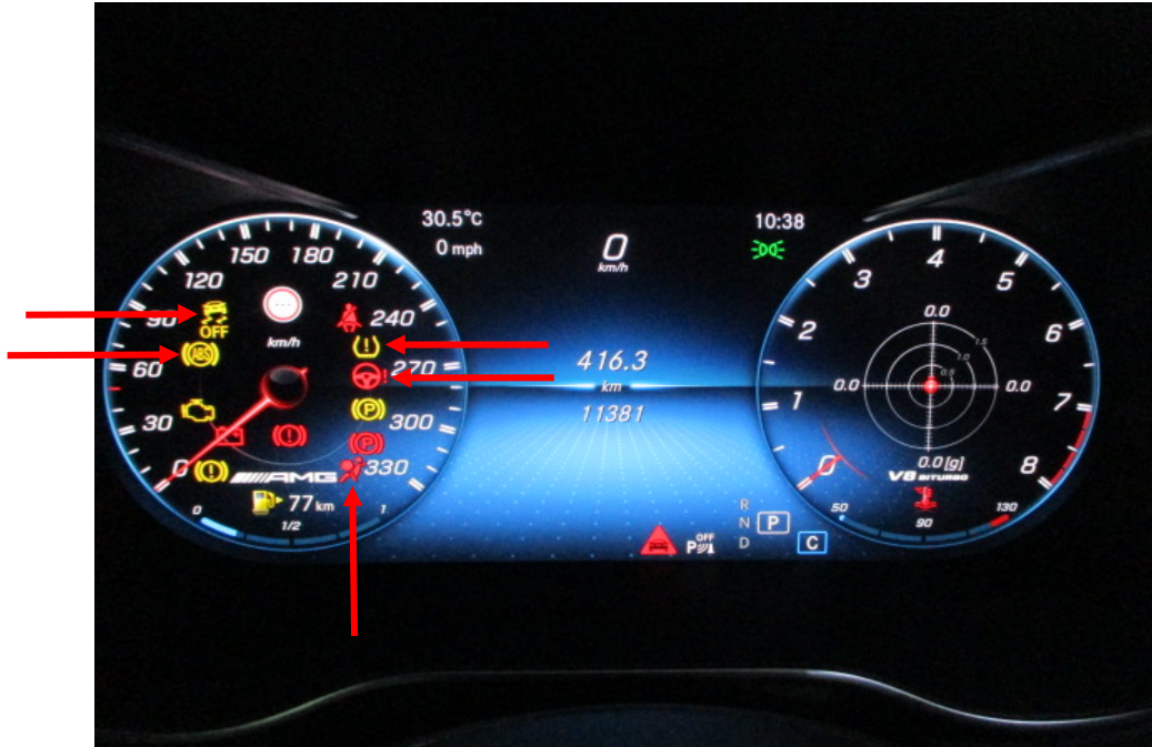
Photo 14 shows the warning lights for the various electronic safety features appearing on the instrument panel of the Motor Car during its self-test when the engine is cranked, in particular the ABS, SRS, EPS, TPM and TCS lights (arrowed).
