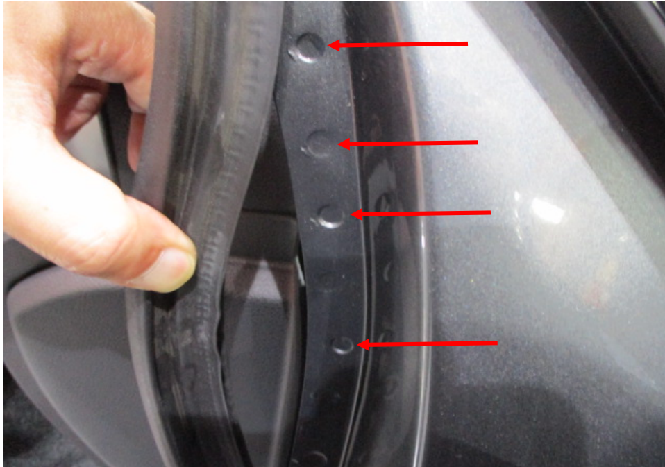
Photo 30 shows the right side "A" pillar of the Motor Car. I did not find any weld marks other than original spot weld marks (arrowed) on the right side "A" pillar of the Motor Car which, indicates that there was no re-welding works carried out. In general, I had found all the non-detachable body panels of the Motor Car to be originally fitted at the time of my inspection.
