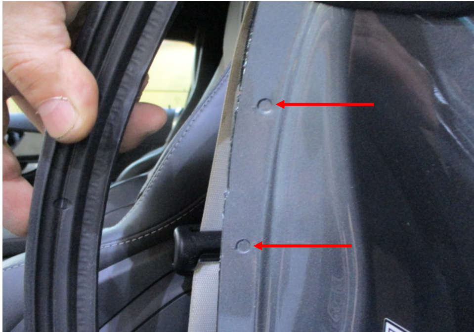
Photo 28 shows the rear left body panel of the Motor Car. I did not find any weld marks other than original spot weld marks (arrowed) on the rear left body panel of the Motor Car, which indicates that there was no re-welding works carried out. In general, I had found all the non-detachable body panels of the Motor Car to be originally fitted at the time of my inspection.
