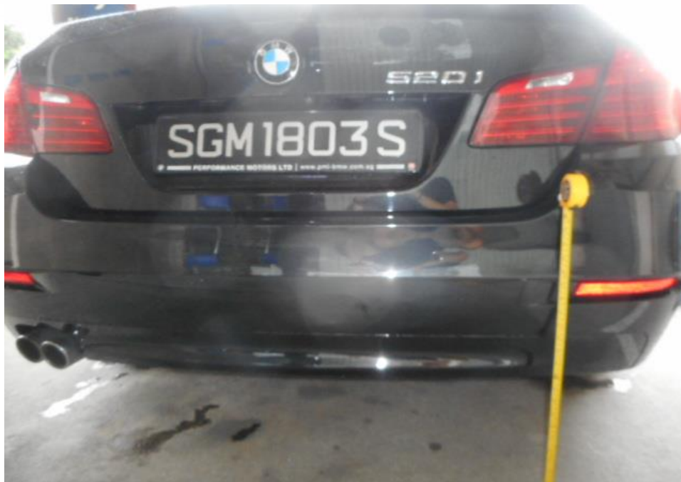
Photo 9 shows the general view of the height measurement being conducted on the rear portion of Car. The height above ground level of where the dent at the rear bumper portion, was at 46cm to 49cm respectively.
