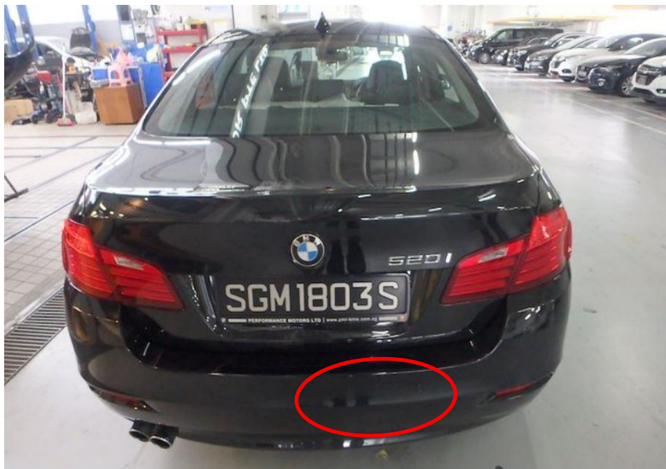
Photo 1 shows the general view of the rear portion of Car at the time of inspection. The rear bumper had been damaged. It was also noted that there were paint crack marks and dent (circled) on the rear bumper of the Car.
