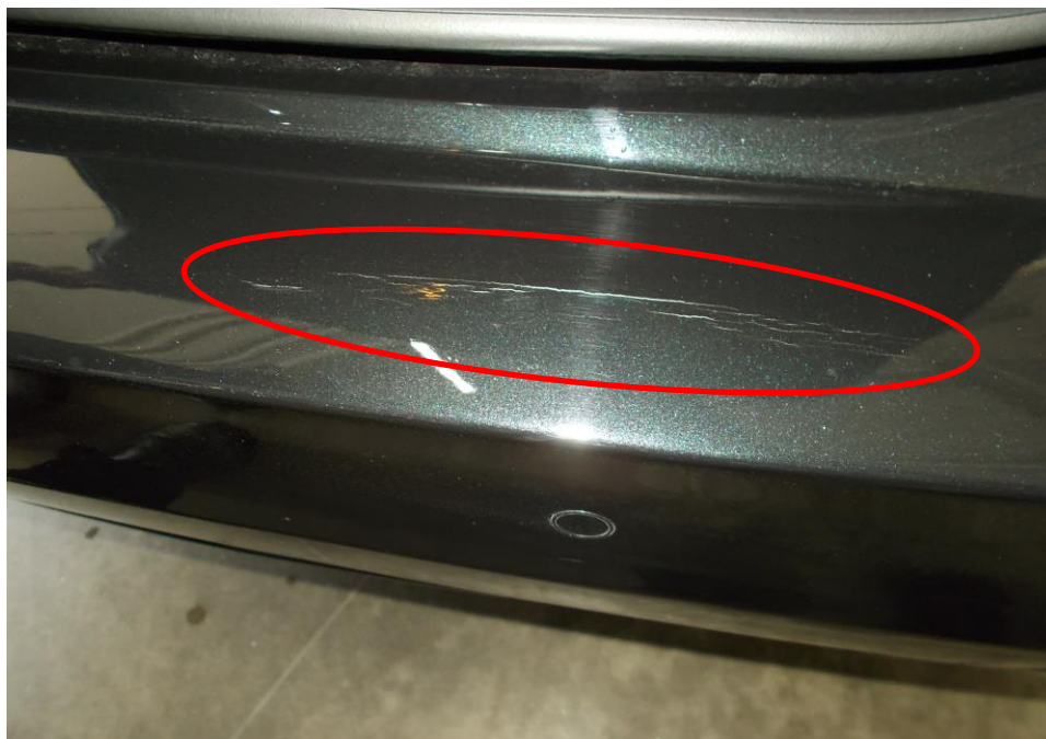
Photo 3 shows the close up view of the rear portion of Car at the time of inspection. The rear bumper had been damaged. It was also noted that there were paint crack marks (circled) on the rear bumper of the Car.
