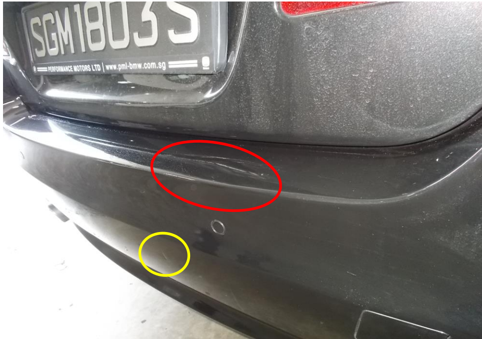
Photo 2 shows the close up view of the rear portion of Car at the time of inspection. The rear bumper had been damaged. It was also noted that there were paint crack marks (red circle) and dent (yellow circle) on the rear bumper of the Car.
