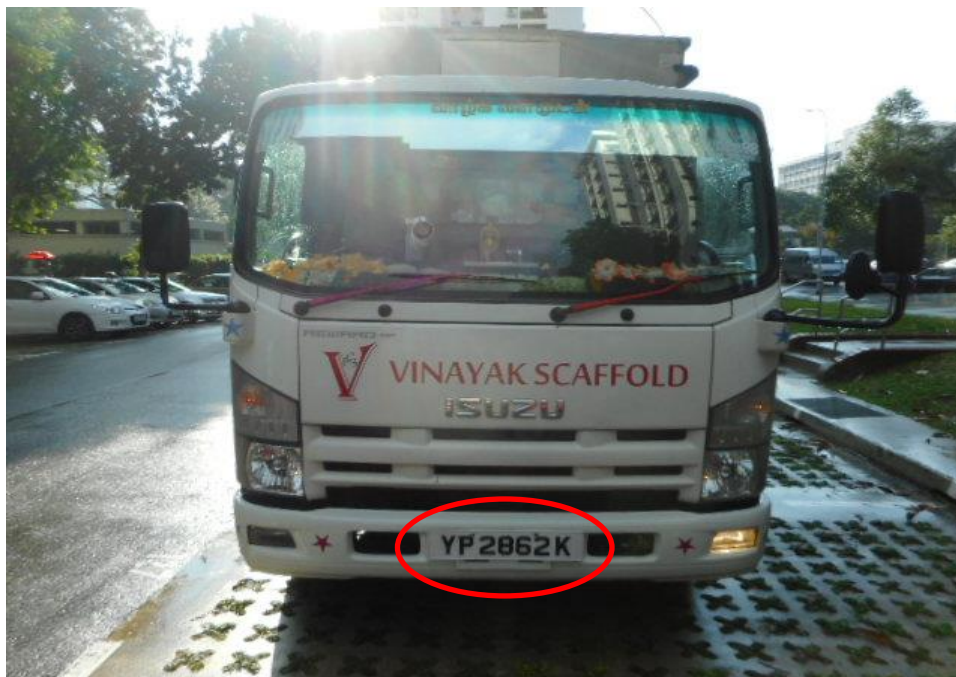
Photo 5 shows the general view of the front portion of Lorry at the time of inspection. The front number plate (circled) had paint transfer and scratch marks.
