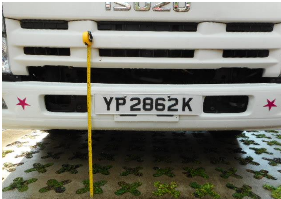
Photo 8 shows a general view of the height measurement being conducted on the front portion of Lorry. The front number plate where the paint transfer and scratched marks is was measured to be at 54cm to 55cm above ground level.
