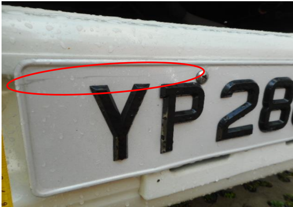
Photo 6 shows the close up view of the front portion of Lorry at the time of inspection. The front number plate (circled) had paint transfer and scratch marks.
