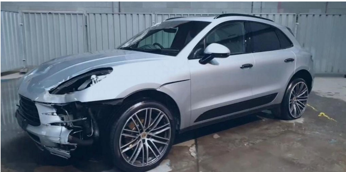
Photo 4 shows another view of the Motor Car's front left body (photograph provided to me). The Motor Car was observed to have sustained damage at its frontal portion. The front bumper, front bumper left lower grille, front bumper left upper grille, front bonnet, front left day light, front left headlamp and front left fender inner shield were amongst the body parts that were observed to have been damaged.
