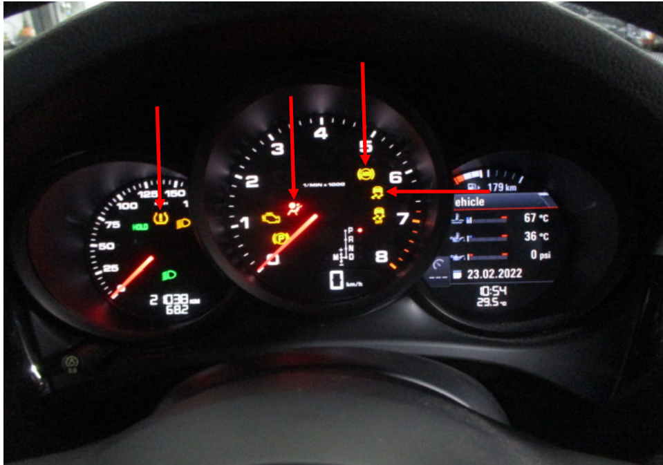
Photo 18 shows the warning lights for the various electronic safety features appearing on the instrument panel of the Motor Car during its self-test when the engine is cranked, in particular the ABS, SRS, TPM and TCS lights (arrowed).
