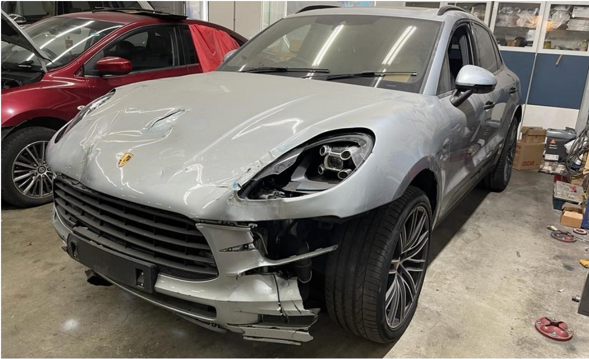
Photo 1 shows the front left body of the Motor Car (photograph provided to me). The Motor Car was observed to have sustained damage at its frontal portion. The front bumper, front bumper left lower grille, front bumper left upper grille, front bumper lower lip, front left day light, front left headlamp and front left fender inner shield were amongst the body parts that were observed to have been damaged.
