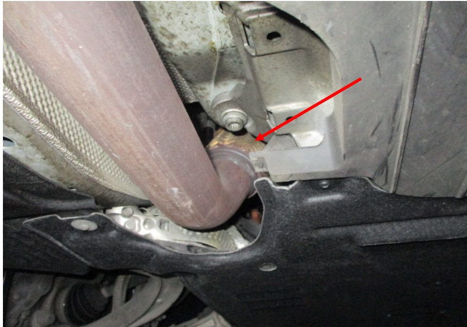
Photo 26 shows the front section of the Motor Car's exhaust system. My examination of the Motor Car's exhaust system revealed no sign(s) or indication(s) of any cut or weld marks along its exhaust pipes, on its rear mufflers and on its catalytic converter (arrowed).
