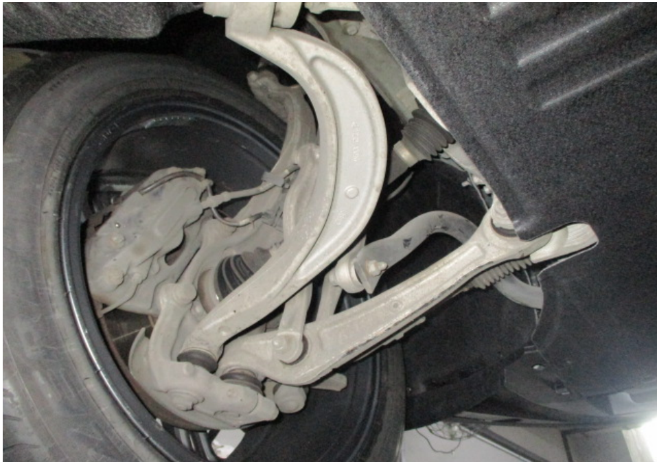
Photo 23 shows a general view of the control arms and linkages at the front left wheel of the Motor Car. I did not observe any fluid leak and/or fluid stain on the underside of the Motor Car. All of the Motor Car's undercarriage components were observed to be intact and secured in an appropriate manner.
