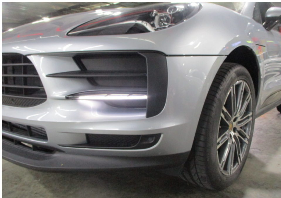
Photo 9 shows a closer view of the Motor Car's front bumper, front bumper left lower grille, front bumper left upper grille, front bumper lower lip and front left day light. The body parts at the frontal portion of the Motor Car were visually examined and it was observed that the repair/restoration works carried out to the damaged area of the Motor Car (refer to photograph 1 - 4 above) were reasonably adequate and in order.
