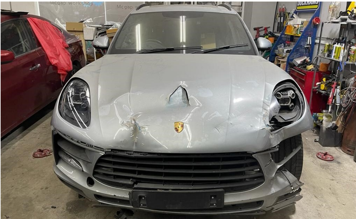
Photo 2 shows the frontal body of the Motor Car (photograph provided to me). The Motor Car was observed to have sustained damage at its frontal portion. The front bumper, front bumper left lower grille, front bumper left upper grille, front bumper number plate garnish, radiator grille and front bonnet were amongst the body parts that were observed to have been damaged.
