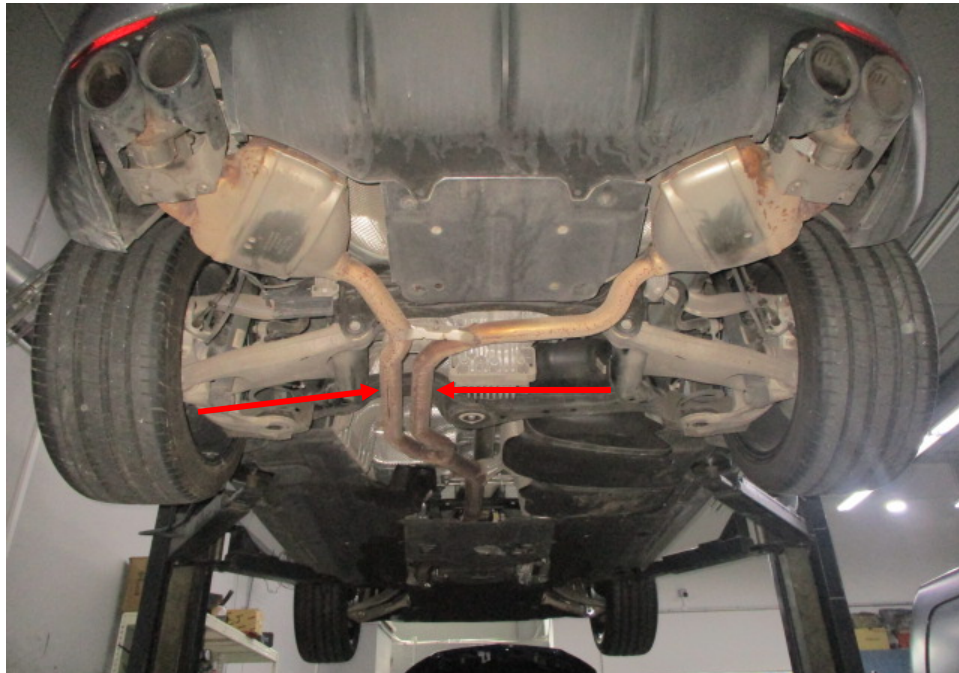
Photo 25 shows the rear section of the Motor Car's exhaust system. My examination of the Motor Car's exhaust system revealed no sign(s) or indication(s) of any cut or weld marks along its exhaust pipes (arrowed), on its rear mufflers and on its catalytic converter.
