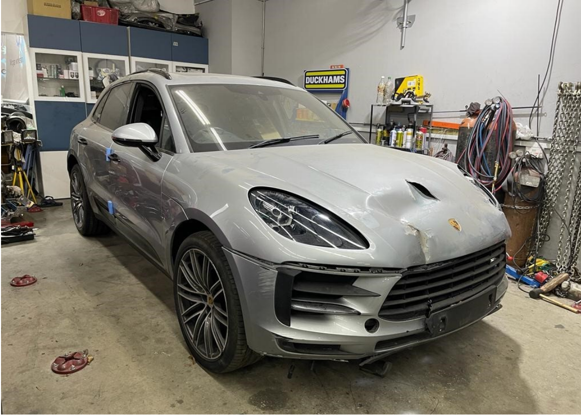
Photo 3 shows the front right body of the Motor Car (photograph provided to me). The Motor Car was observed to have sustained damage at its frontal portion. The front bumper, radiator grille and front bonnet were amongst the body parts that were observed to have been damaged. The airbag(s) of the Motor Car was not deployed as seen from the photographs that were provided.
