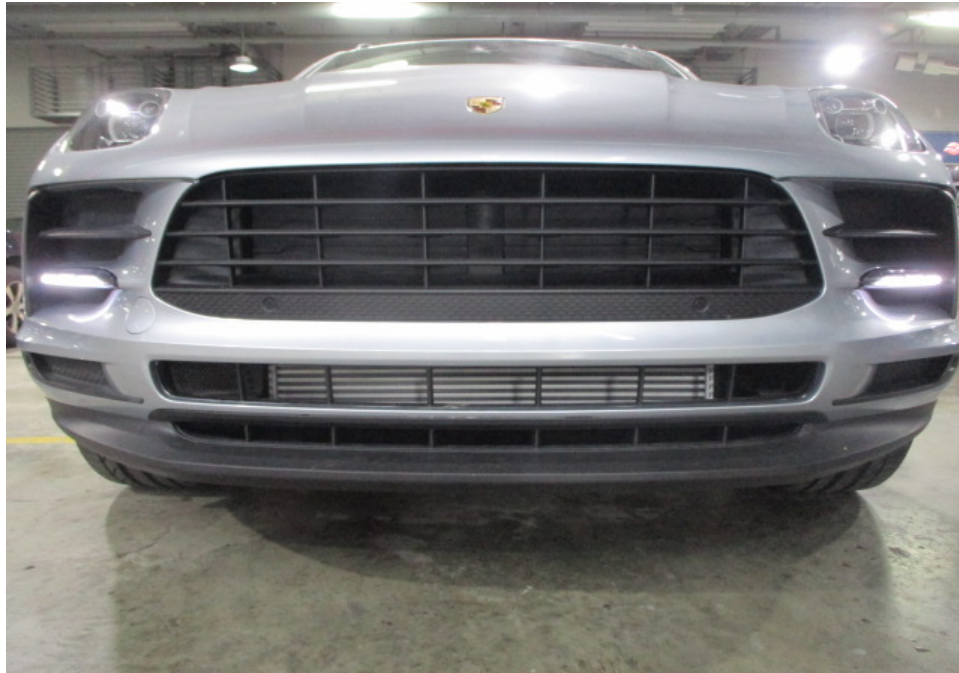
Photo 10 shows a closer view of the Motor Car's front bumper, front bumper centre lower grille, radiator grille and day running lights. The body parts at the frontal portion of the Motor Car were visually examined and it was observed that the repair/restoration works carried out to the damaged area of the Motor Car (refer to photograph 1 - 4 above) were reasonably adequate and in order.
