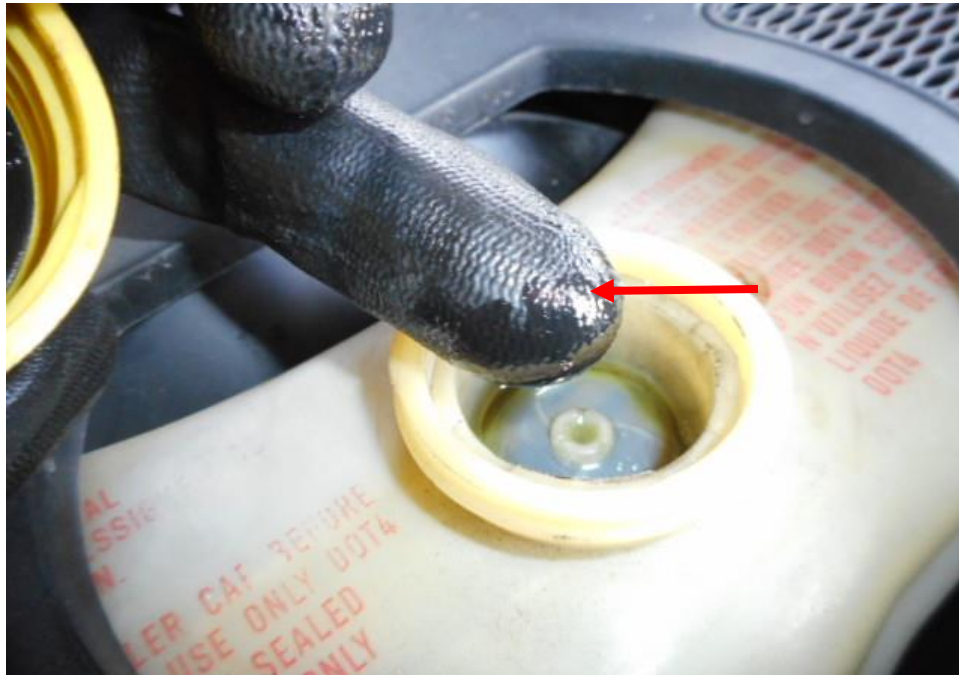
Photo 22 shows the brake fluid reservoir of the Motor Car at the time of my inspection. The brake fluid was observed to be of sufficient level (arrowed) and without any visible contamination.
