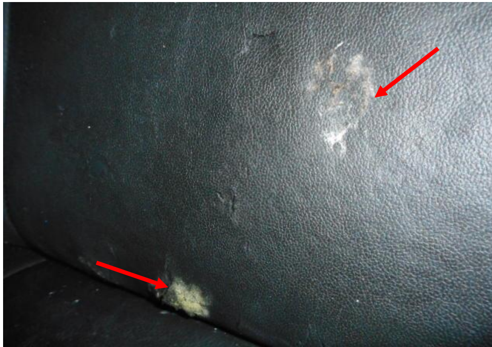
Photo 13 shows a close up view of the Motor Car's interior cabin portion at the time of my inspection. We have observed mouldy stains on the seats (arrowed) at the rear right portion due to water intrusion from the water seeping down from the holes of the cloth roof above.
