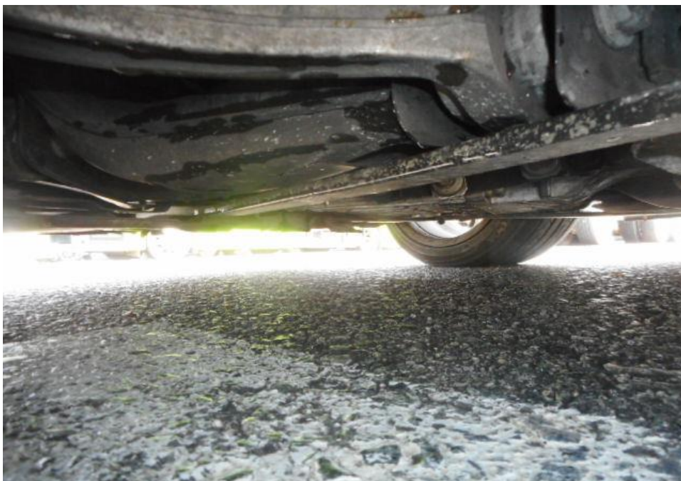
Photo 25 shows the undercarriage of the Motor Car, at the area where the engine housing and transmission housing are located. I did not find any sign(s) or indication(s) of fluid leak and/or fluid stain(s) on the underside of the Motor Car.
