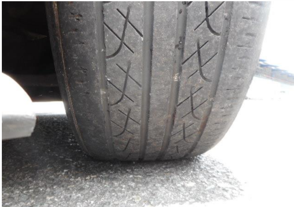
Photo 17 shows the condition of the front right tyre of the Motor Car, which was observed to be in serviceable condition with remaining tread depth of approximately 4mm. The tyre was sufficiently inflated for vehicular operation with no tear, cut or burst mark(s) on the outer and the inner sidewalls as well as across the tread. The 4 tyres of the Motor Car were wrapped around standard steel wheel rims without any damage.
