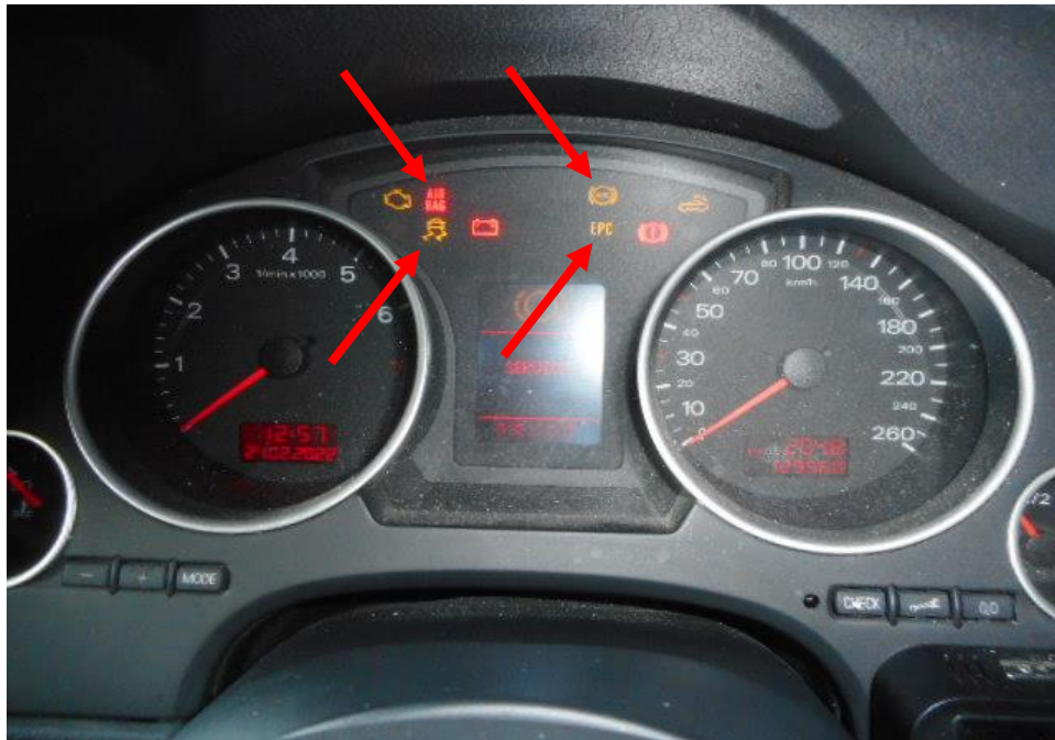
Photo 33 shows the warning light for Anti-Lock Brake System (ABS), Electric Power Steering System (EPS), Traction Control System (TCS) and Supplemental Restraint System (SRS) (arrowed) appearing on the instrument panel of the Motor Car during the self-test of its various electronic operating systems when its engine was cranked.
