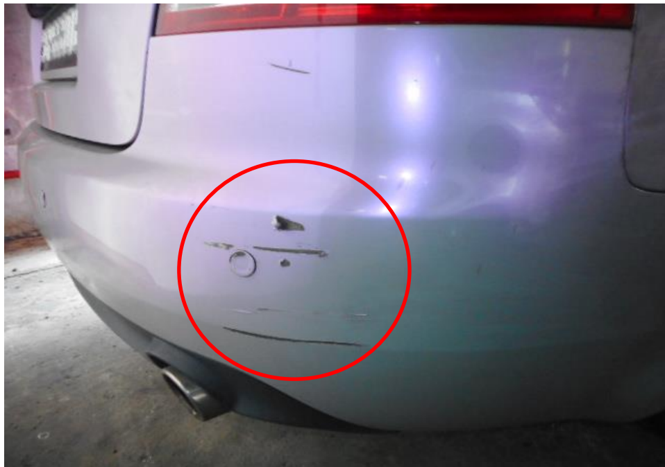
Photo 4 shows a close up view of the Motor Car's rear portion at the time of my inspection. The Motor Car was observed to have sustained damage at its rear bumper portion. Its rear bumper right portion (circled) were the body parts that were damaged as a result of the incident.
