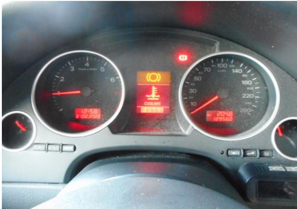
Photo 34 shows no warning lights illuminated on the instrument panel of the Motor Car after the engine was cranked. This would suggest that there was no abnormality to the electronic operating system of the Motor Car, like the ABS, EPS, TCS and SRS etc.
