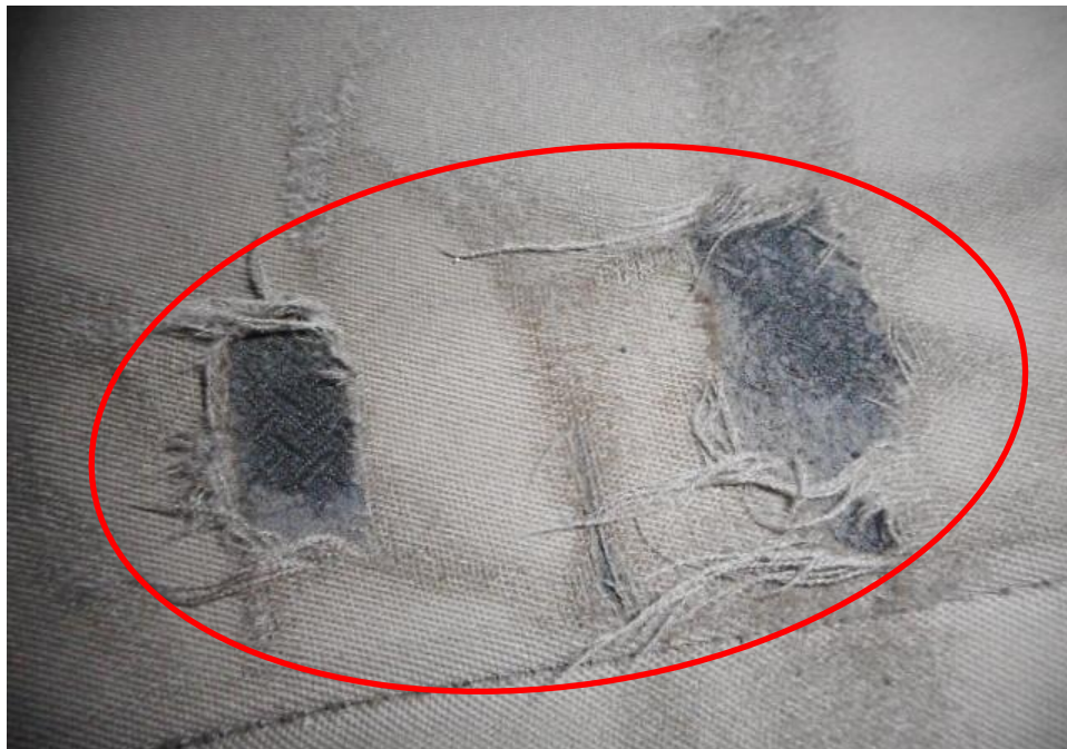
Photo 8 shows a close up view of the Motor Car's cloth roof portion at the time of my inspection. There was holes present prior to the incident at the rear right cloth roof portion (circled) of the Motor Car and water intrusion had likely started from these holes flowing down into the interior cabin of the Motor Car.
