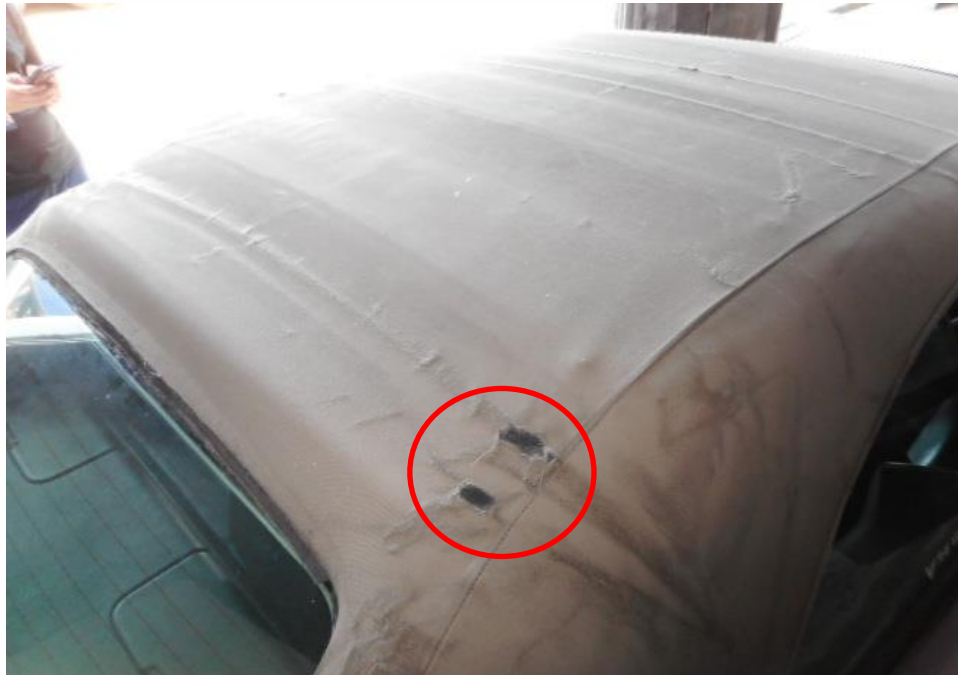
Photo 7 shows a general view of the Motor Car's cloth roof portion at the time of my inspection. There was holes present prior to the incident at the rear right cloth roof portion (circled) of the Motor Car and water intrusion had likely started from these holes flowing down into the interior cabin of the Motor Car.
