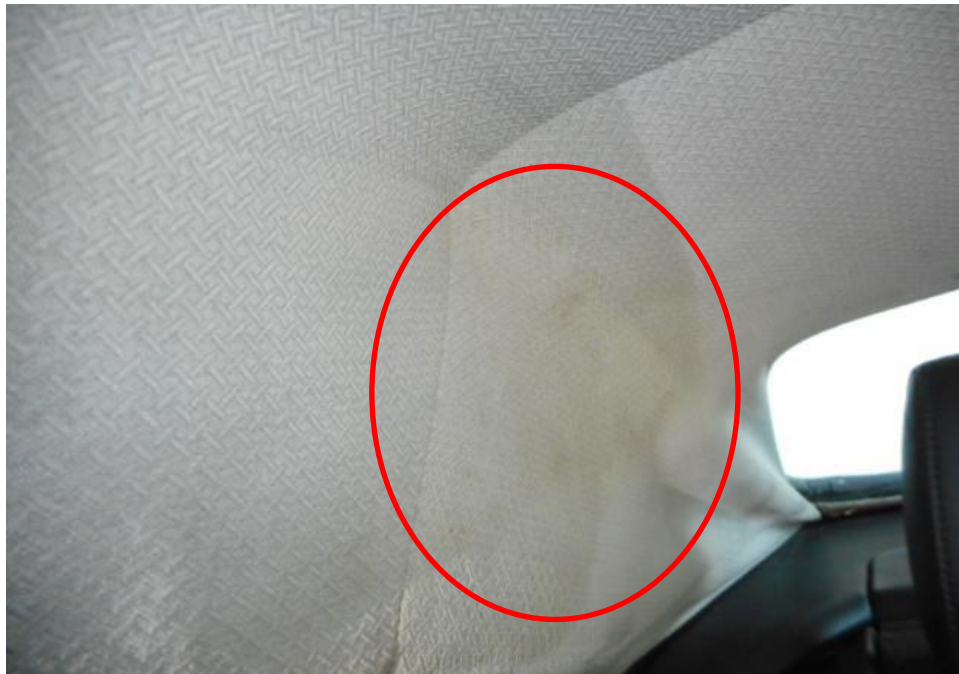
Photo 10 shows a close up view of the Motor Car's interior cabin portion at the time of my inspection. We have observed mouldy stains on its cloth roof (circled) at the rear right portion due to water intrusion from the water seeping down from the holes of the cloth roof above.
