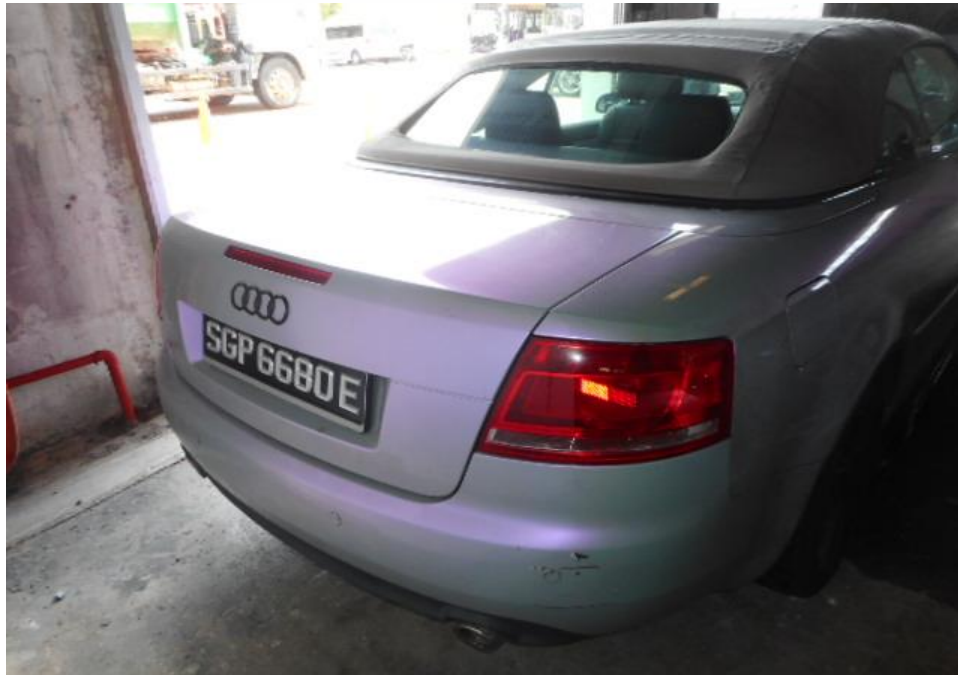
Photo 3 shows the general view of the Motor Car's rear body at the time of my inspection. The Motor Car was observed to have sustained damage at its rear bumper portion. Its rear bumper right portion were amongst were the body parts that were damaged as a result of the incident.
