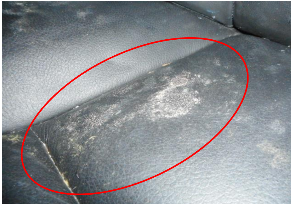
Photo 14 shows a close up view of the Motor Car's interior cabin portion at the time of my inspection. We have observed mouldy stains on the seats (circled) at the rear right portion due to water intrusion from the water seeping down from the holes of the cloth roof above.
