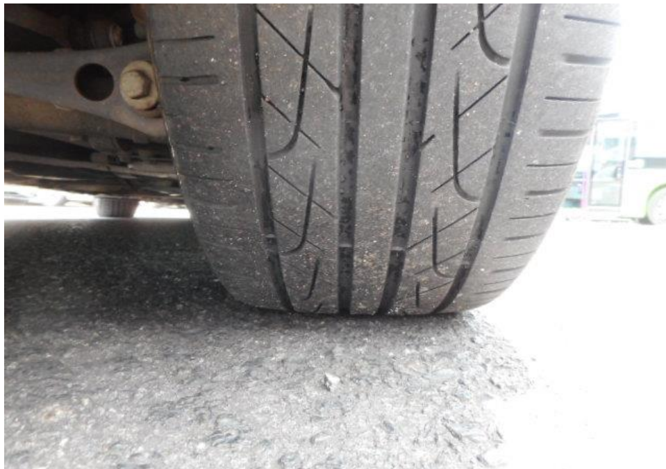
Photo 18 shows the condition of the rear right tyre of the Motor Car, which was observed to be in serviceable condition with remaining tread depth of approximately 4mm. The tyre was also observed to be sufficiently inflated for vehicular operation with no tear, cut or burst mark(s).
