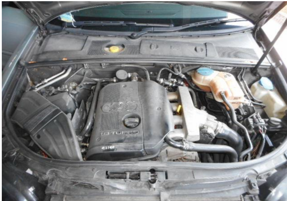
Photo 21 shows a general view of the Motor Car's engine compartment. The various parts and components inside the engine compartment were unaffected by the incident. There was also no sign(s) or indication(s) of fluid leakage and/or fluid stain within the engine compartment.
