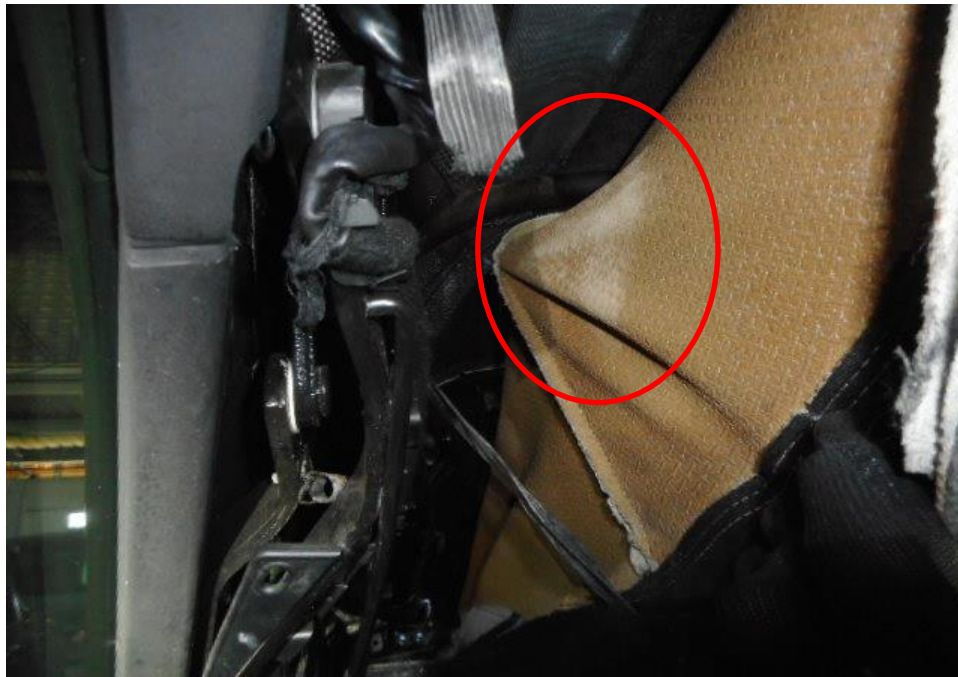
Photo 11 shows a close up view of the Motor Car's interior cabin portion at the time of my inspection. We have observed mouldy stains on inside of the cloth roof (circled) at the rear right portion due to water intrusion from the water seeping down from the holes of the cloth roof above.
