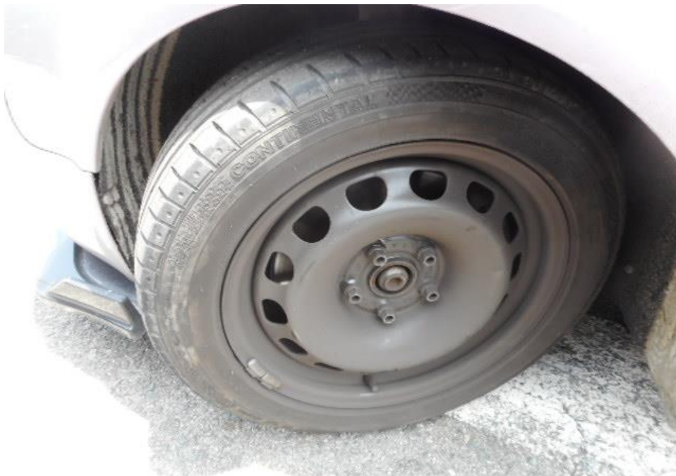
Photo 20 shows the condition of the front left tyre (steel rim spare tyre) of the Motor Car, which was observed to be in serviceable condition with remaining tread depth of approximately 5mm. There was also no tear, cut or burst mark(s) on the outer and the inner sidewalls as well as across the tread of the Motor Car's 4 tyres.
