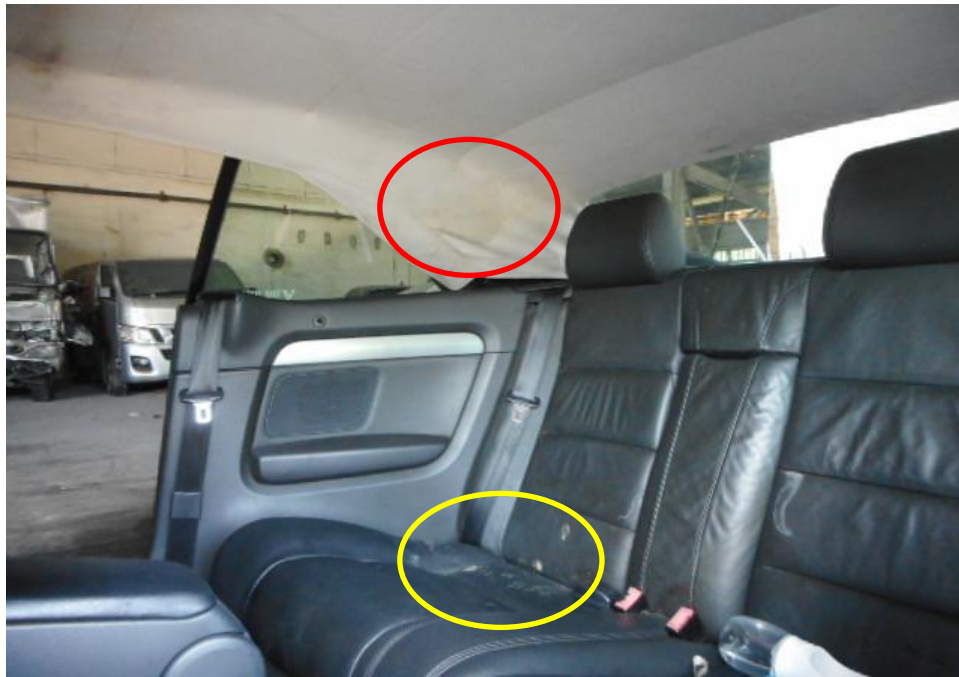
Photo 9 shows a general view of the Motor Car's interior cabin portion at the time of my inspection. Its cloth roof (red circle) and seats (yellow circle) at the rear right portion had suffered water intrusion damages due to water seeping down from the holes on the cloth roof above.
