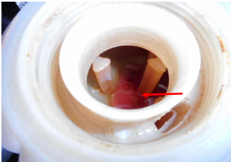
Photo 23 shows checks being carried out to the engine coolant of the Motor Car at the time of my inspection. The engine coolant was observed to be of low level (arrowed) and without any visible contamination.
