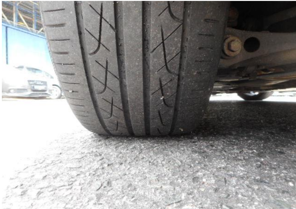
Photo 19 shows the condition of the rear left tyre of the Motor Car, which was observed to be in serviceable condition with remaining tread depth of approximately 4mm. The tyre, which was wrapped around steel wheel rim, was also observed to be sufficiently inflated for vehicular operation. The 4 tyres of the Motor Car were wrapped around standard steel wheel rims.
