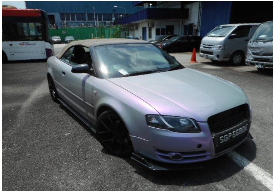
Photo 30 shows the front right wheel of the Motor Car turned to its full left. During my steering system test, I did not experience any abnormal free play and/or resistance when I had turned the steering wheel towards the left and right. This would suggest that the steering system of the Motor Car was likely to be in serviceable condition at the material time of incident.
