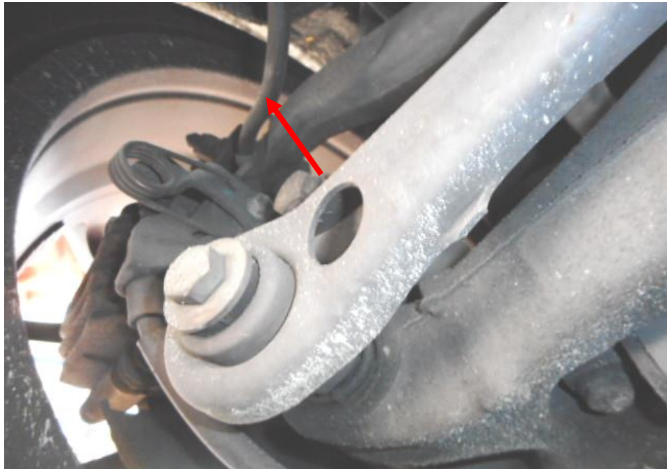
Photo 27 shows the brake hose/pipe (arrowed) at the rear left wheel of the Motor Car. I did not observe any leakage of brake fluid at the time of my inspection of the Motor Car. Static tests of the Motor Car's braking system had indicated that there was no internal leakage of pressure/vacuum. The undercarriage components of the Motor Car were also all found to be intact and without any visible damage.
