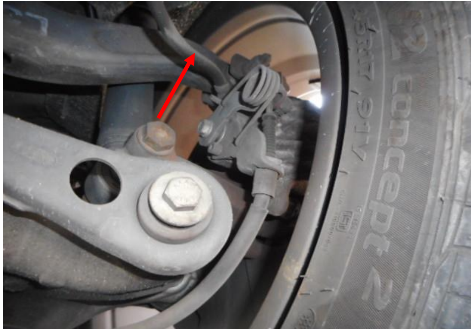
Photo 26 shows the brake hose/pipe (arrowed) at the rear right wheel of the Motor Car. No leakage of brake fluid was observed. Visual examination of the various components of the braking system like the drum brake, brake booster, brake pedal etc. had revealed all to be intact and without visible damage.
