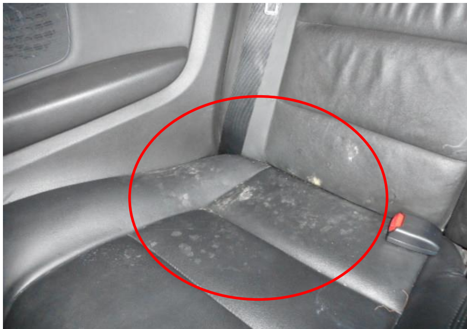
Photo 12 shows a close up view of the Motor Car's interior cabin portion at the time of my inspection. We have observed mouldy stains on the seats (circled) at the rear right portion due to water intrusion from the water seeping down from the holes of the cloth roof above.
