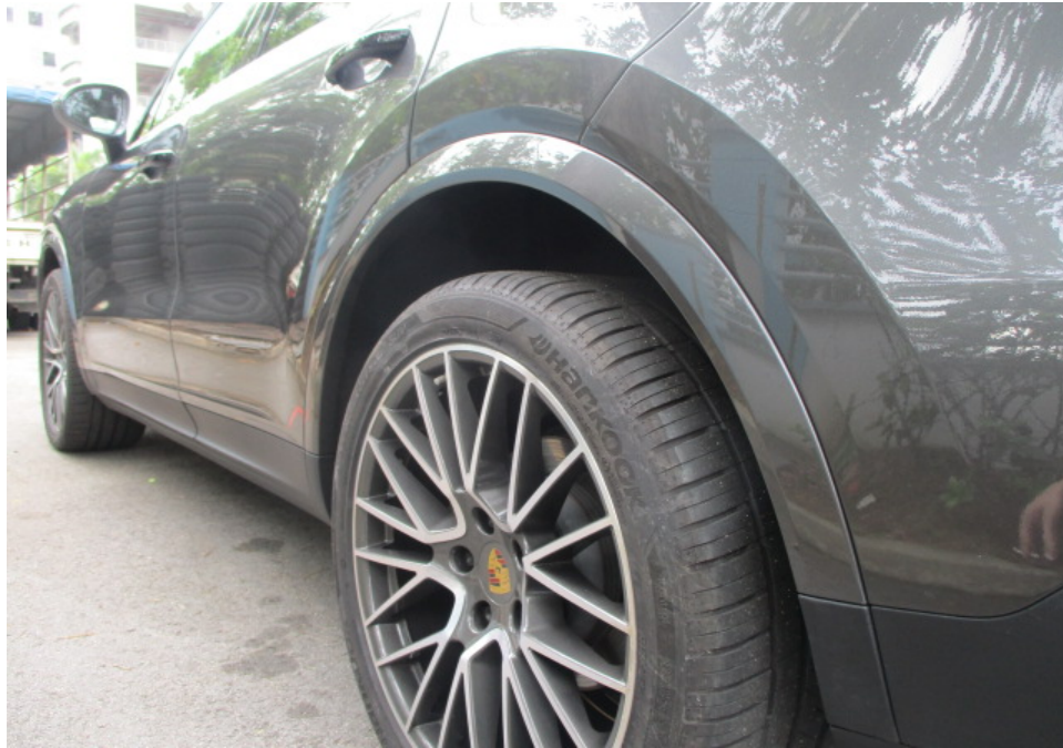
Photo 8 shows a closer view of the Motor Car's rear left fender, rear left fender wheel arc garnish and rear left wheel rim at the time of my inspection. The body parts at the rear left portion of the Motor Car were visually examined and it was observed that the repair/restoration works carried out to the damaged area of the Motor Car (refer to photograph 1 – 3 above) were reasonably adequate and in order.
