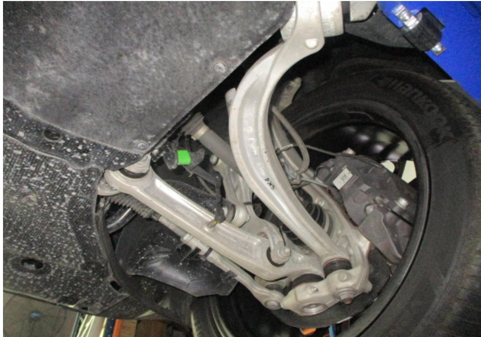
Photo 22 shows the various undercarriage components at the front right wheel of the Motor Car. The mechanical components, control arms and linkages were all found to be intact and secured in an appropriate manner. I also did not observe any fluid leak and/or fluid stain on the underside of the Motor Car.
