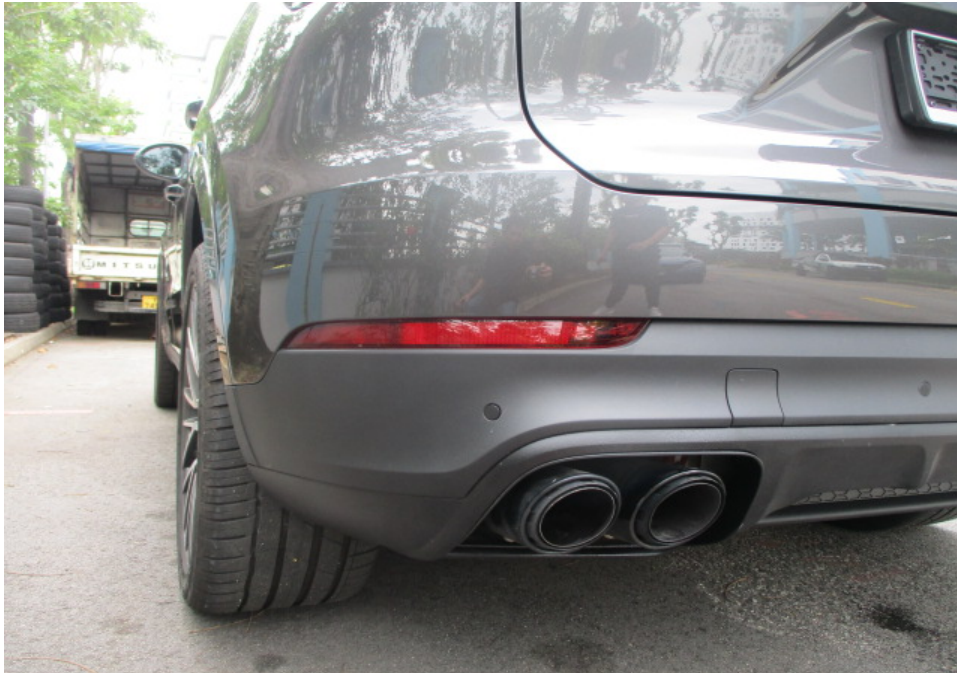
Photo 6 shows a closer view of the Motor Car's rear bumper, rear bumper lower cover, rear bumper lower garnish, rear bumper left sensors and rear bumper left reflector at the time of my inspection. The body parts at the rear left portion of the Motor Car were visually examined and it was observed that the repair/restoration works carried out to the damaged area of the Motor Car (refer to photograph 1 – 3 above) were reasonably adequate and in order.
