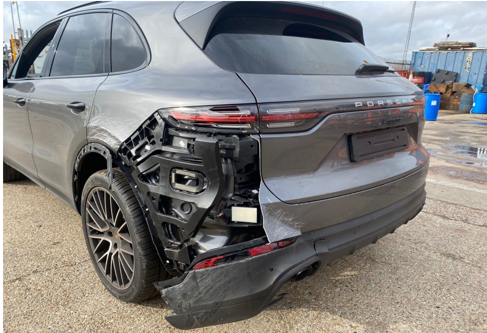
Photo 1 shows the rear left body of the Motor Car (photograph provided to me). The photographs provided to me had showed damage to the rear left portion of the Motor Car. The rear bumper, rear bumper lower cover, rear bumper lower garnish, rear bumper left sensors, rear bumper left reflector, rear bumper left bracket and rear left taillamp were amongst the body parts that were observed to have been damaged.
