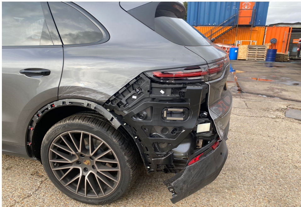
Photo 2 shows another view of the Motor Car's rear left body (photograph provided to me). The photographs provided to me had showed damage to the rear left portion of the Motor Car. The rear bumper, rear bumper lower cover, rear bumper left bracket, rear left taillamp, rear left fender and rear left fender wheel arc garnish were amongst the body parts that were observed to have been damaged.
