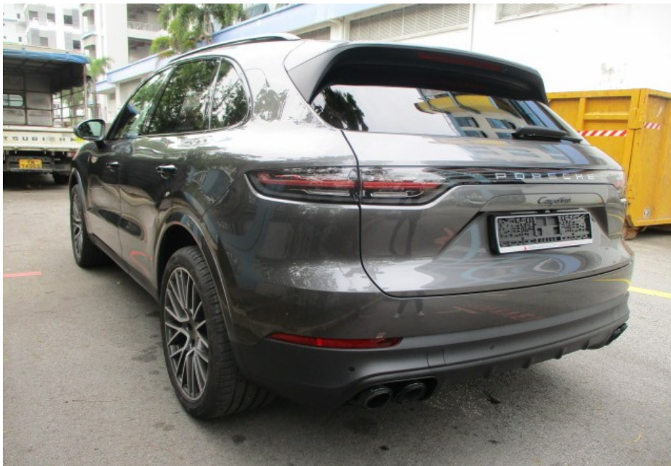
Photo 5 shows a general view of the rear left body of the Motor Car at the time of my inspection. The Motor Car was observed to be in a relatively good general condition with no loose exterior fittings observed. The body parts at the rear left portion of the Motor Car were visually examined and it was observed that the repair/restoration works carried out to the damaged area of the Motor Car (refer to photograph 1 – 3 above) were reasonably adequate and in order.
