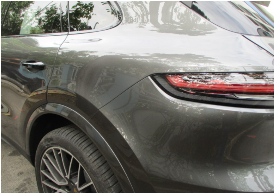
Photo 7 shows a closer view of the Motor Car's rear bumper, rear left taillamp and rear left fender at the time of my inspection. The body parts at the rear left portion of the Motor Car were visually examined and it was observed that the repair/restoration works carried out to the damaged area of the Motor Car (refer to photograph 1 – 3 above) were reasonably adequate and in order.
