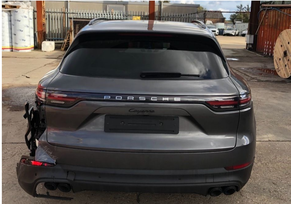
Photo 3 shows the rear body of the Motor Car (photograph provided to me). The photographs provided to me had showed damage to the rear left portion of the Motor Car. Body parts damaged include rear bumper, rear bumper lower cover, rear bumper lower garnish, rear bumper left sensors and rear bumper left reflector amongst others.
