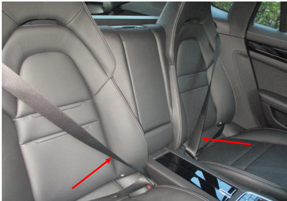
Photo 15 shows the rear seats of the Motor Car. All the seats of the Motor Car were secured via seat rails to the floorboard. They were also fitted with a retractable seat belt reel and a pre-tensioner. The seat belts (arrowed) were tested and were able to be fastened into the respective pre-tensions that were fitted on the side of each individual seat.
