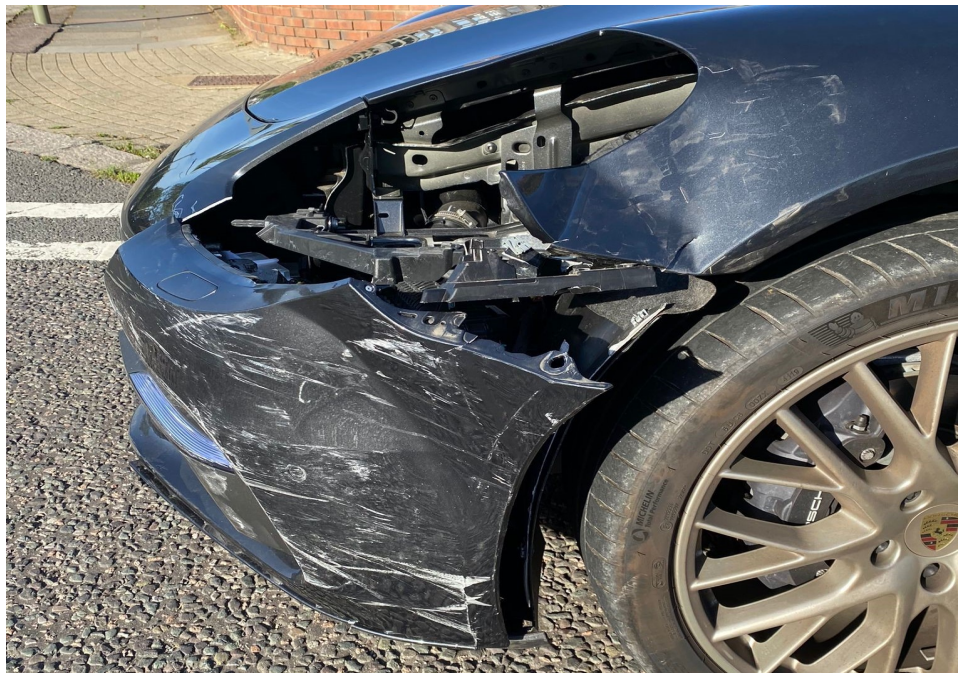
Photo 2 shows another view of the damage at the front left portion of the Motor Car (photograph provided to me). The front bumper, front bumper left sensors, front left headlamp, front left headlamp bracket and front left fender were amongst the body parts that were observed to have been damaged.
