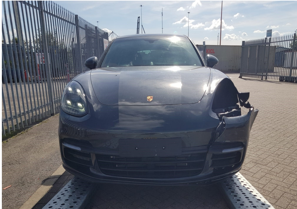
Photo 3 shows the frontal body of the Motor Car (photograph provided to me). The photographs provided to me had showed damage to the front left portion of the Motor Car. The front bumper, front bumper lower lip, front bumper centre lower grille, front bumper left lower grille, front bumper left sensors, front left day light and front left headlamp were amongst the body parts that were observed to have been damaged.
