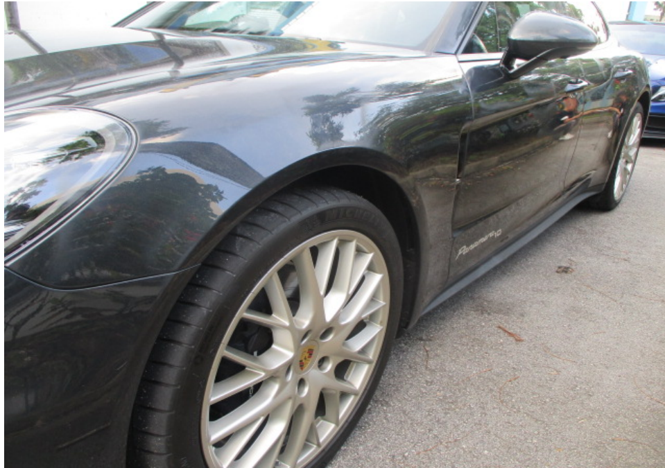
Photo 8 shows a closer view of the Motor Car's front left fender and front left wheel rim at the time of my inspection. The body parts at the front left portion of the Motor Car were visually examined and it was observed that the repair/restoration works carried out to the damaged area of the Motor Car (refer to photograph 1 – 3 above) were reasonably adequate and in order.
