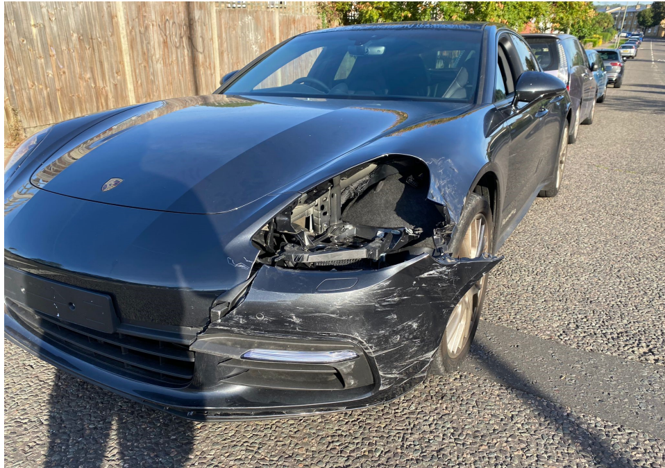
Photo 1 shows the front left body of the Motor Car (photograph provided to me). The photographs provided to me had showed damage to the front left portion of the Motor Car. The front bumper, front bumper lower lip, front bumper centre lower grille, front bumper left lower grille, front bumper left sensors, front left day light, front left headlamp, front left headlamp lower bracket and front left fender were amongst the body parts that were observed to have been damaged.
