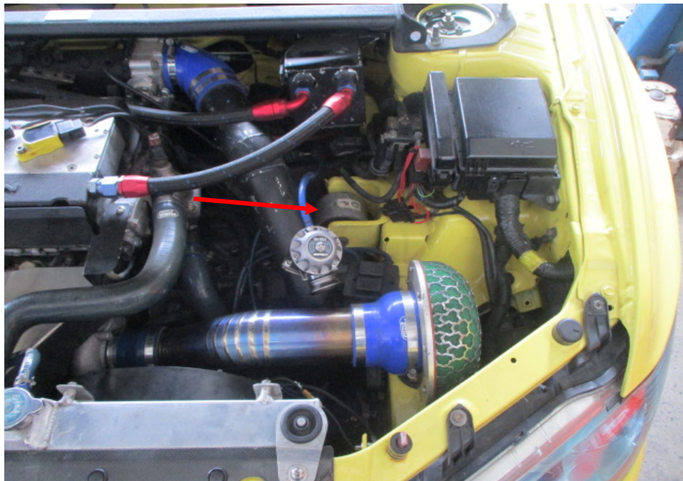
Photo 10 shows the bracket (arrowed) supporting the top left of the Motor Car's transmission. This bracket was found to be mounted onto the left side front chassis, adjacent to the left side front wheel house. The mounting of this bracket is the original mounting point for the this bracket as the welding for the support of this bracket was of original weld.
