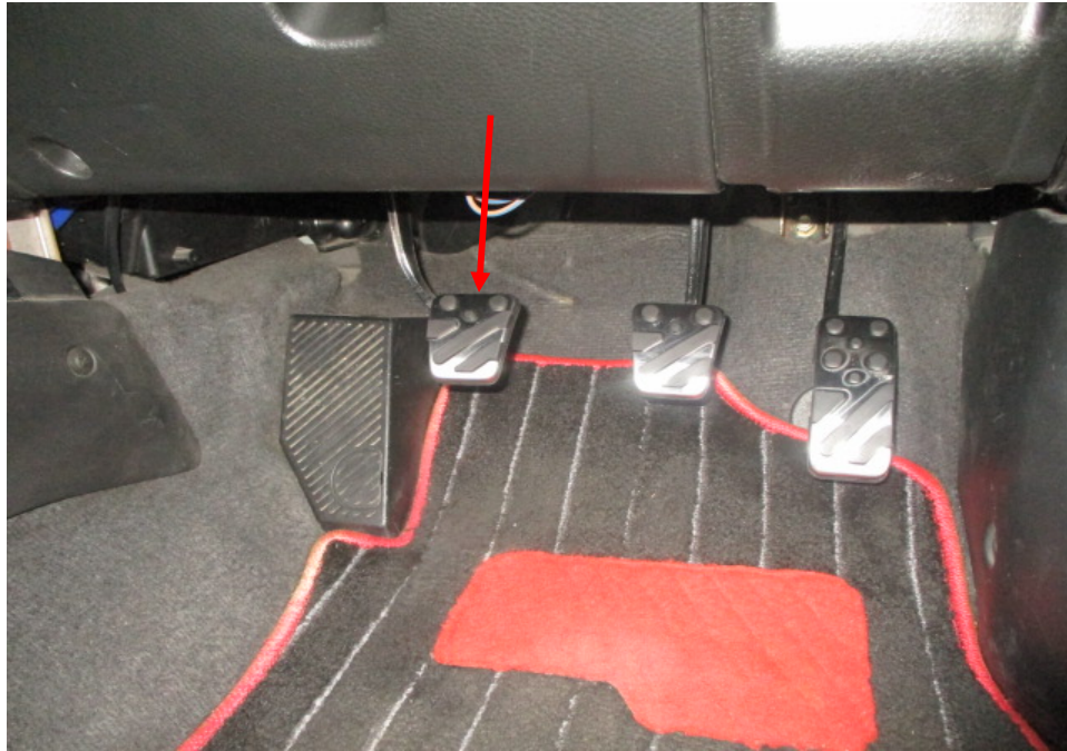
Photo 13 shows the clutch pedal (arrowed) of the Motor Car, for engaging and disengaging the transmission gears.
