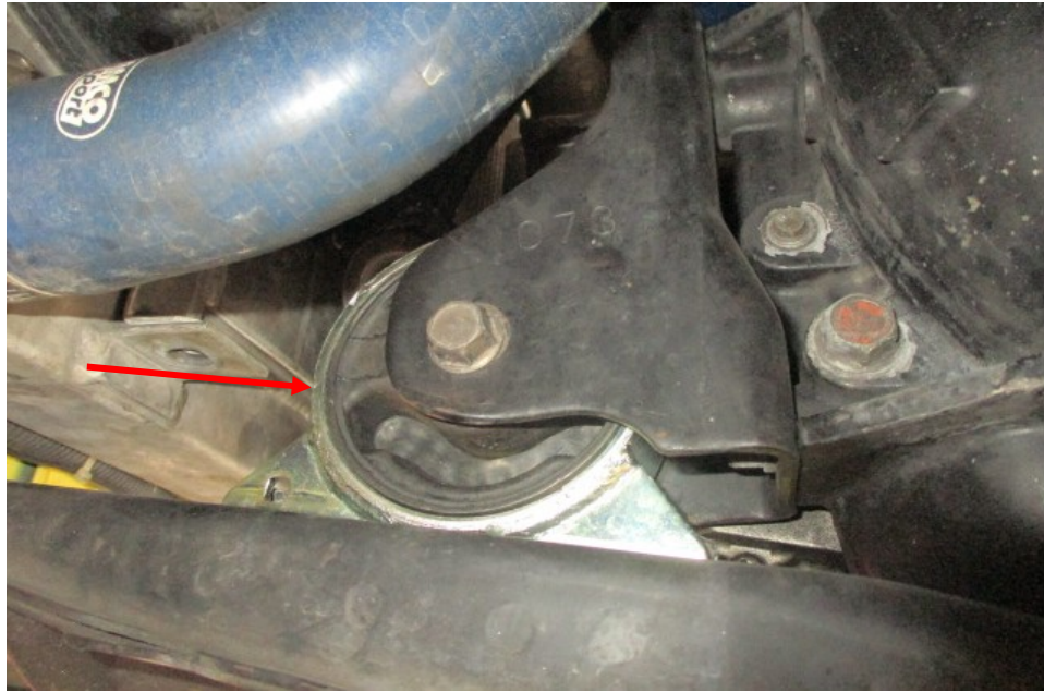
Photo 9 shows a closer view of the bracket supporting the front of the Motor Car's transmission. Similar to the bracket at the rear, this bracket (arrowed) was also with rubber bushing, which absorbs any vibrations arising from the rotation of the transmission gears, minimising any stress to the bracket and correspondingly also minimise any stress to the longitudinal crossmember that this bracket is mounted onto.
