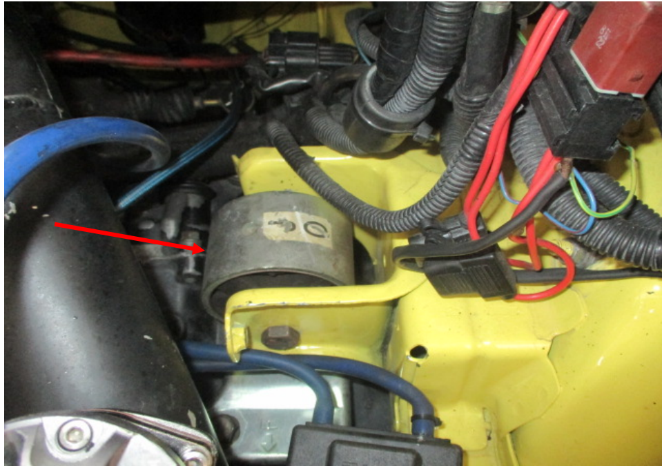
Photo 11 shows a closer view of the bracket (arrowed) supporting the top left of the Motor Car's transmission. This bracket was found to be mounted onto the left side front chassis, adjacent to the left side front wheel house. The mounting of this bracket is the original mounting point for this bracket as the welding for the support of this bracket was of original weld. This bracket was also with rubber bushing, which absorbs any vibrations arising from the rotation of the transmission gears, minimising any stress to the bracket and correspondingly also minimise any stress to the left side front chassis.
