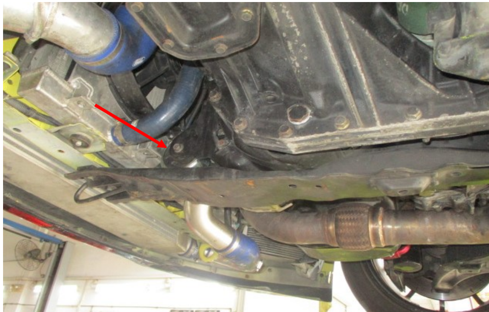
Photo 8 shows the bracket at the front of the Motor Car's transmission, which was observed to be mounted onto the Motor Car's longitudinal crossmember. Similar to the bracket at the rear, this bracket (arrowed) was also with rubber bushing, which absorbs any vibrations arising from the rotation of the transmission gears, minimising any stress to the bracket and correspondingly also minimise any stress to the longitudinal crossmember that this bracket is mounted onto.
