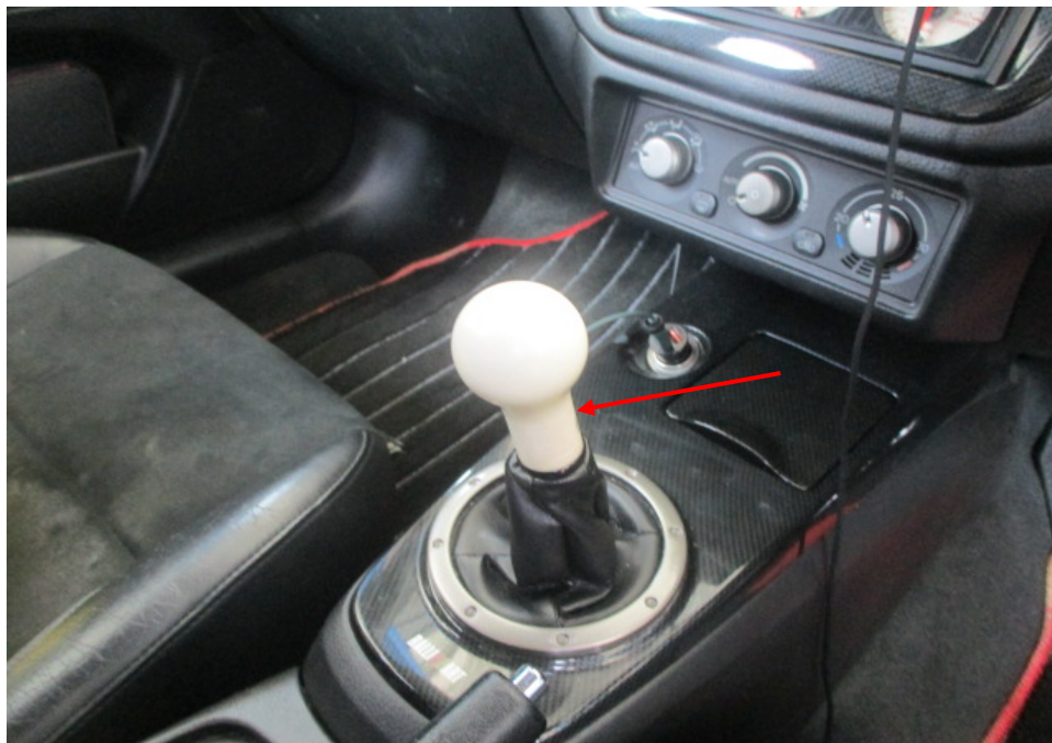
Photo 12 shows the manual gear shifter (arrowed) that was fitted on the Motor Car, for manually selecting the transmission gear to be engaged.
