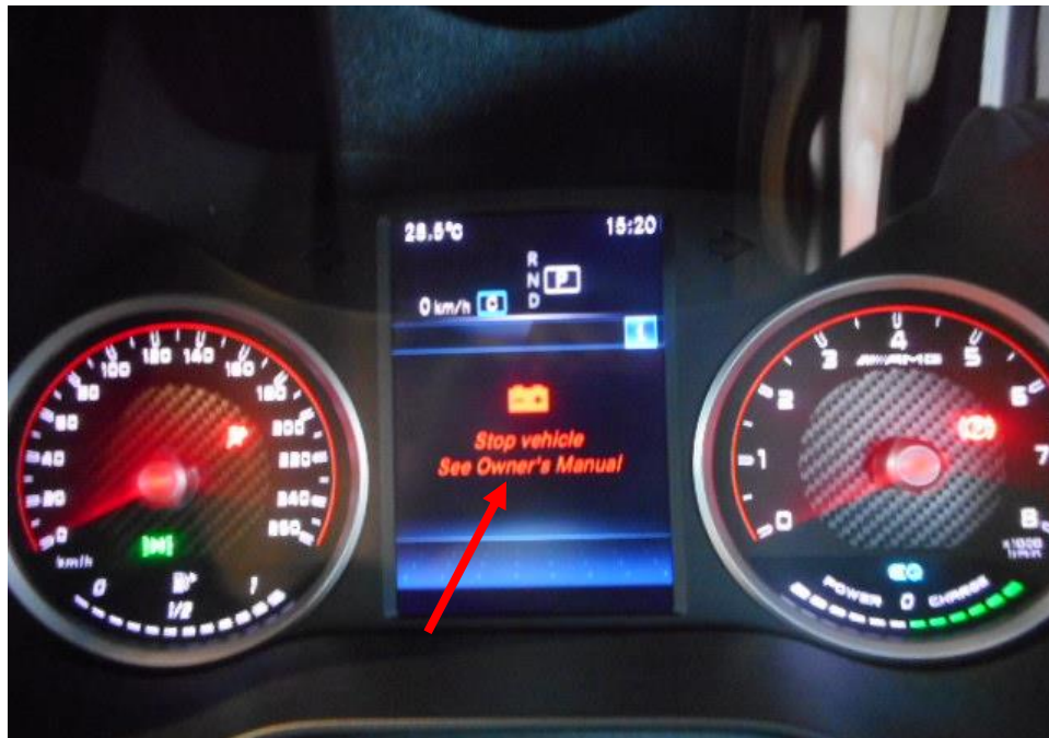
Photo 8 shows the conducted ECU diagnosis of the Insured Vehicle at the time of our inspection. There was an electronic error (arrowed) on the 48v battery integrated starter system (ISG) of the Insured Vehicle.
