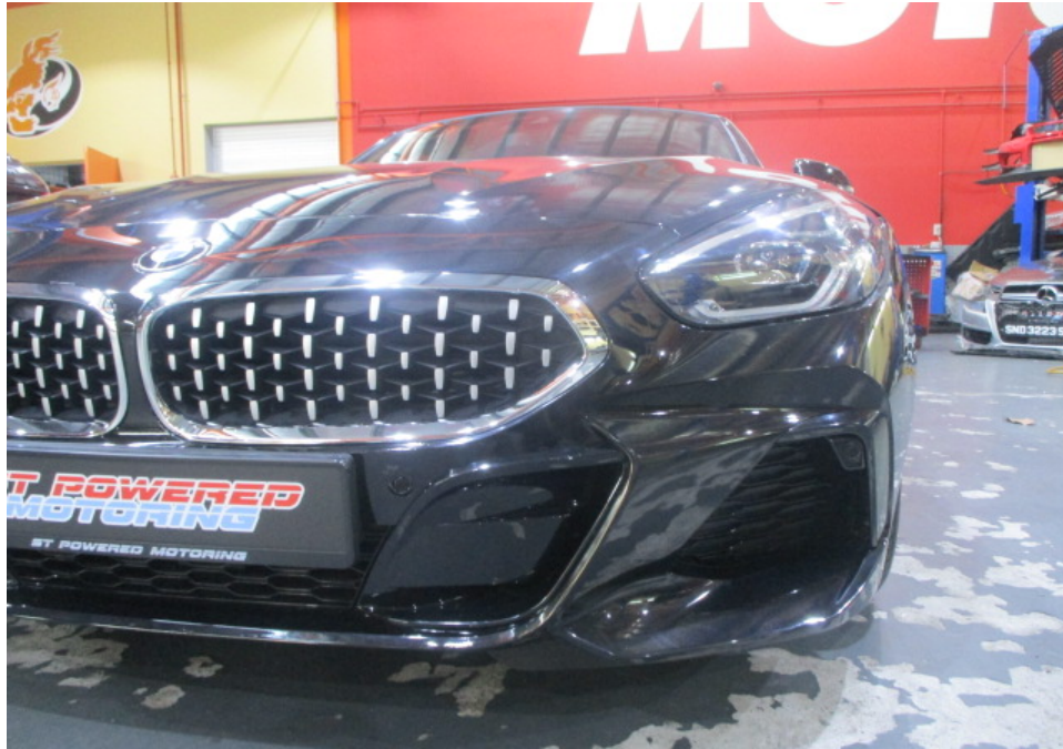
Photo 6 shows a closer view of the Motor Car's front bumper, front bumper centre lower grille, front bumper left lower grille, radiator grilles and front left headlamp. The body parts at the front left portion of the Motor Car were visually examined and it was observed that the repair/restoration works carried out to the damaged area of the Motor Car (refer to photograph 1 above) were reasonably adequate and in order.
