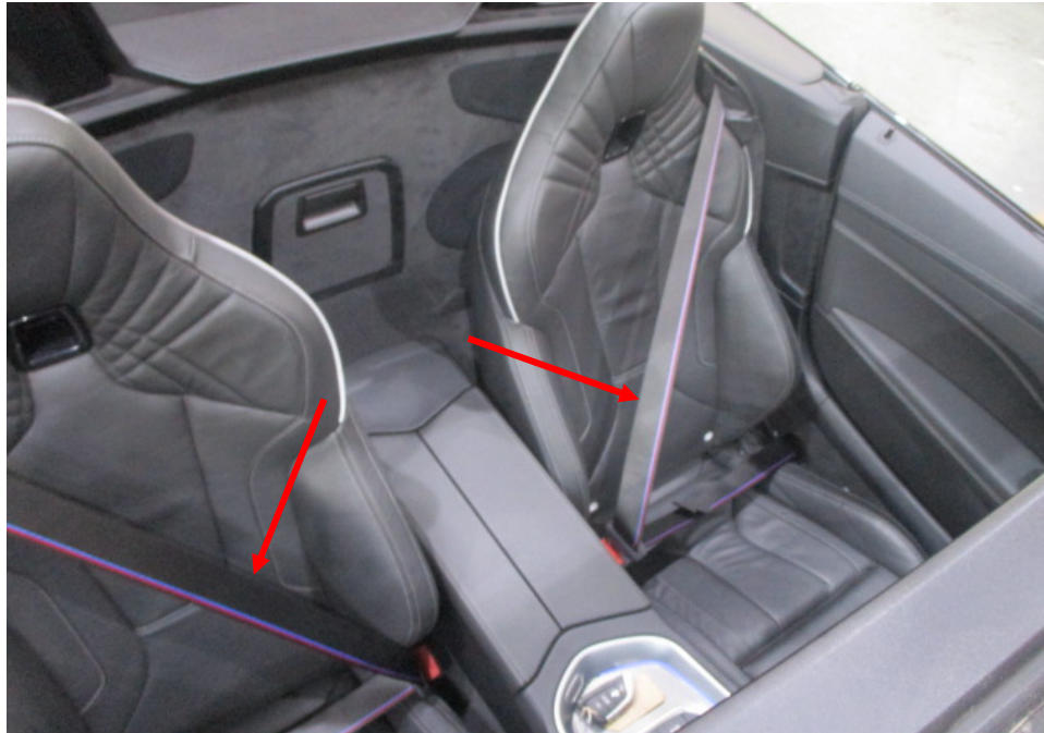
Photo 14 shows the seats of the Motor Car. All the seats of the Motor Car were secured via seat rails to the floorboard. They were also fitted with a retractable seat belt reel and a pre-tensioner. The seat belts (arrowed) were tested and were able to be fastened into the respective pre-tensions that were fitted on the side of each individual seat.
