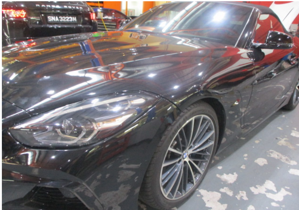
Photo 7 shows a closer view of the Motor Car's front left headlamp, front left fender, front left wheel rim, front bonnet and left wing mirror. The body parts at the front left portion of the Motor Car were visually examined and it was observed that the repair/restoration works carried out to the damaged area of the Motor Car (refer to photograph 1 above) were reasonably adequate and in order.
