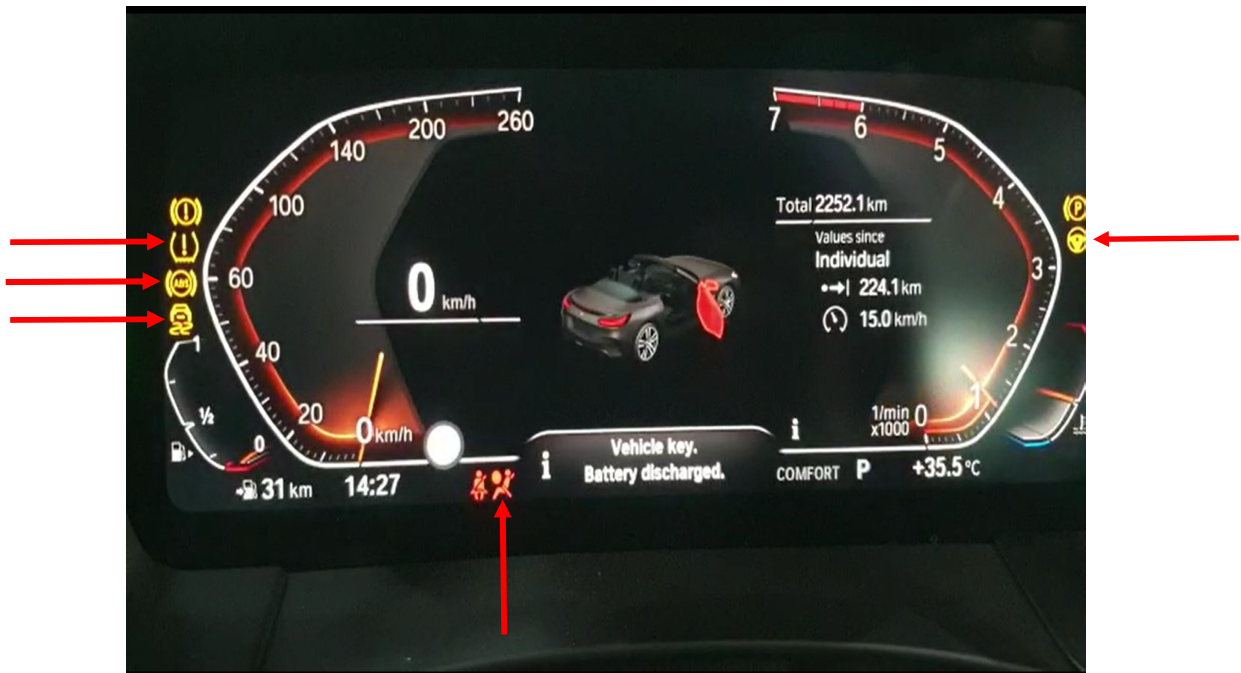
Photo 17 shows the warning lights for the various electronic safety features appearing on the instrument panel of the Motor Car during its self-test when the engine is cranked, in particular ABS, SRS, IAS, TPM and DSC lights (arrowed).
