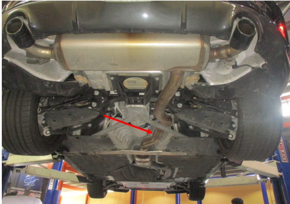
Photo 24 shows the rear section of the Motor Car's exhaust system. My examination of the Motor Car's exhaust system revealed no sign(s) or indication(s) of any cut or weld marks along its exhaust pipes (arrowed), on its rear muffler, on its centre resonator box and on its catalytic converter.
