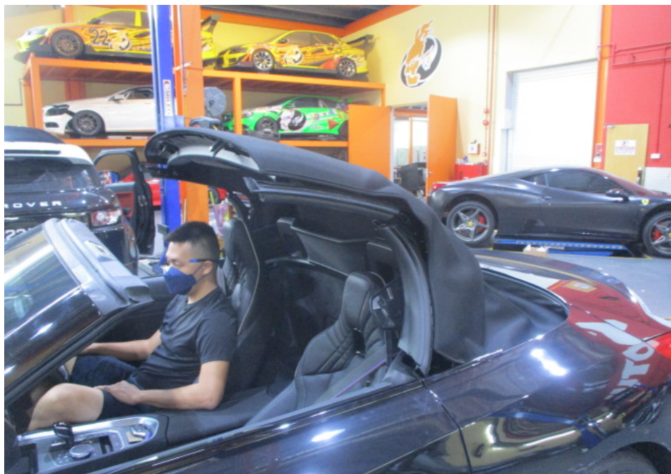
Photo 15 shows the Motor Car's soft top roof being tested. It was observed that as a safety feature, the soft top roof could only open and close when the Motor Car was in a stationary position. When opened, the soft top roof is completely folded into the rear compartment with no parts protruding out of the Motor Car's body. The soft top roof was also found adequately secured to the "A" pillar after closing.
