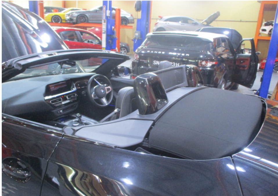
Photo 16 shows the Motor Car with its soft top roof completely folded. It was observed that as a safety feature, the soft top roof could only open and close when the Motor Car was in a stationary position. When opened, the soft top roof is completely folded into the rear compartment with no parts protruding out of the Motor Car's body. The soft top roof was also found adequately secured to the "A" pillar after closing.
