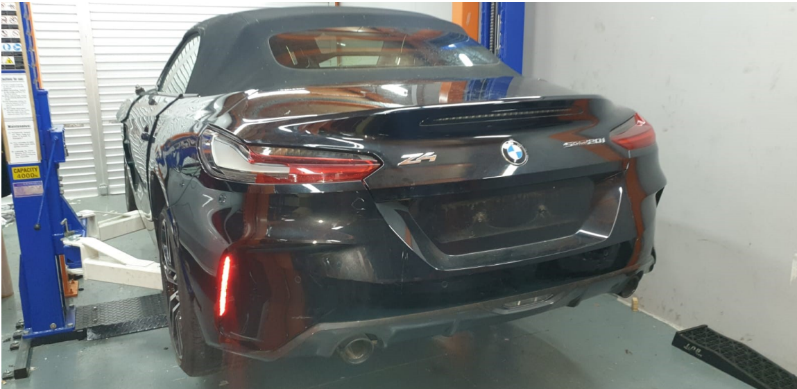
Photo 4 shows the rear left body of the Motor Car (photograph provided to me). The rear left portion of the Motor Car was observed to be relatively unaffected and without any physical damage except for the rear left taillamp, which was observed to be cracked.
