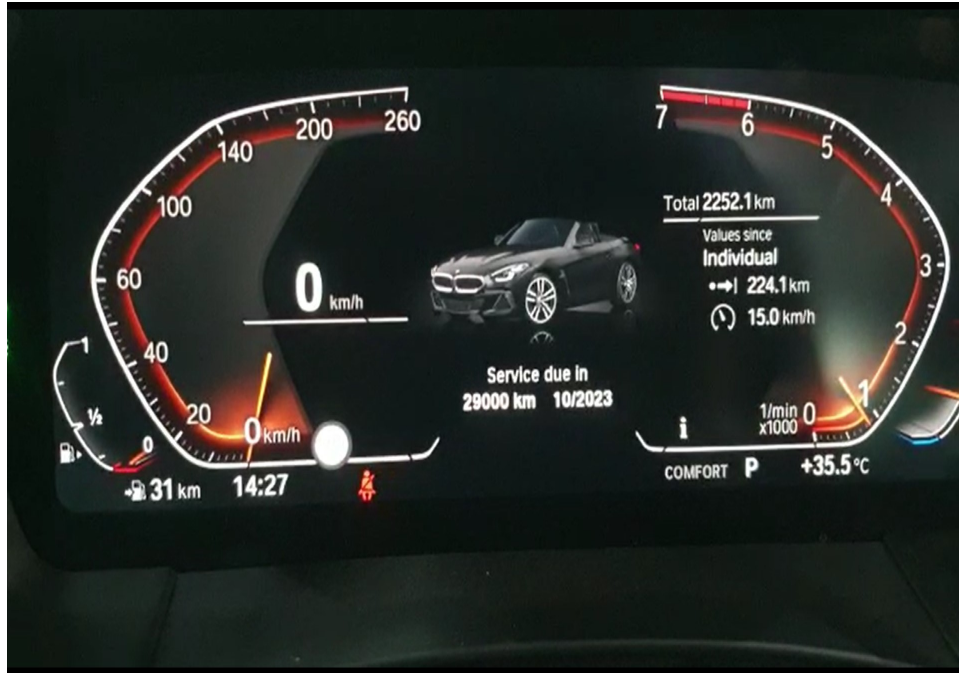
Photo 18 shows the respective warning lights no longer illuminated, indicating that there is no fault detected to ABS, SRS, IAS, TPM and DSC systems of the Motor Car during the self-test. These electronic systems were hence in working condition at the time of my inspection.
