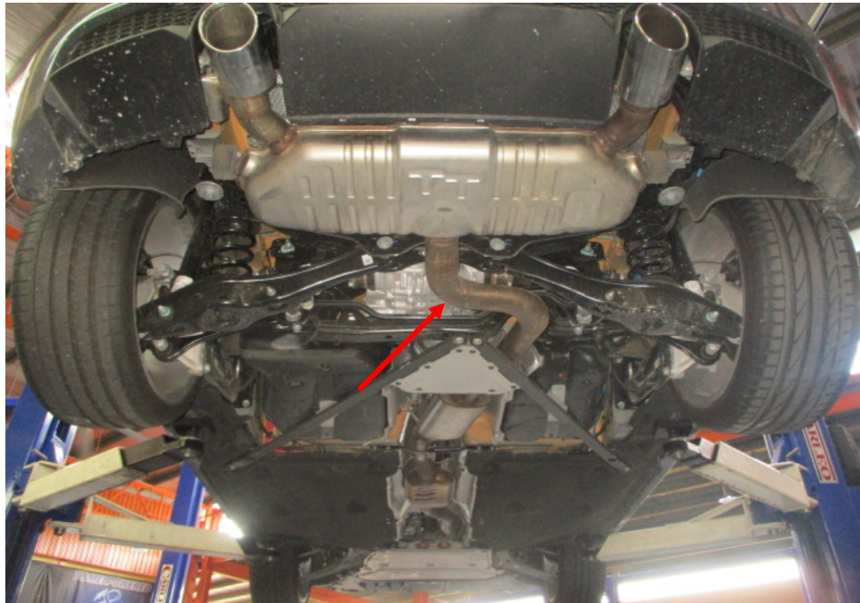
Photo 25 shows the rear section of the Motor Car's exhaust system. My examination of the Motor Car's exhaust system revealed no sign(s) or indication(s) of any cut or weld marks along its exhaust pipes (arrowed), on its rear muffler, on its centre resonator boxes and on its catalytic converter.
