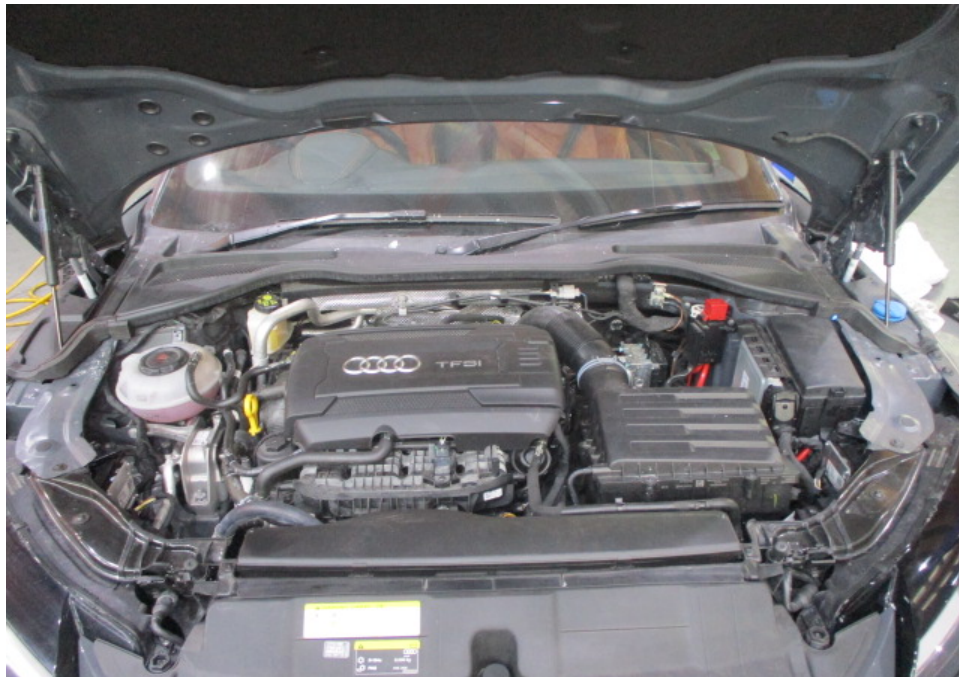
Photo 13 shows a general view of the engine compartment of the Motor Car at the time of my inspection. The various parts and components inside the engine compartment were all observed to be intact and properly fitted. There was also no sign(s) or indication(s) of fluid leak and/or fluid stain found inside the engine compartment. The repair/restoration works carried out to the various parts within the engine compartment like the front right headlamp panel, front right fender top inner panel, front support panel centre garnish and front support panel amongst others, were reasonably adequate and in order.
