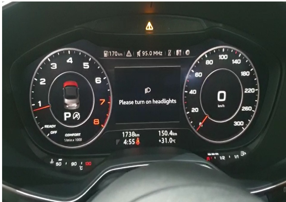
Photo 19 shows the respective warning lights no longer illuminated, indicating that there is no fault detected to ABS, SRS, EPS, TPM and ESC systems of the Motor Car during the self-test. These electronic systems were hence in working condition at the time of my inspection.
