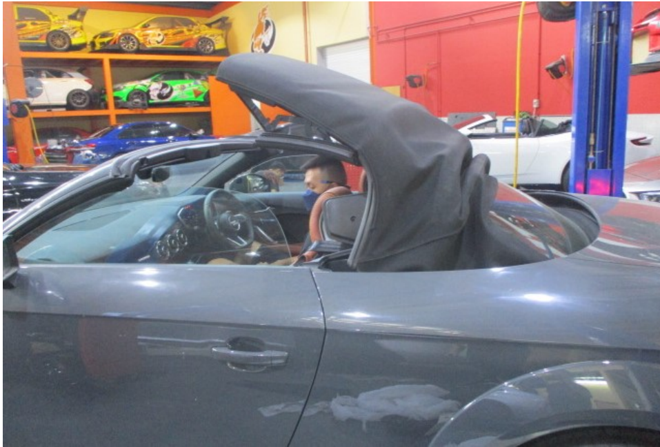
Photo 16 shows the Motor Car's soft top roof being tested. It was observed that as a safety feature, the soft top roof could only open and close when the Motor Car was in a stationary position. When opened, the soft top roof is completely folded into the rear compartment with no parts protruding out of the Motor Car's body. The soft top roof was also found adequately secured to the "A" pillar after closing.
