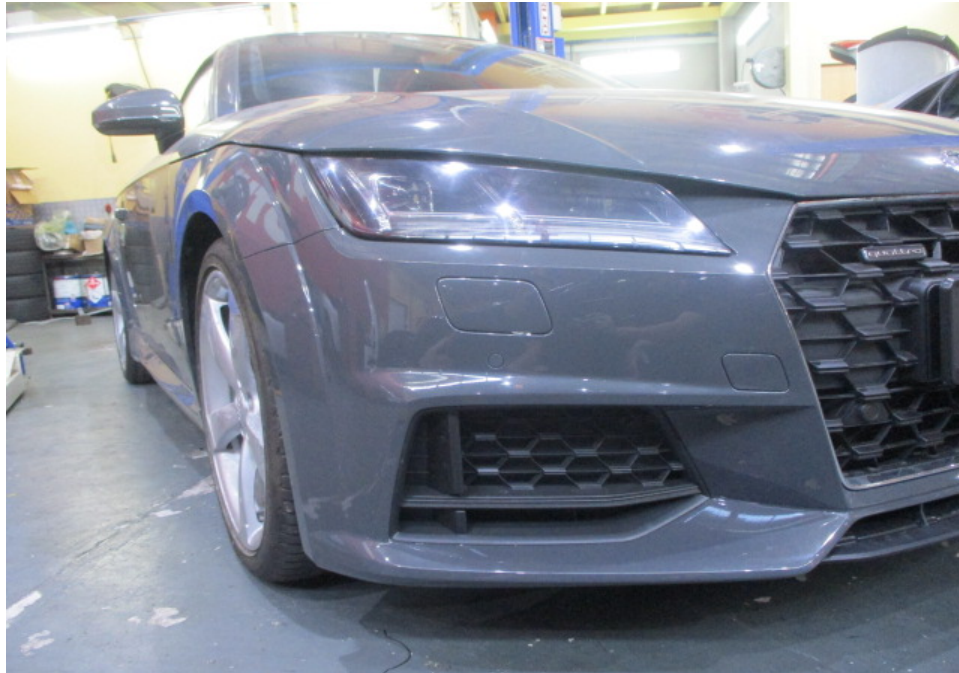
Photo 6 shows a closer view of the Motor Car's front bumper, front bumper right lower grille, front bumper tow hook cover and front right headlamp. The body parts at the front right portion of the Motor Car were visually examined and it was observed that the repair/restoration works carried out to the damaged area of the Motor Car (refer to photograph 1 above) were reasonably adequate and in order.
