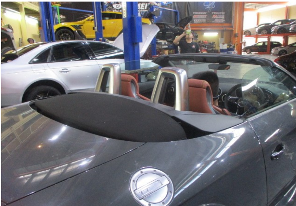
Photo 17 shows the Motor Car with its soft top roof completely folded. It was observed that as a safety feature, the soft top roof could only open and close when the Motor Car was in a stationary position. When opened, the soft top roof is completely folded into the rear compartment with no parts protruding out of the Motor Car's body. The soft top roof was also found adequately secured to the "A" pillar after closing.
