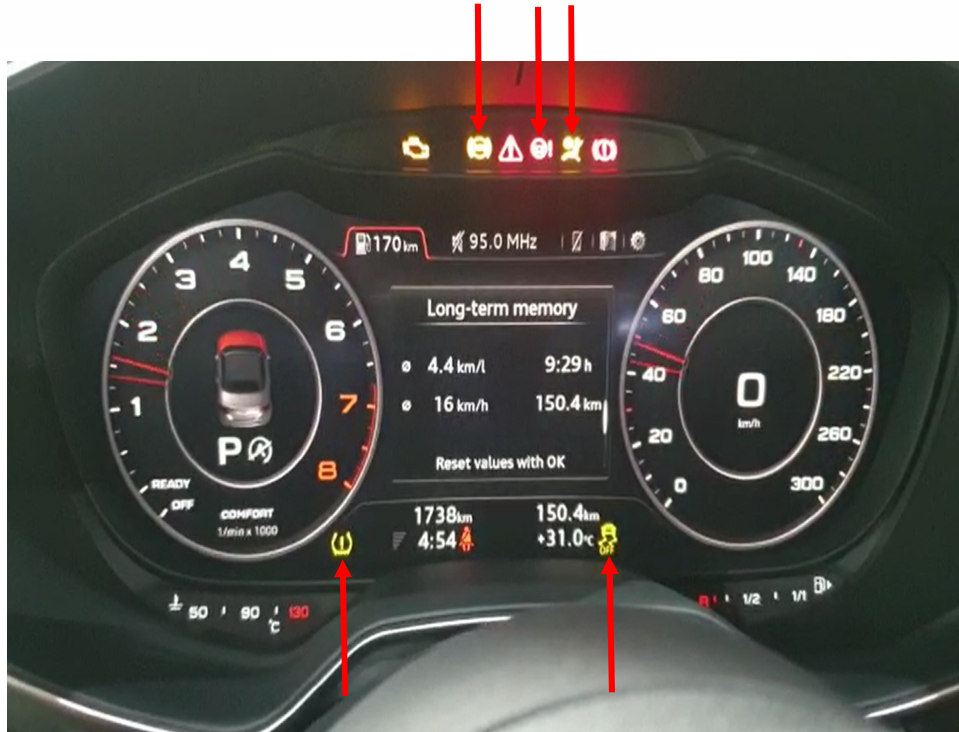
Photo 18 shows the warning lights for the various electronic safety features appearing on the instrument panel of the Motor Car during its self-test when the engine is cranked, in particular ABS, SRS, EPS, TPM and ESC lights (arrowed).
