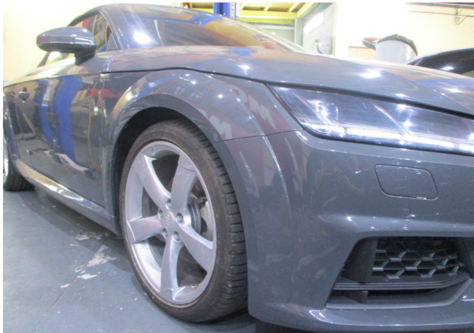
Photo 7 shows a closer view of the Motor Car's front bumper, front right headlamp, front right fender, front right wheel rim and front bonnet. The body parts at the front right portion of the Motor Car were visually examined and it was observed that the repair/restoration works carried out to the damaged area of the Motor Car (refer to photograph 1 above) were reasonably adequate and in order.
