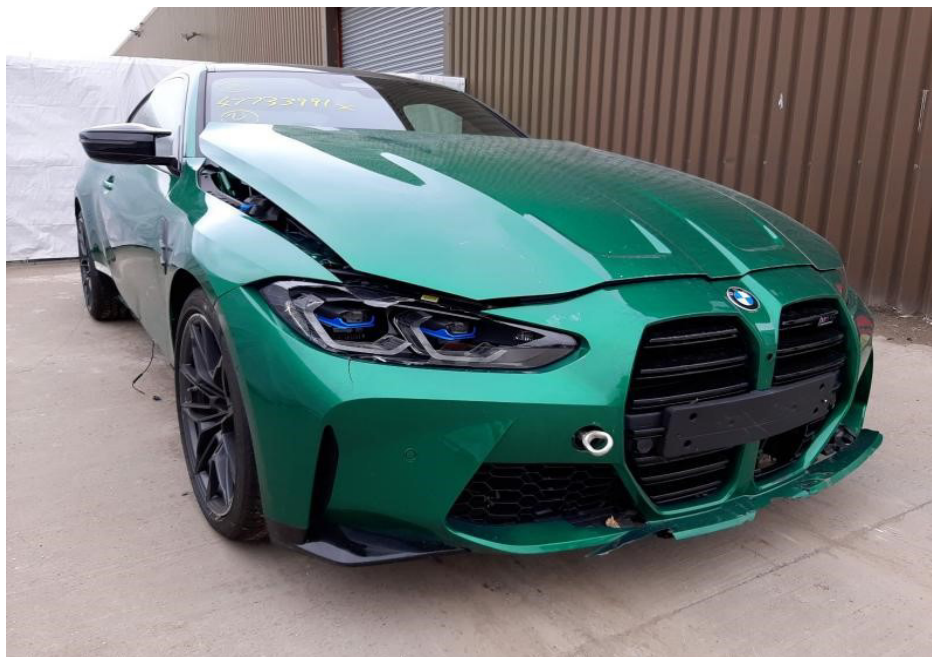
Photo 1 shows the front right body of the Motor Car (photograph provided to me). The photographs provided to me had showed damage to the frontal portion and front underside of the Motor Car. The front bumper, front bonnet and front right headlamp were amongst the body parts that were observed to have been damaged.
