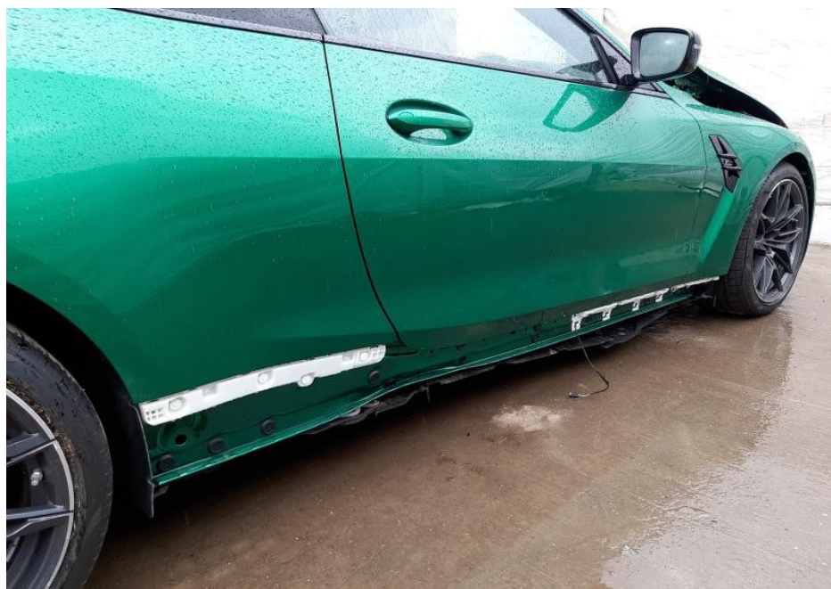
Photo 4 shows the right side body of the Motor Car (photograph provided to me). Apart for the damage to the frontal portion and front underside of the Motor Car, I had also observed that the Motor Car's right side lower skirting was dislodged/damaged/missing.
