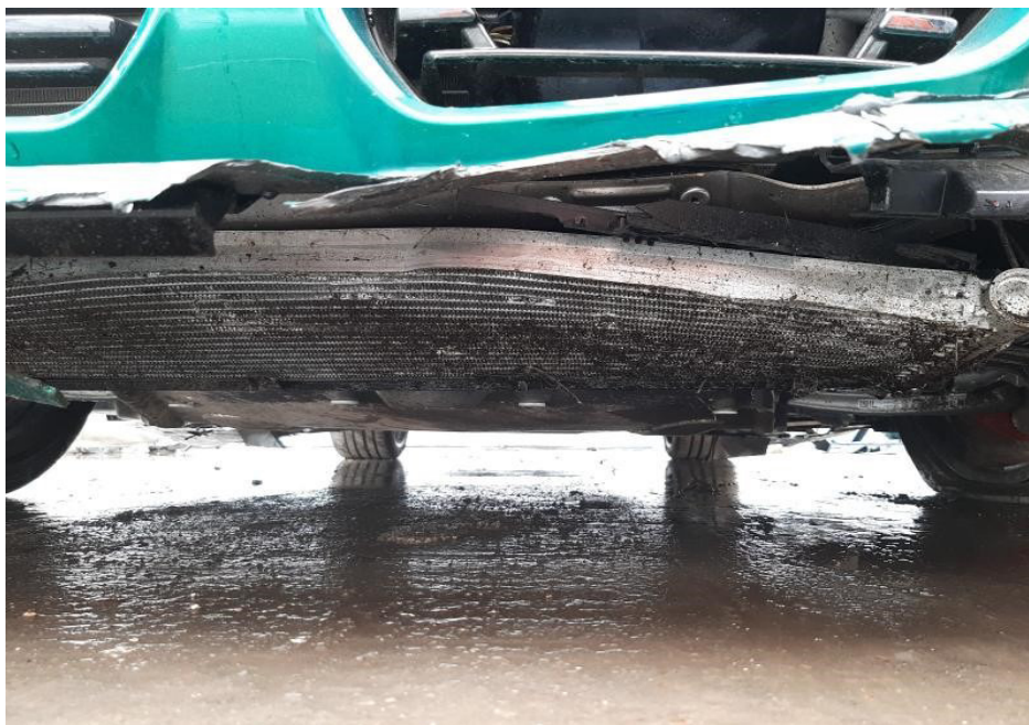
Photo 3 shows the front underside of the Motor Car (photograph provided to me). The front bumper, front under cover and oil cooler were amongst the body parts at the front underside of the Motor Car that were observed to have been damaged.
