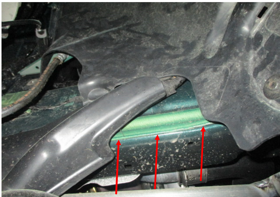
Photo 30 shows the chassis/structural body at the underside front right of the Motor Car. The original factory sealant (arrowed) at the joints along the chassis/structural body was observed to be untouched. In general, I had found no work was carried out on the chassis/structural body of the Motor Car. The chassis/structural body of the Motor Car was originally fitted.
