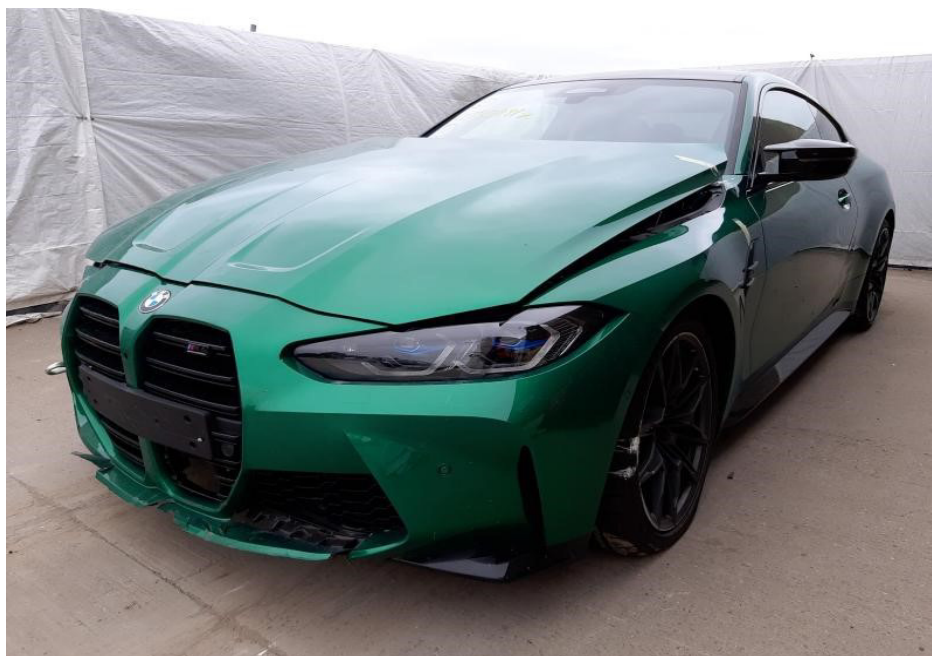
Photo 2 shows the front left body of the Motor Car (photograph provided to me). The photographs provided to me had showed damage to the frontal portion and front underside of the Motor Car. The front bumper, front bumper left lower grille and front bonnet were amongst the body parts that were observed to have been damaged.
