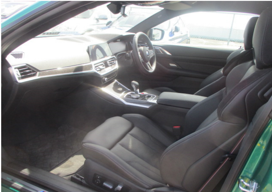
Photo 16 shows the interior compartment of the Motor Car at the time of my inspection. The various parts and components, trims, carpet, and upholstery inside the interior compartment were all observed to be intact and properly fitted.
