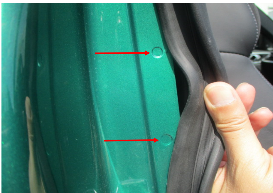
Photo 33 shows the right side rear body panel of the Motor Car. I did not find any weld marks other than original spot weld marks (arrowed) on the right side rear body panel of the Motor Car which, indicates that there was no re-welding works carried out. In general, I had found all the non-detachable body panels of the Motor Car to be originally fitted at the time of my inspection.
