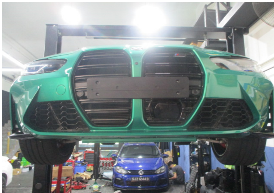
Photo 20 shows the Motor Car hoisted up for checks on its undercarriage. There was no sign(s) or indication(s) of fluid leakage and/or fluid stain(s) on the underside of the Motor Car. The undercarriage components of the Motor Car were also all observed to be intact and secured in an appropriate manner.
