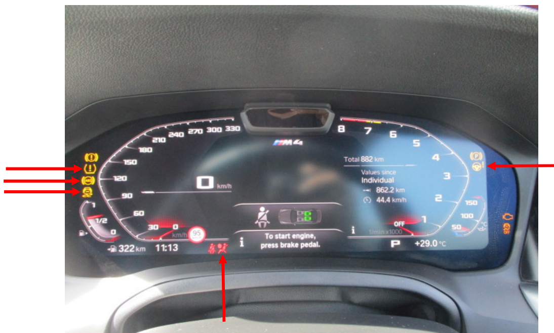
Photo 18 shows the warning lights for the various electronic safety features appearing on the instrument panel of the Motor Car during its self-test when the engine is cranked, in particular the ABS, SRS, IAS, TPM and DSC lights (arrowed).
