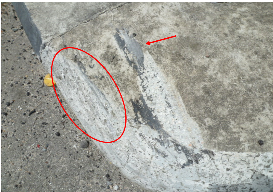
Photo 4 shows a close up view of the graze marks (circled) and tyre marks (arrowed) found on the kerb which Ms Pek had mounted.
