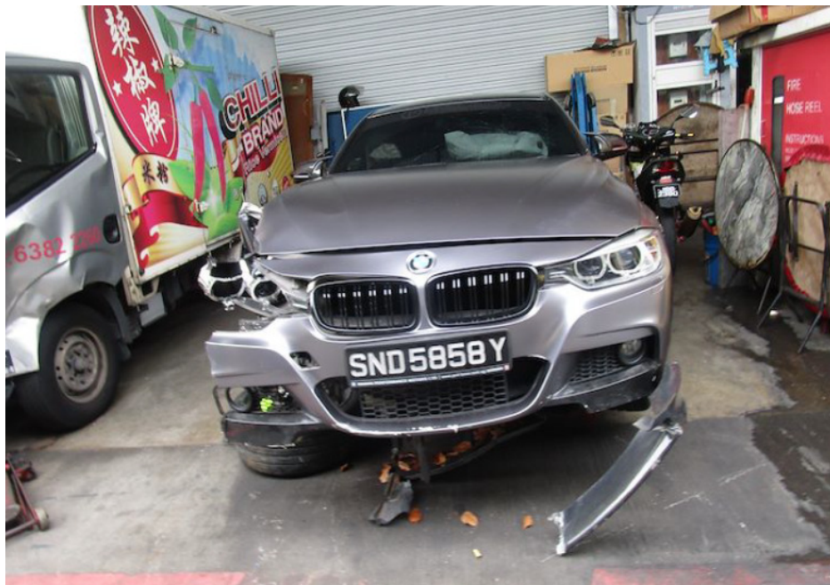
Photo 11 shows the general frontal view of the Insured Vehicle during the physical inspection at SME. The Insured Vehicle had sustained significant damages to its frontal portion and right body.
