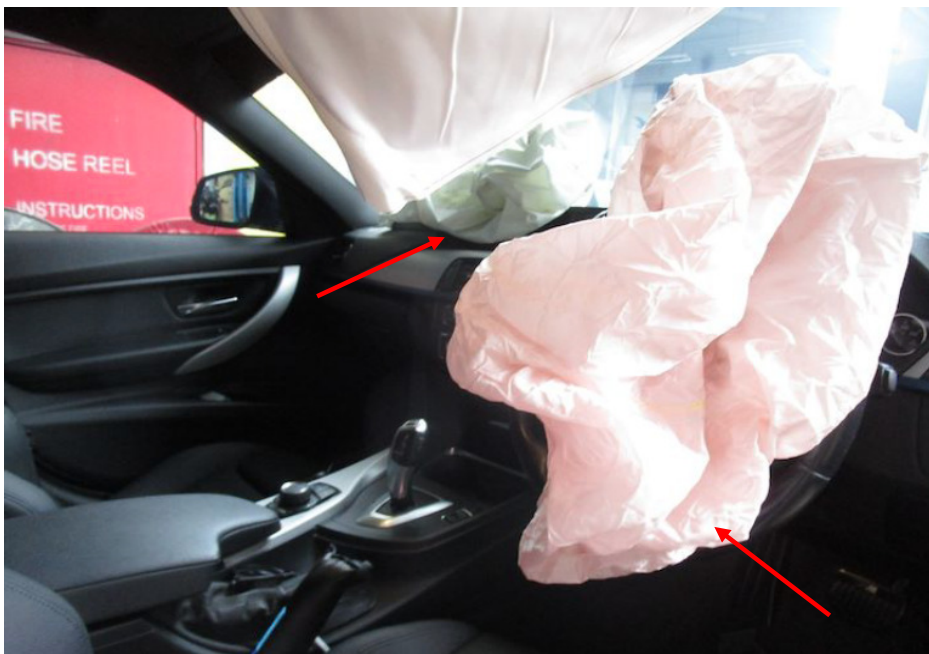
Photo 13 shows the remains of the driver and front passenger airbags of the Insured Vehicle (arrowed) which corroborates with Ms Pek's statement that the airbags were deployed post- incident.
