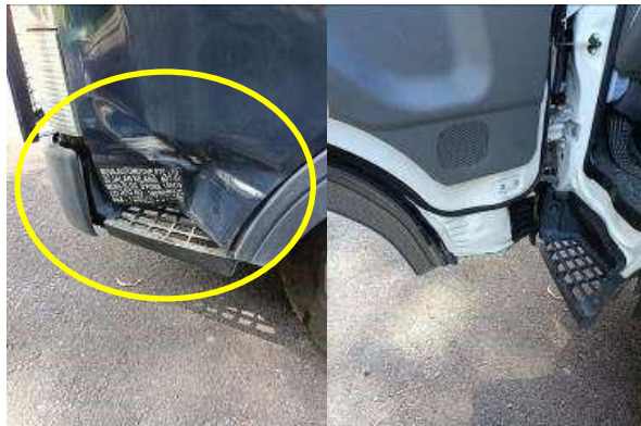
Figure 3. Dent Damage of MMRC's Lorry Left-Hand Side Passenger Side Door
