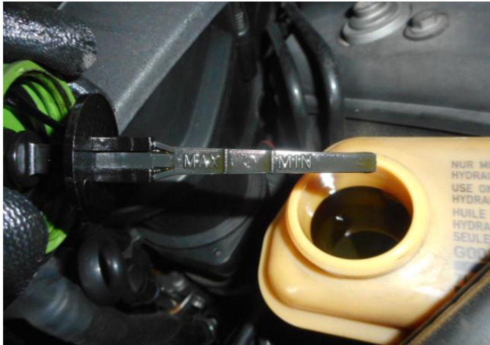
Photo 15 shows the power steering fluid dip stick of the Motor Car at the time of my inspection. The engine oil was observed to be of sufficient level and without any visible contamination.
