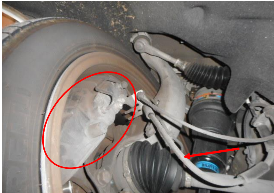
Photo 23 shows the brake hose/pipe (arrowed) at the front left wheel of the Motor Car. No leakage of brake fluid was observed. Visual examination of the various components of the braking system like the brake caliper (circled), brake booster, brake pedal etc had revealed all to be intact and without visible damage at the time of incident. There was also no sign of fluid stain(s) observed on the various undercarriage components.
