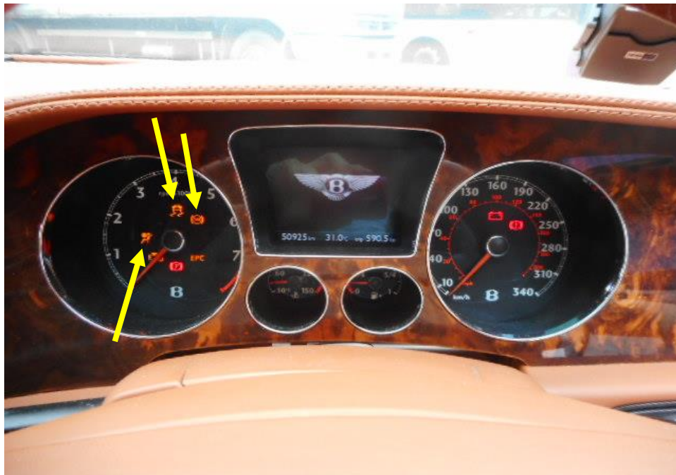
Photo 25 shows the warning light for Anti-Lock Brake System (ABS), Traction Control System (TCS), and Supplemental Restraint System (SRS) appearing on the instrument panel of the Motor Car during the self-test of its various electronic operating systems when its engine was cranked.
