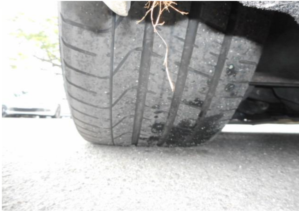
Photo 10 shows the condition of the rear right tyres of the Motor Car, which were observed to be in serviceable condition with remaining, tread depth of approximately 4.8mm. There was also no tear, cut or burst mark(s) on the outer and the inner sidewalls as well as across the tread of the 4 tyres that were fitted on the Motor Car.
