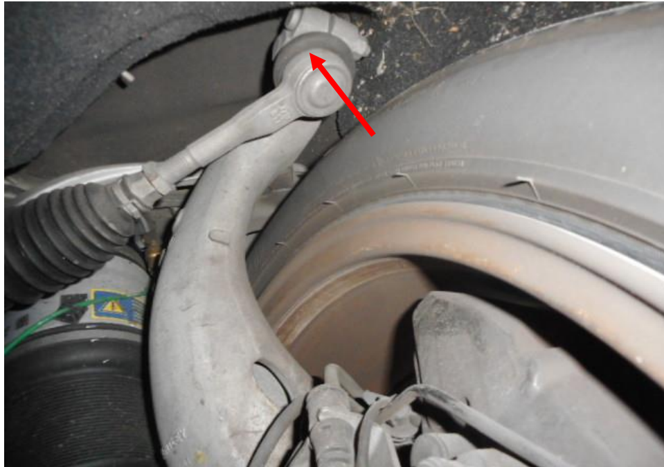
Photo 17 shows the various undercarriage components at the front right wheel of the Motor Car, in particular the steering tie rod end (arrowed). The various steering components were all found to be intact, suggesting that the steering system of the Motor Car was likely to be in serviceable condition at the material time of incident. There was also no sign of fluid stain(s) observed on the various undercarriage components.
