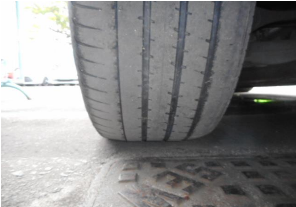
Photo 9 shows the condition of the rear left tyres of the Motor Car, which was observed to be in serviceable condition with remaining tread depth of approximately 2.7mm. The tyres, which were wrapped around standard alloy wheel rim, were also observed to be sufficiently inflated for vehicular operation. There was also no damage found on all 4 alloy wheel rims of the Motor Car.
