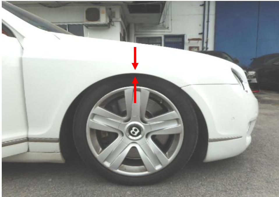
Photo 28 shows the front right wheel of the Motor Car. The vehicle body was observed to be lowered than normal (arrowed) due to the insufficient air in the air suspension as a result of a period of storage in the vehicle pound.
