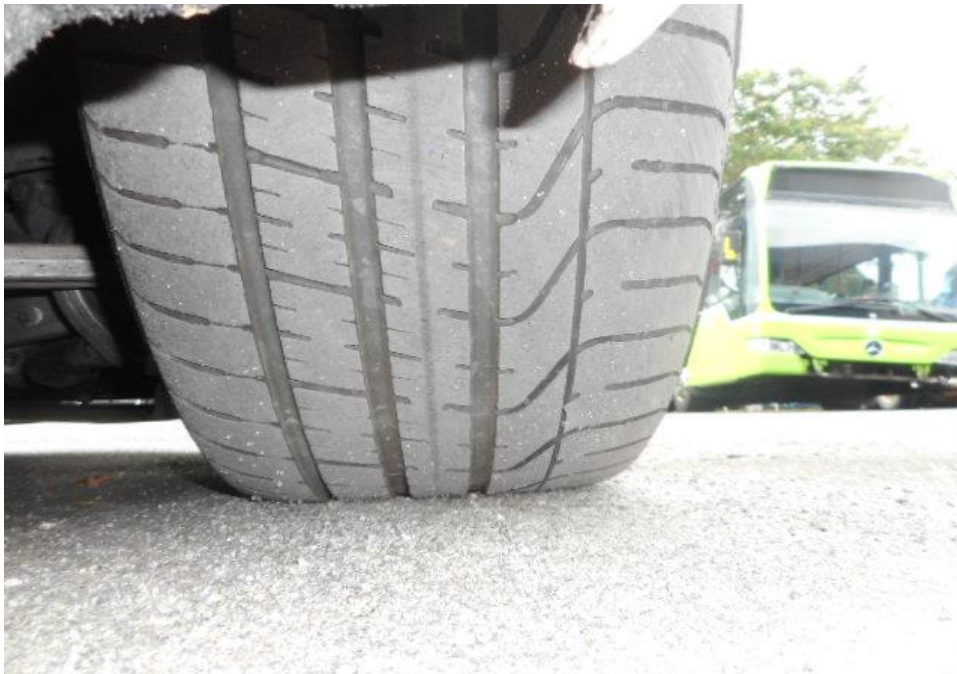
Photo 7 shows the condition of the front right tyre of the Motor Car, which was observed to be in serviceable condition with remaining tread depth of approximately 4.7mm. The tyre, which was wrapped around standard alloy wheel rim, was also observed to be sufficiently inflated for vehicular operation. There was no tear, cut or burst mark(s) on the outer and the inner sidewalls as well as across the tread of the 4 tyres that were fitted on the Motor Car.
