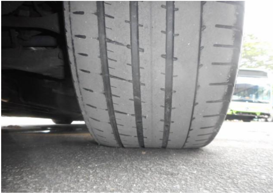
Photo 8 shows the condition of the rear right tyre of the Motor Car, which was observed to be in serviceable condition with remaining tread depth of approximately 3.1mm. The tyre, which was wrapped around standard alloy wheel rim, was also observed to be sufficiently inflated for vehicular operation.
