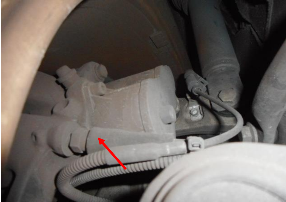
Photo 21 shows the brake pipe (arrowed) at the rear left wheel of the Motor Car. I did not observe any leakage of brake fluid at the time of my inspection of the Motor Car. My static tests of the Motor Car's braking system, along with my visual examination of the various mechanical components in the braking system had indicated that there was no internal leakage of pressure/vacuum. Hence the braking system of the Motor Car was likely to be in serviceable condition at the material time of incident.
