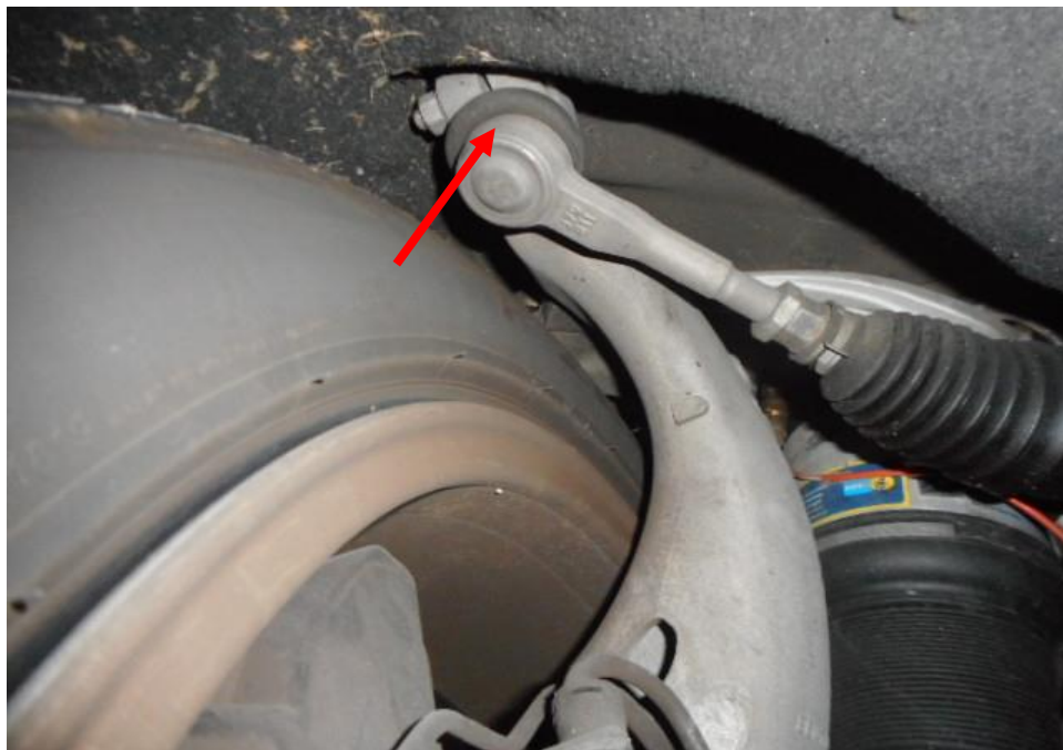
Photo 18 shows the various undercarriage components at the front left wheel of the Motor Car, in particular the steering tie rod end (arrowed). The various Undercarriage components of the Motor Car were all found to be intact without any visible damage. There was also no sign of fluid stain(s) observed on the various undercarriage components.
