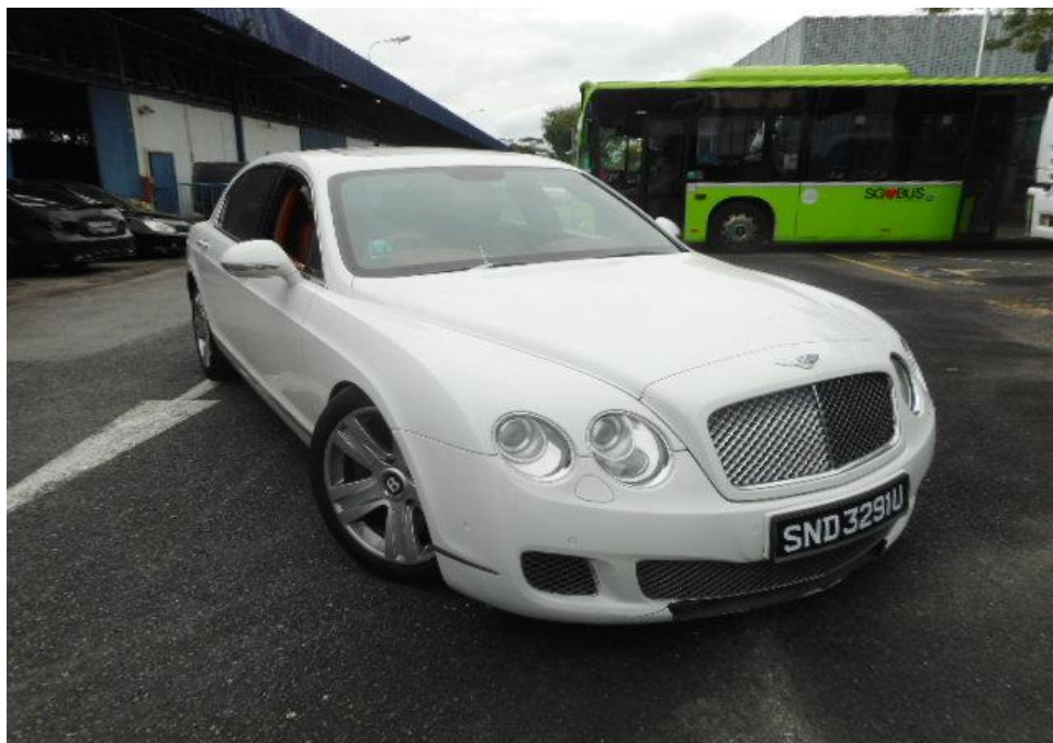
Photo 24 shows the front right wheel of the Motor Car turned to its full left. During my steering system test, I did not experience any abnormal free play and/or resistance when I had turned the steering wheel towards full left and full right. This would suggest that the steering system of the Motor Car was likely to be in serviceable condition at the material time of incident.
