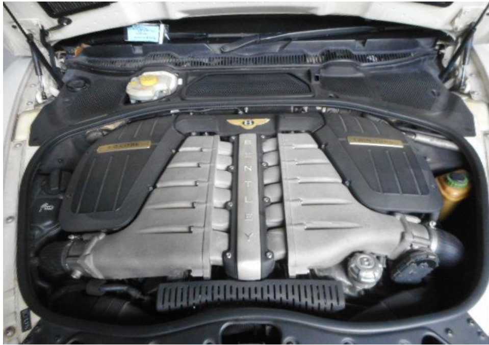
Photo 11 shows a general view of the Motor Car's engine compartment, which was accessed by lifting the front cabin of the Motor Car. The various parts and components inside the engine compartment were unaffected by the incident. There was also no sign(s) or indication(s) of fresh fluid leakage and/or fluid stain within the engine compartment
