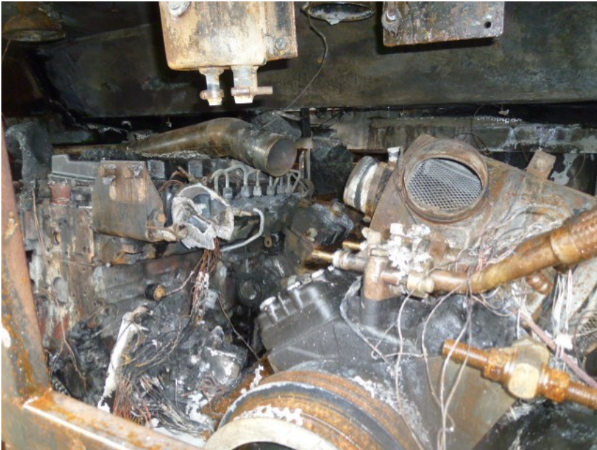
Upon closer examination of the area where the fire to the Insured Vehicle had likely started, we had found greenish residue on several stretches of original factory fitted wirings leading towards the Engine Control Module (ECM) of the Insured Vehicle.
