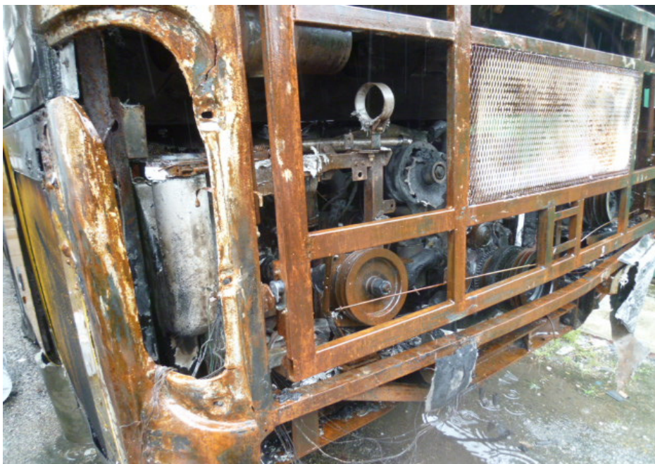
Photo 6 shows a general view of the engine compartment of the Insured Vehicle at the time of our inspection. The engine compartment of the Insured Vehicle was severely affected by the fire. Most of the parts inside the engine compartment were found to be completely burnt and/or melted as a result of the fire.
