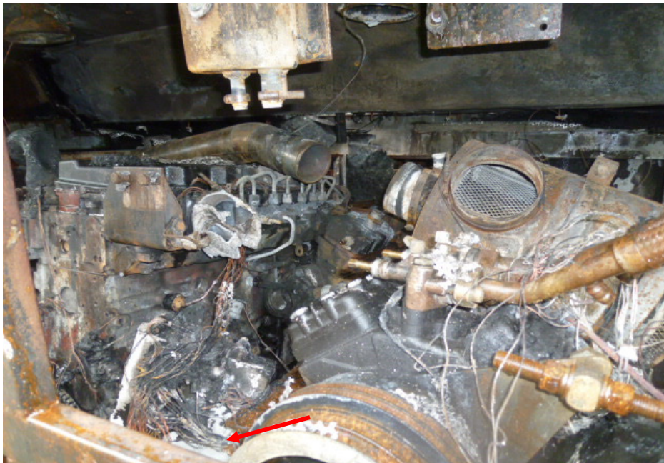
Photo 9 shows a closer view of the faint traces of greenish residue found on several burnt stretches of original factory fitted wirings leading from the ECM (arrowed) of the Insured Vehicle. The presence of such greenish residue indicates internal heating of copper wires, a sign of an electrical short circuit occurring. The greenish residue is normally left behind from oxidation as a result of chemical reaction involving the copper wires.
