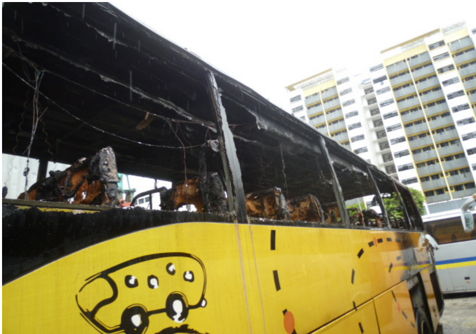
Photo 4 shows the general view of the top portion of the Insured Vehicle at the time of our inspection. The roof of the Insured Vehicle had sustained serious fire damage.
