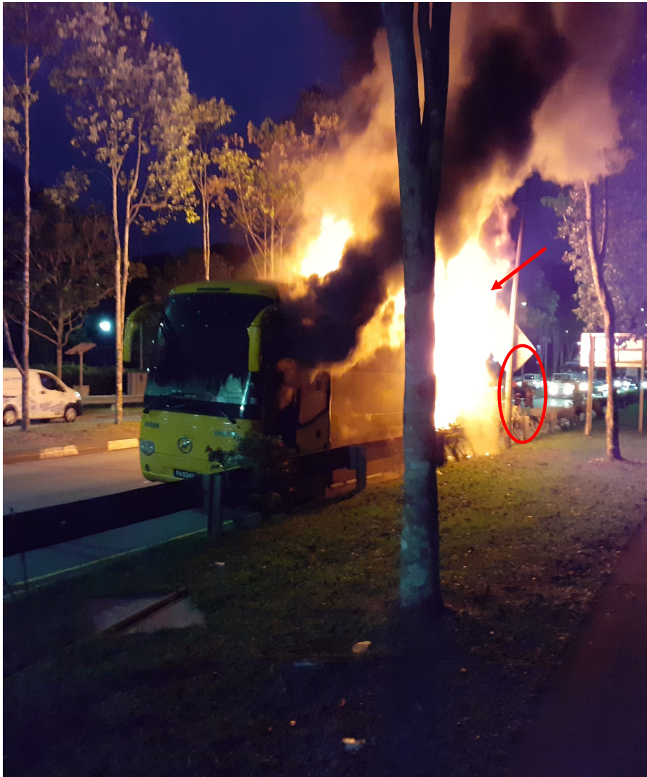
Photo 11 shows the SCDF having arrived at the incident location and attempting to put out the fire (circled). In general, the information gathered from this photograph had corresponded to Mr Ng's statement, which is the fire had started from the rear portion of the Insured Vehicle (arrowed).
