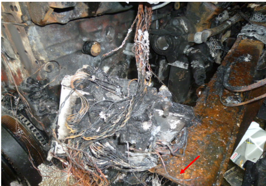
Photo 10 shows a close up view of the faint traces of greenish residue that was found on several burnt stretches of original factory fitted wirings leading from the ECM (arrowed) of the Insured Vehicle. This seems to suggest the occurrence of an electrical short circuit.
