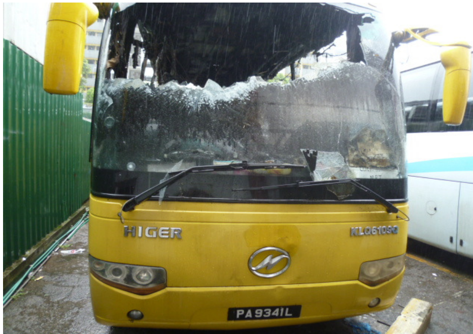
Photo 1 shows the general view of the frontal portion of the Insured Vehicle at the time of our inspection. The frontal portion of the Insured Vehicle was significantly affected by the fire.
