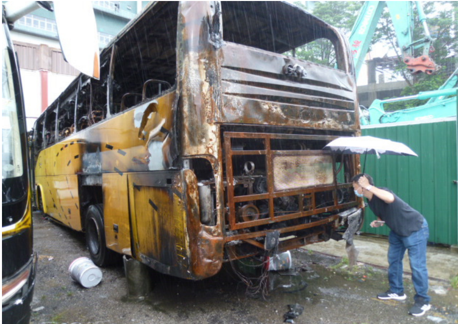
Photo 3 shows a closer view of the rear portion of the Insured Vehicle at the time of our inspection together with principal consultant Mr Lau. The fire damage was observed to be more severe at its rear portion.
