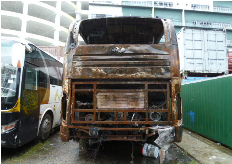
Photo 5 shows the general view of the rear portion of the Insured Vehicle at the time of our inspection. The Insured Vehicle had sustained severe fire damage at the rear portion.
