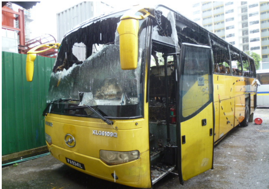
Photo 2 shows the general view of the left frontal portion of the Insured Vehicle at the time of our inspection. The exterior body of the Insured Vehicle had sustained fire damage at the top portion as well as rear portion. Affected parts had included the side mirrors, roof, windows, rear panels, both windscreens and engine panel, amongst others.
