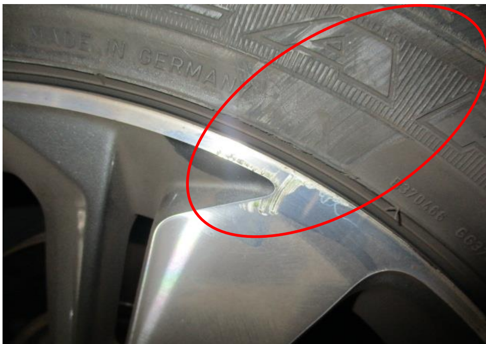
Photo 5 shows the close up view of the front left wheel rim and tyre of Car at the time of inspection. The front left wheel rim and tyre had sustained damages. It was also noted that there were scratched marks and paint transfer marks (circled) on it.
