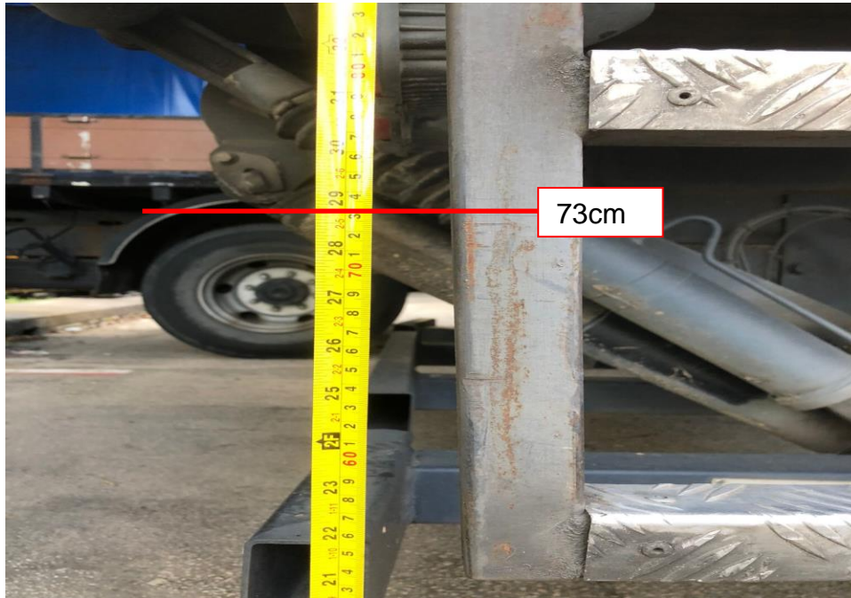
Photo 17 shows the close up view of the height measurement being conducted on the rear right portion of Insured Vehicle. The height above ground level of where the scratched marks damage that were found from the front bumper left portion, the front left wheel rim and tyre and the front left fender of the Car was between 53cm to 73cm as compared to the rear right portion of the Insured Vehicle.
