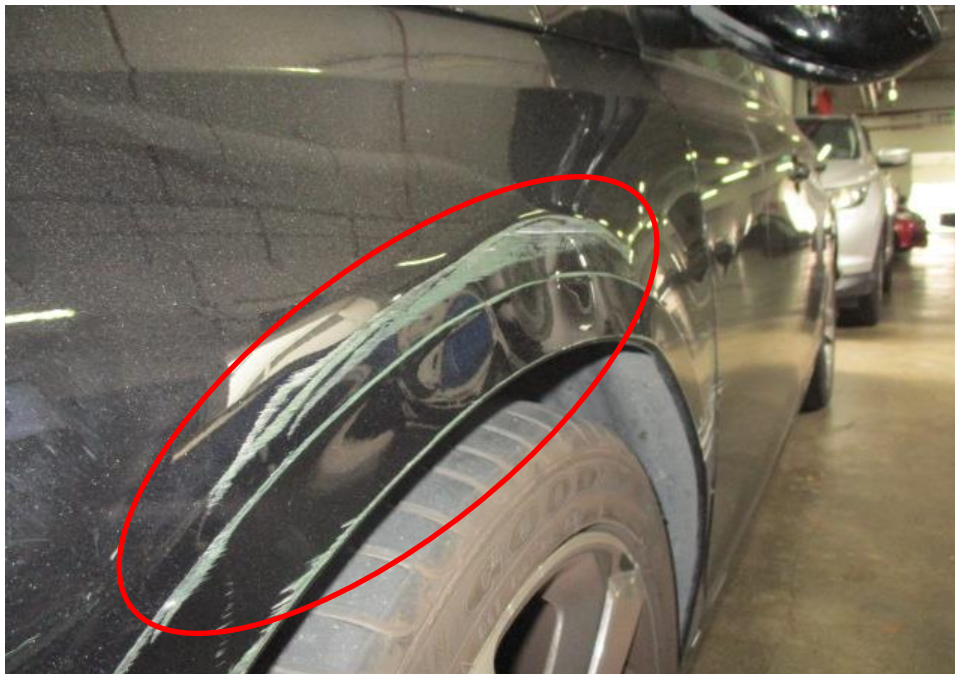
Photo 4 shows the close up view of the front left fender portion of Car at the time of inspection. The front left bumper portion had been damaged. It was also noted that there were scratched marks and paint transfer marks (circled) on it.
