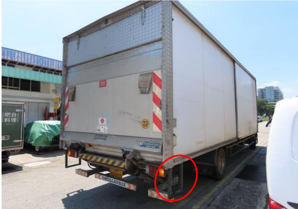
Photo 7 shows the general view of the right-side rear portion of Insured Vehicle at the time of inspection. We are of the opinion that the possible point of contact of Insured Vehicle would be at its right side rear portion (circled) since Insured Vehicle was on the left side and in front of the Car and drove into the Car from the left side at the mentioned point of collision.
