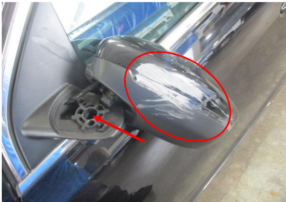
Photo 6 shows the close up view of the front left rear view mirror of Car at the time of inspection. The front left rear view mirror had been damaged. It was also noted that there were scratched marks and paint transfer marks (circled) and it was dislodged off (arrowed).
