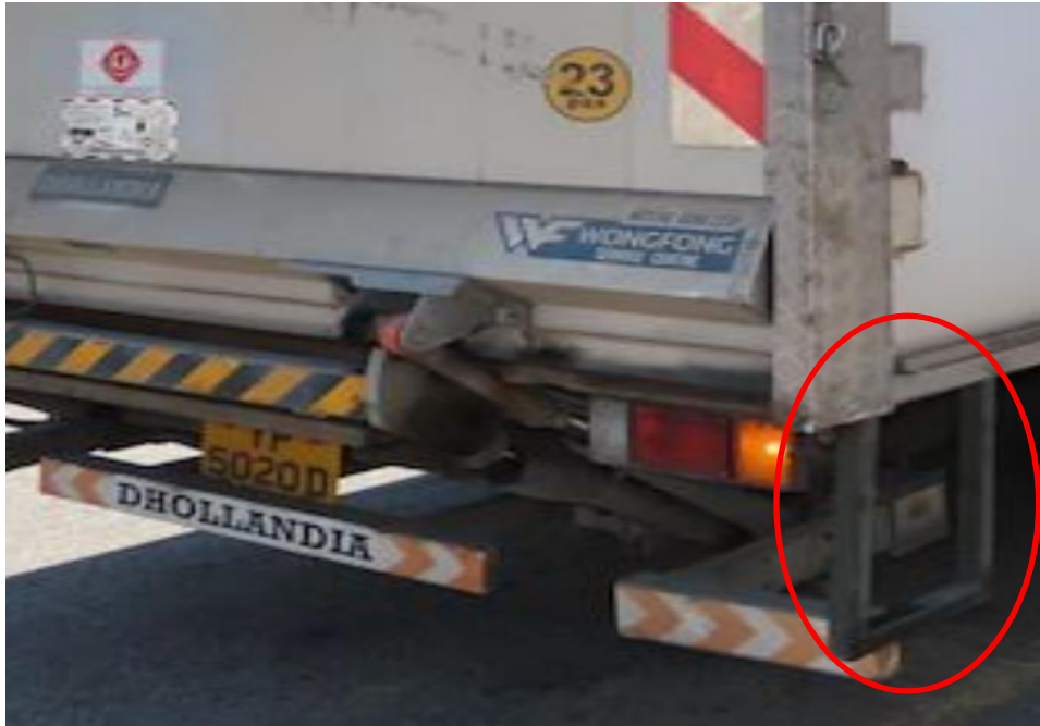
Photo 8 shows the close up view of the right side rear portion of Insured Vehicle at the time of inspection. We are of the opinion that the possible point of contact of Insured Vehicle would be at its right side rear portion (circled) since Insured Vehicle was on the left side and in front of the Car and drove into the Car from the left side at the mentioned point of collision.
