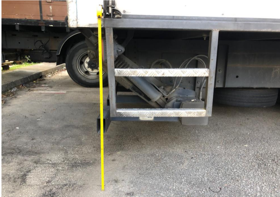
Photo 15 shows the general view of the height measurement being conducted on the rear right portion of Insured Vehicle. The height above ground level from 53cm to 73cm and 99cm to 102cm is where the possible damages height of the Car compared to the Insured Vehicle.
