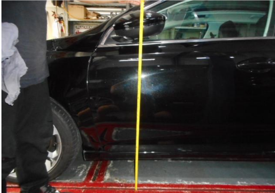
Photo 13 shows a general view of the height measurement being conducted on the front left portion of Car. The front left rear view mirror where the scratched marks is was measured to be at 99cm to 102cm above ground level.
