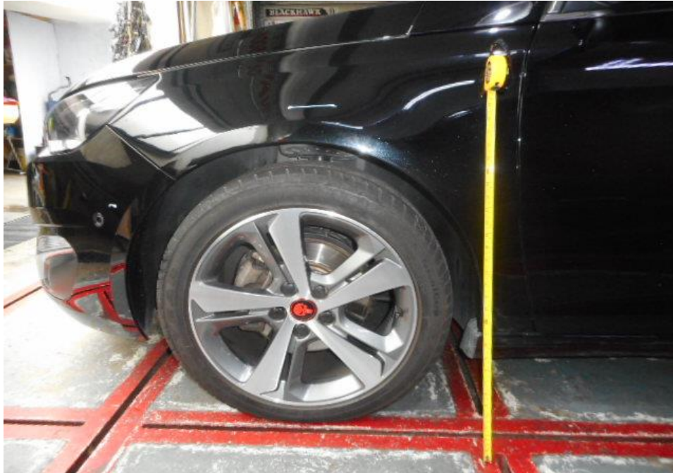
Photo 9 shows a general view of the height measurement being conducted on the front left portion of Car. The front bumper left portion to the front left fender where the scratched marks is was measured to be from 53cm to 73cm above ground level.
