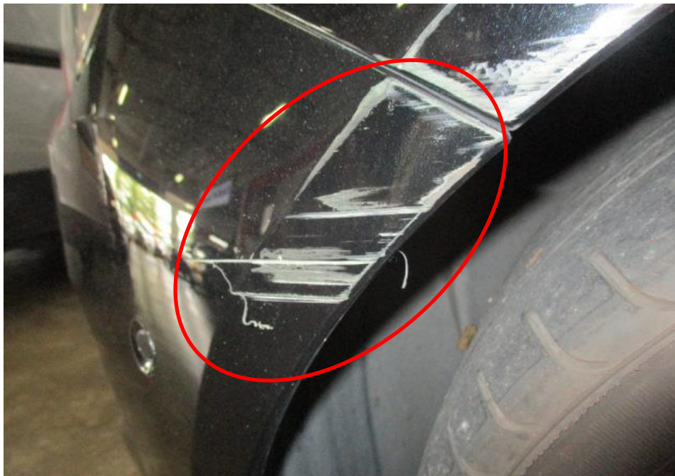
Photo 3 shows the close up view of the front bumper left portion of Car at the time of inspection. The front bumper left portion had been damaged. It was also noted that there were scratched marks and paint transfer marks (circled) on it.
