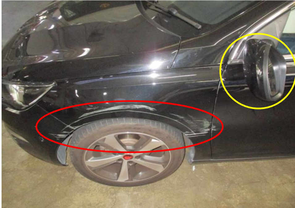
Photo 2 shows the close up view of the front left portion of Car at the time of inspection. The front bumper left portion, front left fender and front left rear view mirror had been damaged. It was also noted that there were scratched marks and paint transfer marks on the front bumper left portion, front left fender, front left wheel rim and tyre (red circle) as well as its left rear view mirror (yellow circle) was also scratched and dislodged off the Car.
