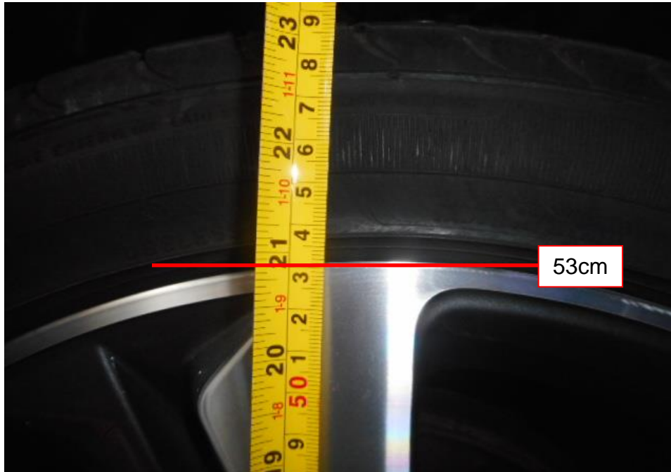
Photo 11 shows the close up view of the height measurement being conducted on the front left wheel rim and tyre portion of Insured Vehicle. The front left wheel rim and tyre where the scratched marks is was measured to be from 53cm to 73cm above ground level.
