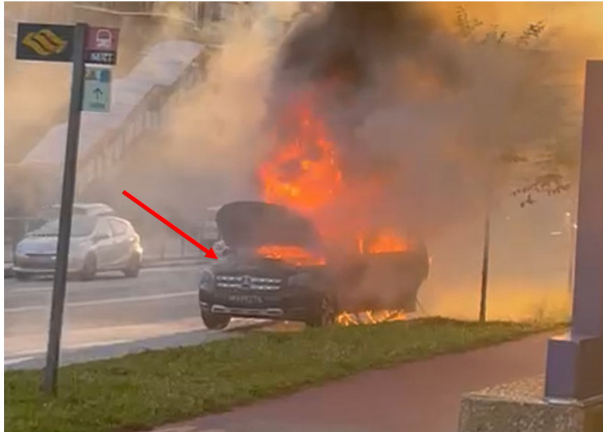
Photo 8 shows the Insured Vehicle at the incident scene (screenshot extracted from the video recording provided by Madam Quek). No fire was seen from the engine compartment area (red arrow) of the Insured Vehicle at the initial stage of the fire. In fact, the frontal portion of the Insured Vehicle was seen to be unaffected even after the fire started spreading.
