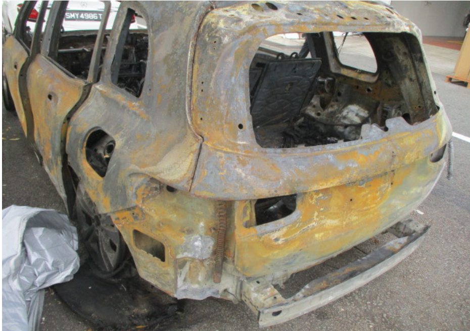
Photo 5 shows the rear left body of the Insured Vehicle. The Insured Vehicle was observed to have sustained extensive fire damage all around. The body panels at the rear portion and the undercarriage components at the rear underside were all severely burnt.
