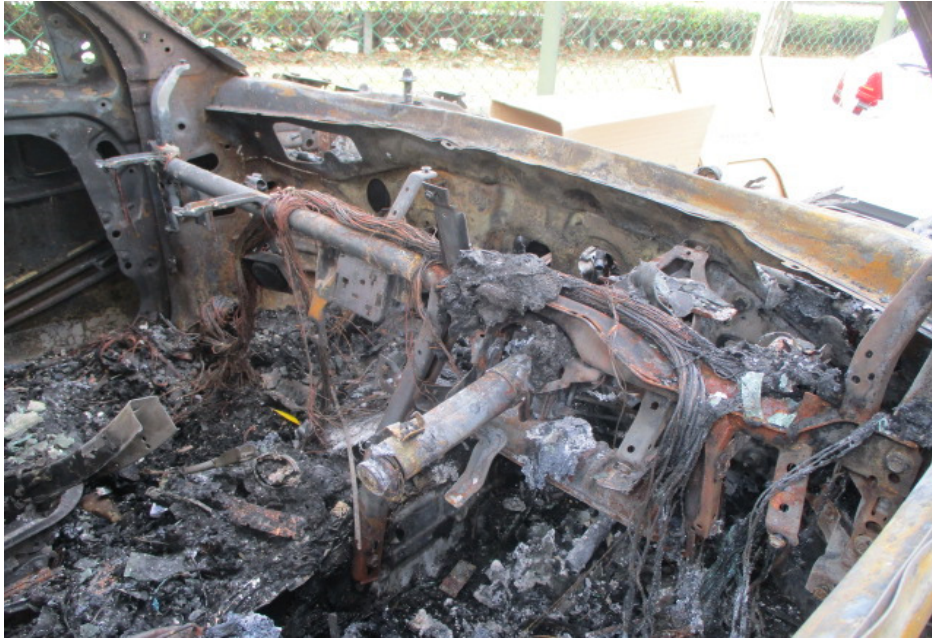
Photo 10 shows the front dashboard area of the Insured Vehicle at the time of my inspection. The fire to the Insured Vehicle was likely to be of electrical nature (electrical fault) originating from one or more of the wirings located behind the front dashboard of the Insured Vehicle. However, given that the wirings behind the front dashboard were all completely burned to its bare copper state, I was not able to determine the electrical fault had occurred along which wiring(s).
