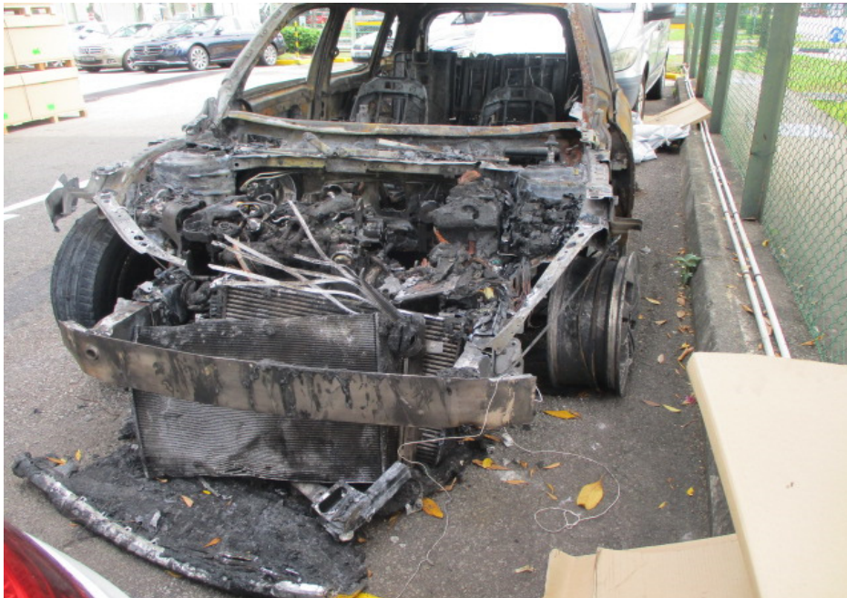
Photo 2 shows a general view of the front left body of the Insured Vehicle at the time of inspection. The Insured Vehicle was observed to have sustained extensive fire damage all around. The body panels at the frontal portion and the undercarriage components at the front underside were all severely burnt.
