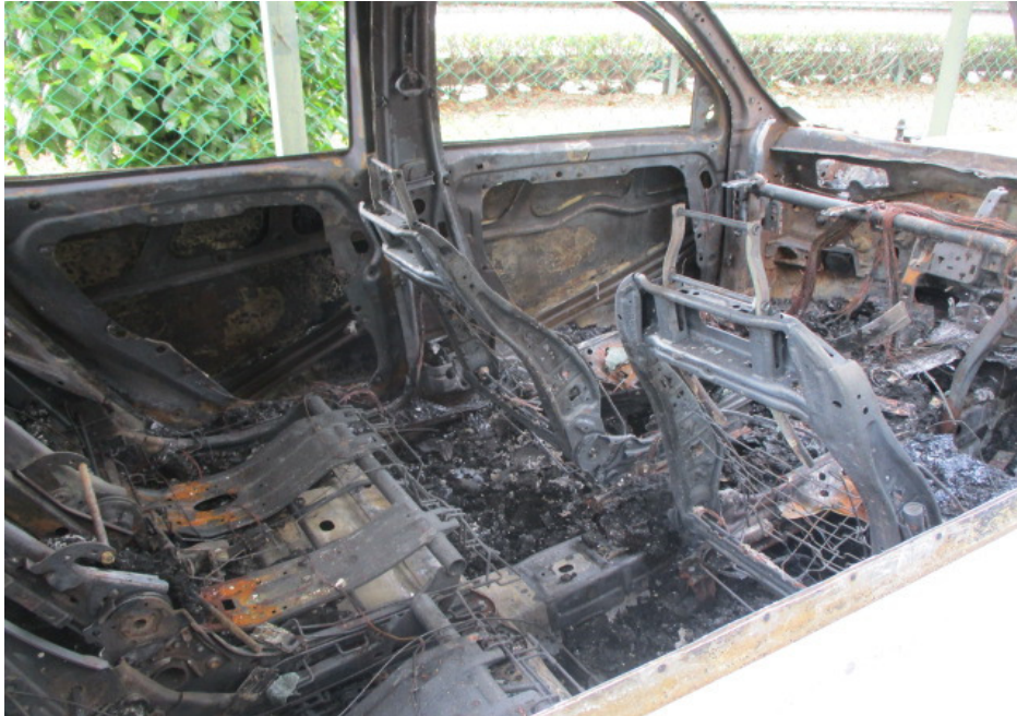
Photo 3 shows the interior compartment of the Insured Vehicle. All the parts inside the interior compartment were found to be extensively burnt. Its front seats, rear seats, roof upholstery, carpet and various trims were all burnt and/or melted as a result of the fire, leaving skeletal remains.
