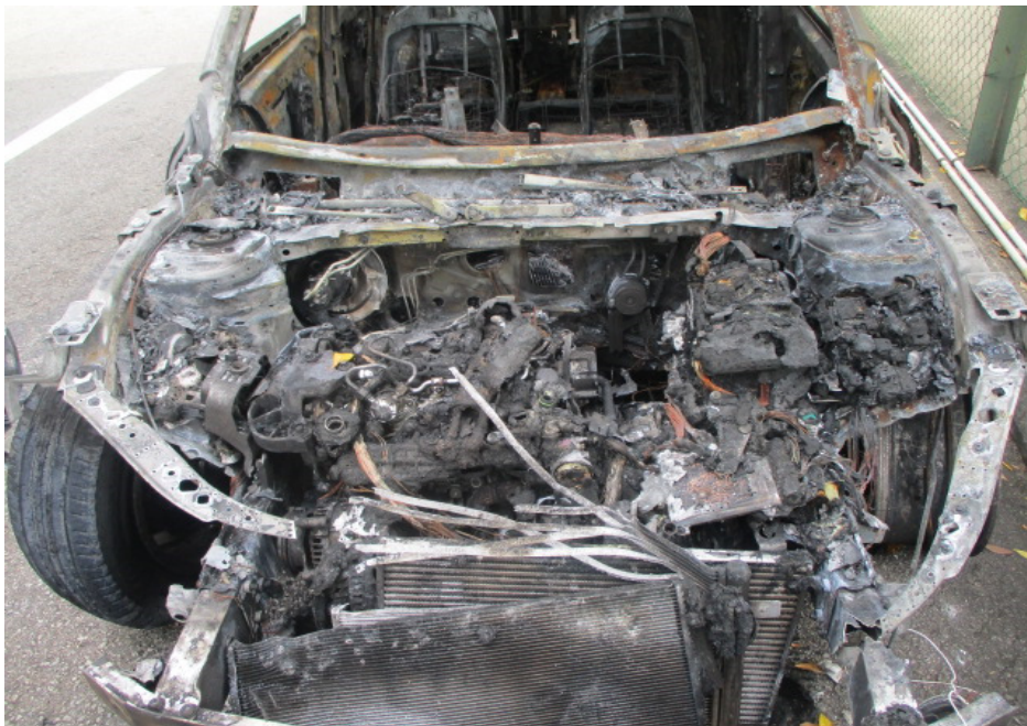
Photo 4 shows a general view of the Insured Vehicle's engine compartment. The various parts and components within the engine compartment of the Insured Vehicle were all extensively affected by the fire. This had included the engine and transmission of the Insured Vehicle.
