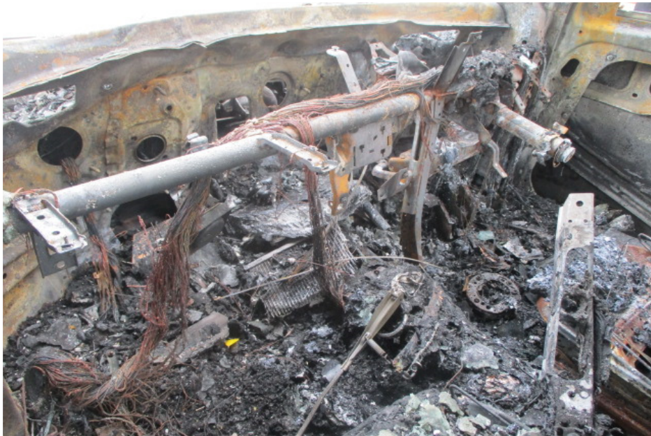
Photo 11 shows another view of the front dashboard area of the Insured Vehicle at the time of my inspection. The wirings behind the front dashboard of the Insured Vehicle were all completely burned to its bare copper state. Because of this, I was not able to determine the electrical fault had occurred along which wiring(s).
