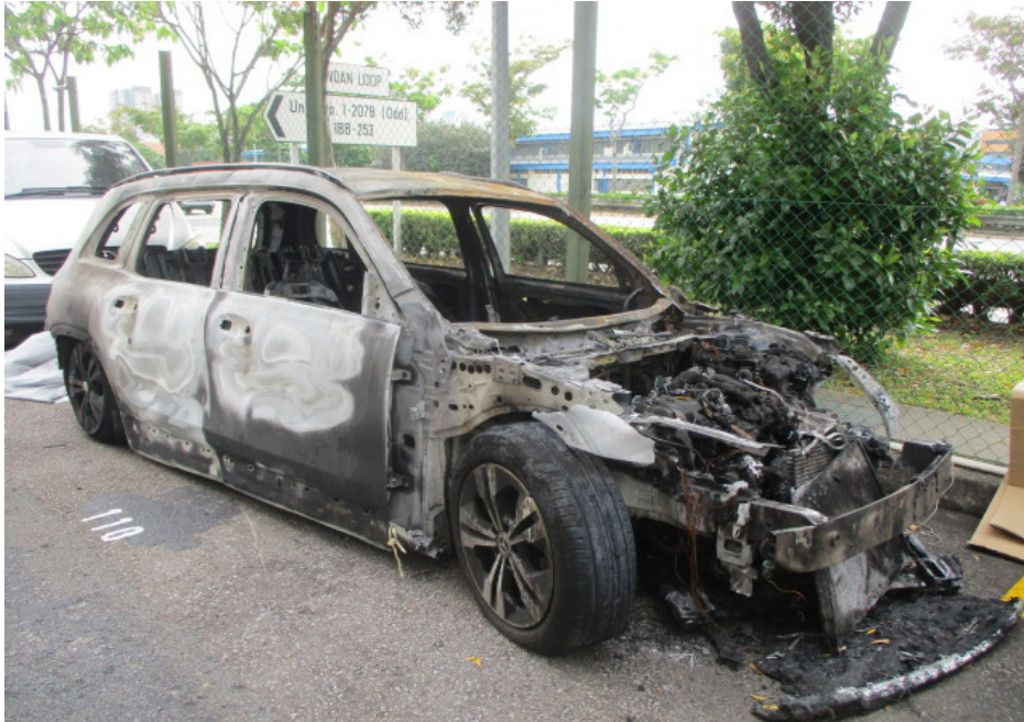
Photo 1 shows a general view of the front right body of the Insured Vehicle at the time of inspection. The Insured Vehicle was observed to have sustained extensive fire damage all around. The body panels at the frontal portion and the undercarriage components at the front underside were all found to have been severely burnt.
