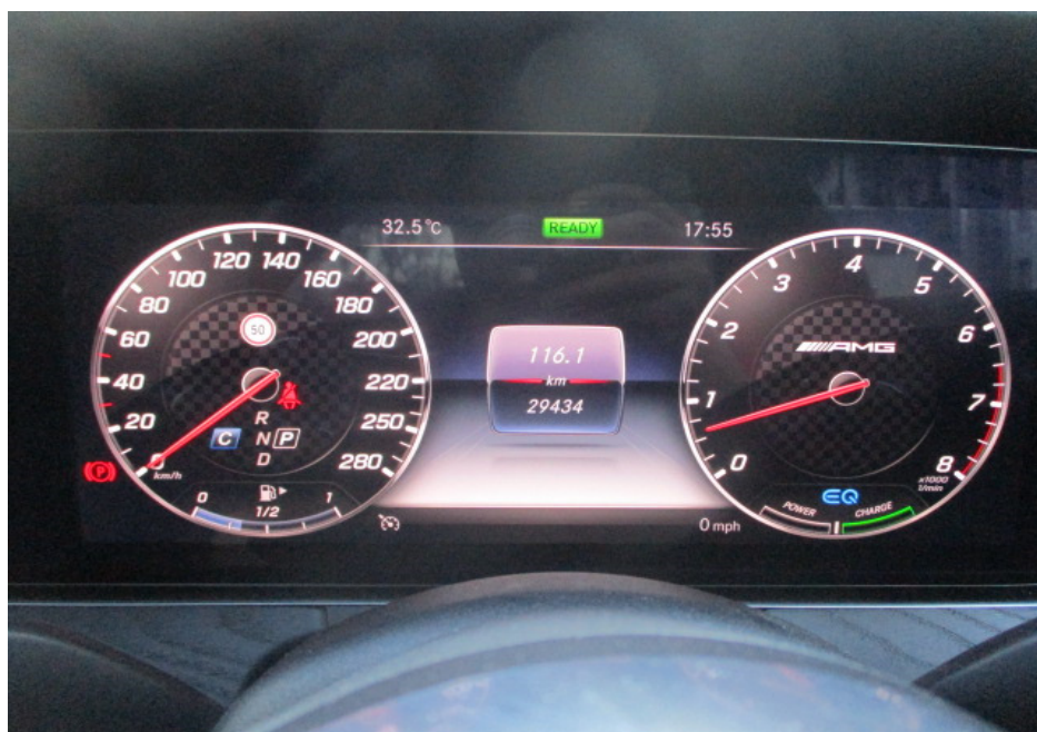
Photo 20 shows the respective warning lights no longer illuminated, indicating that there is no fault detected to the ABS, SRS, EPS, TPM and TCS systems of the Motor Car during the self-test. These electronic systems were hence in working condition at the time of my inspection.
