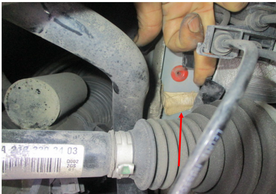
Photo 31 shows the chassis/structural body at the underside front right of the Motor Car. The original factory sealant (arrowed) at the joints along the chassis/structural body was observed to be untouched. In general, I had found no work was carried out on the chassis/structural body of the Motor Car. The chassis/structural body of the Motor Car was originally fitted.
