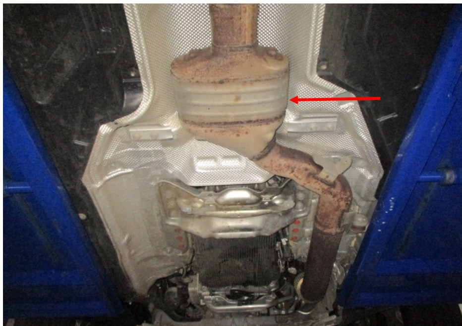
Photo 27 shows the front section of the Motor Car's exhaust system. My examination of the Motor Car's exhaust system revealed no sign(s) or indication(s) of any cut or weld marks along its exhaust pipes, on its rear mufflers, on its centre resonator box (arrowed) and on its catalytic converter.
