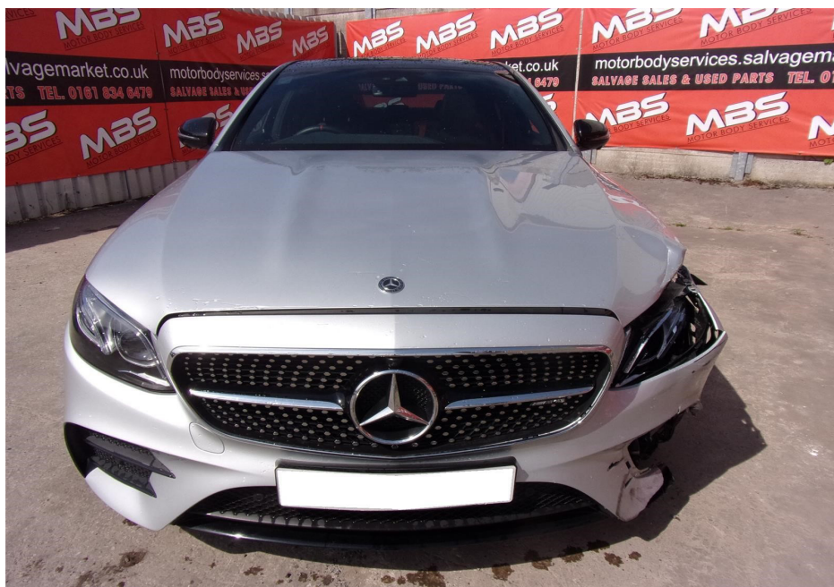
Photo 2 shows the frontal body of the Motor Car (photograph provided to me). The photographs provided to me had showed damage to the front left portion of the Motor Car. The front bumper, front bumper left lower grille, front bonnet and front left headlamp were amongst the body parts that were observed to have been damaged.
