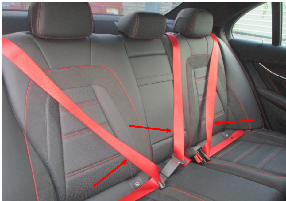
Photo 18 shows the rear seats of the Motor Car. All the seats of the Motor Car were secured via seat rails to the floorboard. They were also fitted with a retractable seat belt reel and a pre-tensioner. The seat belts (arrowed) were tested and were able to be fastened into the respective pre-tensions that were fitted on the side of each individual seat.
