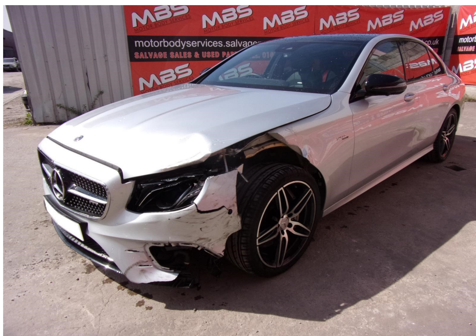
Photo 1 shows the front left body of the Motor Car (photograph provided to me). The photographs provided to me had showed damage to the front left portion of the Motor Car. The front bumper, front bumper left lower grille, front bumper left sensor, front bonnet, front left headlamp, front left fender and front left fender inner shield were amongst the body parts that were observed to have been damaged.
