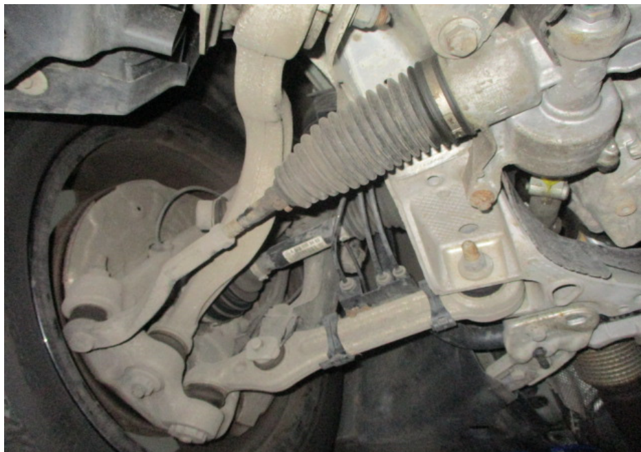
Photo 25 shows the various undercarriage components at the front right wheel of the Motor Car. The mechanical components, control arms and linkages were all found to be intact and secured in an appropriate manner. I also did not observe any fluid leak and/or fluid stain on the underside of the Motor Car.
