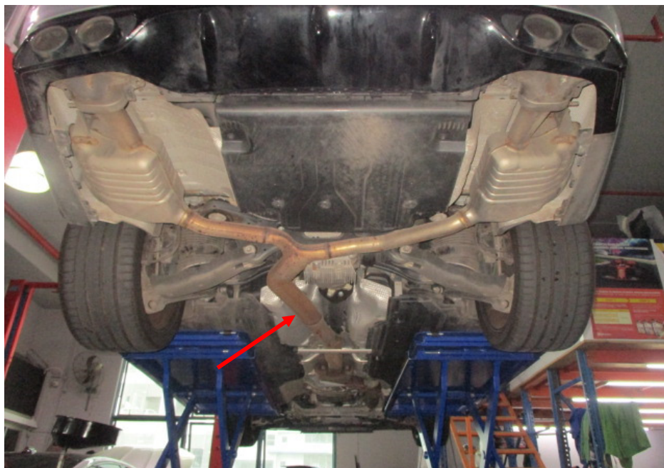
Photo 26 shows the rear section of the Motor Car's exhaust system. My examination of the Motor Car's exhaust system revealed no sign(s) or indication(s) of any cut or weld marks along its exhaust pipes (arrowed), on its rear mufflers, on its centre resonator box and on its catalytic converter.
