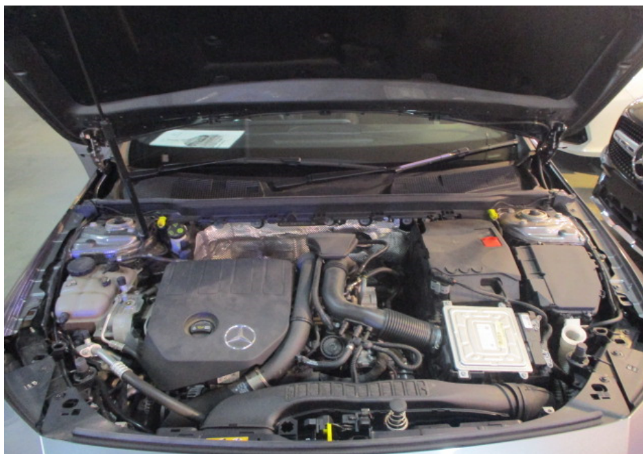
Photo 16 shows a general view of the engine compartment of the Motor Car at the time of my inspection. The various parts and components inside the engine compartment were all observed to be intact and properly fitted. There was also no sign(s) or indication(s) of fluid leak and/or fluid stain found inside the engine compartment.
