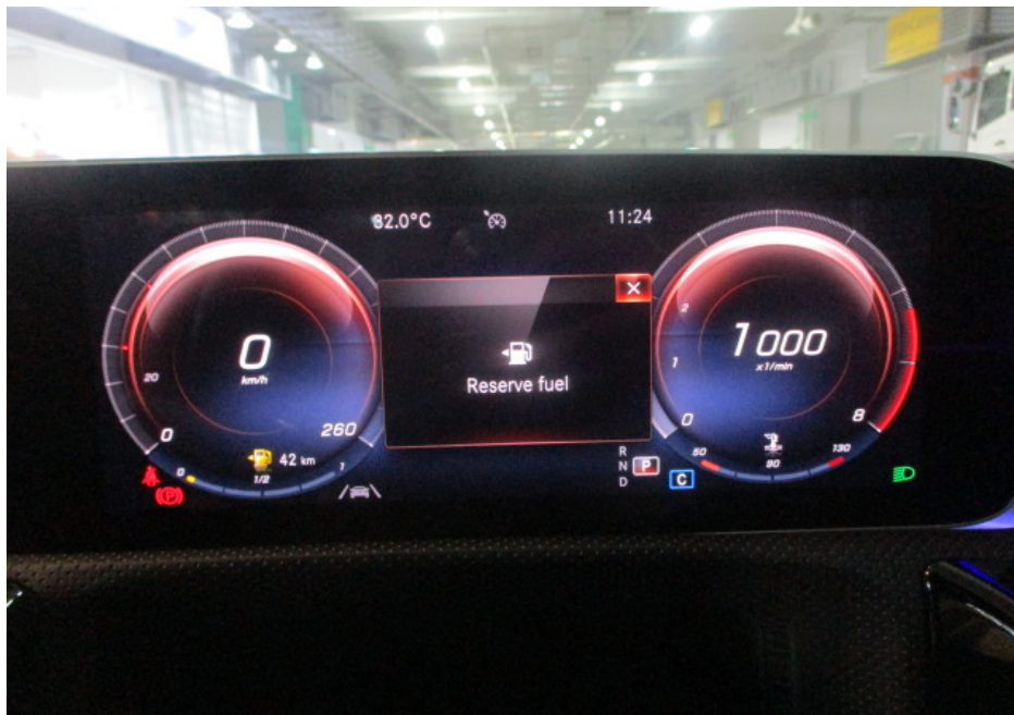
Photo 20 shows the respective warning lights no longer illuminated, indicating that there is no fault detected to the ABS, SRS, EPS and TCS systems of the Motor Car during the self-test. These electronic systems were hence in working condition at the time of my inspection.
