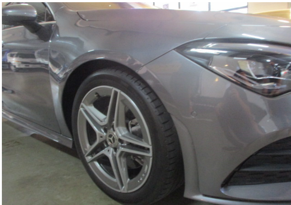
Photo 7 shows a closer view of the Motor Car's front bumper, front right headlamp, front right wheel rim and front right fender at the time of my inspection. The body parts at the right side portion of the Motor Car were visually examined and it was observed that the repair/restoration works carried out to the damaged area of the Motor Car (refer to photograph 1 & 2 above) were reasonably adequate and in order.
