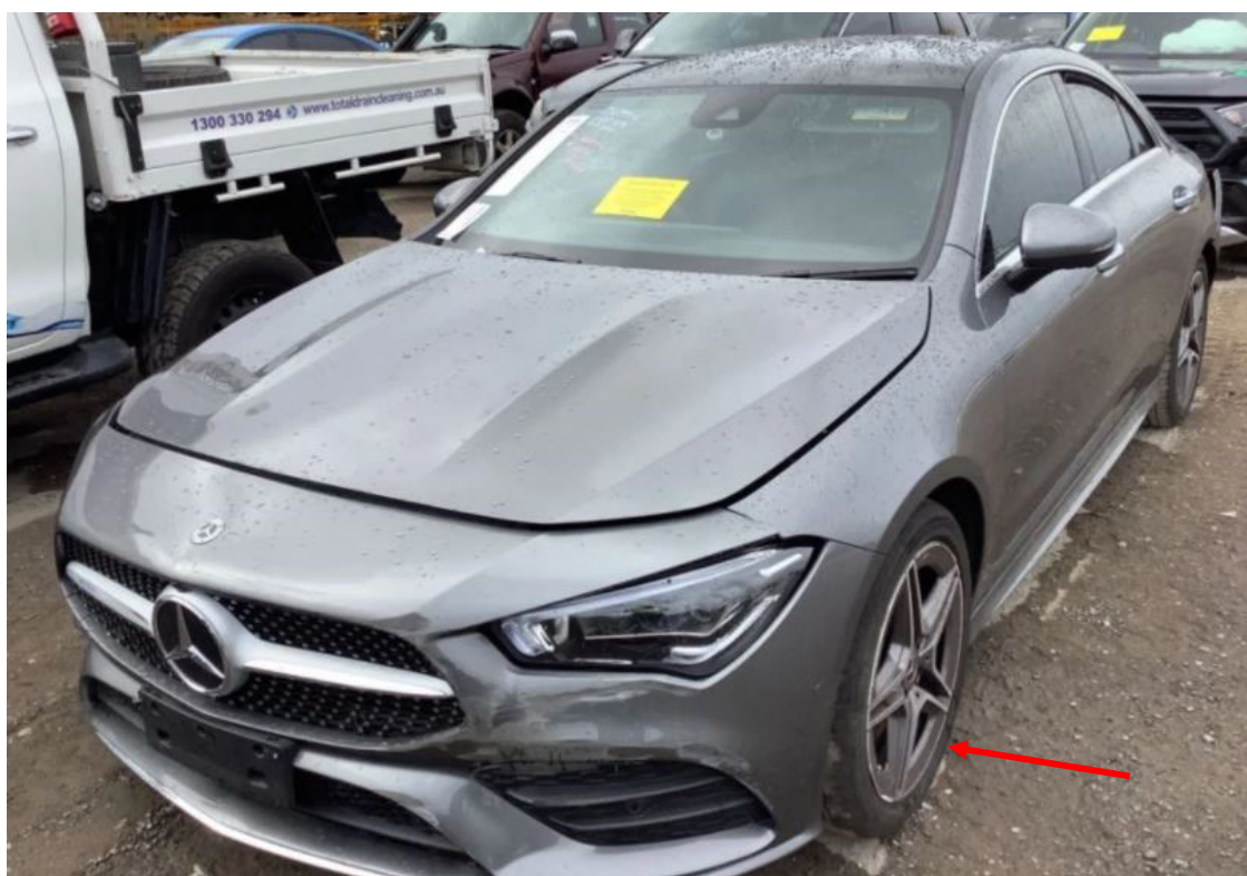
Photo 4 shows the front left body of the Motor Car (photograph provided to me). Marks of grazing nature were also seen at the left side of the Motor Car's front bumper. The orientation of the Motor Car's front left wheel (arrowed) as compared to the orientation of the front right wheel (refer to photograph 1 above) indicates damage to the front right undercarriage parts of the Motor Car.
