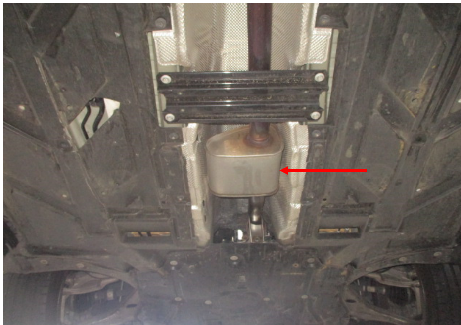
Photo 27 shows the front section of the Motor Car's exhaust system. My examination of the Motor Car's exhaust system revealed no sign(s) or indication(s) of any cut or weld marks along its exhaust pipes, on its rear muffler, on its centre resonator box (arrowed) and on its catalytic converter.
