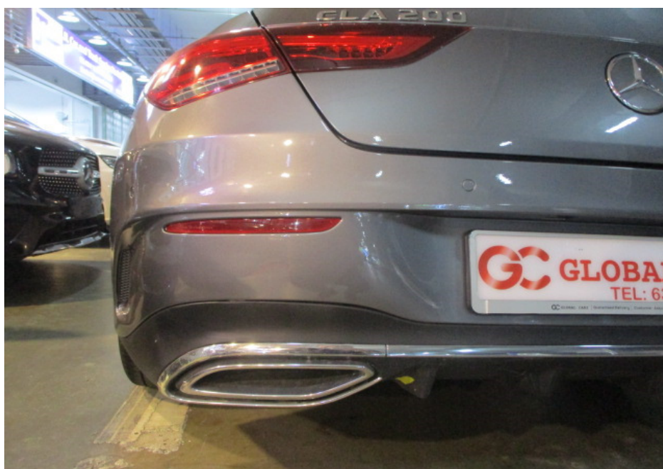
Photo 12 shows a closer view of the Motor Car's rear bumper, rear bumper lower cover, rear bumper lower chrome moulding and rear left taillamp at the time of my inspection. The body parts at the rear left portion of the Motor Car were visually examined and it was observed that the repair/restoration works carried out to the damaged area of the Motor Car (refer to photograph 3 above) were reasonably adequate and in order.
