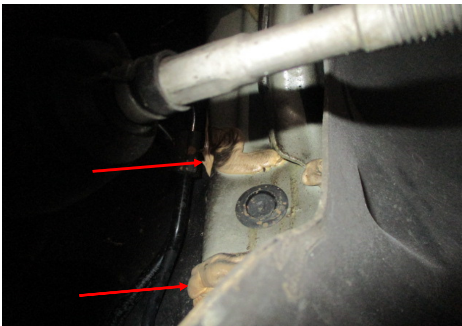
Photo 30 shows the chassis/structural body at the underside front left of the Motor Car. I did not find any weld marks other than original spot weld marks on the chassis/structural body of the Motor Car. The original factory sealant (arrowed) at the joints along the chassis/structural body was untouched, indicating no work was done on the chassis/structural body of the Motor Car and that the chassis/structural body was originally fitted.
