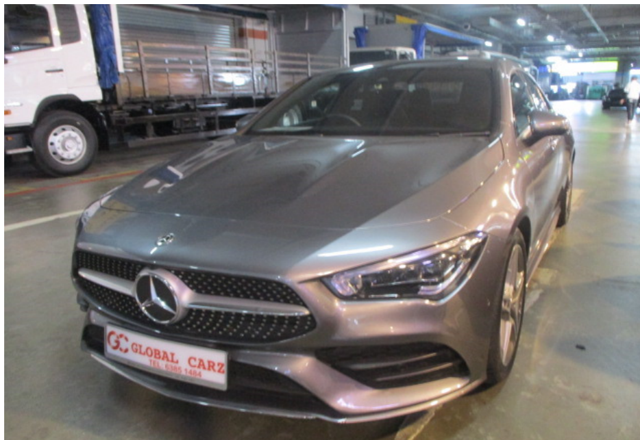
Photo 14 shows a general view of the front left body of the Motor Car at the time of my inspection. The Motor Car was observed to be in a relatively good general condition with no loose exterior fittings observed. The body parts at the front left portion of the Motor Car were visually examined and it was observed that the repair/restoration works carried out to the damaged area of the Motor Car (refer to photograph 4 above) were reasonably adequate and in order.
