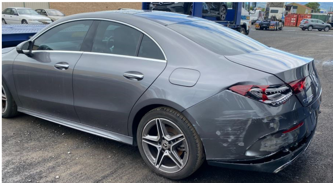
Photo 3 shows the rear left body of the Motor Car (photograph provided to me). Apart for the right side portion, I had also observed damage to the rear left portion of the Motor Car. The rear bumper, rear bumper lower cover, rear bumper lower chrome moulding, rear left taillamp and rear left fender were amongst the body parts that were observed to have been damaged.
