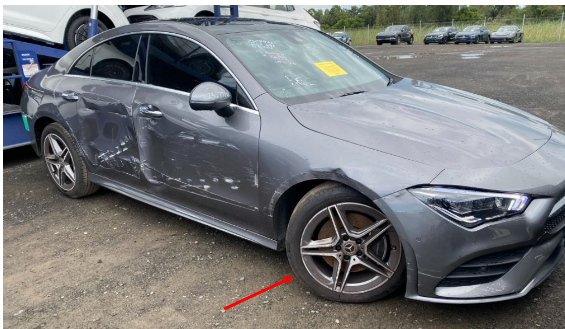
Photo 1 shows the front right body of the Motor Car (photograph provided to me). The photographs provided to me had showed damage to the right side portion of the Motor Car. The front bumper, front right fender, front right door, front right door handle, right wing mirror, rear right door and rear right fender were amongst the body parts that were observed to have been damaged. The orientation of the Motor Car's front right wheel (arrowed) as compared to the orientation of the front left wheel (refer to photograph 4 below) indicates damage to the front right undercarriage parts of the Motor Car.
