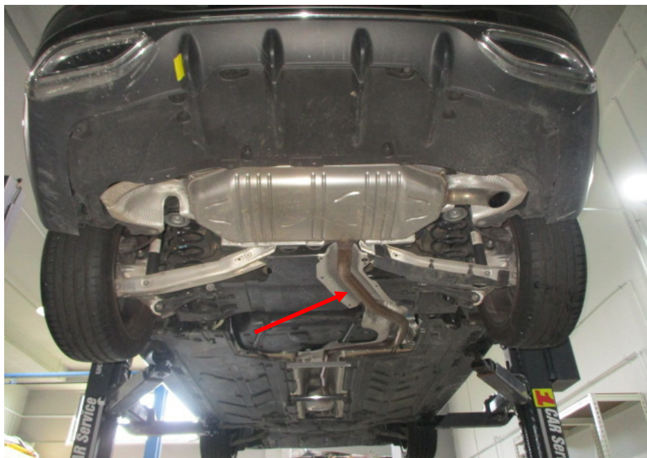
Photo 26 shows the rear section of the Motor Car's exhaust system. My examination of the Motor Car's exhaust system revealed no sign(s) or indication(s) of any cut or weld marks along its exhaust pipes (arrowed), on its rear muffler, on its centre resonator box and on its catalytic converter.
