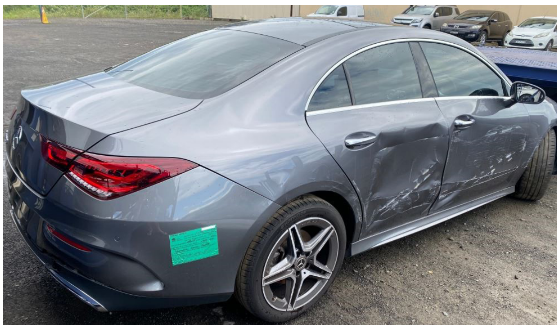
Photo 2 shows the rear right body of the Motor Car (photograph provided to me). The photographs provided to me had showed damage to the right side portion of the Motor Car. The front right door, front right door handle, right wing mirror, rear right door and rear right fender were amongst the body parts that were observed to have been damaged.
