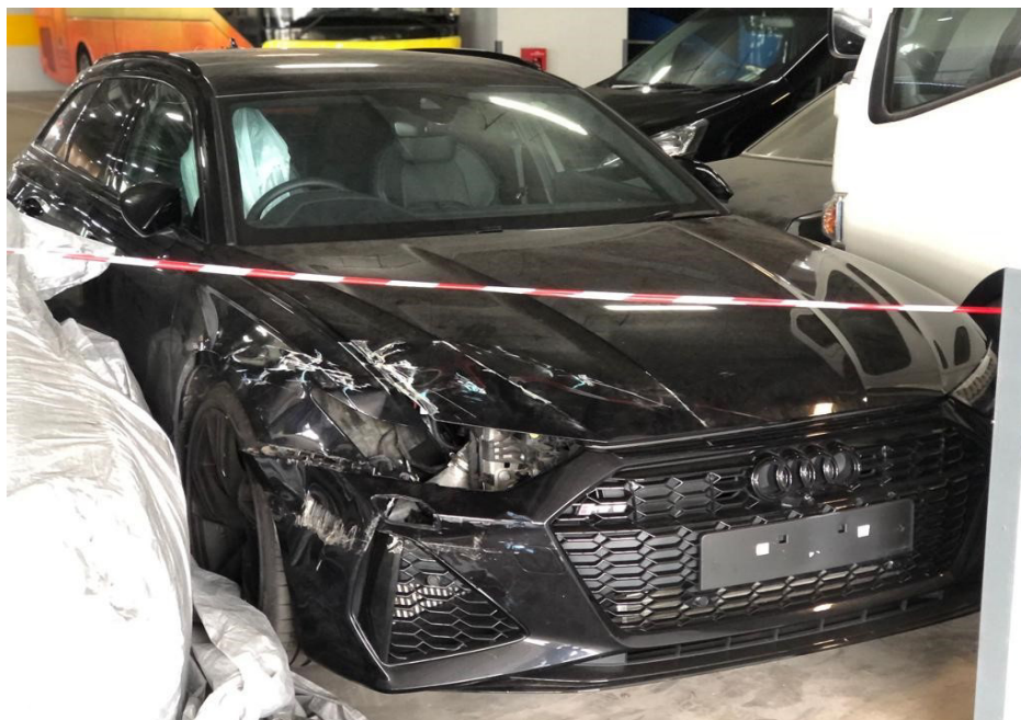
Photo 1 shows the front right body of the Motor Car (photograph provided to me). The photographs provided to me had showed damage to the front right portion of the Motor Car. The front bumper, front bumper right lower grille, front bumper tow hook cover, front bonnet and front right fender were amongst the body parts that were observed to have been damaged.
