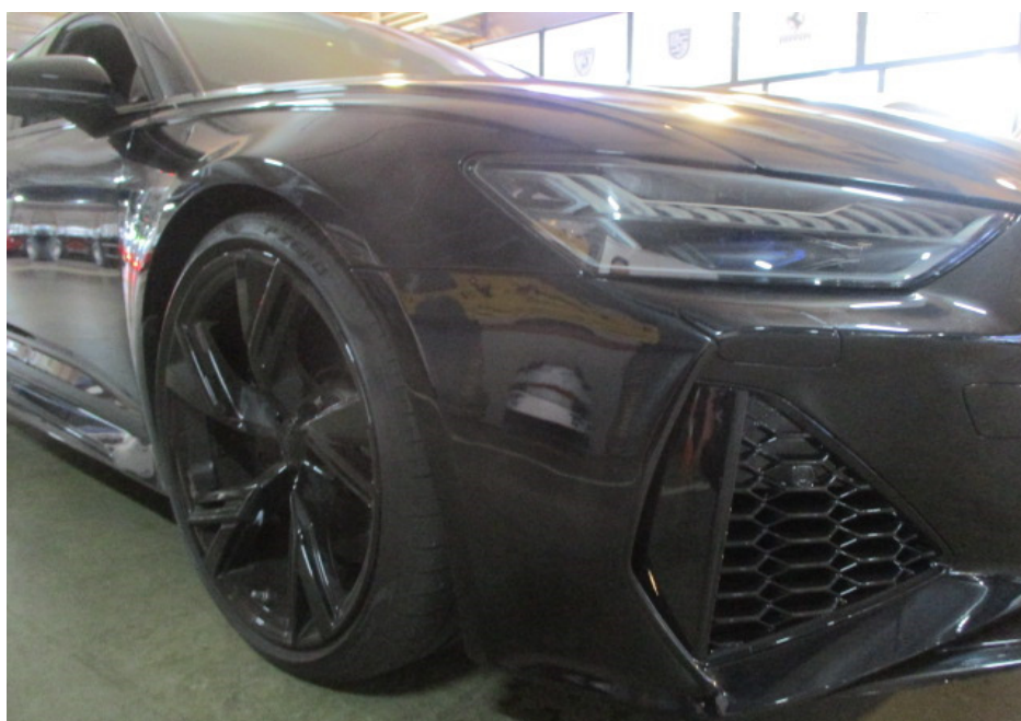
Photo 7 shows a closer view of the Motor Car's front bumper, front bumper right lower grille, front right headlamp and front right fender at the time of my inspection. The body parts at the front right portion of the Motor Car were visually examined and it was observed that the repair/restoration works carried out to the damaged area of the Motor Car (refer to photograph 1 & 2 above) were reasonably adequate and in order.
