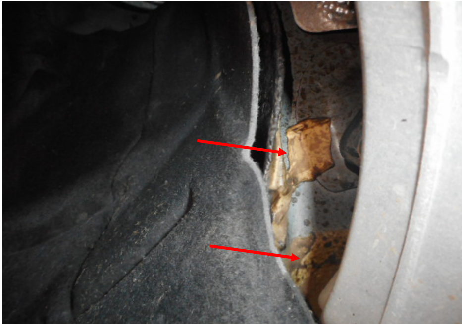
Photo 28 shows the chassis/structural body at the underside front right of the Motor Car. The original factory sealant (arrowed) at the joints along the chassis/structural body was observed to be untouched. In general, I had found no work was carried out on the chassis/structural body of the Motor Car. The chassis/structural body of the Motor Car was originally fitted.
