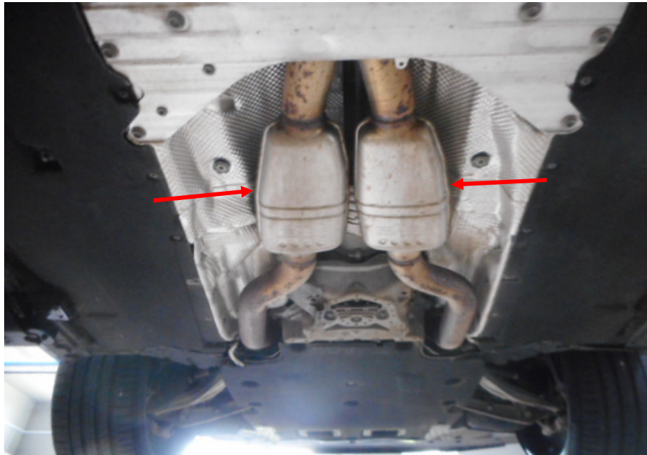
Photo 24 shows the front section of the Motor Car's exhaust system. My examination of the Motor Car's exhaust system revealed no sign(s) or indication(s) of any cut or weld marks along its exhaust pipes, on its rear muffler, on its centre resonator boxes (arrowed) and on its catalytic converters.
