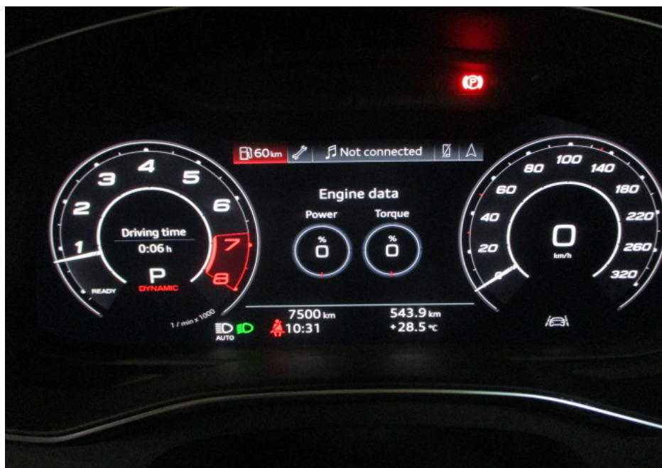
Photo 17 shows the respective warning lights no longer illuminated, indicating that there is no fault detected to the ABS, SRS, EPS, TPM and ESC systems of the Motor Car during the self-test. These electronic systems were hence in working condition at the time of my inspection.
