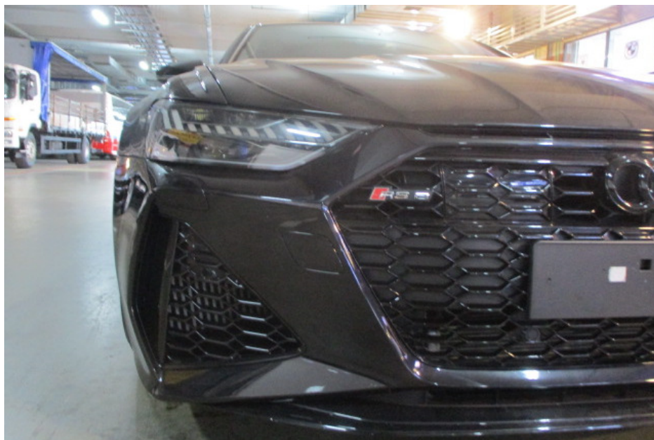
Photo 6 shows a closer view of the Motor Car's front bumper, front bumper right lower grille, front right headlamp and radiator grille at the time of my inspection. The body parts at the front right portion of the Motor Car were visually examined and it was observed that the repair/restoration works carried out to the damaged area of the Motor Car (refer to photograph 1 & 2 above) were reasonably adequate and in order.
