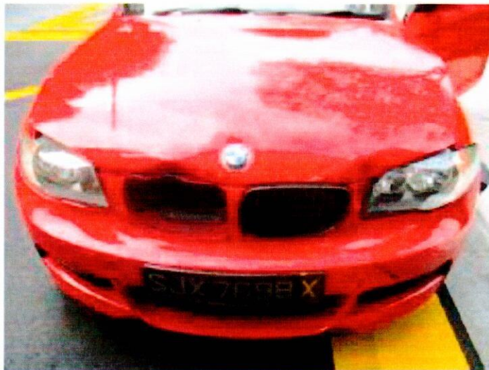
The civilian car's bonnet and engine cover of SJX 7698X sustained a small upwards dent.
