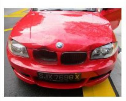
The civilian car's bonnet and engine cover of SJX 7698X sustained a small upwards dent.
