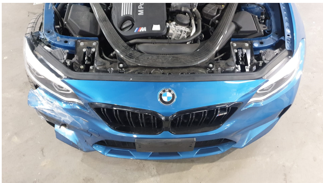
Photo 3 shows the engine compartment of the Motor Car (photograph provided to me). The various parts and components within the engine compartment were all intact and unaffected.
