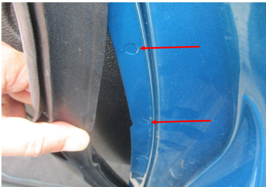
Photo 31 shows the right side "A" pillar of the Motor Car. I did not find any weld marks other than original spot weld marks (arrowed) on the right side "A" pillar of the Motor Car which, indicates that there was no re-welding works carried out. In general, I had found all the non-detachable body panels of the Motor Car to be originally fitted at the time of my inspection.
