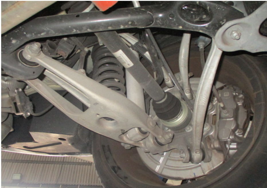
Photo 20 shows a general view of the control arms and linkages at the rear left wheel of the Motor Car. I did not observe any fluid leak and/or fluid stain on the underside of the Motor Car. All of the Motor Car's undercarriage components were observed to be intact and secured in an appropriate manner.
