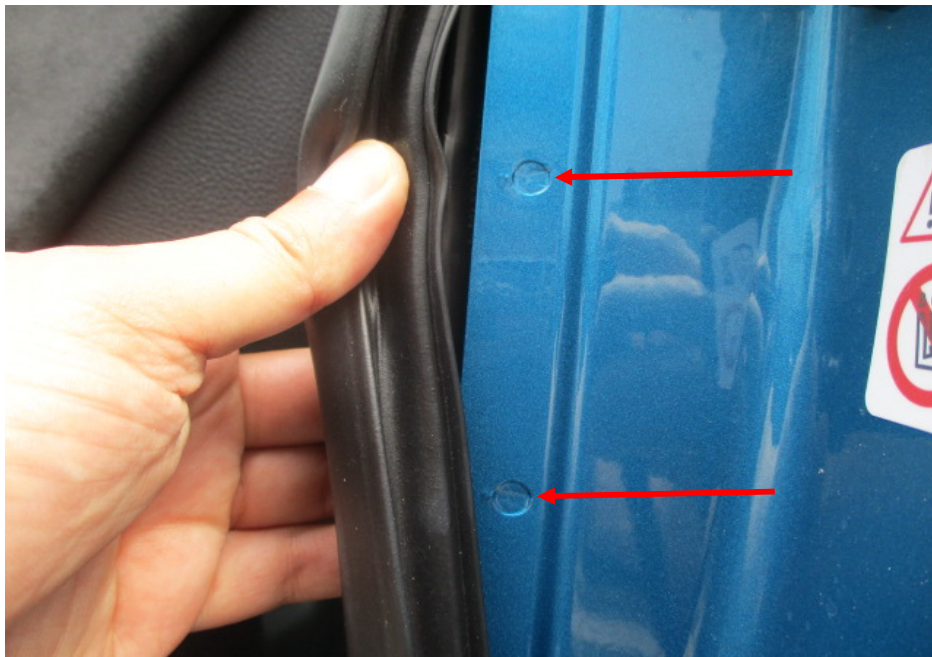
Photo 30 shows the rear left body panel of the Motor Car. I did not find any weld marks other than original spot weld marks (arrowed) on the rear left body panel of the Motor Car which, indicates that there was no re-welding works carried out. In general, I had found all the non-detachable body panels of the Motor Car to be originally fitted at the time of my inspection.
