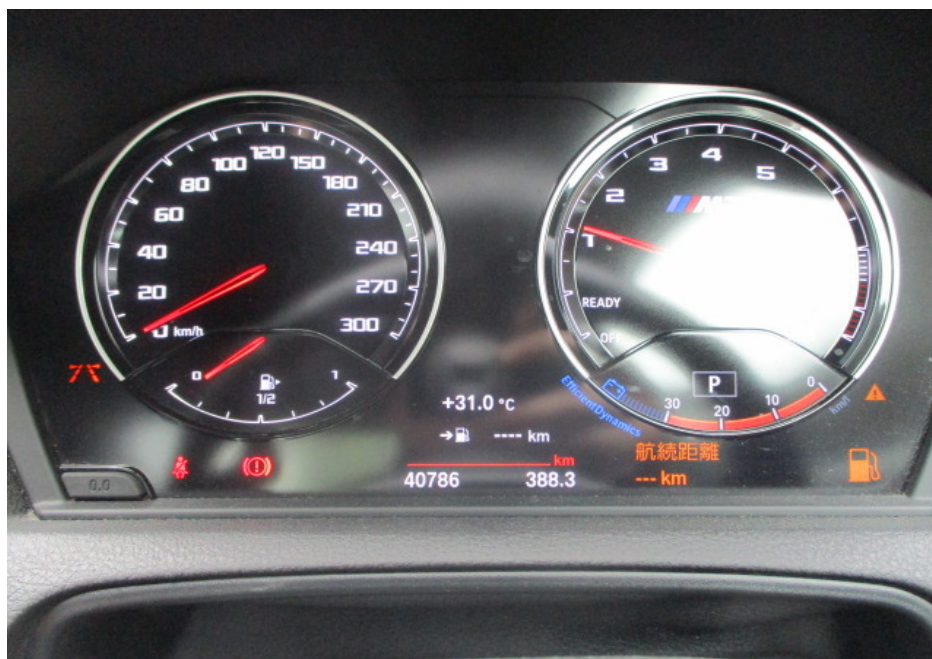
Photo 17 shows the respective warning lights no longer illuminated, indicating that there is no fault detected to the ABS, SRS, IAS, TPM and DSC systems of the Motor Car during the self-test. These electronic systems were hence in working condition at the time of my inspection.
