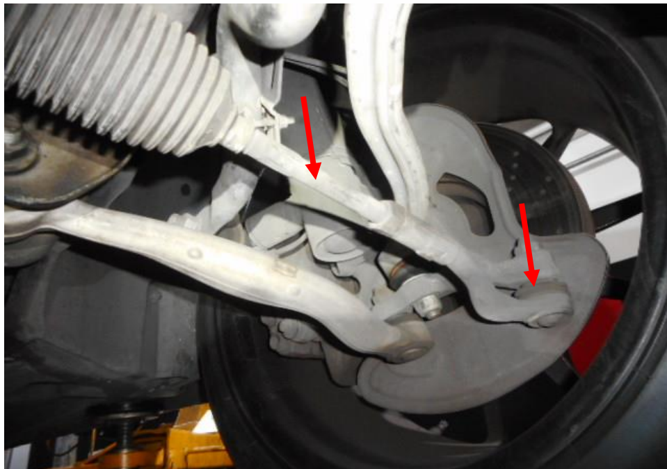
Photo 8 shows the close up view of the front right wheel of the Insured Vehicle at the time of our inspection. The steering tie rod (arrowed) is observed to be unaffected and by any signs of accident.
